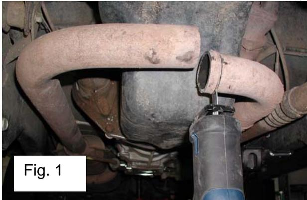
Federal (49-state)-emissions TJ with the second cut partially completed. After making both cuts, look into the larger (downstream) tube for any remnants of the end of the smaller tube – if there is a 'sliver' left, remove it with a pliers. When you re-weld the exhaust later, you will be able to slide the larger tube slightly over the smaller one for an overlapping fit.
