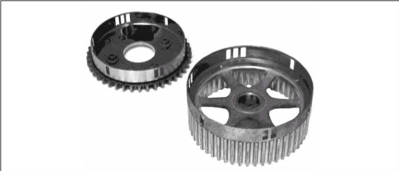
Figure 39 Typical 6 Cylinder CMP Triggers (2.7L NGC shown)
