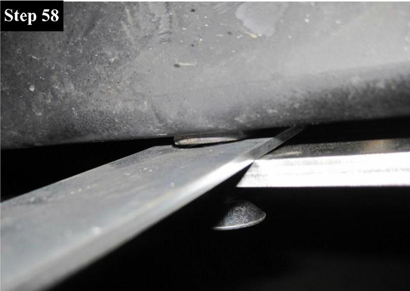
On the driver side of the vehicle, rotate the Wing Spacer (D) outwards and begin tightening the 12mm X 1.75 X 40mm Flat Head Allen Screw. As you tighten the bolt make sure that the Wing Spacer (D) is centered around the frame nutsert.
