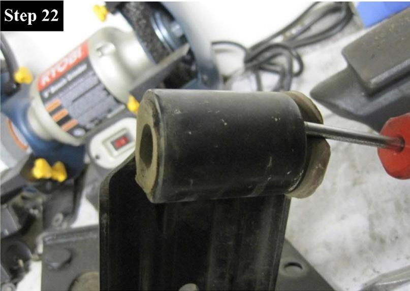
Using a flat head screw driver as a shoehorn, carefully tug the exhaust hanger bushing from the stock transmission mount.
