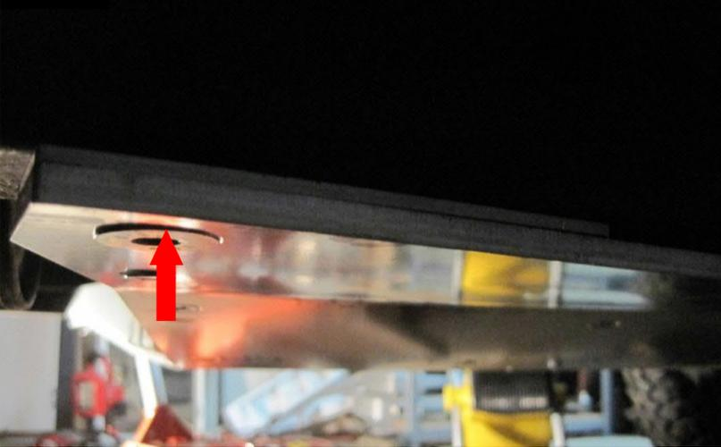
Tighten the 12mm X 1.75 X 40mm Flat Head Screw.
