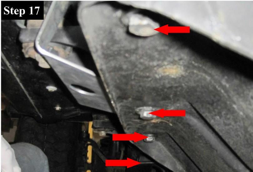
At this point SLOWLY raise the drivetrain at the output shaft of the transfercase so that the transmission studs are clear of the transfercase skid.
