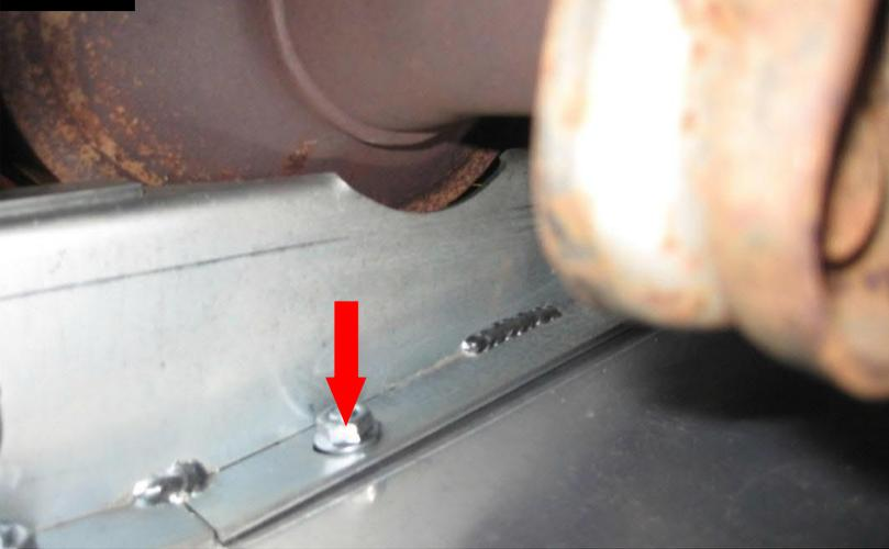
On the passenger side of the vehicle, loosely install the (2) 5/16 - 18 X 3/4" Flat Head Phillips Screws and 5/16 - 18 Flange Nuts. One is located behind the muffler and is not shown in the picture.
