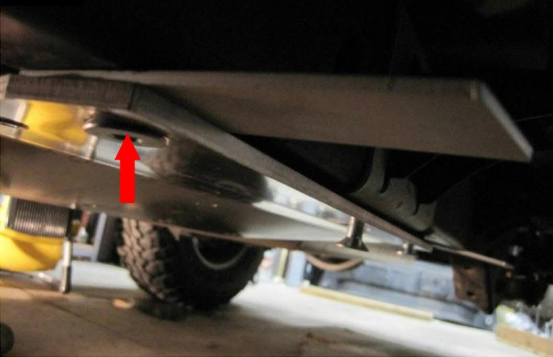
Rotate the Wing Spacer (D) outwards and begin tightening the 12mm X 1.75 X 40mm Flat Head Allen Screw. As you tighten the bolt make sure that the Wing Spacer (D) is centered around the frame nutsert.
