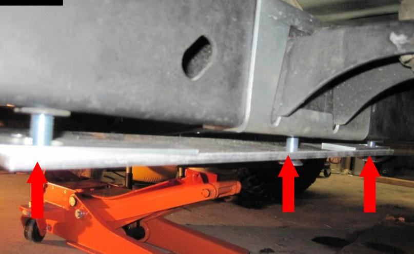
Moving on to the passenger side of the vehicle, loosely install the (3) 12mm X 1.75 X 40mm Flat Head Allen Screws and Wing Spacers (D).
