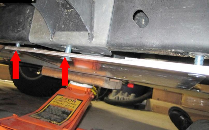
Loosely install the remaining (2) 12mm X 1.75 X 40mm Flat Head Allen Screws and Wing Spacers (D).
