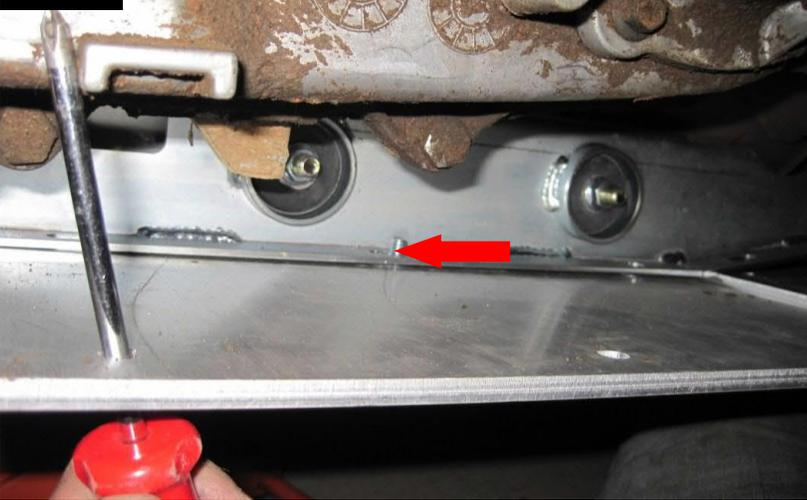
Moving on to the back, you will find it will be initially difficult to line up the fasteners to the Crossmember (H).
