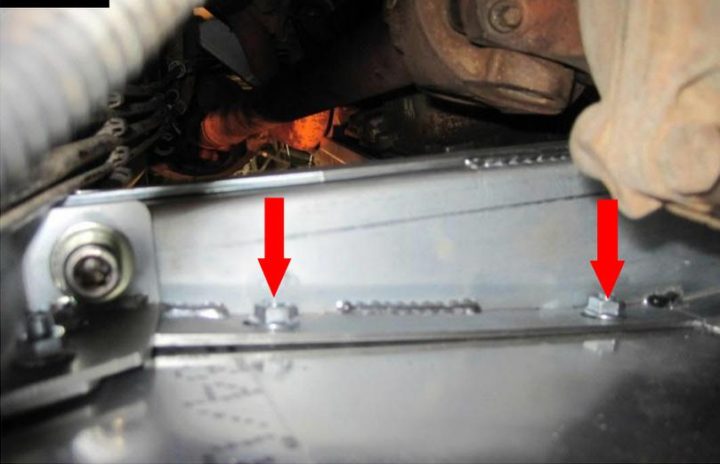
On the driver side of the vehicle, loosely install the (2) 5/16 - 18 X 3/4" Flat Head Phillips Screws and 5/16 - 18 Flange Nuts.
