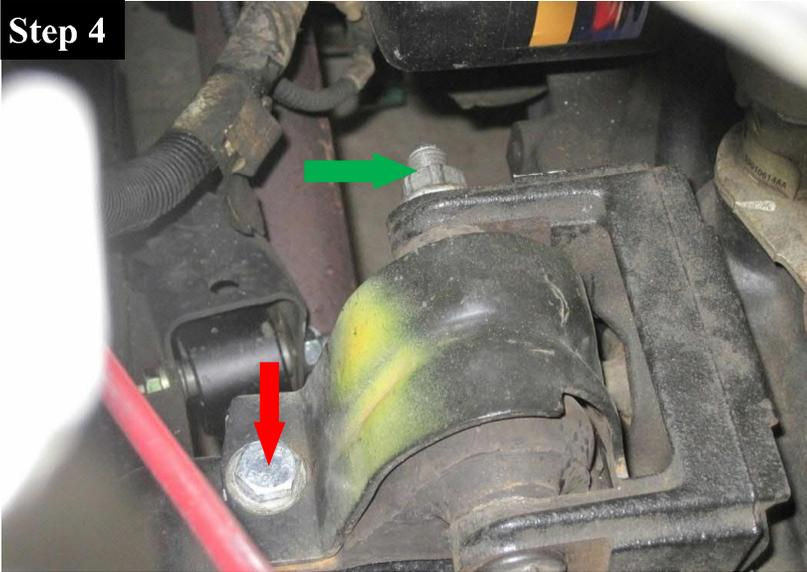
Loosen the motor mount through bolt using 18mm socket (DO NOT REMOVE) shown by the green arrow.
