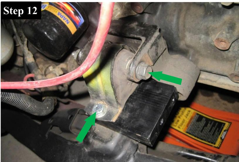
It is now time to install Motor Mount Spacers (G). Both Motor Mount Spacers should be installed with the threaded side facing the front of the vehicle. The L-shaped motor mount spacer should be installed on the passenger side of the vehicle.
