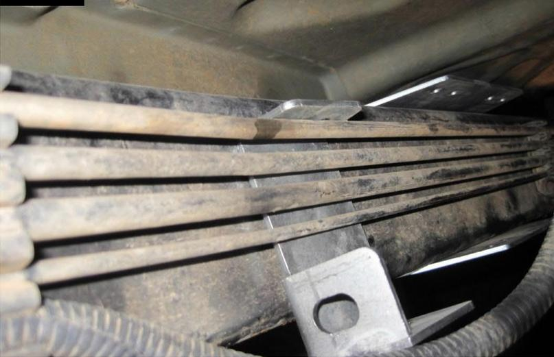
Slide the Frame Inner C Bracket (J) all the way down to the Frame C (I).
