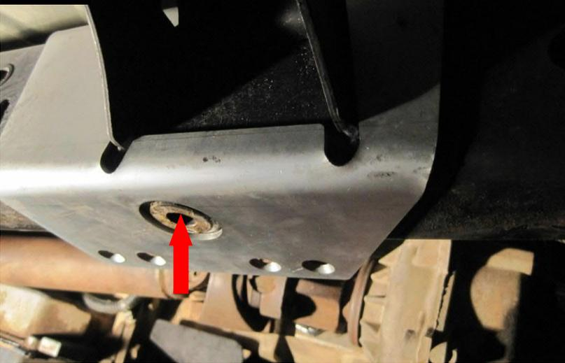
Using a rubber mallet tap the Frame C (I) so that it is centered in the frame nutsert. Now install the passenger side Frame C.
