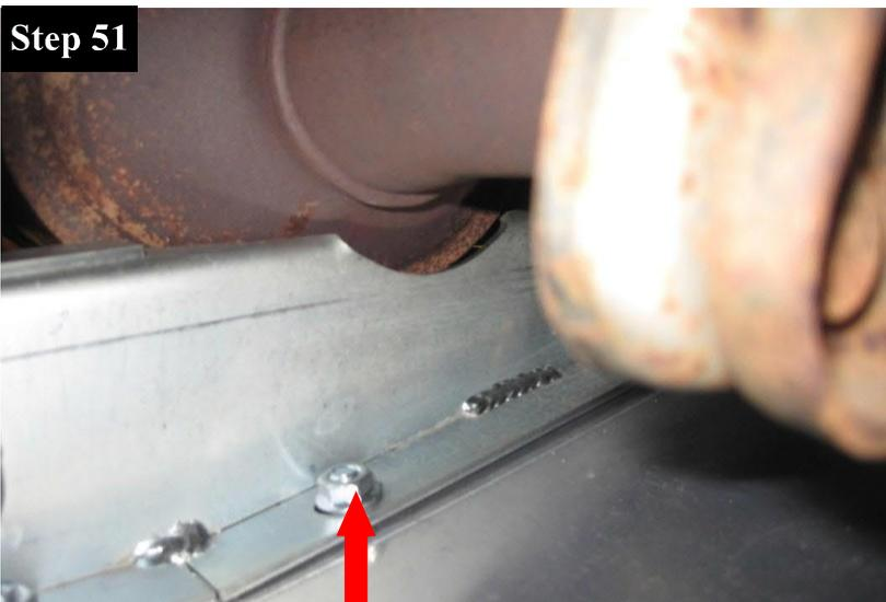
On the passenger side of the vehicle, tighten the (2) 5/16 - 18 X 3/4" Flat Head Phillips Screw and (2) 5/16 - 18 Flange Nuts. One fastener is located behind the exhaust system and is not shown in the picture.
