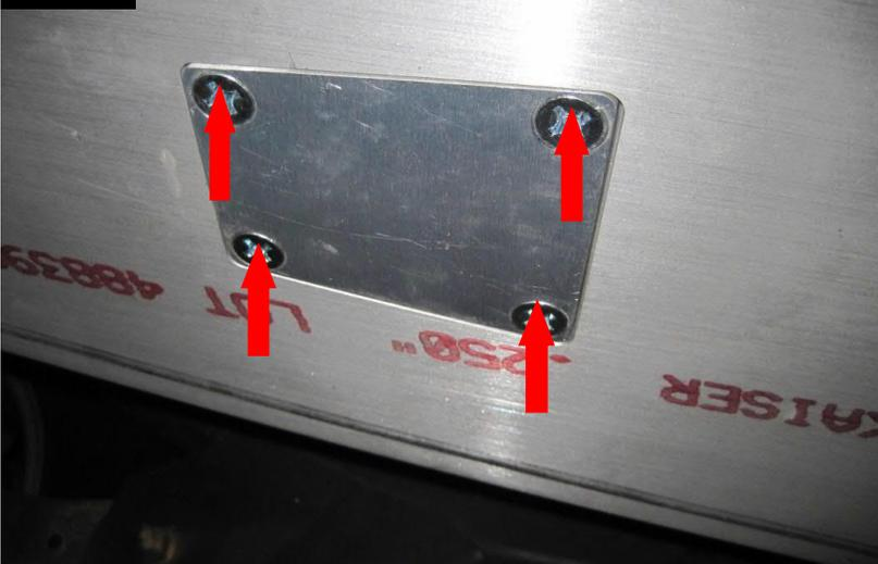
Moving to the middle of the Main Skid (A), install the Drain Cover with the (4) 5/16 - 18 X 1" Flat Head Phillips Screws and (4) 5/16 - 18 Flange Nuts.
