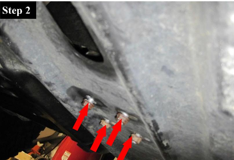
Start by removing each of the four transmission mount nuts on your transfer case skid plate.
