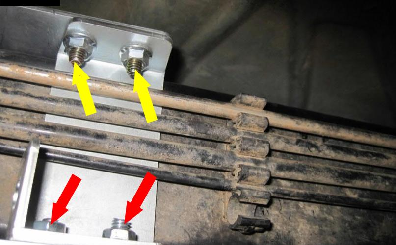
Loosely install the (2) 5/16 - 18 X 3/4" HHCS G8 Zinc Bolts with two 5/16 - 18 Flange. (yellow arrows)
