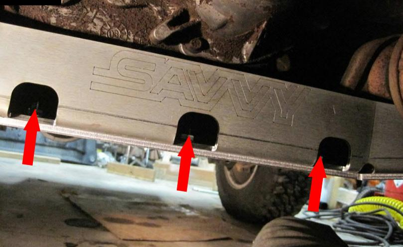
Slip the Rear Brace (M) onto the Main Skid (A). You may have to rotate it around the exhaust system to install it.
