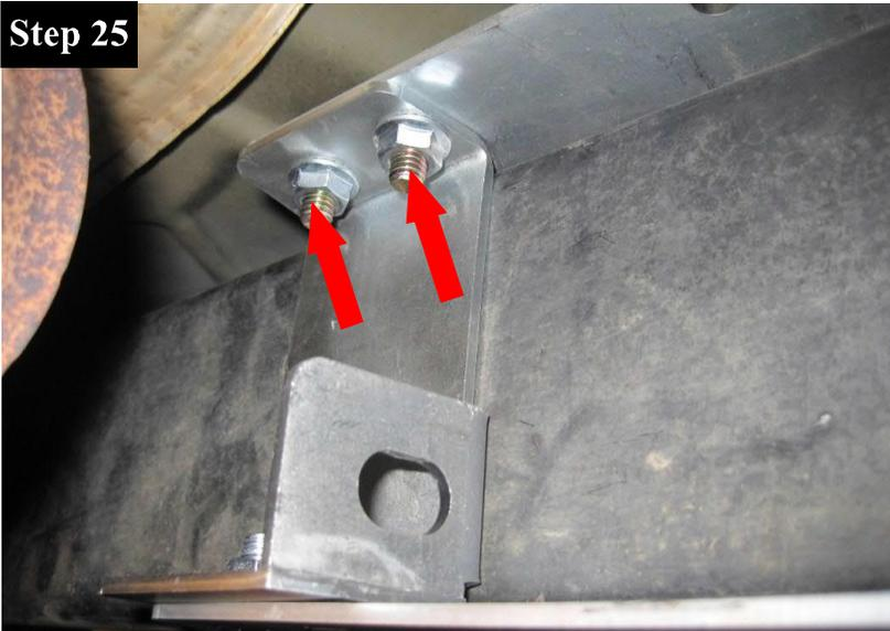
Working on the passenger side, slide the Frame Inner C Bracket (J).
