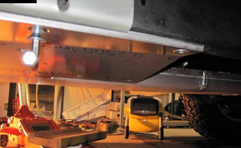
Tighten the middle 12mm X 1.75 X 40mm Flat Head Allen Screw.
