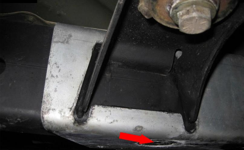
On the passenger side, Using a rubber mallet tap the Frame C (I) so that it is centered in the frame nutsert.
