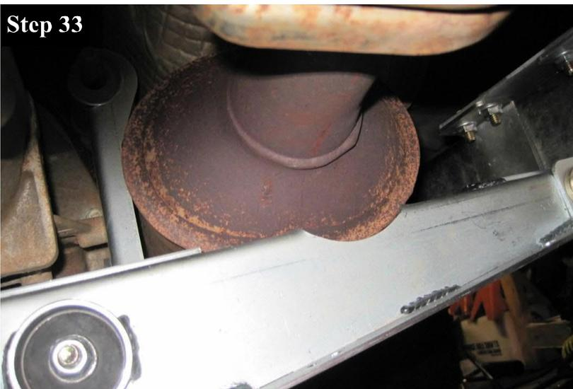
Loosen the two exhaust hangers at the rear of the vehicle. They are located near the passenger rear upper control arm and behind the passenger rear tire.
