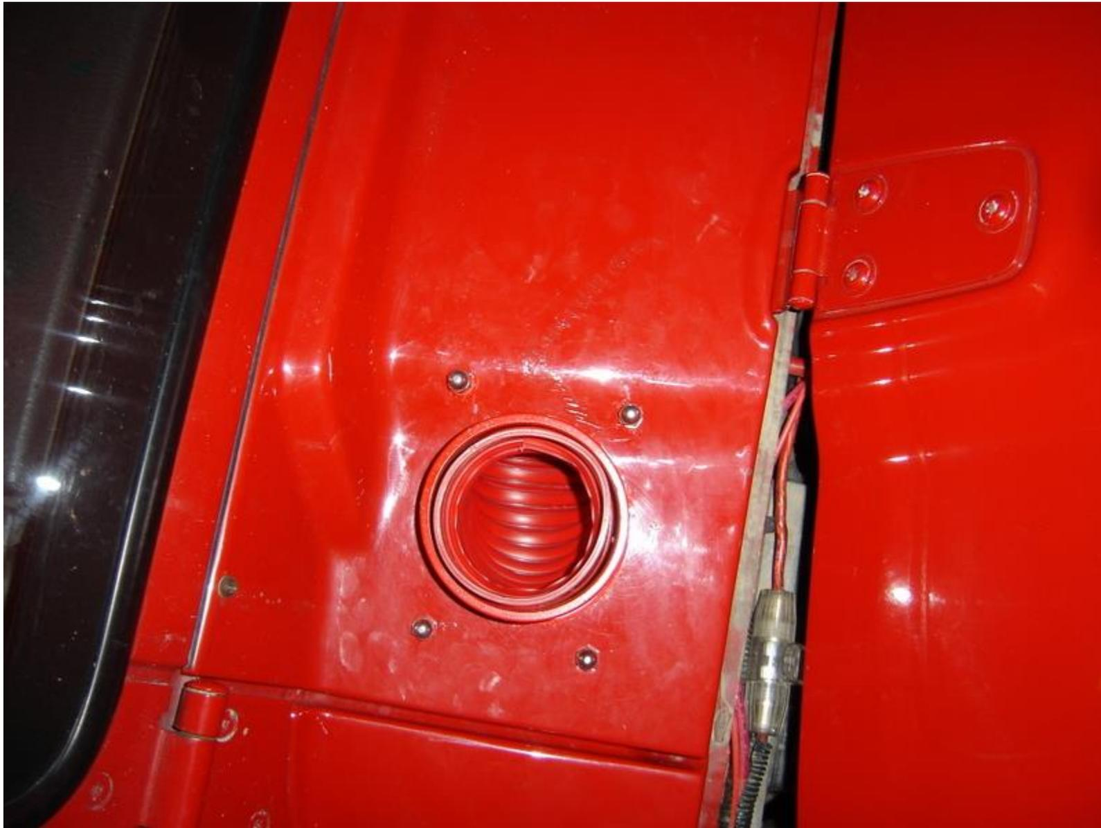
Ok, I will say this again; the cowl cover does not fit as nice anymore. It's pretty cramped in the corner since the cover slopes down and the cowl slopes up. No to mention the flex tube needs to make a 90 degree bend in that area. I was able to press the
