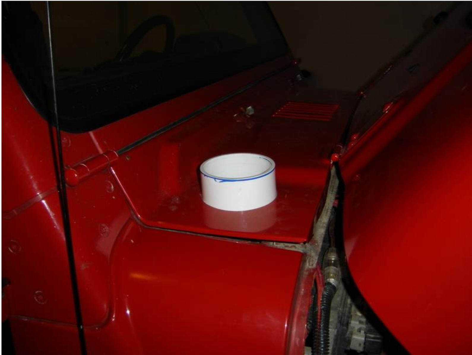
I trimmed up the fresh air intake and then test fit the flex tubing as you can see in this next pic.
