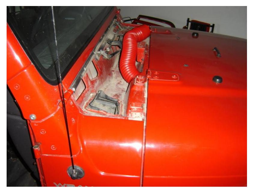
I then used the dremel to cut trim the black cover so I could re-install that and keep water out of the A/C/Heater unit. I opted to use it since DC designed it and started using it, there must be a reason. To make my "new" cover, I used some aluminum air
