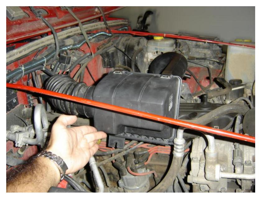
For the bracket I opened up the bottom end and attached that to the motor mount. I twisted and bent it with some pliers so everything would line up.
