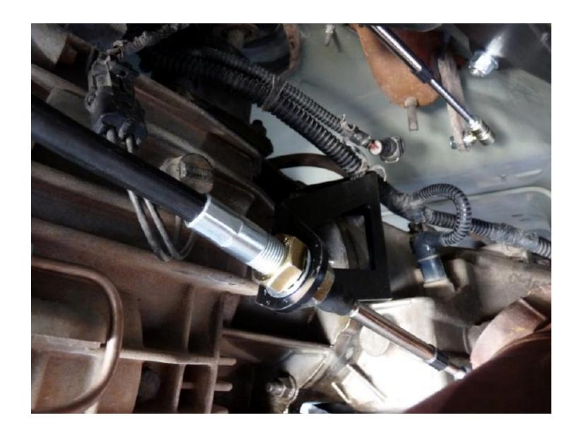
as you turn the drive shafts for shifting ease. Verify that the shift lever position corresponds with the detent positions in the transfer case.
