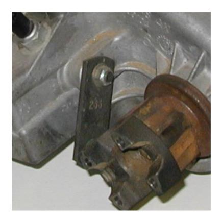
done with a 9/16" box end wrench or socket wrench and a little prying or side force against the plate. Keep the factory nut for your installation of the provided Novak shift rotator plate.
