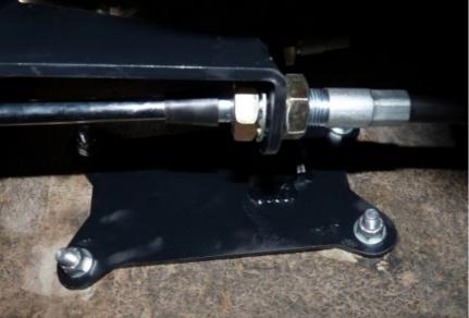
Remove one nut and threaded cable housing. is about in the middle of Feed the cable rearward through the hole in the body anchor bracket.
