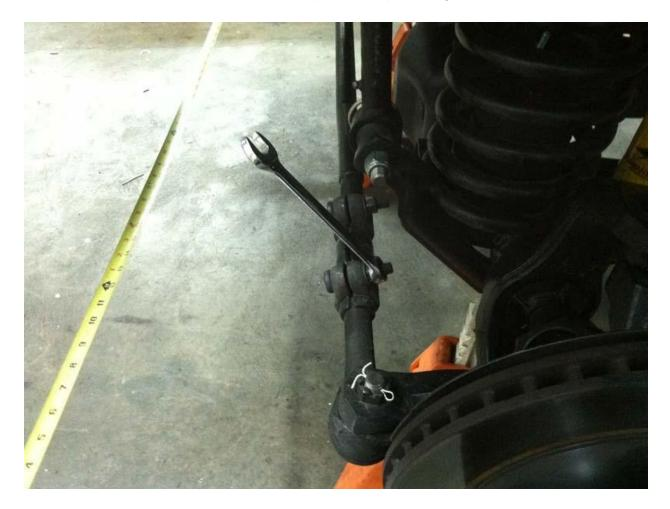
Once the toe in is adjusted you may find that your steering wheel is no longer centered, but this is easily corrected. Take the Jeep for a short drive to allow the suspension to kind of settle, and when you pull in to your work area, pull in with your wheels pointed as straight as possible (no matter where your steering wheel is.
