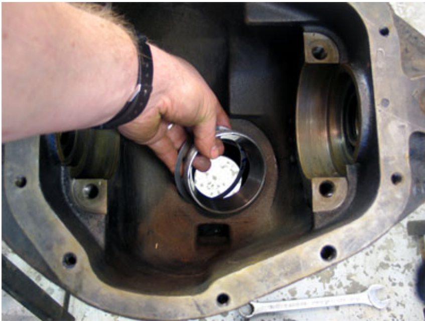
Figure 19 – Installing inner pinion-bearing shims and cup
