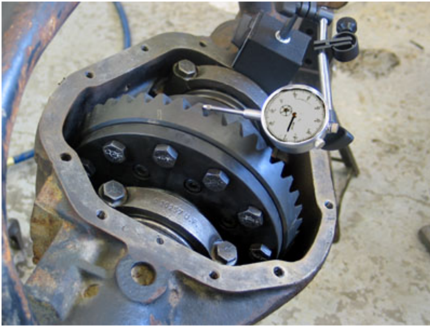
Figure 27 – Measuring backlash with dial indicator
