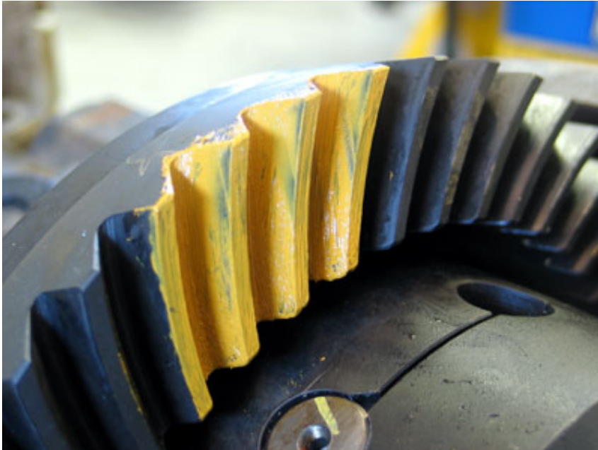
Figure 31 – Drive-side contact pattern - top / heel. The dark area on the yellow is where the pinion and ring-gear have come into contact, removing the marking compound from the teeth and illustrating the contact pattern. In this case, it is on the drive-side of the ring-gear teeth and is clearly towards the top and at the heel of the teeth, illustrating that the pinion depth is way too shallow
