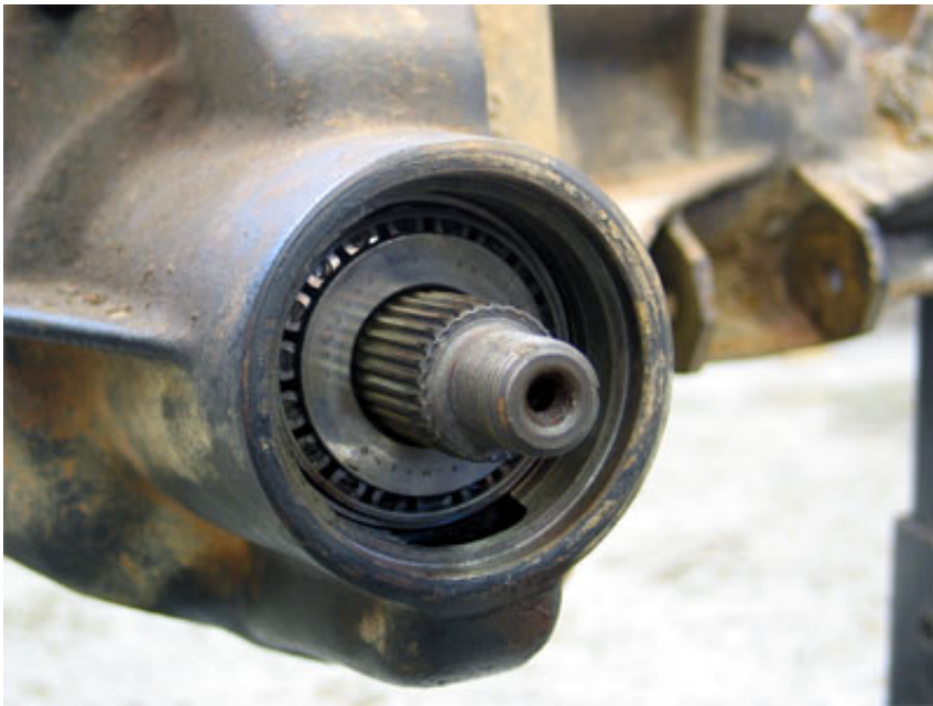
Figure 23 – Installed outer pinion set-up bearing
