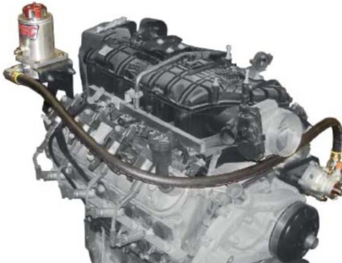
Here the feed line is kinked, cutting off flow to the pump.
