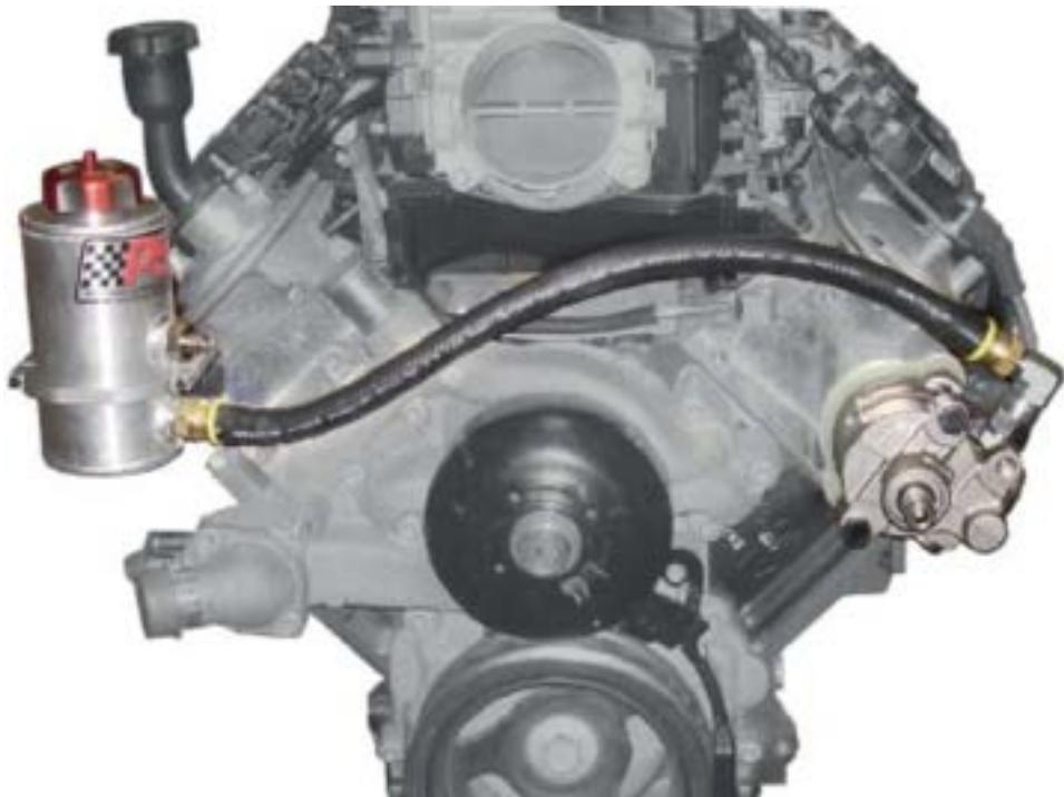
In addition to a loop, this picture illustrates a bend that is too tight resulting in a collapsed hose.
