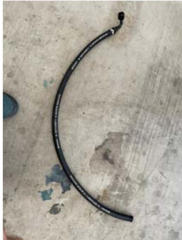
Don't install a fitting on the other end just yet and don't cut the hose either. Install the end with the fitting onto the passenger side of the cooler. Tighten the fitting snug to the adapter on the cooler, then run the hose down and under the cooler, back to the drivers side and out through the bottom of the grille right next to where the steering gearbox is:
