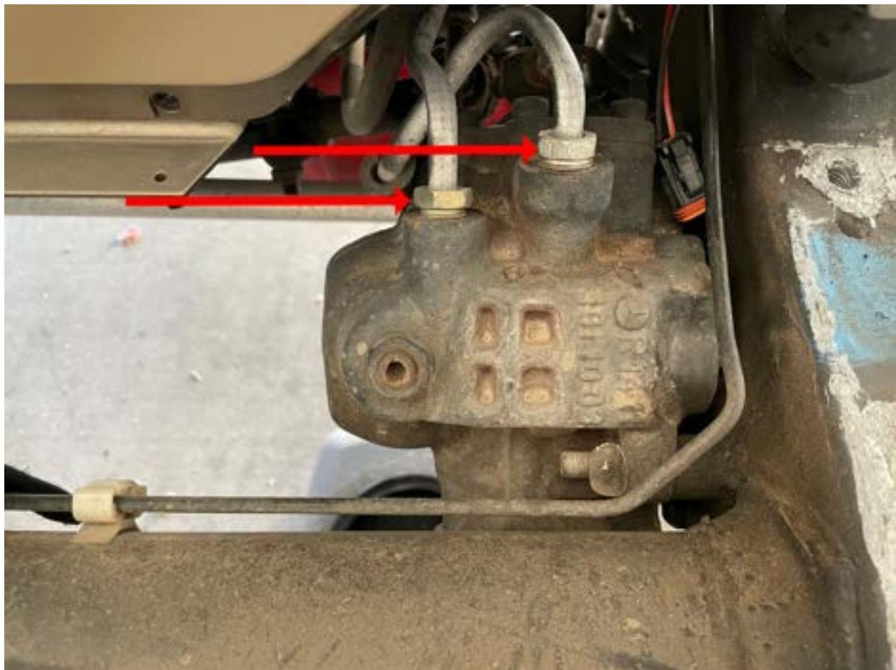
I put a drip pan below the steering box, loosened and removed the fittings, and then waited for the system to drain out. Note that even after doing this there will still be fluid that comes out as you remove other pieces of the system, but this should at least get the bulk of the fluid out.
