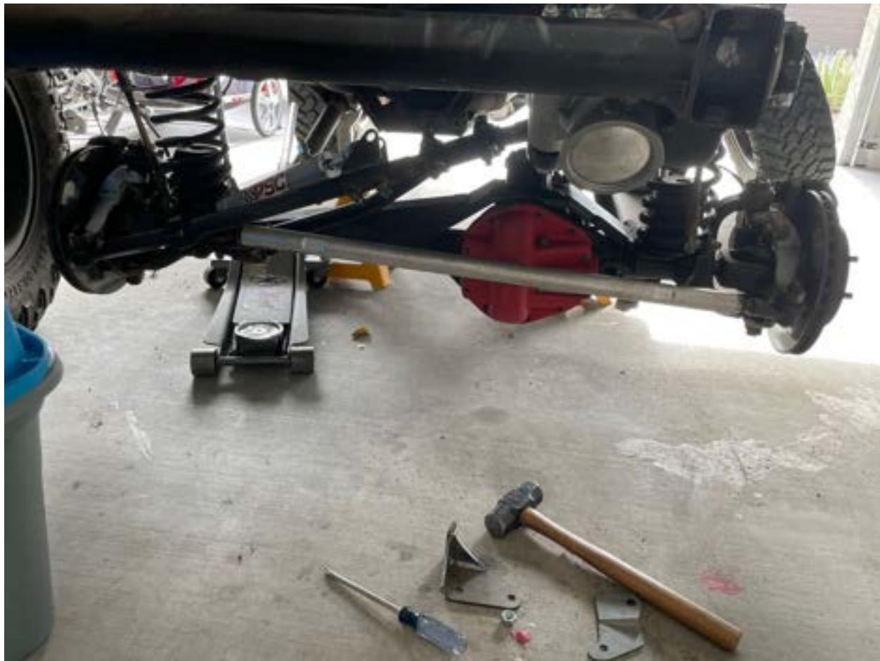
Your drag link should still be hanging there as we have not yet bolted things back up. If you haven't already, you'll need to remove the drag link collar and tie-rod from the end. This is done so that we can slide the drag link clamp (part number 17 in the diagram) over the drag link itself.
