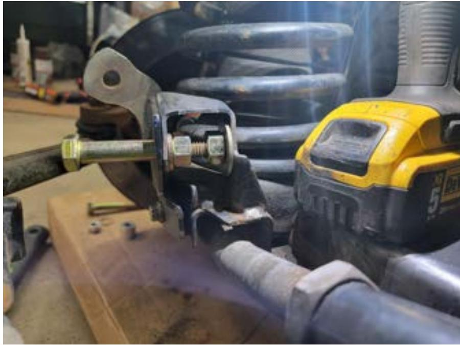
If the assist cylinder rod end with spacers don't fit in the OEM stabilizer bracket, you can widen the bracket by placing a bolt or all thread through with 2 nuts and use them to expand the area wide enough.
