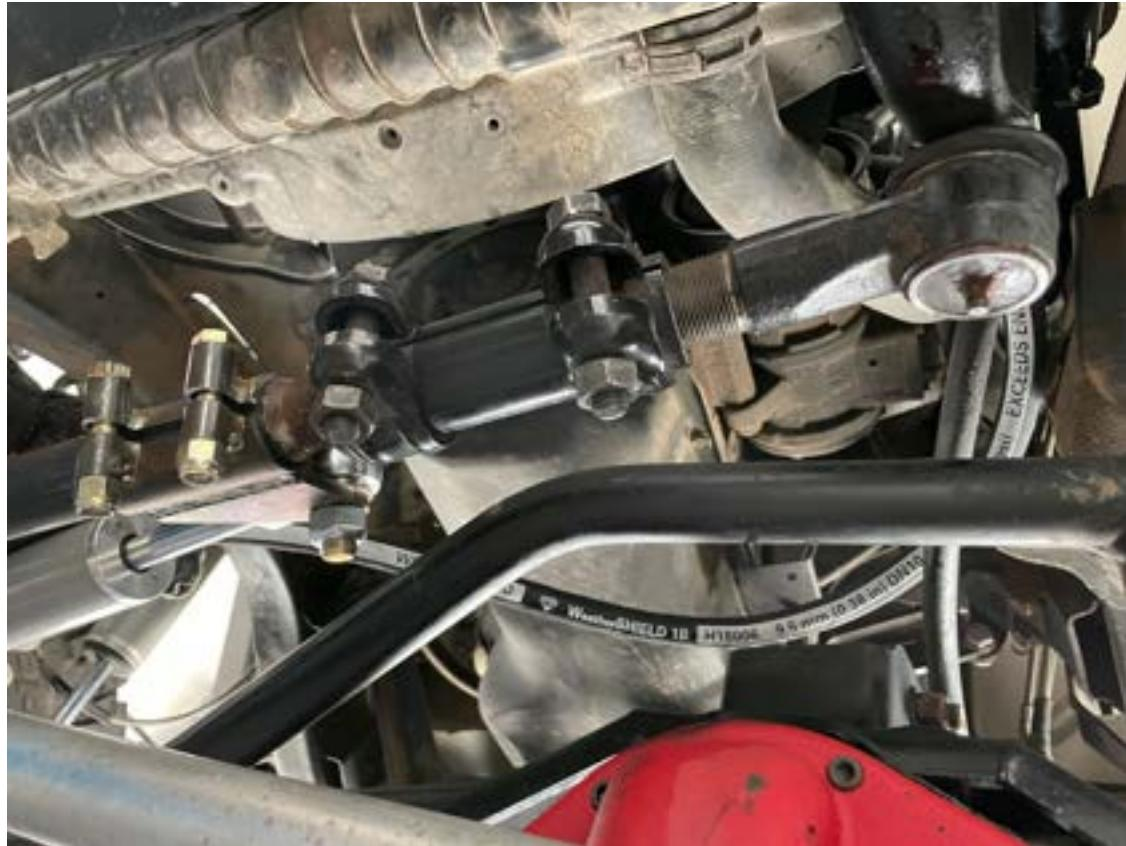
At this point you should be able to see where you'll need to cut this hose to install the other -6 field serviceable high pressure hose end where it attaches to the cylinder assist (part number 16 in the diagram). When doing this, please pay close attention to the red arrows on the diagram and notice where each hose goes on the steering box and where it goes to on the cylinder assist. Do not mix these up, it's important that they are installed correctly!
