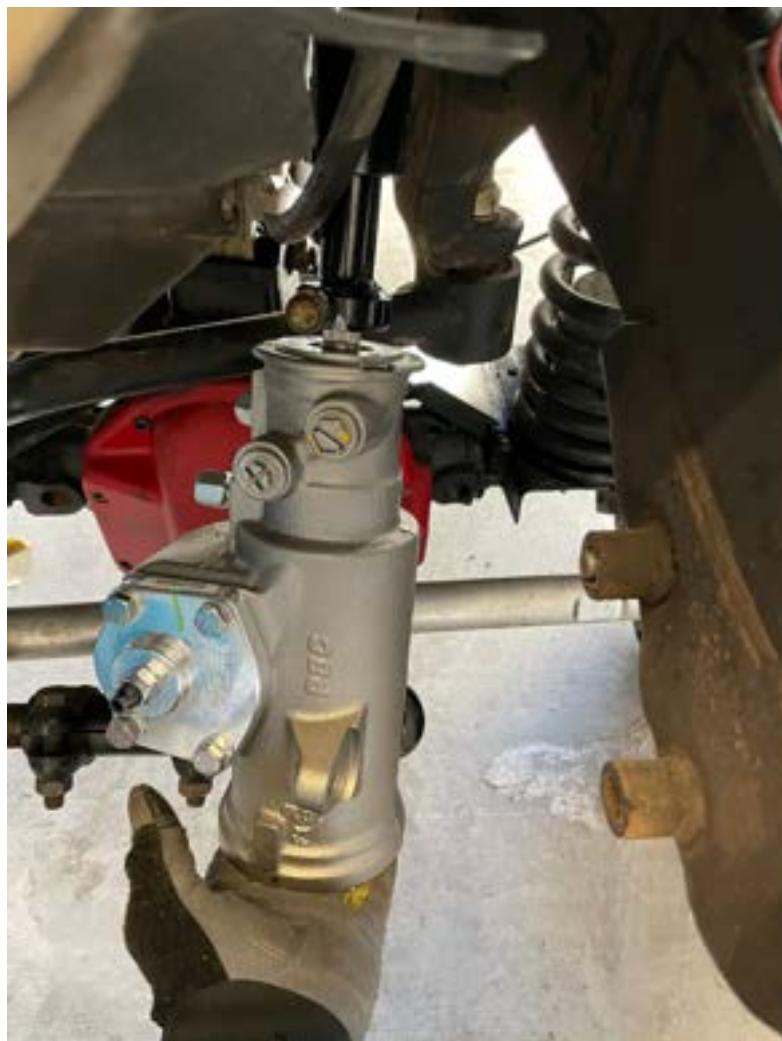
Now raise the steering box up and use the three bolts to attach it to the frame, making sure to torque them all to 70 ft/lbs.
