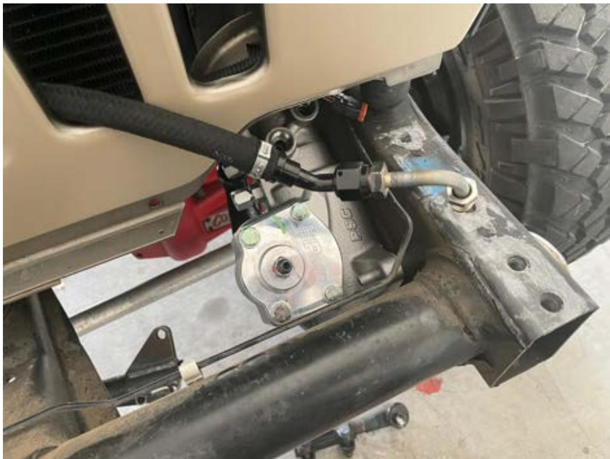
Tighten the Oetiker clamp but lead the two fittings slightly loose as you'll need to play around with the correct angle for the fittings before tightening them down.
