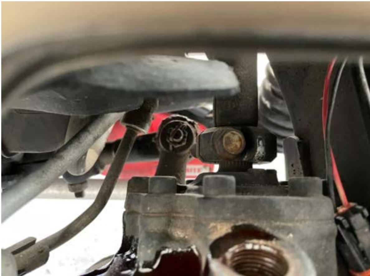
Once the bolt is removed, I used a pry bar to pry the steering shaft back enough so that it would slide off the splines. The pry bar helped a lot since the shaft is stuck on there pretty good from all the years of never having been removed.
