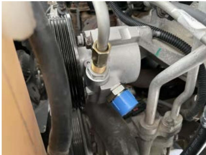
Screw in the fitting at the steering gear but leave it a little loose so the hard line can rotate. Now insert a pry bar or long screw driver and clock the tubing so that it comes off the steering gear pointed toward the center of the Jeep. This will give the other fitting more room to point where it should.
