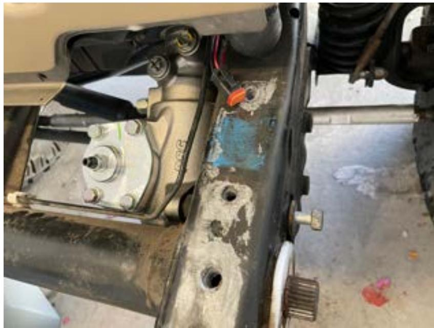
Be aware that the red lines on the steering gearbox and the steering shaft need to be aligned. This is how you know the steering box is centered. If they are not aligned, you will have issues with your steering.
