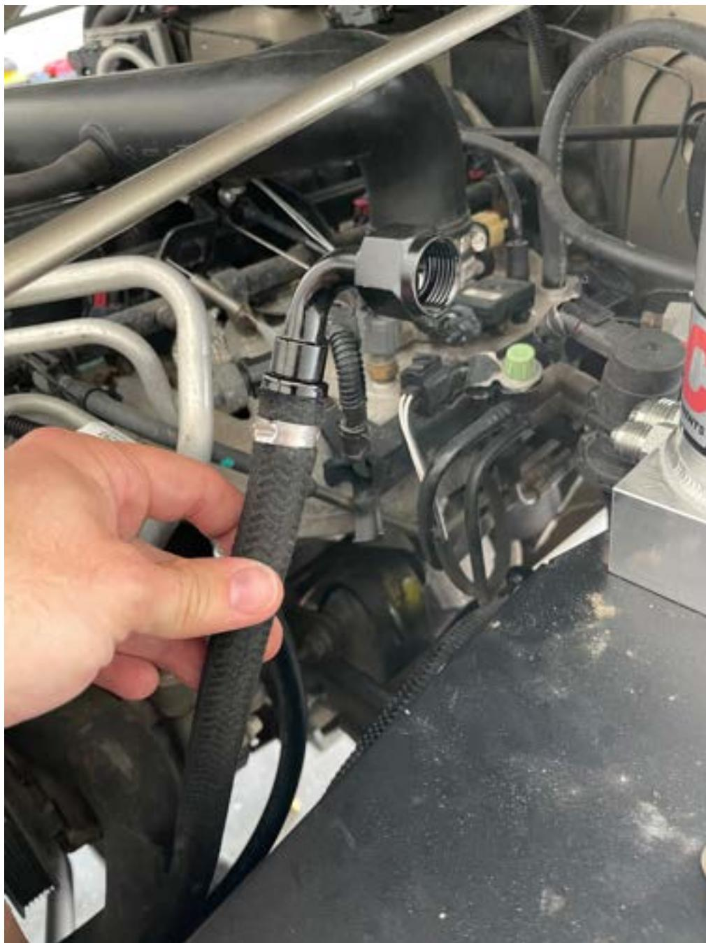
Tighten this fitting snug onto the adapter on the cooler -8 adapter on the cooler (it only fits on one of them so this should be obvious) and now you'll move on to the -12 feed line from the reservoir to the pump.
