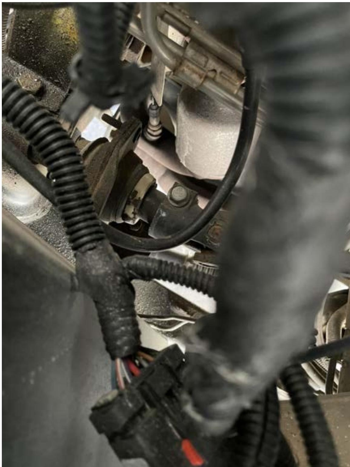
Once all the bolts were removed, my pry bar came in handy again to give the lower steering shaft a good nudge in separating it from the upper steering shaft. If it's never been removed before, it can be in there pretty good.
