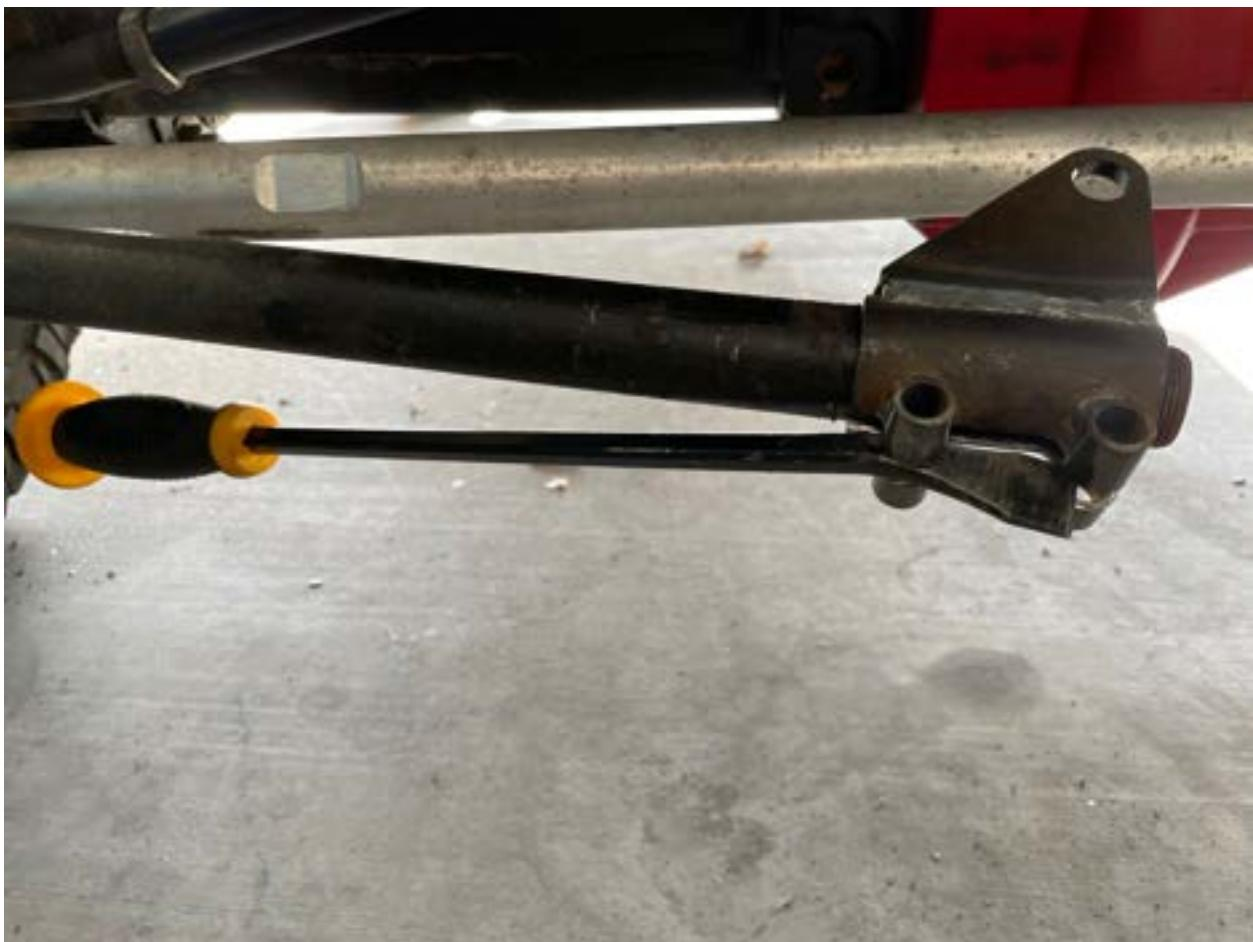
Next you'll want to get the cylinder assist (part number 16 in the diagram) and the two misalignment spacers (part number 24 in the diagram). Install the misalignment spacers onto the end of the cylinder assist like this:
