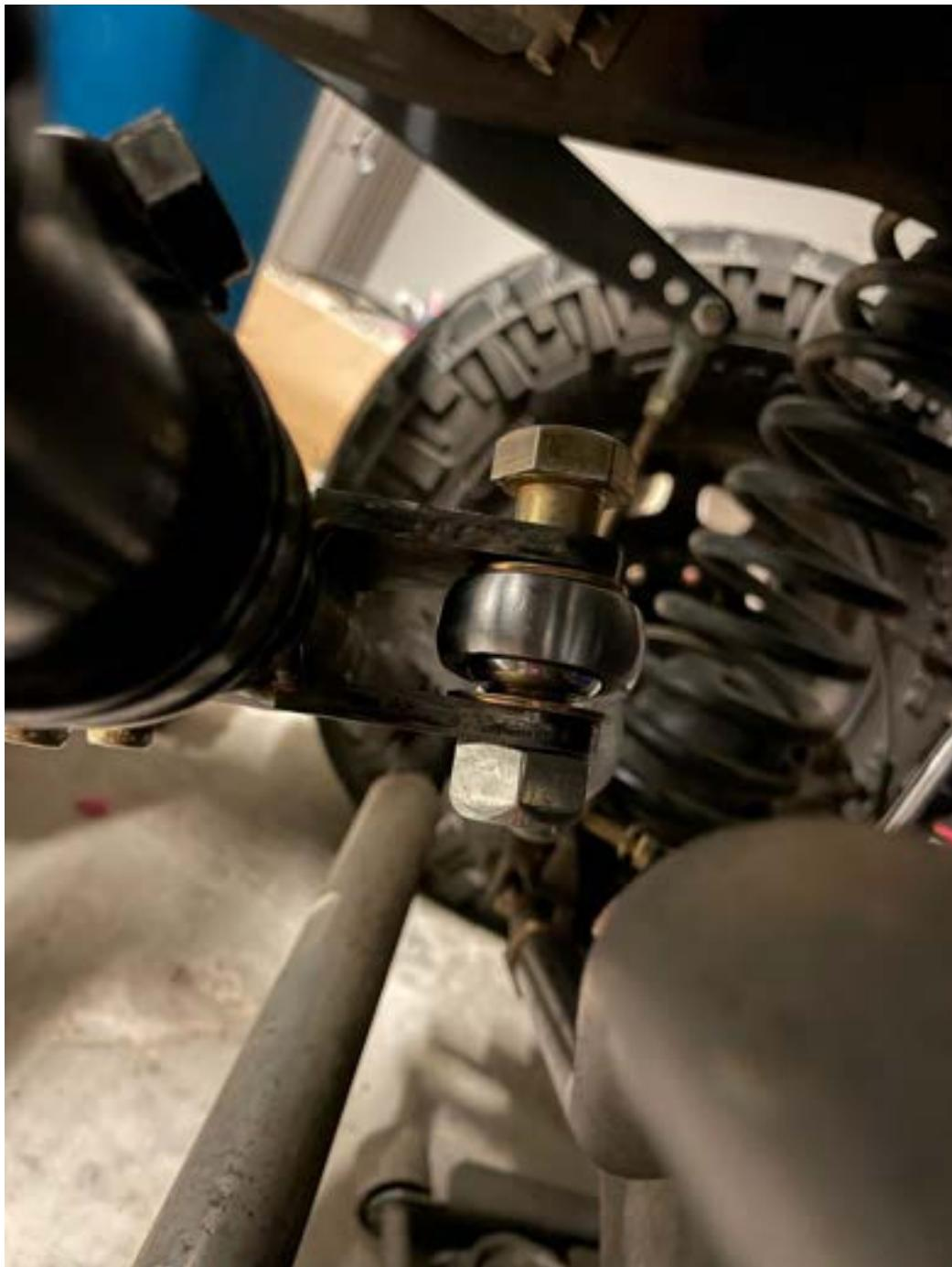
The drag link clamp will be rotated back about 45 degrees. You'll need the cylinder bolt (part number 18 from the diagram), both thin washers, and the nut that goes with it. Pay close attention here because the two thin washers go inside the clamp.
