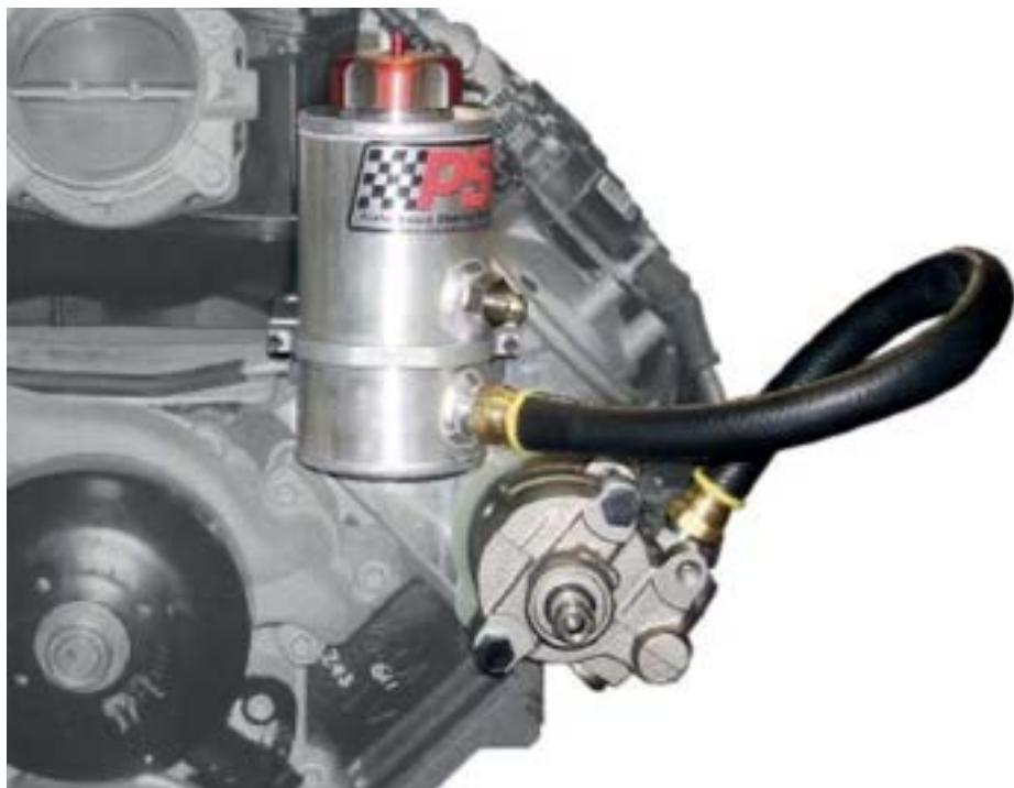
Fill level should be 1" below the top of the reservoir. On single ended cylinder applications this should be measured with the cylinder collapsed. Your reservoir may differ from that pictured here.
