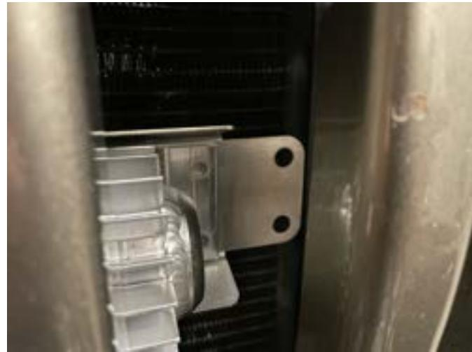
What this does is capture the v-bar from the backside so that the cooler will be securely fastened in place.
