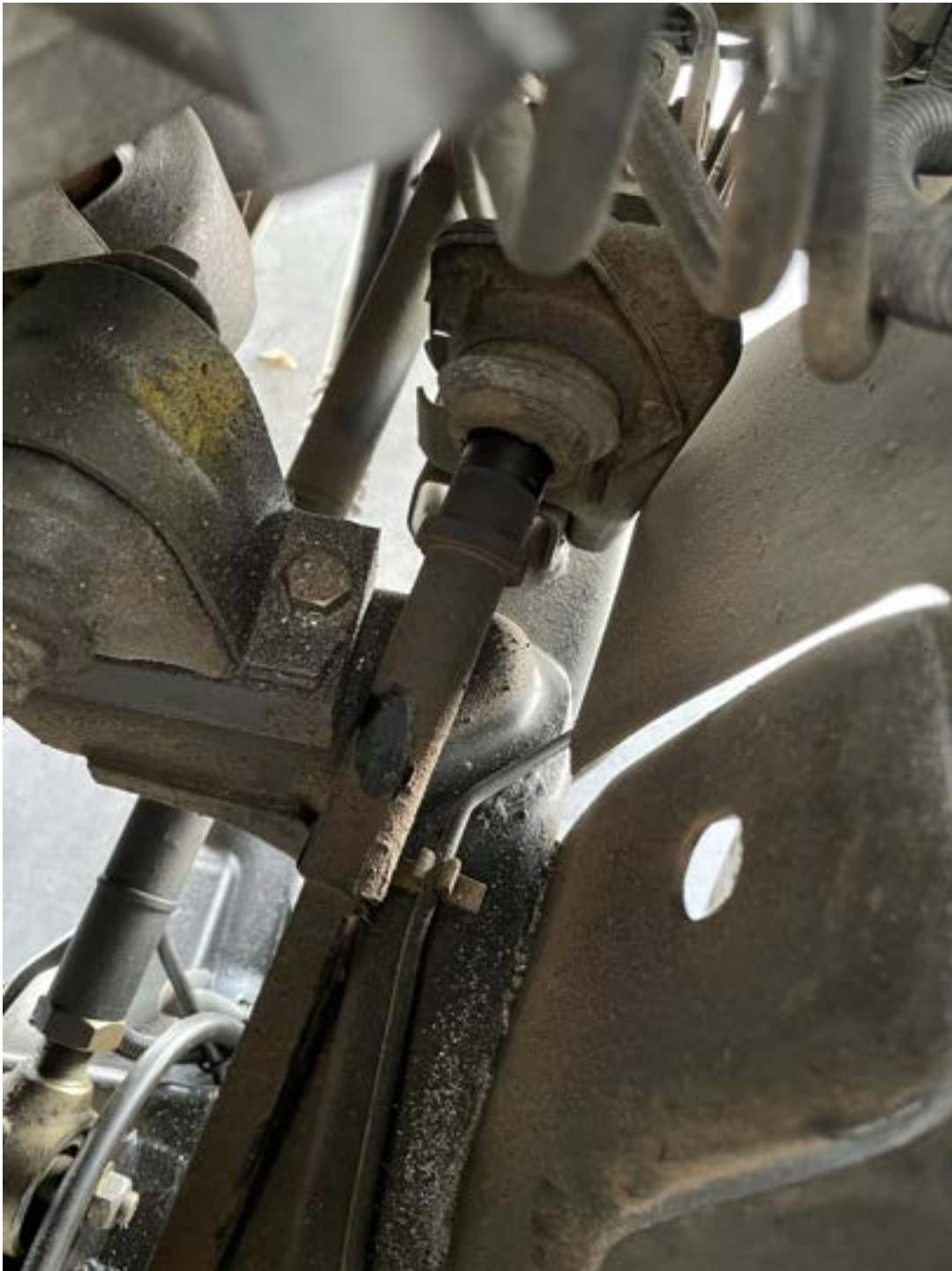
You'll also need to loosen this larger bolt in the clamp and holds the end of the lower steering shaft into the upper steering shaft:
