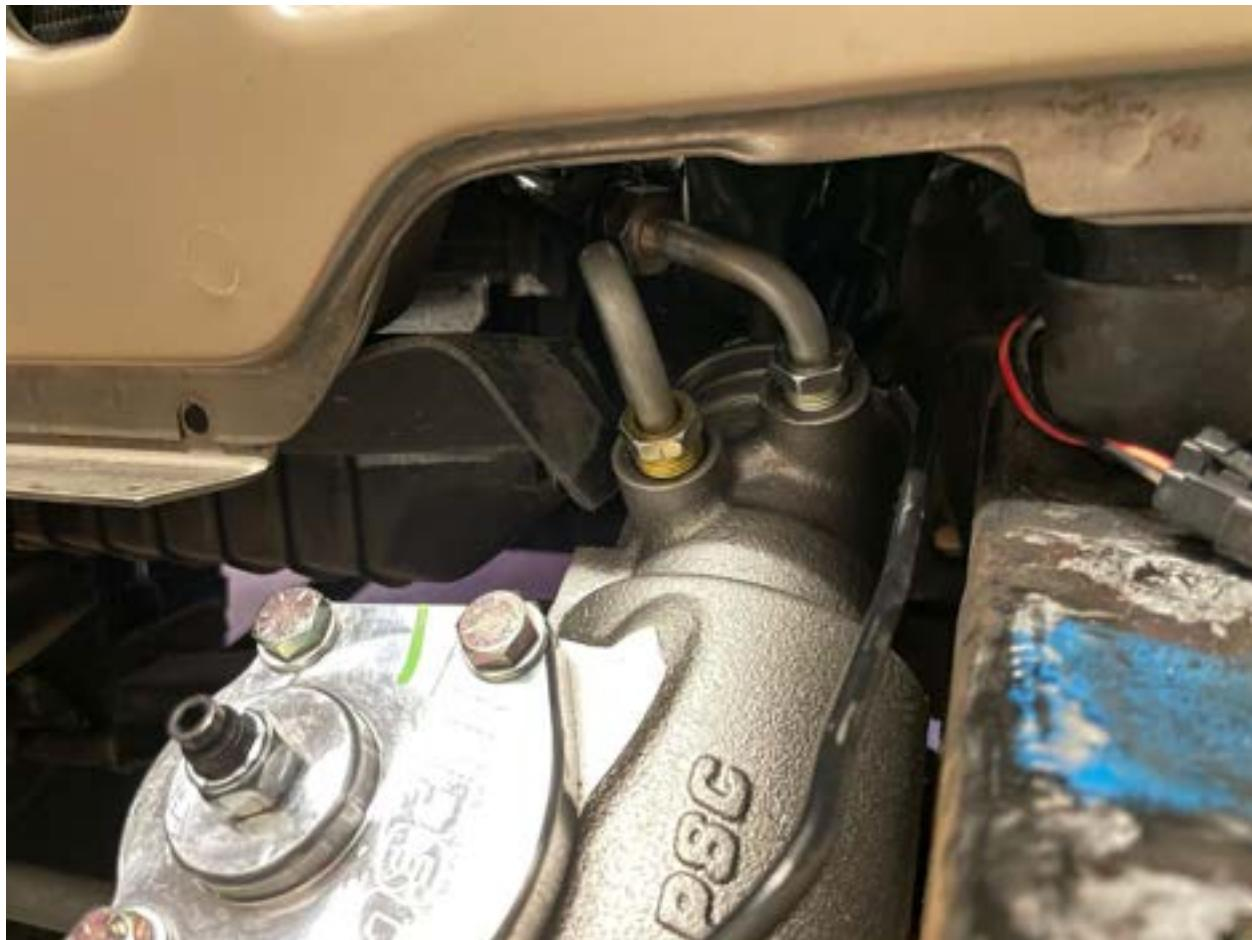
It should go without saying that this line goes into the port on the steering gearbox that is closest to the driver. Once you have installed it, tighten it down.
