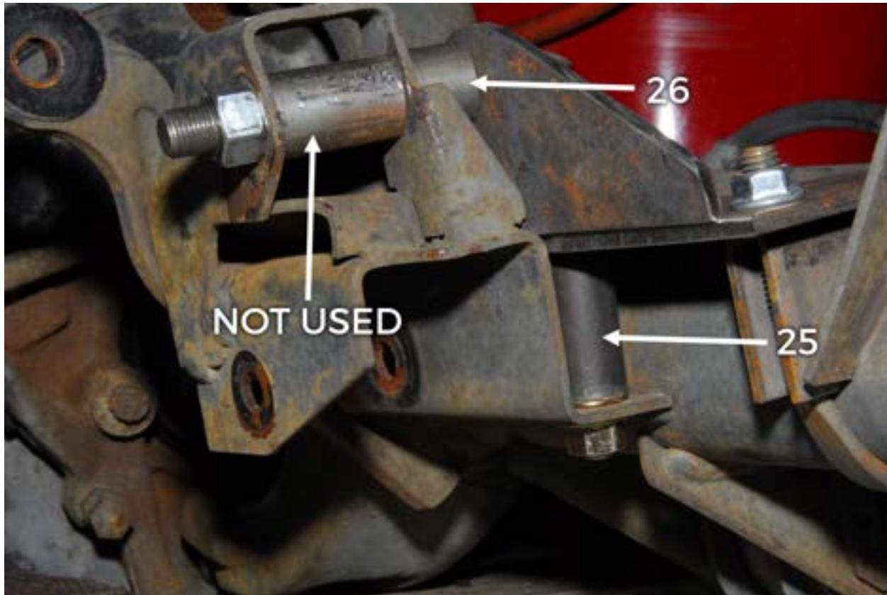
The rear bracket (number 21 in the diagram) bolts on the back side of the stabilizer mount, then the cylinder mount axle clamp (part number 27 in the diagram) or u-bolt goes around the bottom of the axle and bolts-in from the top of the mount.
