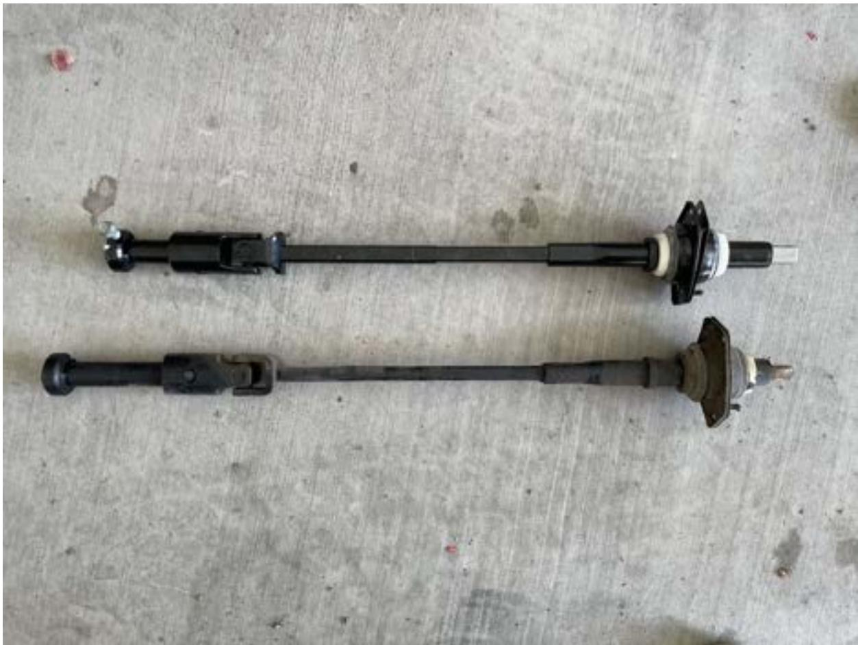
In that photo, the 97-02 steering shaft is on top, and the 03-06 steering shaft is on bottom. The longer section that connects to the steering gear input shaft is the problem. The PSC gear is based on the early Saginaw steering gear which is longer and needs the shorter section to keep the steering shaft angles correct.
