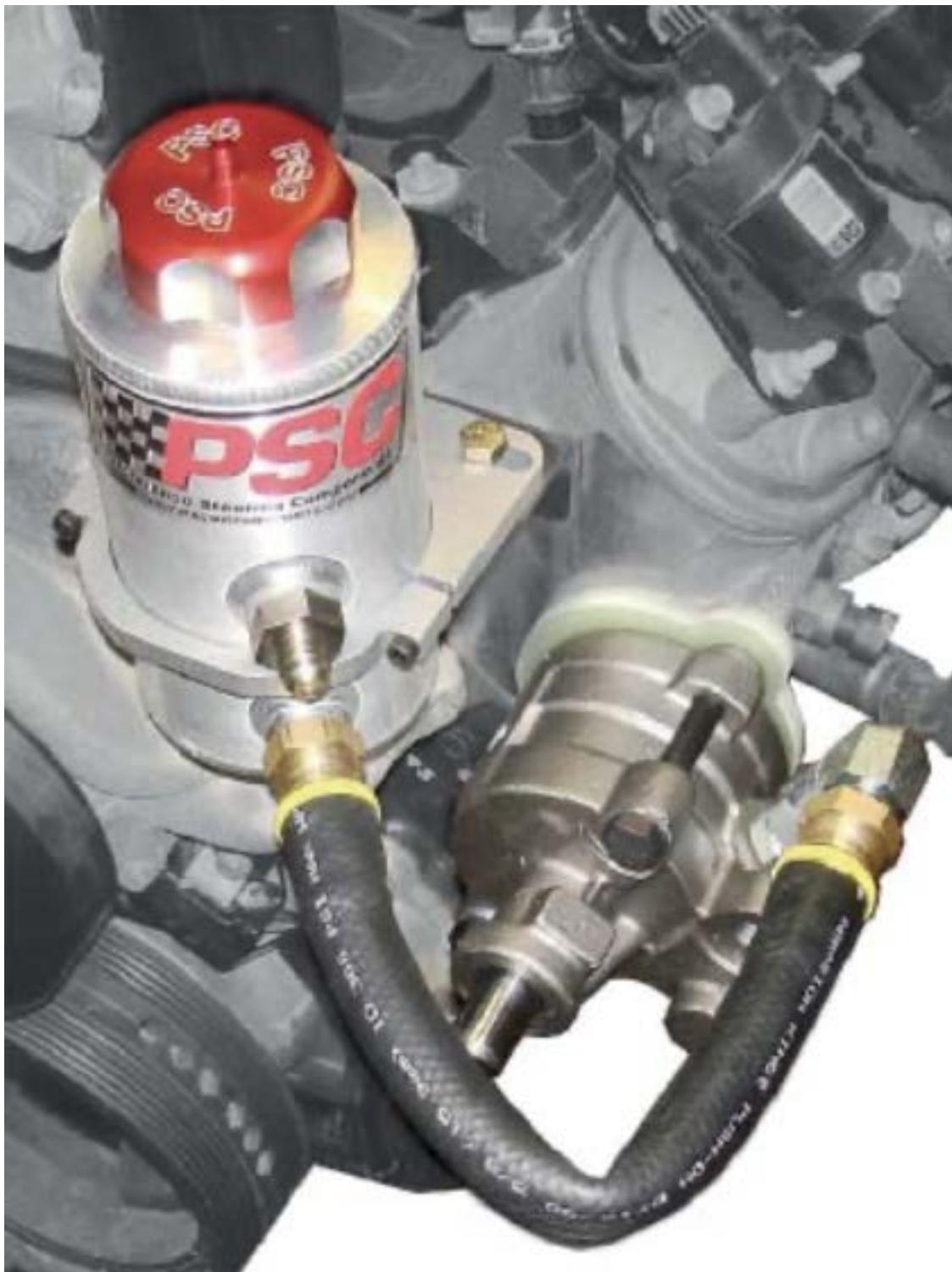
This picture shows another hose that has collapsed from using a bend that is too tight. It also shows a big dip in the hose which will cause pump starvation. It also has a drilled tight 90 degree fitting which should be avoided.
