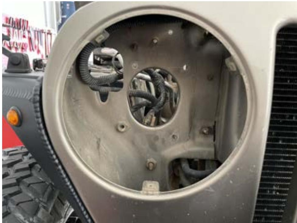
Now that the headlight bucket is removed, you can slide the cooler mount (part number 33 in the diagram) in through the headlight and onto the v-bar support like so:
