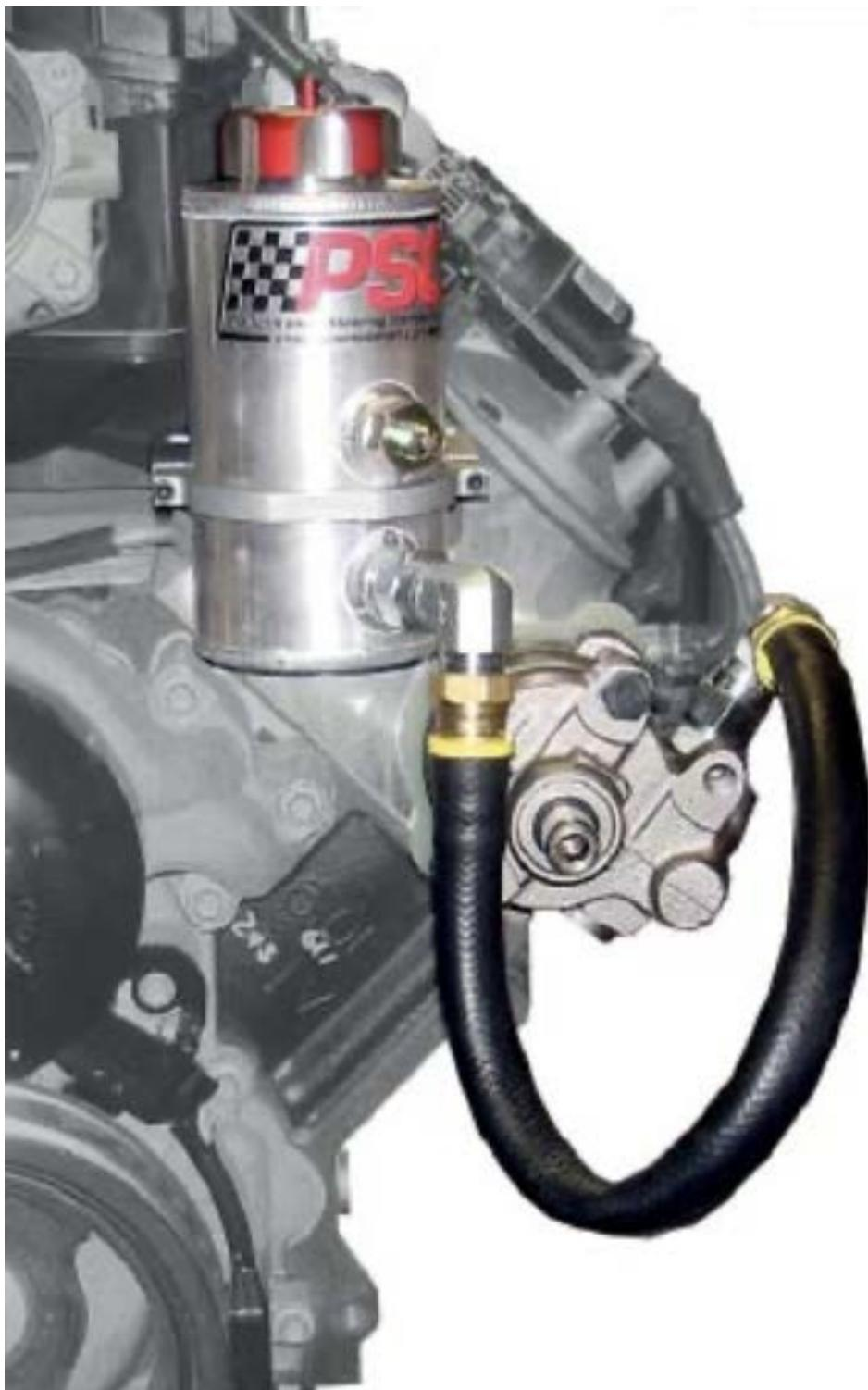
Here the feed line starts out just above the center line of the pump and must go uphill to meet the inlet of the pump.
