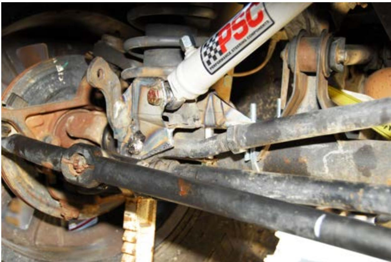
Now we need to determine exactly where to position the drag link clamp on the drag link.
