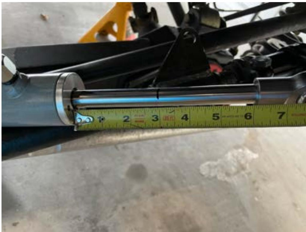
Now that the cylinder assist is in the center of it's travel, you can further position the drag link clamp into place so that it the holes align perfectly and you can get the bolt through.
