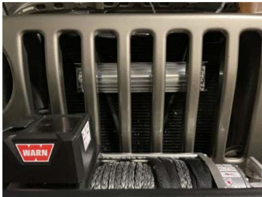
While you're installing the cooler, now is a perfect time to install the -8 x 3/8" NPT adapters (part number 32 in the diagram) onto each end of the cooler. As mentioned in the important installation notes above, these adapters will need Red Liquid Loctite on the ends that go into the cooler only.
