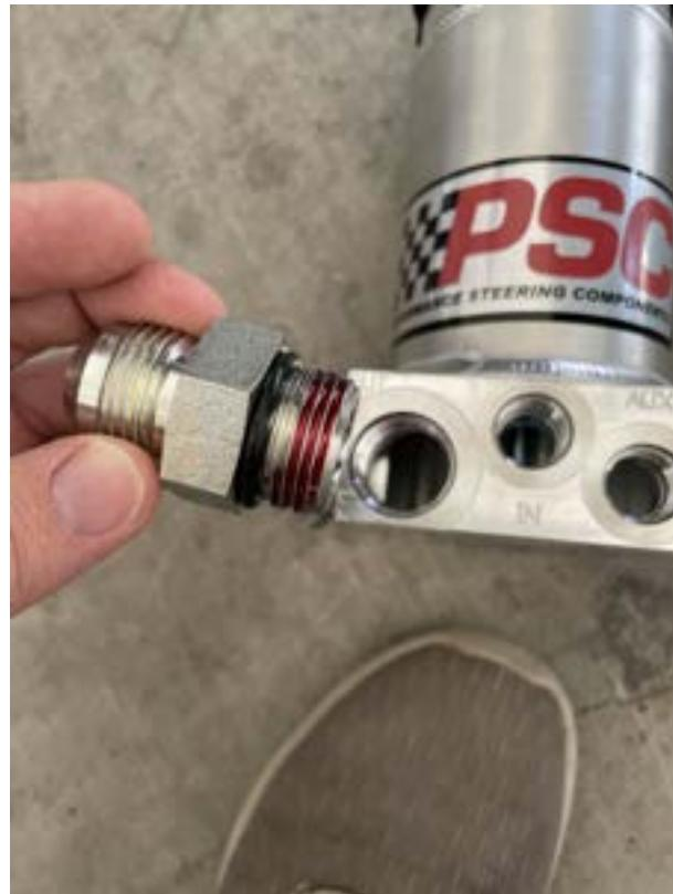
Now thread the adapter in all the way, then tighten it down with a ratchet and socket until it's tight and flush with the housing as shown:
