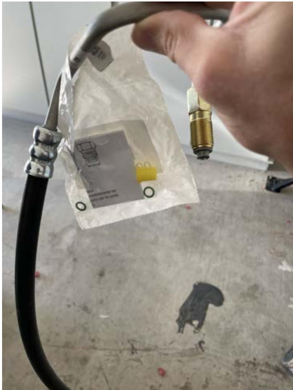
In the bag there are instructions which show how the o-rings need to be installed on this type of fitting:
