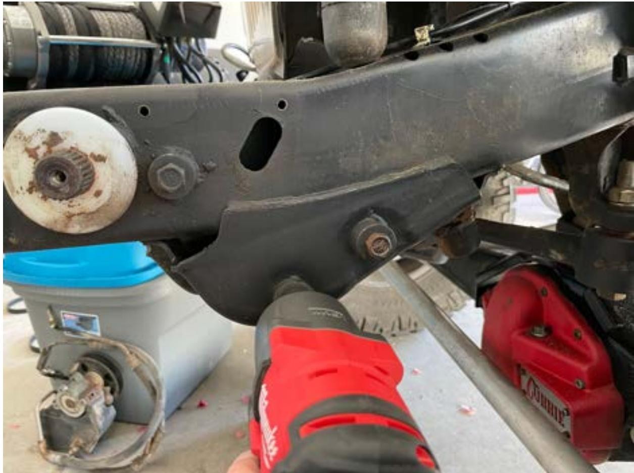
Make sure to hold the steering box from underneath, as once you get to the last bolt it will fall to the ground and it's very, very heavy!
