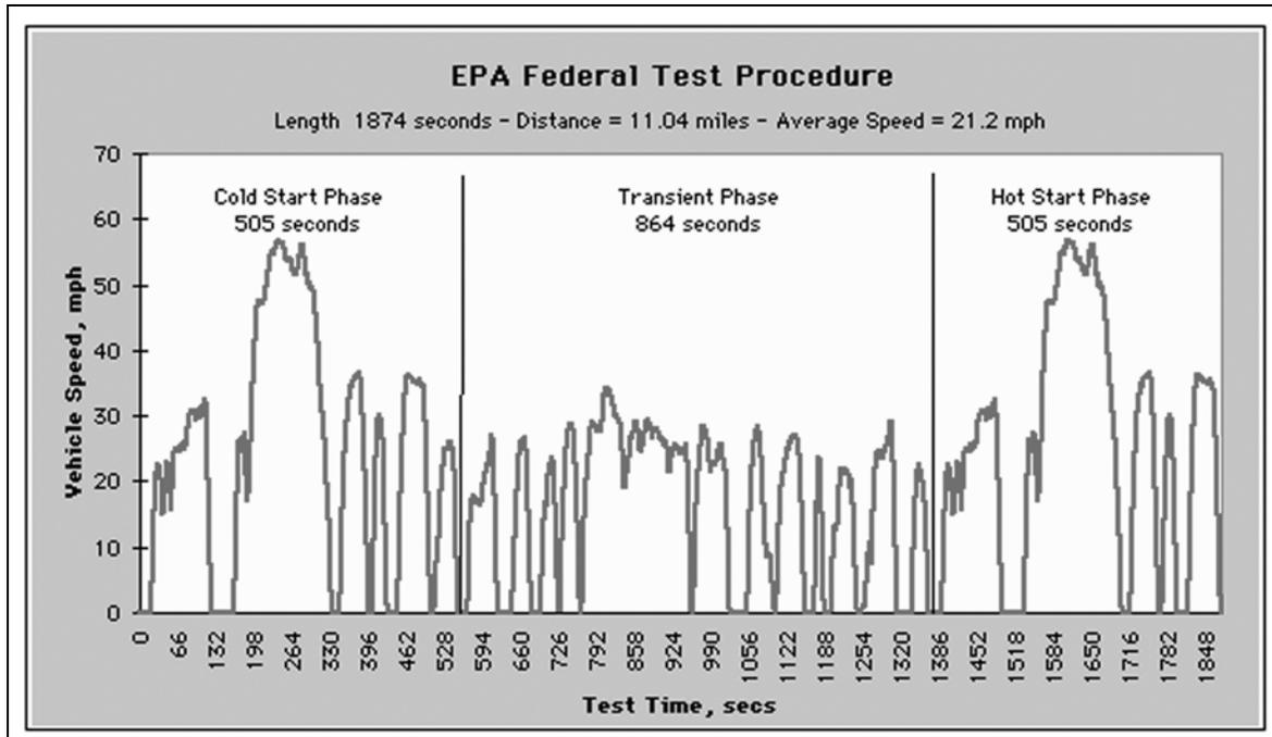
Figure 3 EPA Federal Test Procedure Drive Cycle
