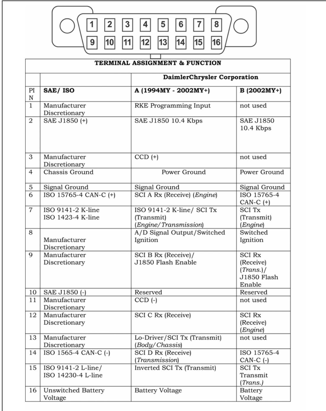
Figure 25 Data Link Connector Pin Locations
