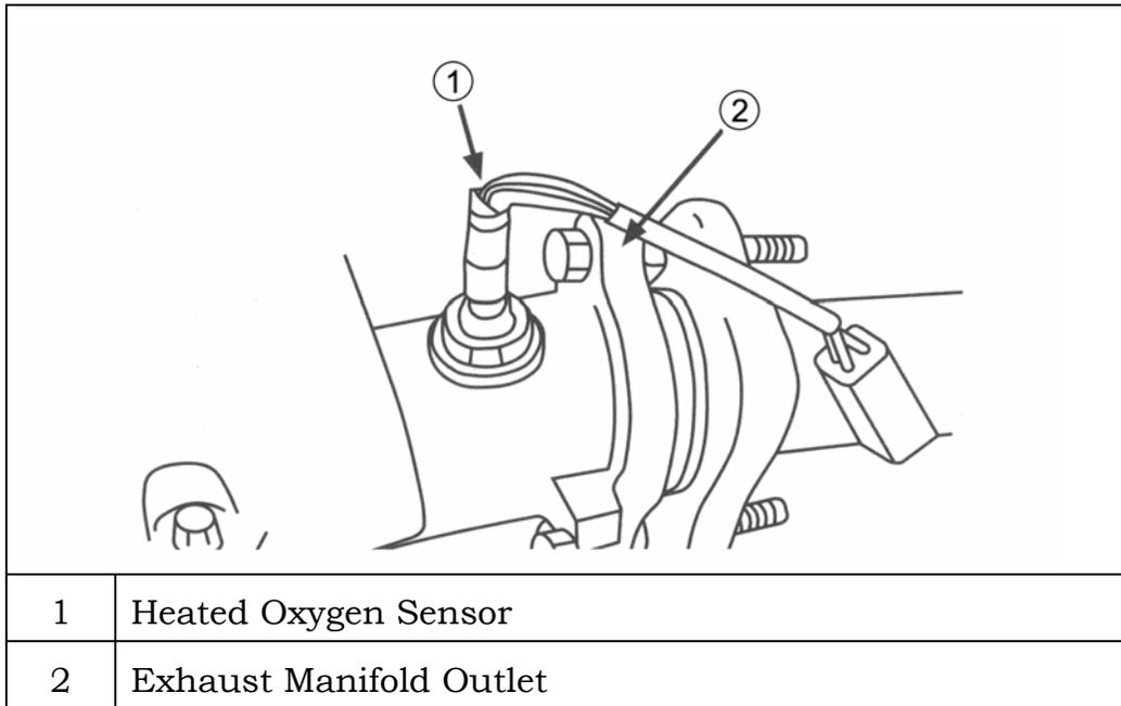
Figure 16 Heated Oxygen Sensor
