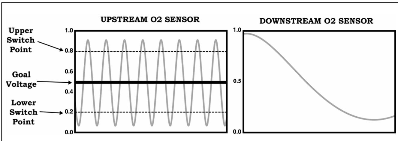
Figure 19 Upstream and Downstream O<sub>2</sub> Sensor Signals
