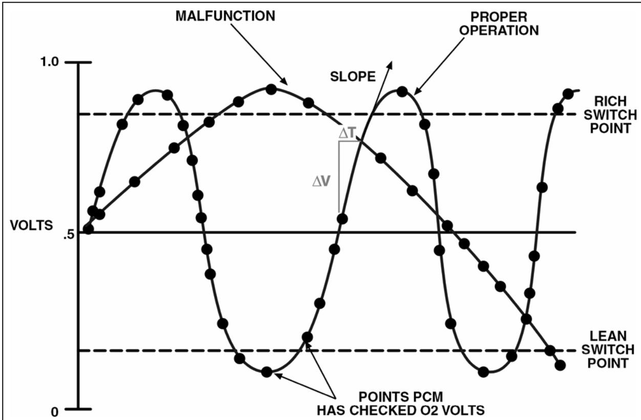
Figure 33 JTEC/SBEC Oxygen Sensor Big Slope
