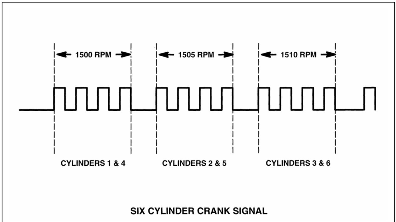
Figure 50 RPM Error
