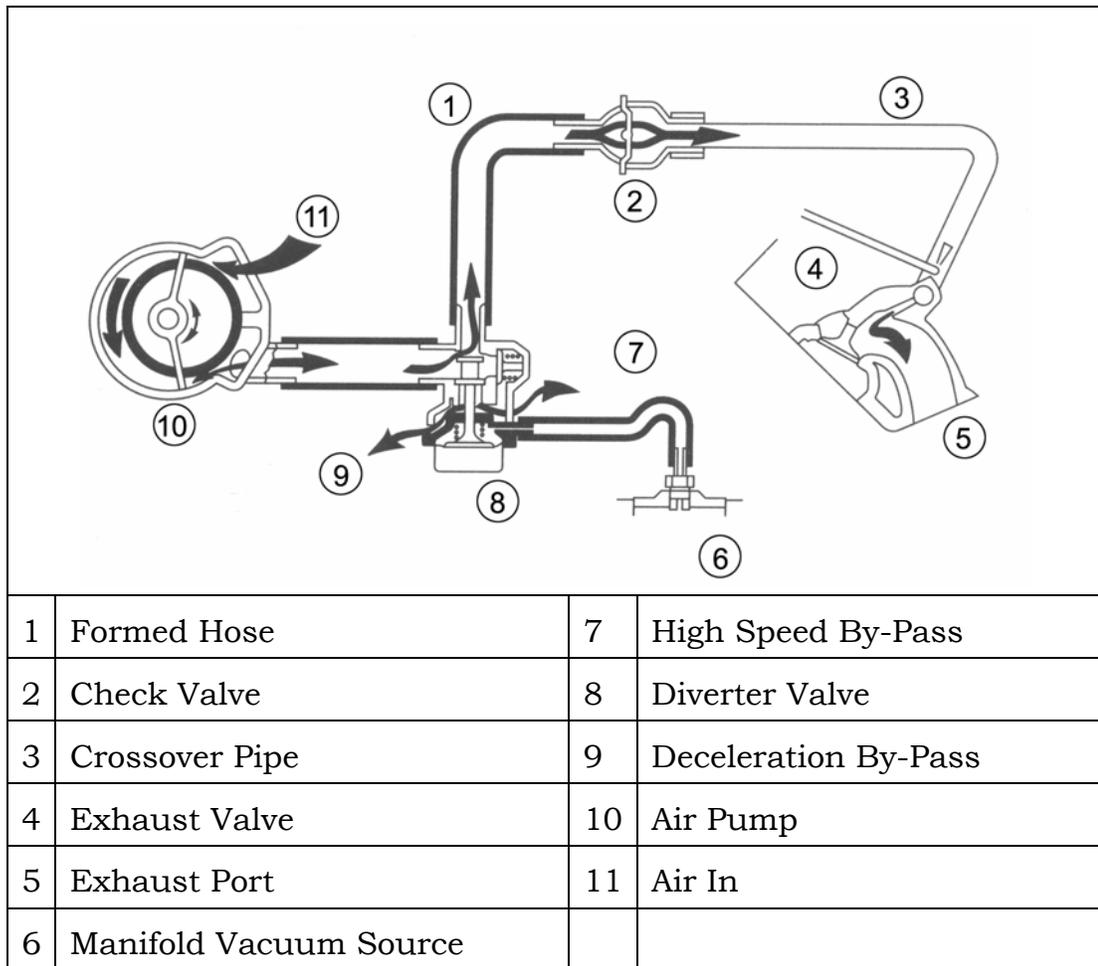
Figure 11 AIR System – Engine Driven Pump
