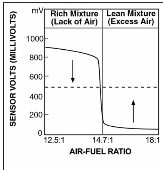
Figure 31 O<sub>2</sub> Sensor Signal
