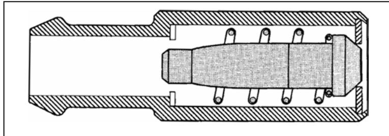
Figure 8 PCV Valve Plunger Back Seated - Closed
