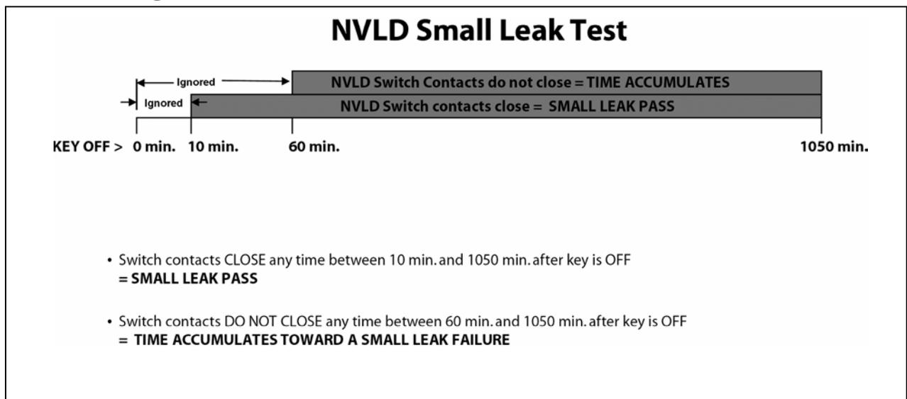
Figure 63 Small Leak Pass or Fail
