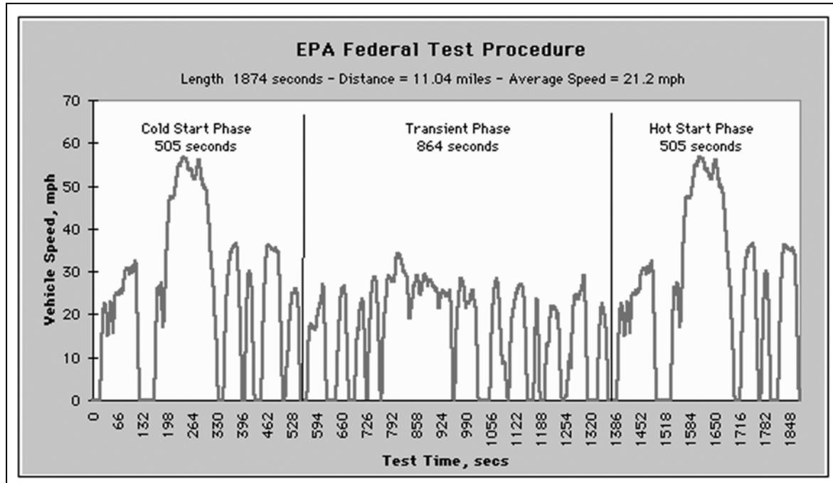
Figure 28 EPA Federal Test Procedure Drive Cycle
