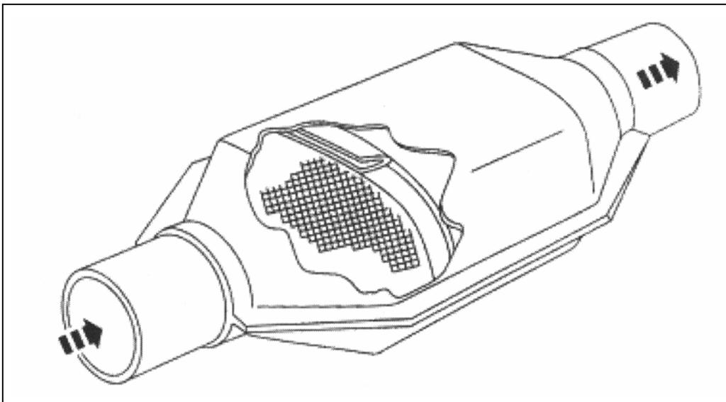
Figure 14 Catalytic Converter
