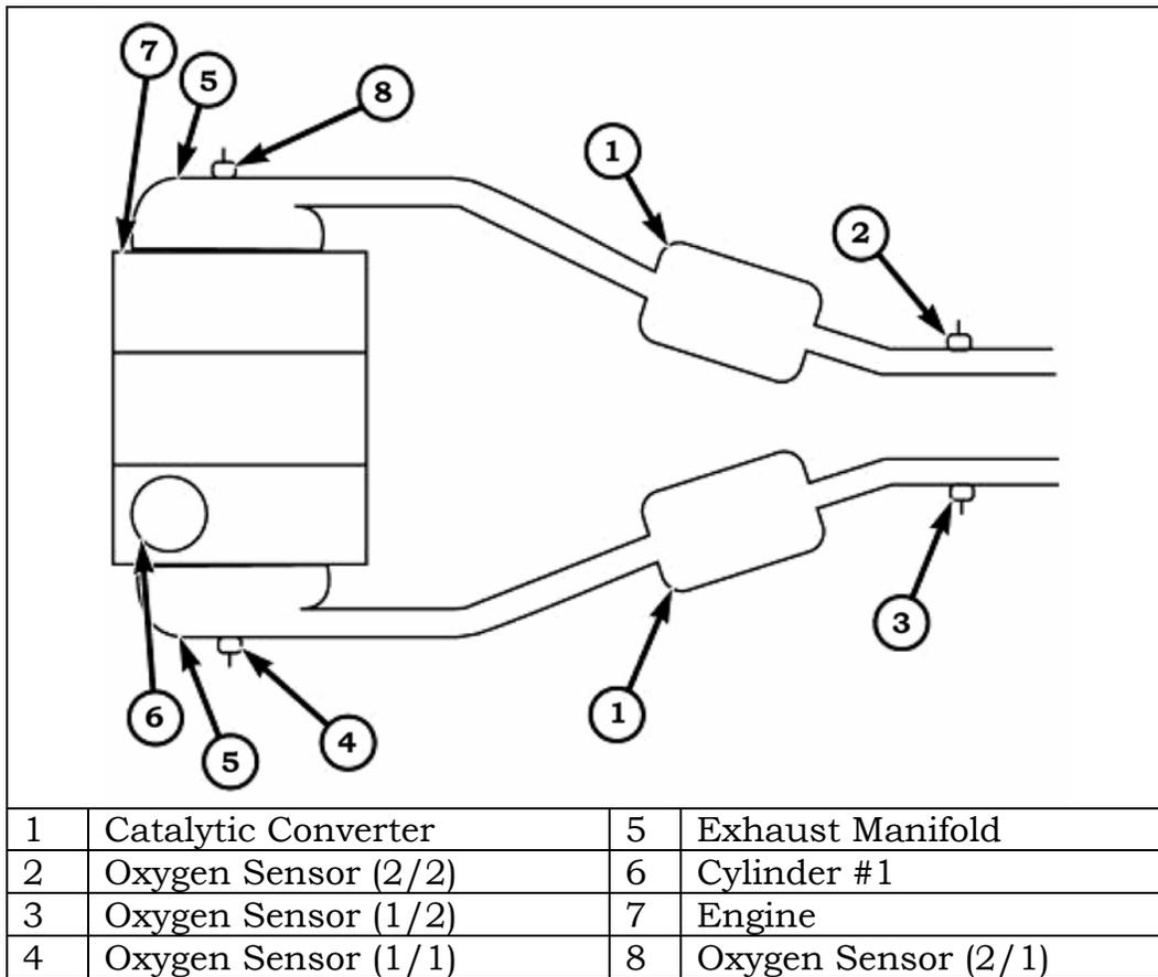
Figure 20 Oxygen Sensor Naming Conventions
