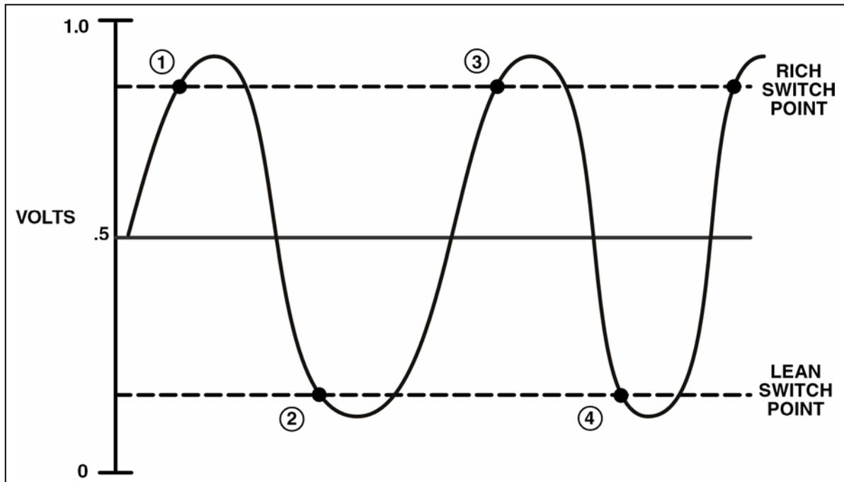
Figure 34 JTEC/SBEC Oxygen Sensor Half Cycles
