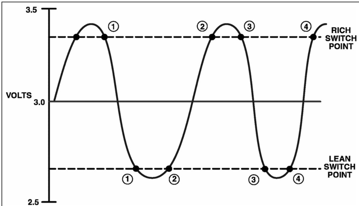
Figure 35 NGC Oxygen Sensor Switch Counts
