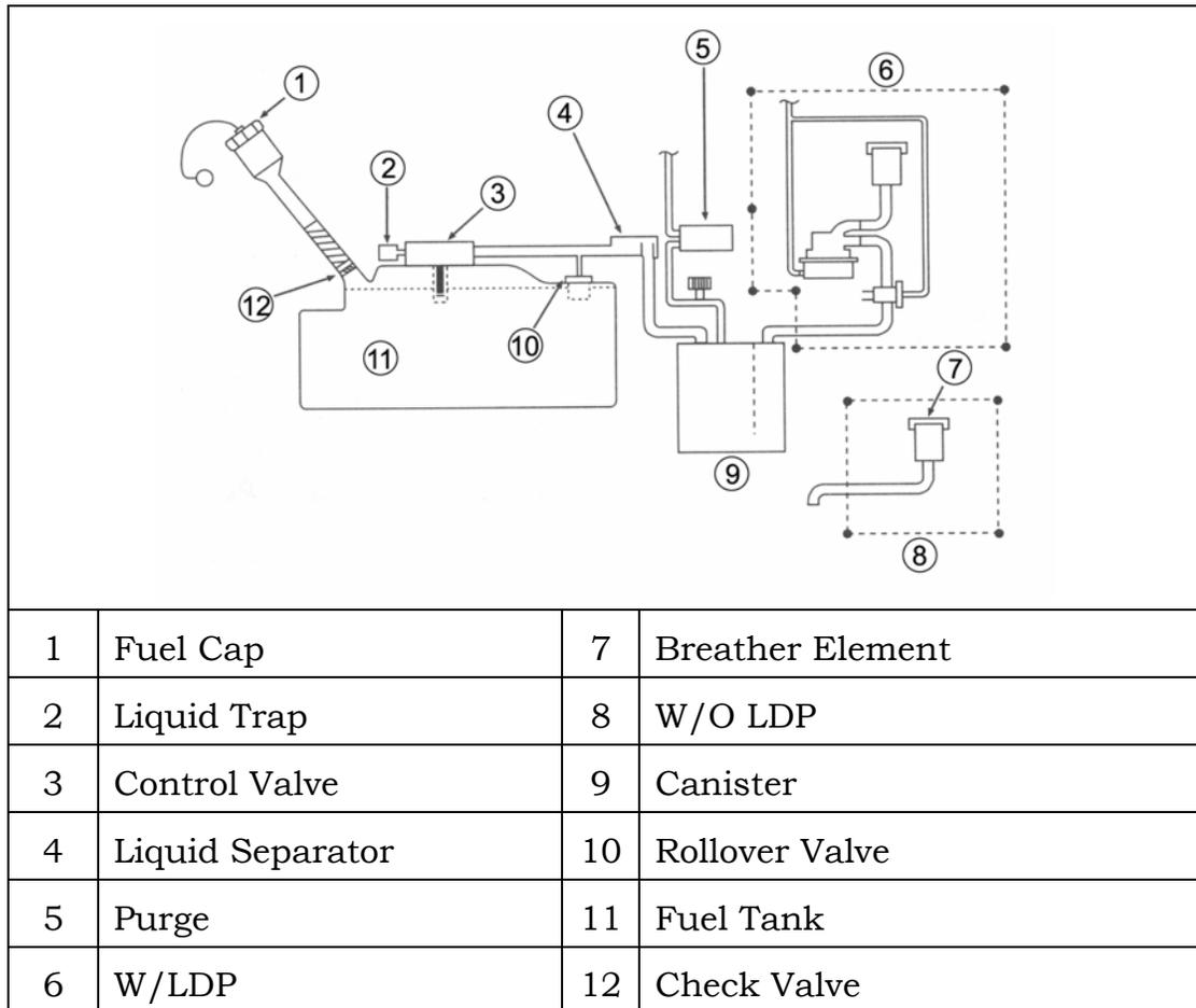
Figure 21 Onboard Refueling Vapor Recovery System
