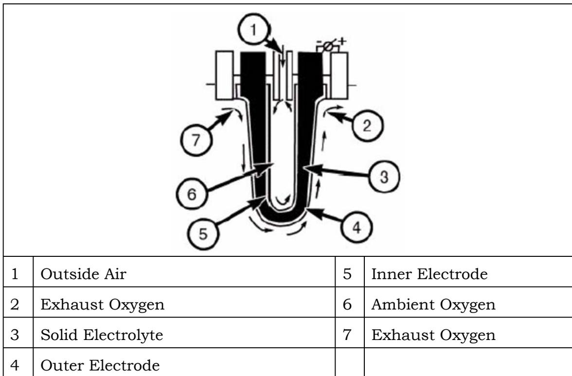
Figure 15 Oxygen Sensor Operation
