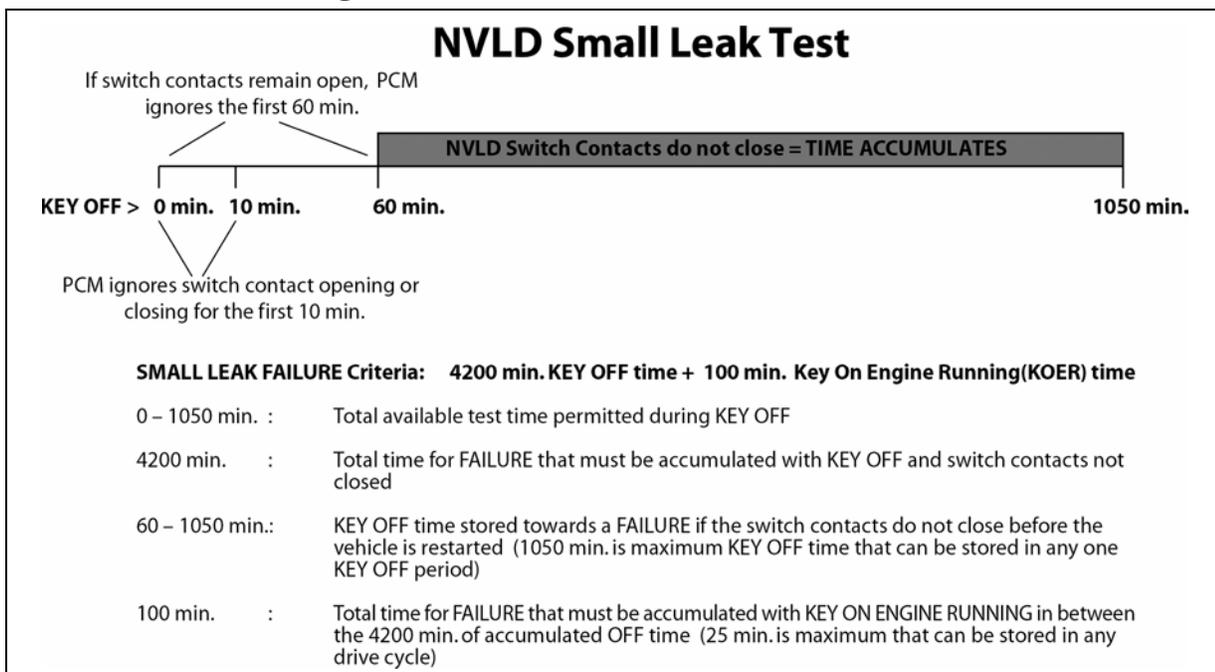
Figure 64 Small Leak Failure Time Thresholds
