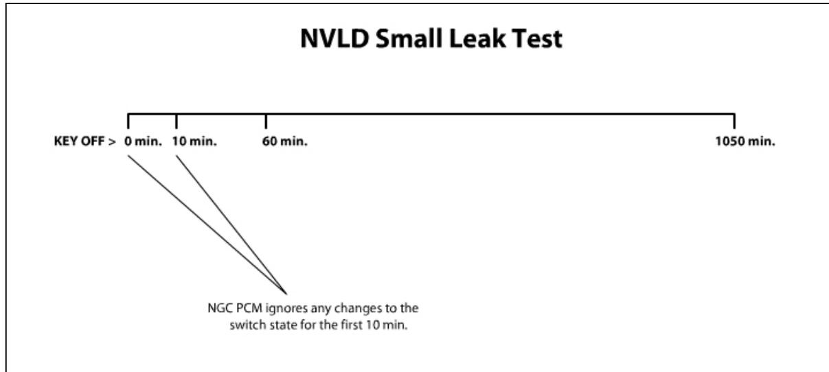
Figure 62 Small Leak Test Main Time Thresholds
