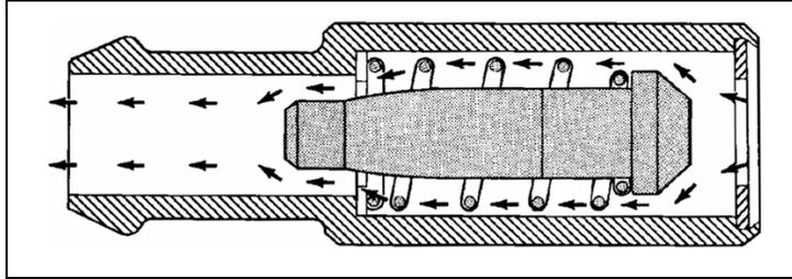
Figure 10 PCV Valve Plunger Mid-Position – High Flow
