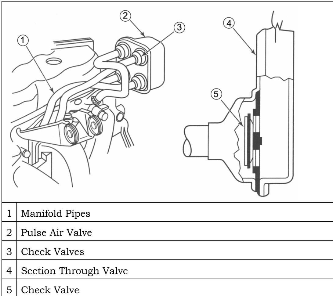
Figure 12 Pulsed AIR System
