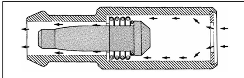
Figure 9 PCV Valve Plunger Front Seated - Low Flow
