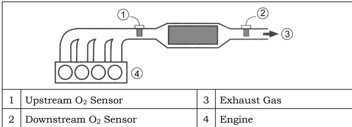
Figure 18 Downstream Oxygen Sensor Location
