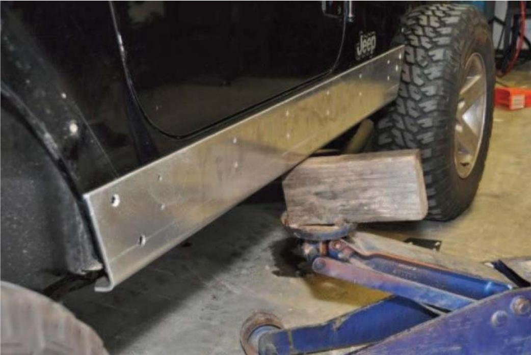
Take your time as this is the single most critical element of the installation. When you drop onto a rock or log with your rig, several thousand pounds of force can be developed that try to force the rail upwards. We are trying to get all the slack out of the rocker when they are installed so when they take hard hits, it will be impossible to move them.
