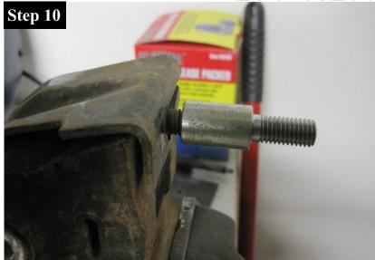
At this point you will need to cut the studs on both motor mounts. Cut each stud so that the 10mm stud extension sits flush against the motor mount. Take care and make your cut straight.
