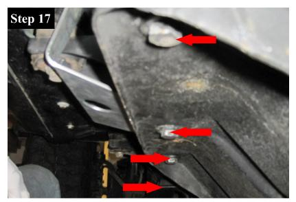
At this point <u>SLOWLY</u> raise the drivetrain at the output shaft of the transfercase so that the transmission studs are clear of the transfercase skid.
