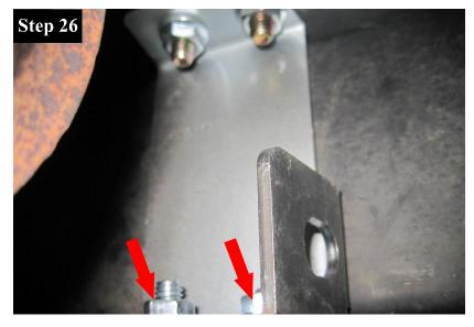
Loosely install the (2) lower 5/16 - 18 X 3/4" Flat Head Phillips Screws with 5/16 - 18 Flange Nuts.
