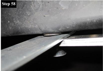
On the driver side of the vehicle, rotate the Wing Spacer (D) outwards and begin tightening the 12mm X 1.75 X 40mm Flat Head Allen Screw. As you tighten the bolt make sure that the Wing Spacer (D) is centered around the frame nutsert.
