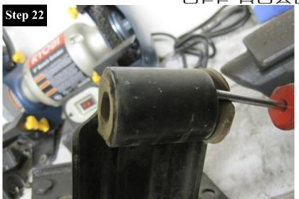
Using a flat head screw driver as a shoehorn, carefully tug the exhaust hanger bushing from the stock transmission mount.
