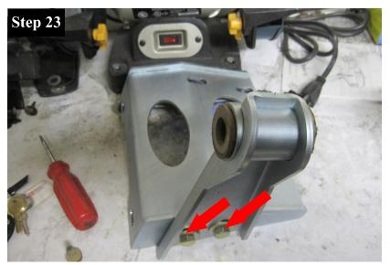
Push the rubber bushing onto the supplied exhaust hanger (L) as shown.
