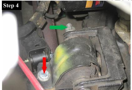
Loosen the motor mount through bolt using 18mm socket (DO NOT REMOVE) shown by the green arrow.
