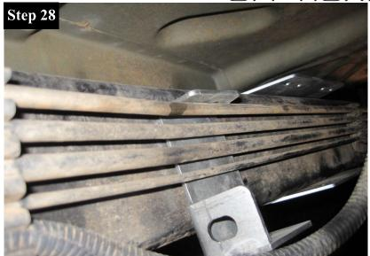
Slide the Frame Inner C Bracket (J) all the way down to the Frame C (I).
