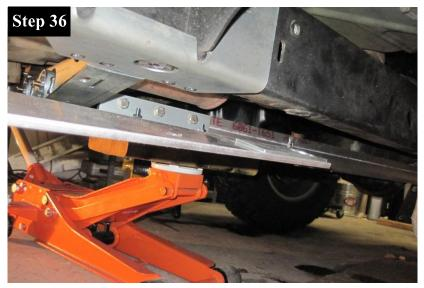
Using a jack you can support the Main Skid (A) with the Wings (C). Slowly raise the assembly and line up the Front Brace (F) and the Crossmember (H).
