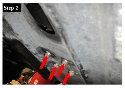
Start by removing each of the four transmission mount nuts on your transfer case skid plate.
