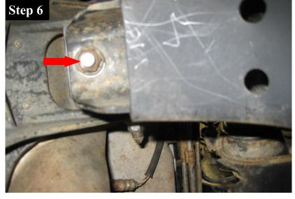
Remove the 13mm nut on the motor mount stud. (red arrow).
