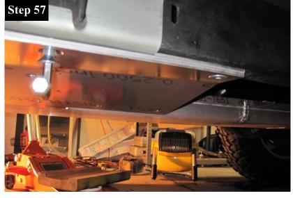
Tighten the middle 12mm X 1.75 X 40mm Flat Head Allen Screw.
