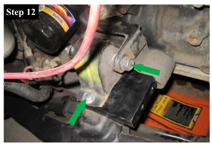
It is now time to install Motor Mount Spacers (G). Both Motor Mount Spacers should be installed with the threaded side facing the front of the vehicle. The L-shaped motor mount spacer should be installed on the passenger side of the vehicle.
