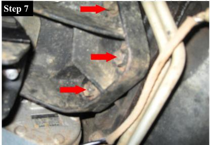
There are 3 bolts that hold the motor mount bracket to the engine. With the engine raised off the frame, start by removing these bolts using a 15mm socket.
