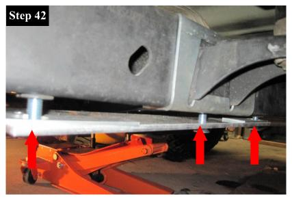
Moving on to the passenger side of the vehicle, loosely install the (3) 12mm X 1.75 X 40mm Flat Head Allen Screws and Wing Spacers (D).
