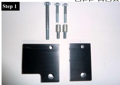
Organize the following components to install the Savvy Motor Mount Lift:
