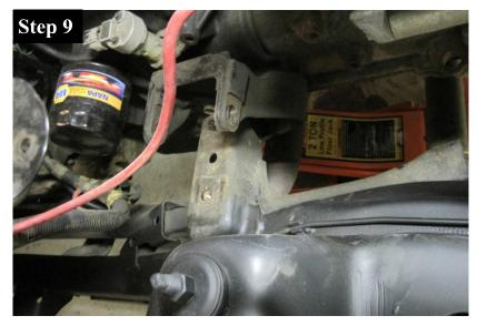
On the passenger side, remove the motor mount through bolt and the motor mount out of the vehicle.
