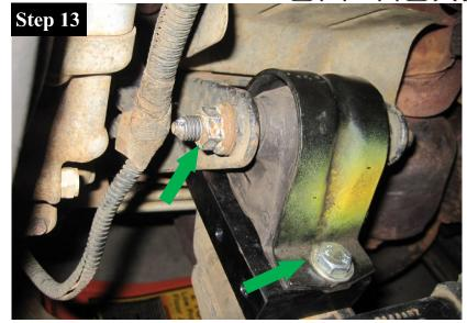
On the driver side of the vehicle, reinstall motor mount bracket if it was removed and torque the 3 bracket bolts to 40 ft-lbs.
