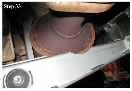
Loosen the two exhaust hangers at the rear of the vehicle. They are located near the passenger rear upper control arm and behind the passenger rear tire.
