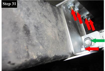
At this point tighten the 1/2 - 13 Flange Nut on each side of the vehicle. (green arrow)
