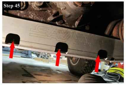
Slip the Rear Brace (M) onto the Main Skid (A). You may have to rotate it around the exhaust system to install it.
