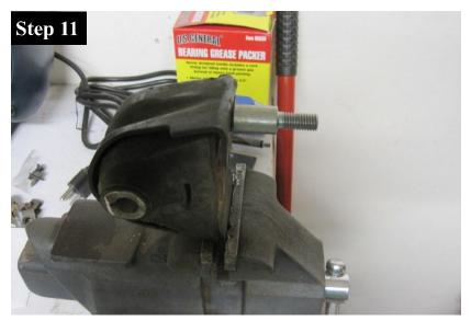
Remove the stud extensions and apply a removable thread locker on the motor mount studs. Tighten the stud extension onto the motor mount studs.
