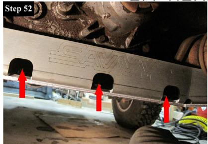
Tighten the (3) 5/16 - 18 X 1" Flat Head Phillips Screws and 5/16 - 18 Flange Nuts.
