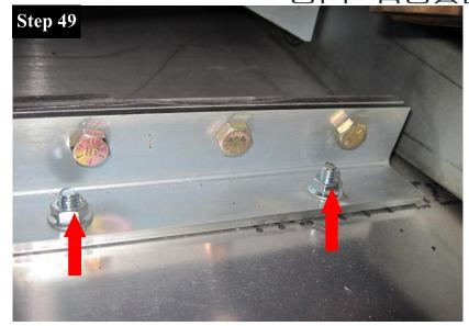
On the driver side, tighten the (2) 5/16 - 18 X 1" Flat Head Phillips Screws and 5/16 - 18 Flange Nuts,
