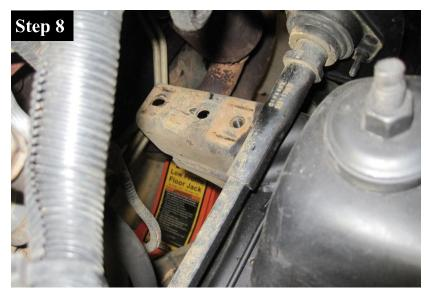
Remove the entire motor mount and engine bracket off the frame and out of the engine bay.
