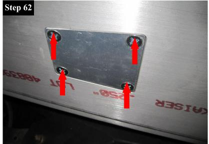
Moving to the middle of the Main Skid (A), install the Drain Cover with the (4) 5/16 - 18 X 1" Flat Head Phillips Screws and (4) 5/16 - 18 Flange Nuts.
