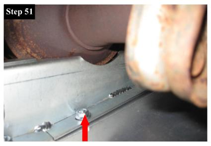
On the passenger side of the vehicle, tighten the (2) 5/16 - 18 X 3/4" Flat Head Phillips Screw and (2) 5/16 - 18 Flange Nuts. One fastener is located behind the exhaust system and is not shown in the picture.
