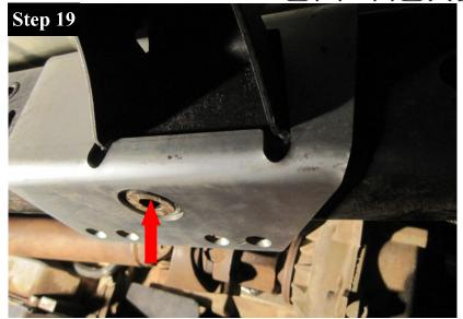
Using a rubber mallet tap the Frame C (I) so that it is centered in the frame nutsert. Now install the passenger side Frame C.
