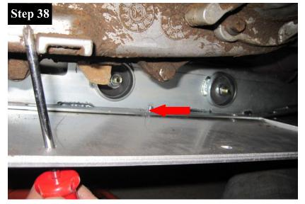
Moving on to the back, you will find it will be initially difficult to line up the fasteners to the Crossmember (H).
