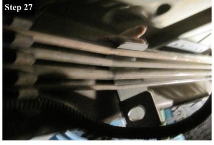
On the driver side, you can slip the Frame Inner C Bracket (J) onto the frame where the frame begins to bend at the rear of the vehicle.
