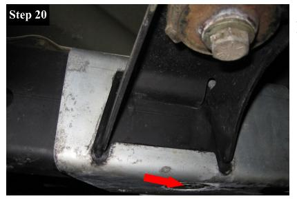
On the passenger side, Using a rubber mallet tap the Frame C (I) so that it is centered in the frame nutsert.
