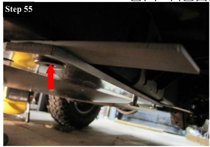
Rotate the Wing Spacer (D) outwards and begin tightening the 12mm X 1.75 X 40mm Flat Head Allen Screw. As you tighten the bolt make sure that the Wing Spacer (D) is centered around the frame nutsert.
