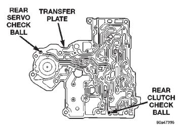
Fig. 56 Rear Servo and Rear Clutch Check Balls
