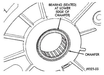
Fig. 48 Output Shaft Rear Bearing Installation Depth
