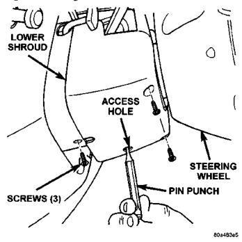
Fig. 13 Steering Column Shrouds Remove/Install
