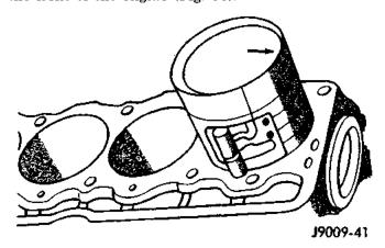
Fig. 56 Rod and Piston Assembly Installation
