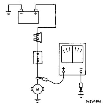
Fig. 8 Testing for Voltage
