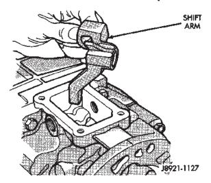
Fig. 42 Position Shift Arm in Transmission Case
