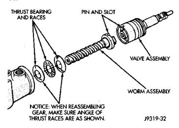
Fig. 14 Bearing, Worm and Valve Assembly
