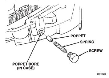
Fig. 23 Detent Plug, Spring And Plunger Removal
