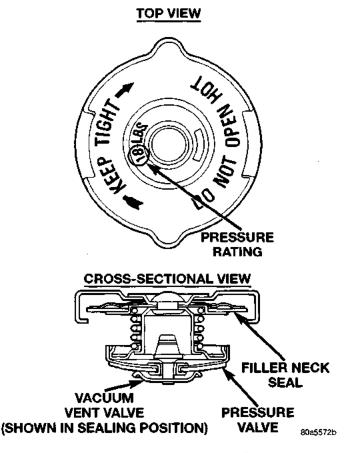
Fig. 17 Radiator Pressure Cap
