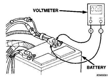
Fig. 3 Test Battery Positive Connection Resistance -Typical
