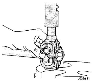
Fig. 29 Press In Bearing Assembly
