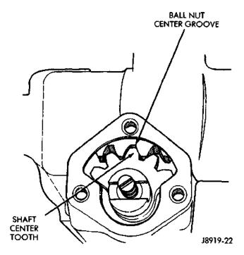
Fig. 8 Pitman Shaft and Ball Nut
