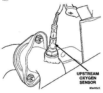
Fig. 41 Upstream Oxygen Sensor Location
