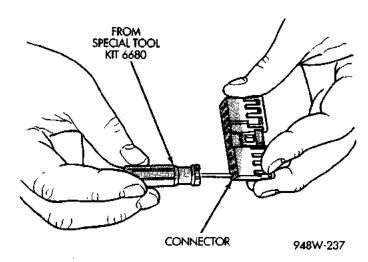
Fig. 19 Terminal Removal Using Special Tool
