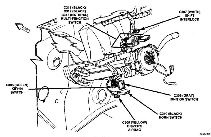
Fig. 16 Steering Column Connectors
