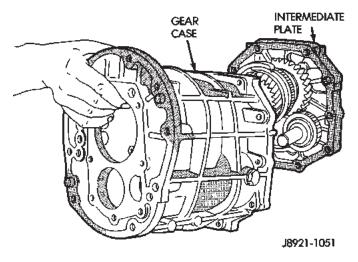
Fig. 37 Install Transmission Gear Case to the Intermediate Plate
