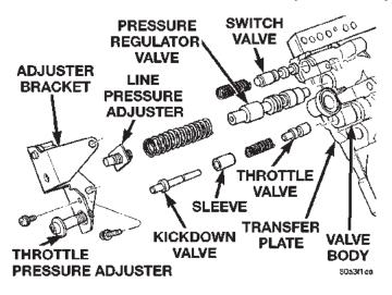
Fig. 68 Adjusting Screw Bracket, Springs, and Valves
