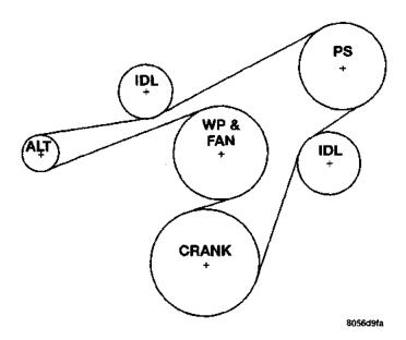
Fig. 34 Vehicles with 2.5L or 4.0L Engine–Without A/C
