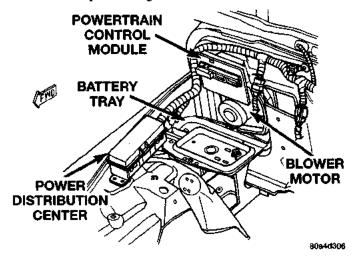
Fig. 26 Blower Motor Remove/Install
