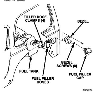
Fig. 22 Fuel Filler Hoses/Fuel Fill Cap
