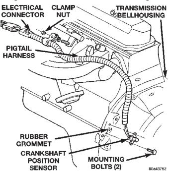
Fig. 8 Crankshaft Position Sensor —4.0L Engine
