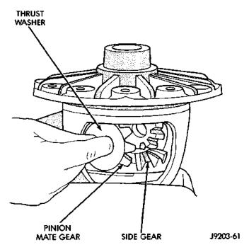
Fig. 45 Pinion Mate Gear Removal
