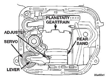
Fig. 80 Rear Band Adjuster Location
