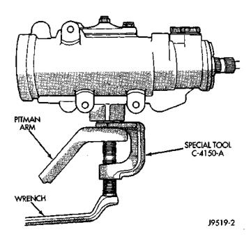
Fig. 2 Pitman Arm Puller
