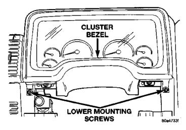
Fig. 5 Cluster Bezel Lower Screws Remove/Install
