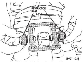
Fig. 23 Shift Arm Rstrictor Pins
