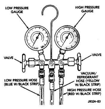
Fig. 4 Manifold Gauge Set
