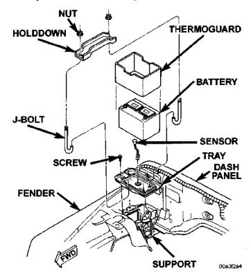
Fig. 12 Battery Hold-down
