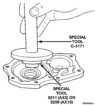
Fig. 11 Install Front Bearing Retainer Seal
