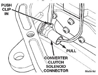
Fig. 27 Solenoid Wire Connector
