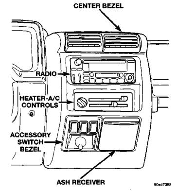
Fig. 9 Center Bezel Remove/Install
