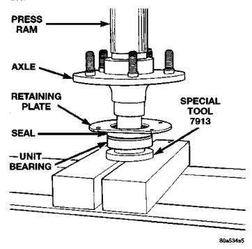
Fig. 19 Press Bearing On Axle
