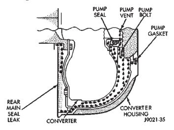
Fig. 11 Converter Housing Leak Paths
