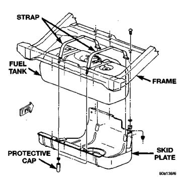
Fig. 7 Fuel Tank Skid Plate
