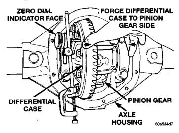
Fig. 75 Hold Differential Case and Zero Dial Indicator
