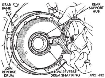
Fig. 81 Low-Reverse Drum Snap Ring
