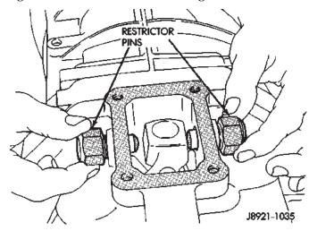
Fig. 43 Install Shifter Restrictor Pins
