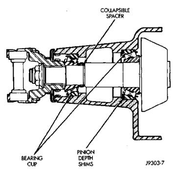
Fig. 1 Axle Adjustment Shims and Spacer
