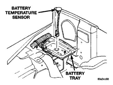
Fig. 5 Battery Temperature Sensor Remove/Install
