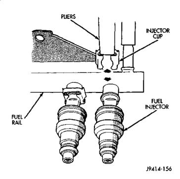
Fig. 21 Injector Retaining Clips—Typical Injector
