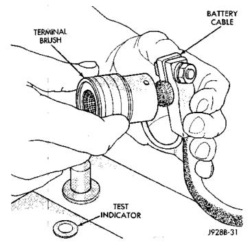
Fig. 11 Clean Battery Cable Terminal Clamp -Typical
