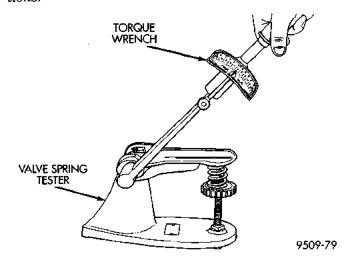
Fig. 57 Valve Spring Tester
