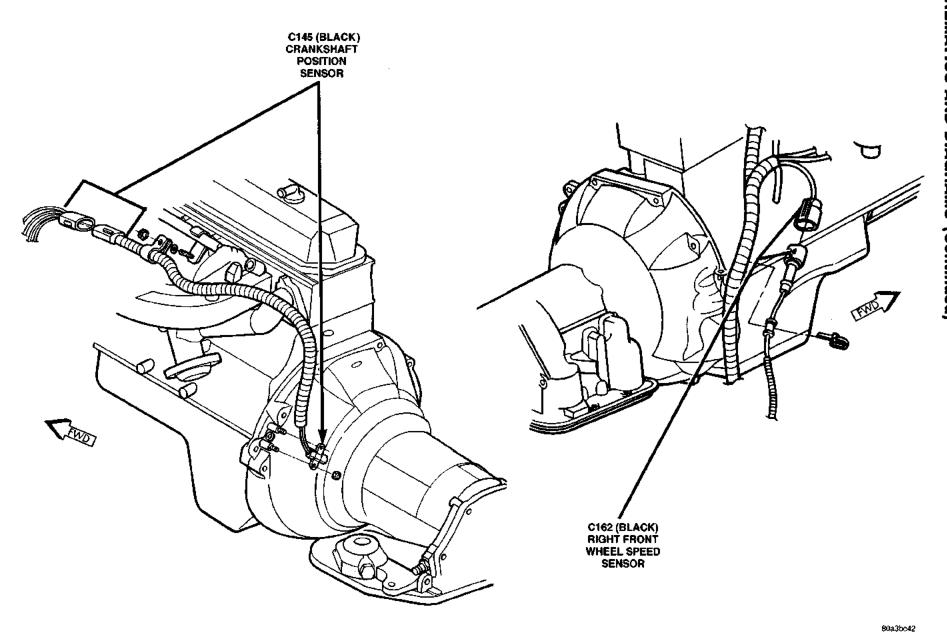
Fig. 11 Crankshaft Position Sensor and Right Front Wheel Speed Sensor
