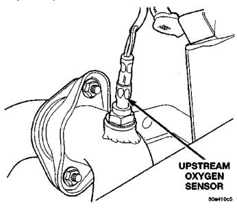
Fig. 21 Upstream Oxygen Sensor
