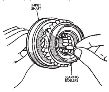
J8921-64 Fig. 100 Install Output Shaft Pilot Bearing Rollers
