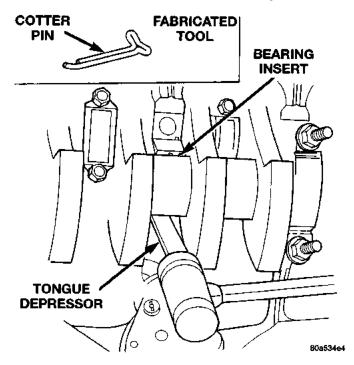
Fig. 44 Removing Upper Inserts
