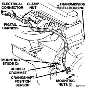
Fig. 20 Crankshaft Position Sensor—2.5L 4-Cyl. Engine—Auto. Trans.
