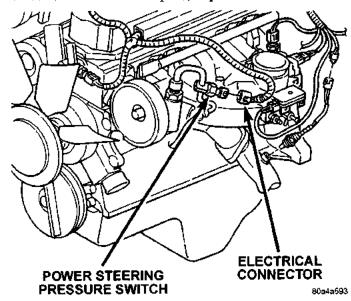
Fig. 32 Power Steering Pump Pressure Switch
