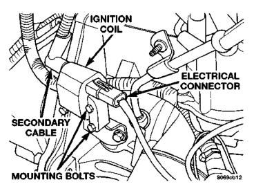
Fig. 11 Ignition Coil—2.5L Engine
