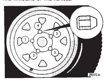
Fig. 5 Lug Nut Tightening Pattern
