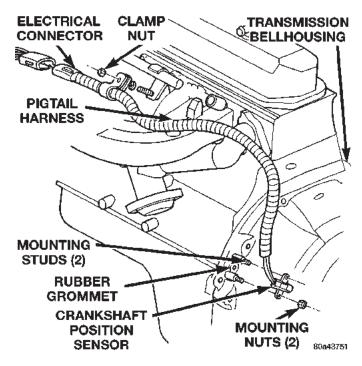
Fig. 7 Crankshaft Position Sensor—2.5L Engine
