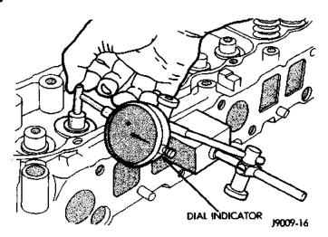
Fig. 61 Measurement of Lateral Movement Of Valve Stem
