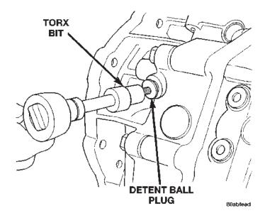
Fig. 46 Install Detent Ball Plug
