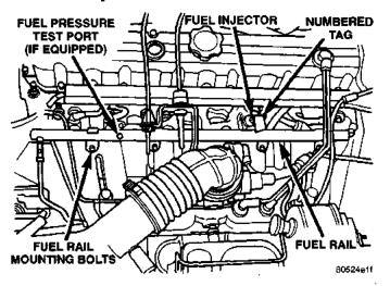
Fig. 4 Fuel Injectors—Typical—4.0L Shown
