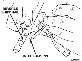
Fig. 71 Remove Interlock Pin From Reverse Shift Rail
