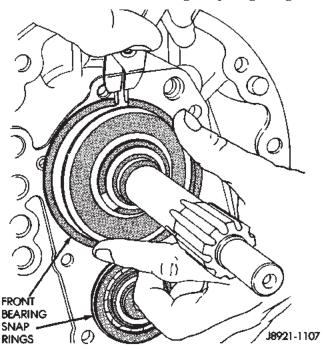
Fig. 35 Install Front Bearing Snap-rings
