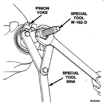
Fig. 47 Pinion Yoke Installation
