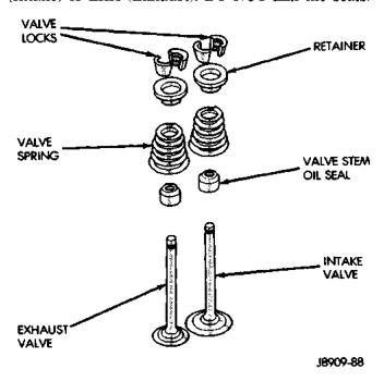
Fig. 25 Valve and Valve Components
