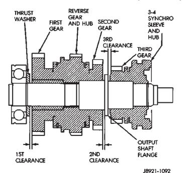
Fig. 123 Check First-Second Gear Thrust Clearance
