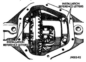
Fig. 27 Differential Bearing Cap Reference Letters
