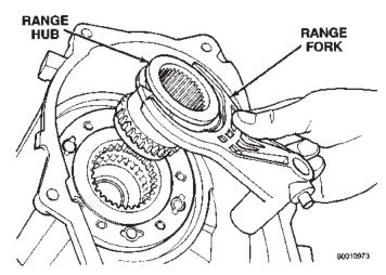
Fig. 25 Range Fork And Hub Removal
