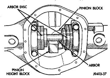
Fig. 71 Gauge Tools In Housing—Typical
