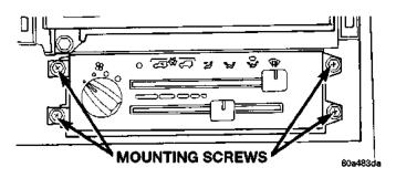
Fig. 28 Heater-A/C Control Remove/Install
