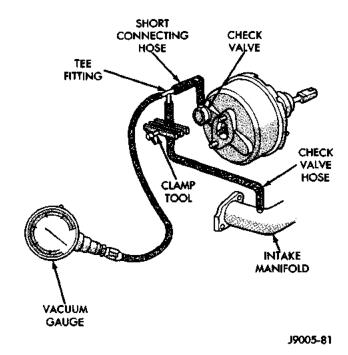
Fig. 8 Typical Booster Vacuum Test Connections
