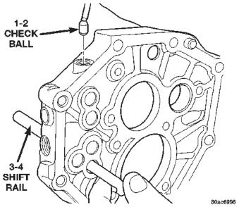
Fig. 76 Install 1-2 Check Ball
