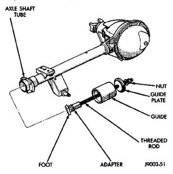
Fig. 16 Axle Shaft Bearing Removal Tool
