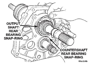
Fig. 80 Remove Output Shaft Rear Bearing Snap-ring
