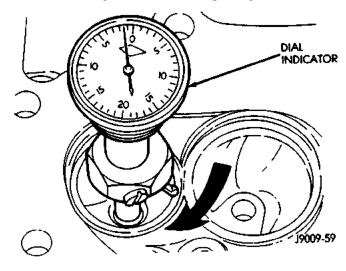
Fig. 54 Measurement of Valve Seat Runout
