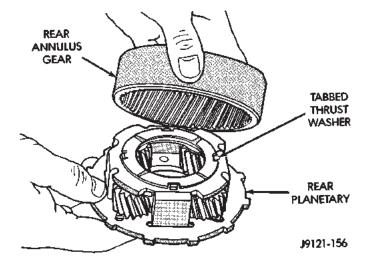
Fig. 149 Assembling Rear Annulus And Planetary Gear
