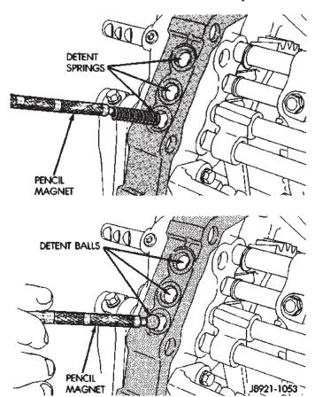
Fig. 104 Install Detent Balls And Springs
