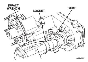
Fig. 15 Yoke Nut Removal
