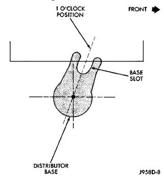
Fig. 48 Distributor Pre-position—All Engines
