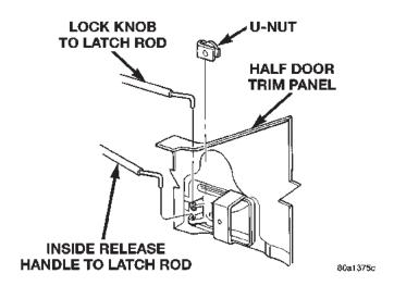
Fig. 40 Inside Handle Actuator
