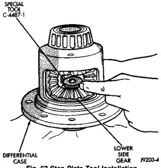
Fig. 52 Step Plate Tool Installation
