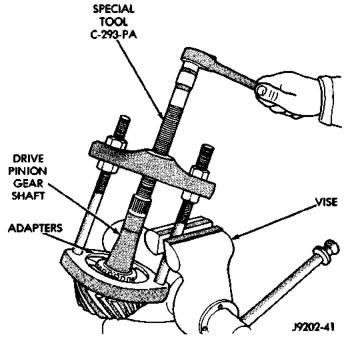
Fig. 32 Inner Bearing Removal
