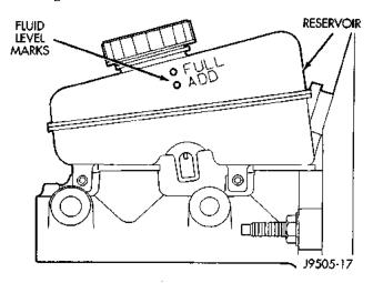
Fig. 12 Master Cylinder Fluid Level
