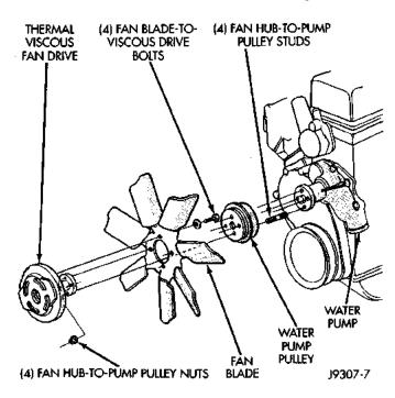
Fig. 9 Water Pump Mounted Fan Drive
