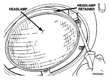
Fig. 2 Headlamp Retaining Ring
