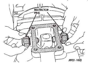
Fig. 46 Install Shifter Restrictor Pins
