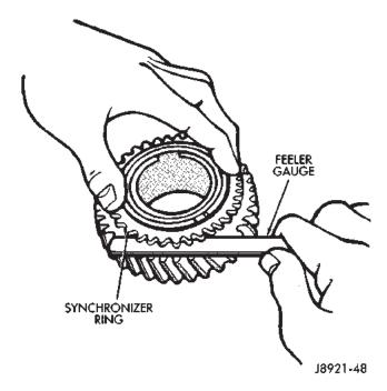
Fig. 127 Check Synchronizer Ring Wear
