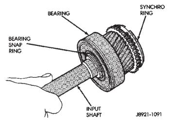
Fig. 108 Input Shaft Components
