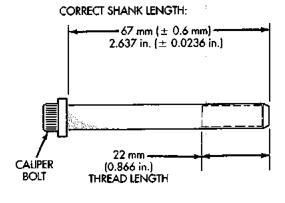
Fig. 31 Mounting Bolt Dimensions
