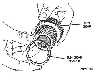
Fig. 152 Installing Spacer On Sun Gear
