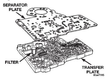
Fig. 49 Transfer And Separator Plates
