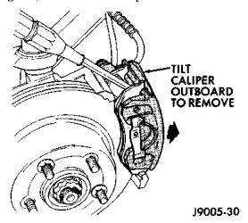
Fig. 26 Caliper Removal
