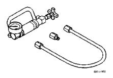
Analyzer Set, Power Steering Flow/Pressure 6815
