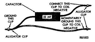
Fig. 15 Special Jumper Ground-to-Coil Negative
