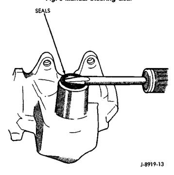
Fig. 6 Pitman Shaft Seal
