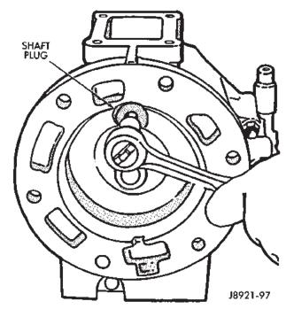
Fig. 45 Shifter Arm Shaft Plug Installation
