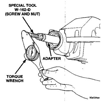
Fig. 46 Check Pinion Gear Rotation Torque
