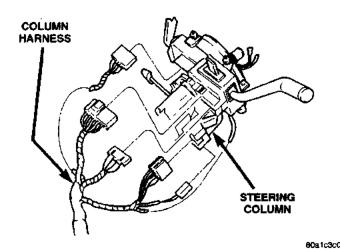
Fig. 4 Steering Column Harness
