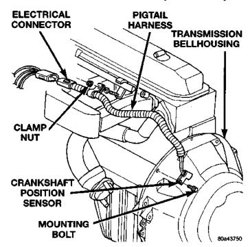
Fig. 19 Crankshaft Position Sensor—4.0L 6-Cyl. Engine—Auto. Trans.
