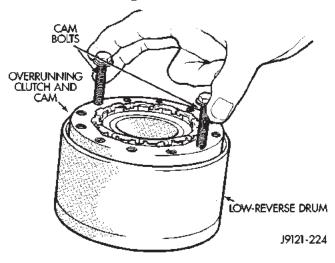
Fig. 111 Removing Overrunning Clutch From Low-Reverse Drum
