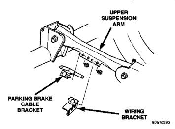
Fig. 4 Parking Brake Cable/Bracket And Wiring Bracket
