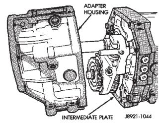
Fig. 27 Remove Adapter/Extension Housing-Typical
