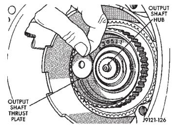
Fig. 99 Output Shaft Thrust Plate
