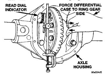
Fig. 74 Hold Differential Case and Read Dial Indicator
