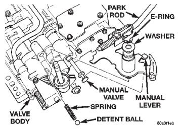
Fig. 66 Manual And Throttle Levers
