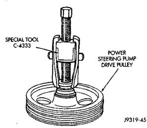
Fig. 5 Pulley Removal
