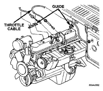
Fig. 27 Throttle Cable Routing
