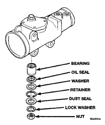
Fig. 25 Pitman Shaft Seals & Bearing
