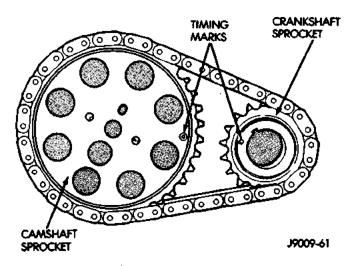
Fig. 36 Timing Chain Alignment—Typical
