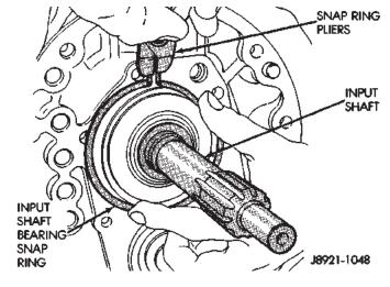
Fig. 32 Remove Input Shaft Bearing Snap-ring
