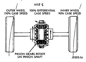
Fig. 3 Differential Operation—On Turns
