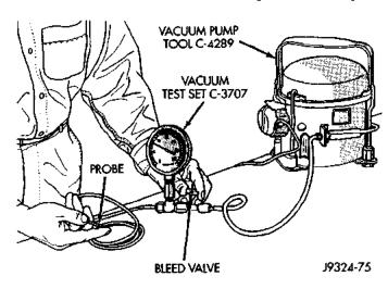
Fig. 6 Adjust Vacuum Test Bleed Valve
