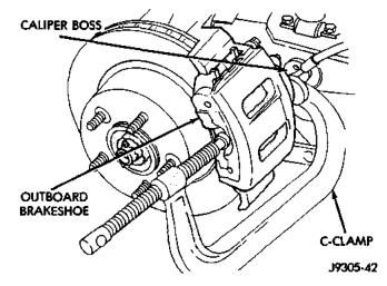
Fig. 24 Bottoming Caliper Piston With C-Clamp
