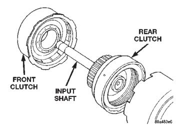
Fig. 98 Front and Rear Clutches
