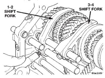
Fig. 87 Install Shift Fork Bolts
