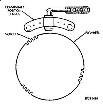
Fig. 7 Sensor Operation—4.0L 6-Cyl. Engine— Manual Transmission
