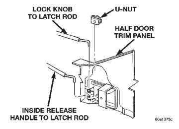
Fig. 27 Inside Handle Actuator
