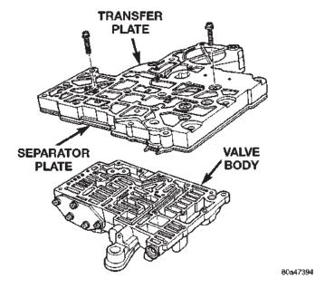
Fig. 59 Valve Body Transfer Plate Screws
