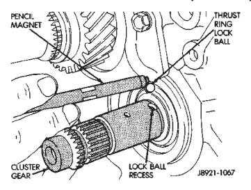
Fig. 95 Install Fifth Gear Thrust Ring Lock Ball
