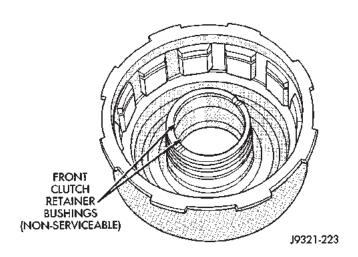
Fig. 174 Retainer Bushing Location/Inspection
