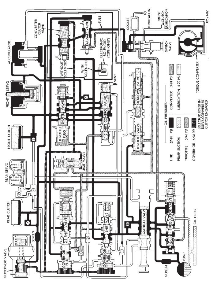
HYDRAULIC FLOW IN D-THIRD GEAR (CONVERTER CLUTCH APPLIED)
