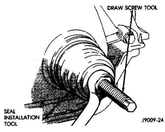
Fig. 34 Timing Case Cover Oil Seal Installation
