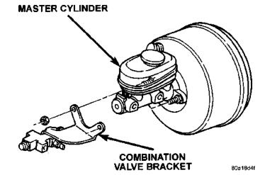
Fig. 20 Combination Valve Bracket
