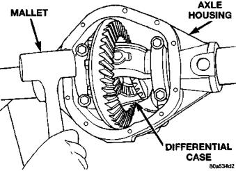
Flg. 76 Seat Pinion Gear Side Differential Dummy Side Bearing
