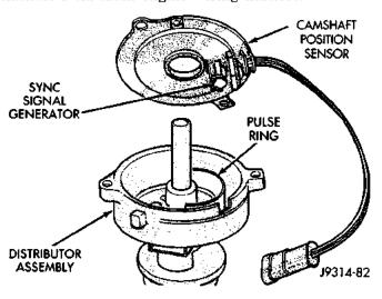
Fig. 41 Camshaft Position Sensor
