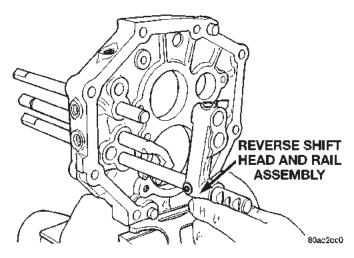
Fig. 69 Remove Reverse Shift Head And Rail Assembly
