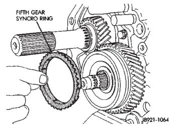
Fig. 57 Remove Fifth Gear Synchro Ring
