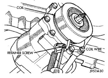
Fig. 17 Clutch Coll Lead Wire
