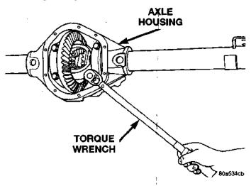
Fig. 28 Tighten Differential Bearing Cap Bolts
