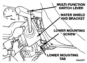
Fig. 6 Water Shield Lower Screw Remove/Install
