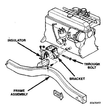
Fig. 20 Right Front Engine Mount
