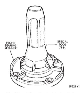
Fig. 53 Install Front Bearing Retainer Seal
