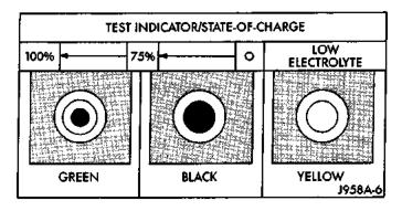
Fig. 3 Built-In Test Indicator Sight Glass
