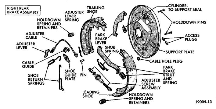
Flg. 33 Drum Brake Components—Typical
