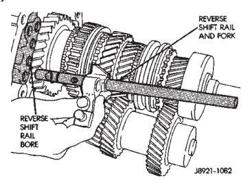
Fig. 83 Install Reverse Shift Rail
