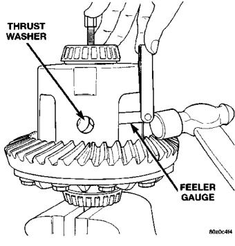
Fig. 55 Remove Pinion Thrust Washer
