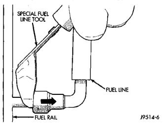
Fig. 10 Fuel Line Disconnection-Typical
