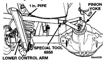
Fig. 30 Pinion Yoke Holder
