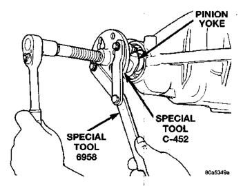
Fig. 8 Pinion Yoke, Remove
