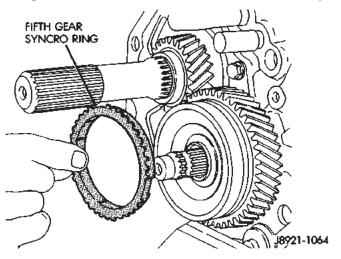
Fig. 99 Install Fifth Gear Synchronizer Ring
