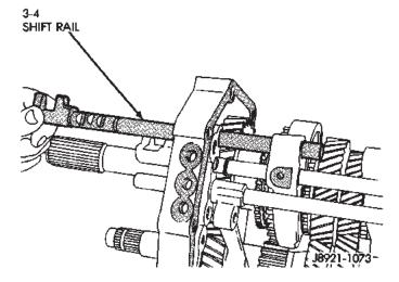
Fig. 89 Install 3-4 Shift Rail
