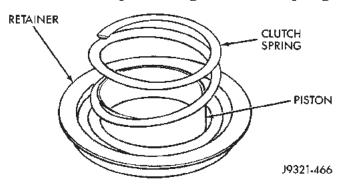
Fig. 134 Clutch Piston Spring Installation
