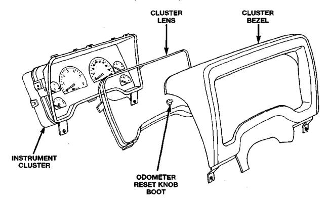
Fig. 7 Instrument Cluster Components
