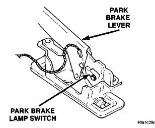
Fig. 36 Parking Brake Lamp Switch
