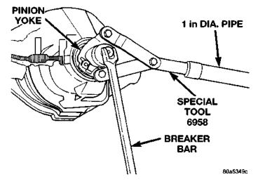
Fig. 8 Pinion Nut
