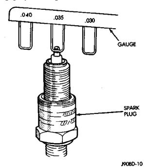
Fig. 34 Setting Spark Plug Gap—Typical
