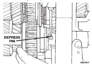
Fig. 92 Depress Pin In Reverse Idler Gear Shaft
