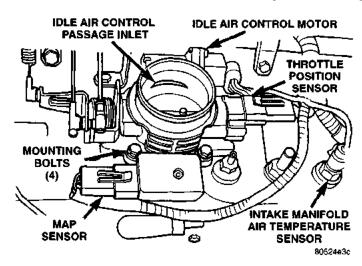
Fig. 45 Intake Air Sensor Location—Typical—4.0L Shown
