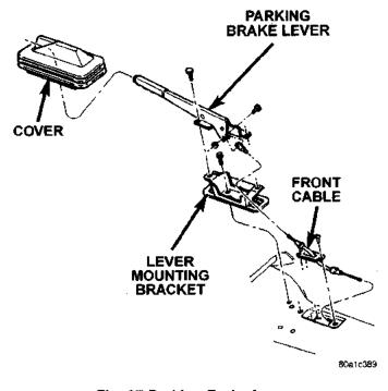
Fig. 37 Parking Brake Lever
