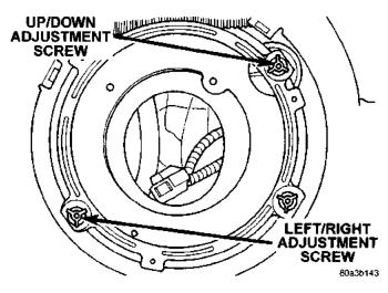
Fig. 2 Headlamp Adjustment Screws
