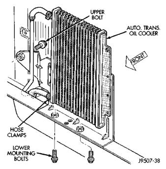
Fig. 20 Auxiliary Air-To-Oil Cooler COOLANT RESERVE/OVERFLOW BOTTLE
