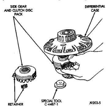
Fig. 62 Side Gear & Clutch Disc Removal
