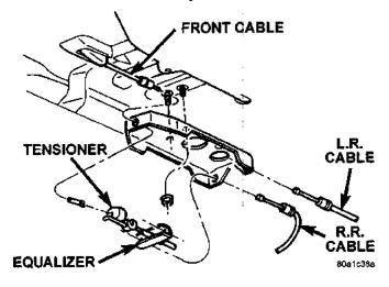
Fig. 35 Parking Brake Cable Attachment
