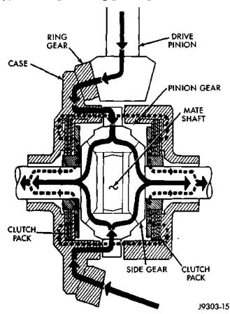
Fig. 4 Trac-lok Limited Slip Differential Operation
