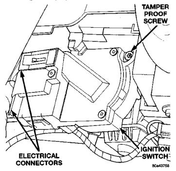
Fig. 53 Ignition Switch Removal/Installation
