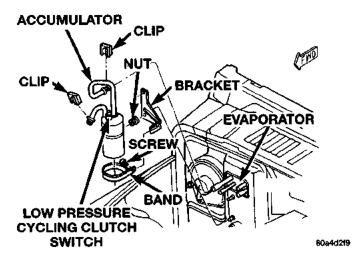
Fig. 25 Accumulator Remove/Install
