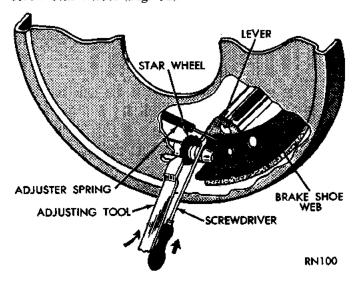
Fig. 61 Brake Adjustment
