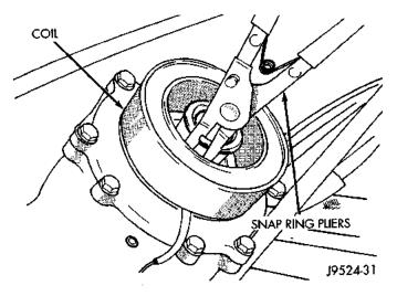
Fig. 18 Clutch Field Coll Snap Ring Remove
