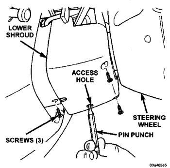
Fig. 13 Steering Column Shrouds Remove/Install
