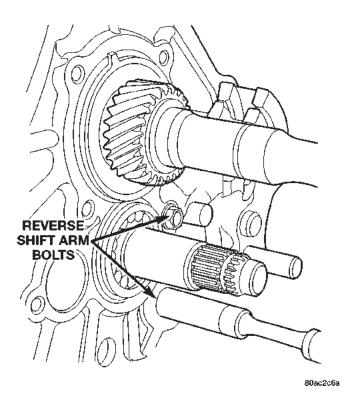
Fig. 60 Remove Reverse Shift Arm Bracket Bolts
