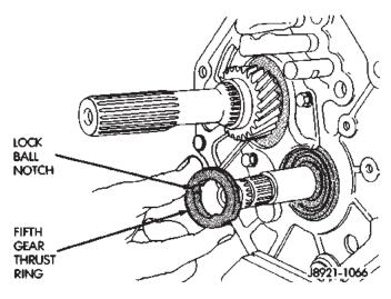
Fig. 55 Remove Fifth Gear Thrust Ring
