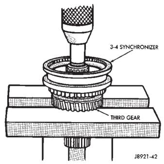
Fig. 107 Remove 3-4 Synchronizer And Third Gear
