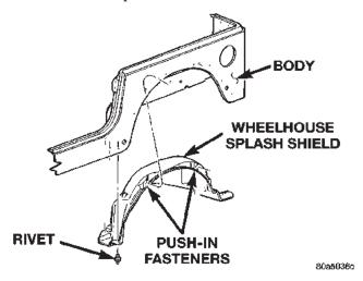
Fig. 73 Wheelhouse Splash Shield
