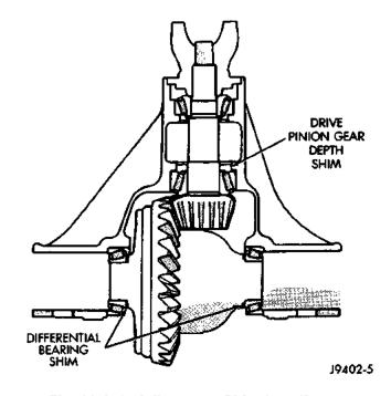
Fig. 68 Axle Adjustment Shim Locations
