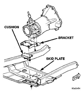
Fig. 21 Rear Mount (Manual Transmission)
