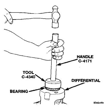
Fig. 30 Install Differential Side Bearings
