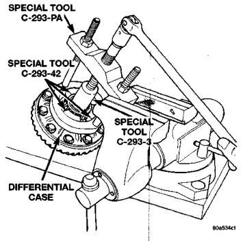
Fig. 29 Differential Bearing Removal
