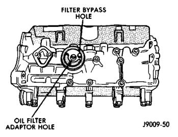
Fig. 63 Oil Filter Adaptor Hole
