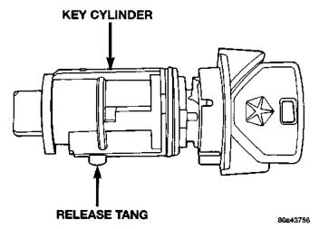
Fig. 51 Key Cylinder Release Tang
