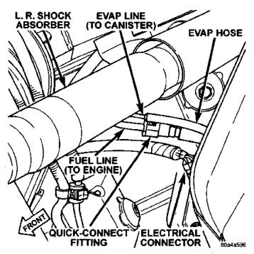
Fig. 23 Fuel Tank Connections
