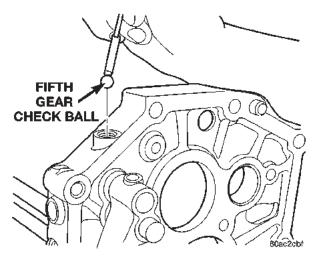
Fig. 68 Remove Fifth Gear Check Ball
