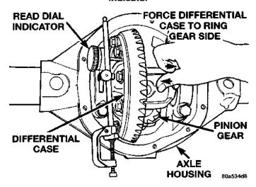
Fig. 76 Hold Differential Case and Read Dial Indicator
