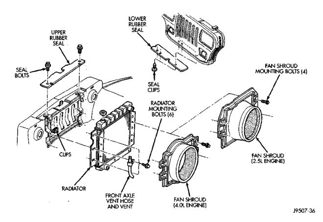
Fig. 30 Radiator—Remove/Install
