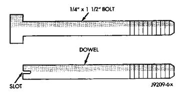
Fig. 38 Fabrication of Alignment Dowels
