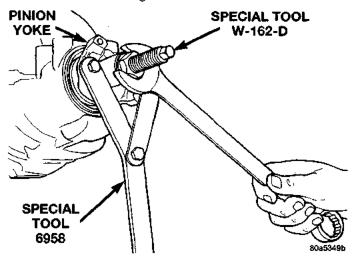
Fig. 12 Pinion Yoke, Install
