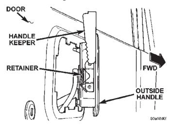
Fig. 23 Outside Door Handle Removal
