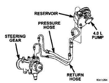
Fig. 1 Power Steering Gear & Pump-4.0L
