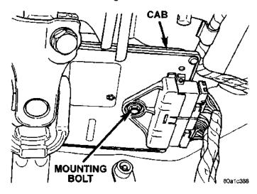
Fig. 6 Controller Antilock Brakes
