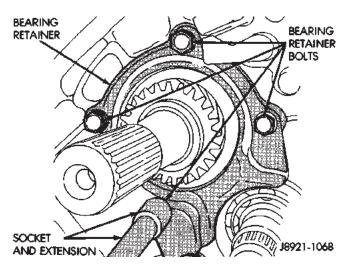
Fig. 61 Remove Output Shaft Rear Bearing Retainer
