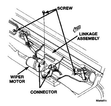
Fig. 11 Wiper Linkage Assembly Remove/Install
