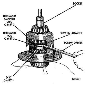
Fig. 58 Threaded Adapter Installation—Shown With 6963-A Holder
