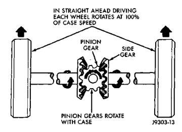
Fig. 1 Differential Operation—Straight Ahead Driving
