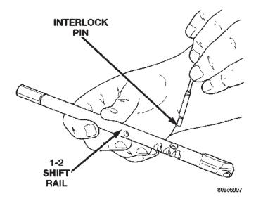
Fig. 73 Remove 1-2 Shift Rail Interlock Pin
