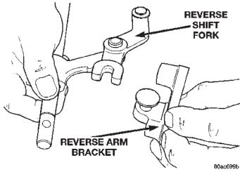
Fig. 80 Install Reverse Arm Bracket to Fork
