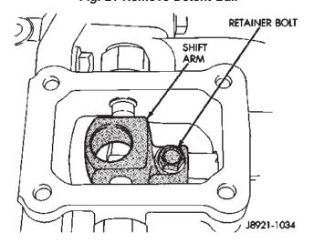
Fig. 22 Shift Arm Retainer Bolt Removal
