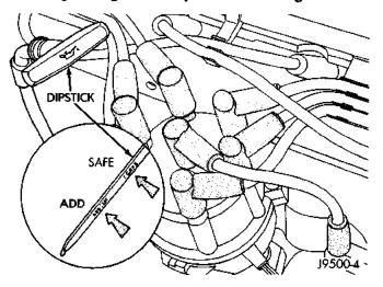
Fig. 8 Engine Oil Dipstick-4.0L Engine
