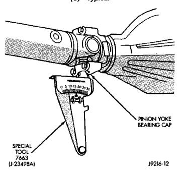
Fig. 11 Rear (input) Angle Measurement (B)—Typical
