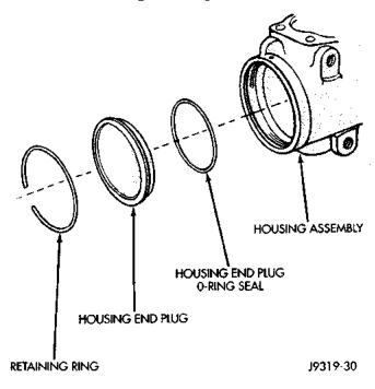
Fig. 6 End Plug Components
