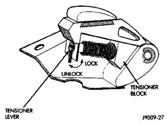
Fig. 41 Loading Timing Chain Tensioner
