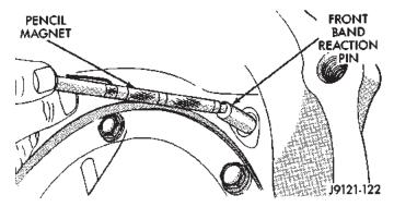
Fig. 88 Front Band Reaction Pin
