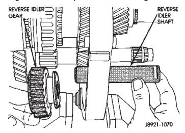
Fig. 63 Remove Reverse Idler Shaft And Gear
