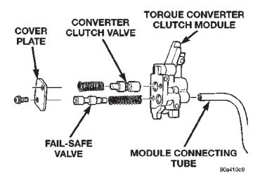
Fig. 47 Converter Clutch and Fail Safe Valves
