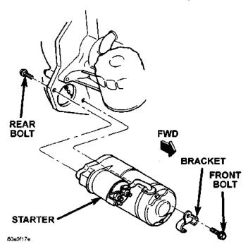
Fig. 12 Starter Remove/Install - 4.0L Engine
