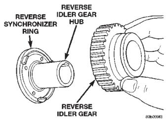
Fig. 117 Remove Reverse Idler Gear
