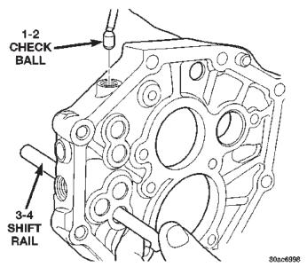
Fig. 74 Remove 1-2 Check Ball
