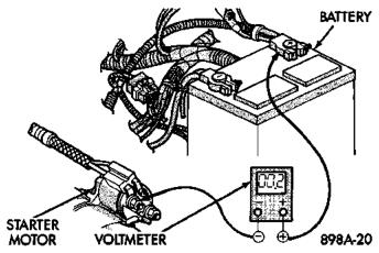
Fig. 4 Test Battery Positive Cable Resistance -Typical
