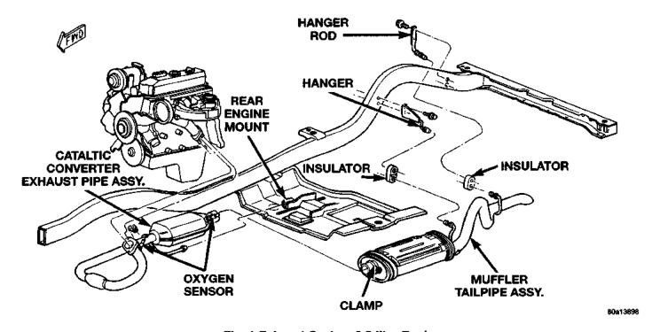
Fig. 1 Exhaust System 2.5 liter Engine
