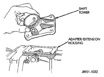
Fig. 47 Install Shift Tower
