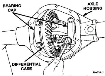
Fig. 54 Tighten Bolts Holding Bearing Caps
