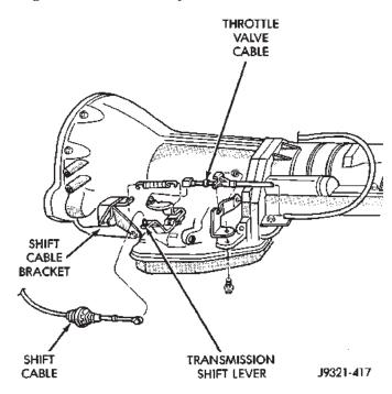
Fig. 175 Shift Cable Attachment At Transmission-Typical
