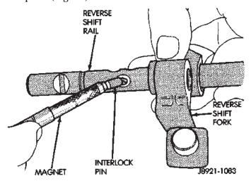
Fig. 82 Install Reverse Shift Rail Interlock Pin
