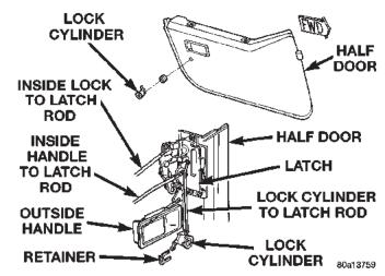
Fig. 37 Half Door Latch Rods
