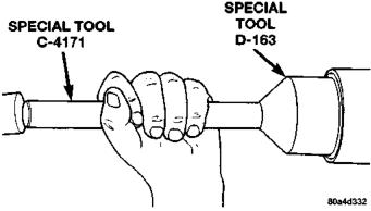
Fig. 10 Pinion Seal Installation
