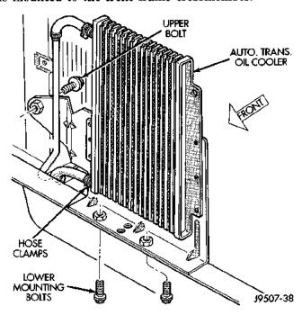
Fig. 3 Auxiliary Air-To-Oil Cooler
