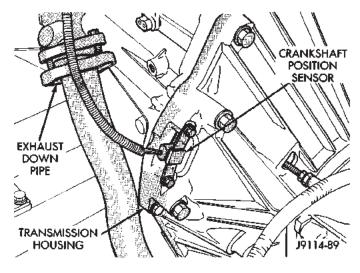
Fig. 16 Crankshaft Position Sensor—2.5L Engine
