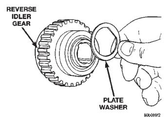
Fig. 116 Remove Reverse Idler Gear Plate Washer
