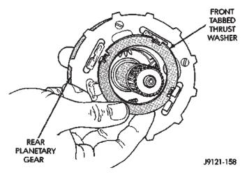
Fig. 151 Installing Rear Planetary Front Thrust Washer
