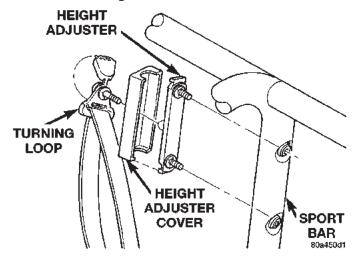
Fig. 53 Front Turning Loop
