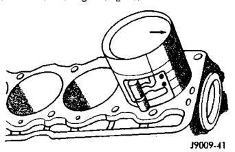
Fig. 49 Rod and Piston Assembly Installation
