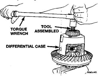
Fig. 59 Tighten Belleville Spring Compressor Tool—Shown With 696\$-A Holder
