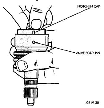
Fig. 18 Stub Shaft Installation
