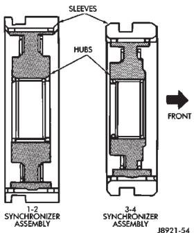
Fig. 108 Synchronizer Identification
