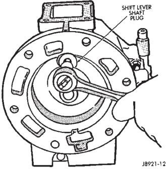
Fig. 24 Removing Shift Lever Shaft Plug
