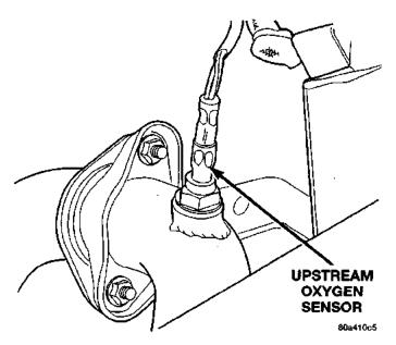
Fig. 28 Upstream Oxygen Sensor Location
