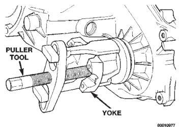
Fig. 16 Yoke Removal
