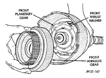
Fig. 159 Installing Front Planetary And Annulus Gears
