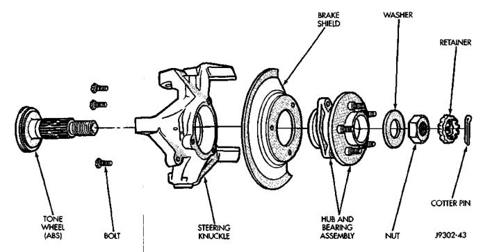
Fig. 8 Hub Bearing & Knuckle
