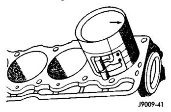
Fig. 14 Rod and Piston Assembly Installation
