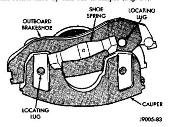
Fig. 27 Outboard Brake Shoe Removal
