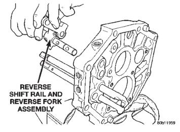
Fig. 81 Install Reverse Shift Rail
