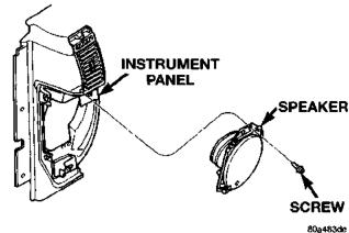
Fig. 6 Instrument Panel Speaker Remove/Install
