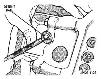
Fig. 22 Remove Detent Ball
