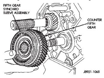
Fig. 54 Remove Fifth Gear and Synchro Assembly
