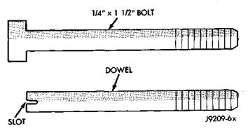
Fig. 50 Fabrication of Alignment Dowels
