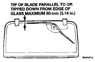
Fig. 9 Rear Wiper Arm Installation
