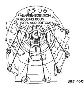
Fig. 27 Adapter/Extension Housing Bolts
