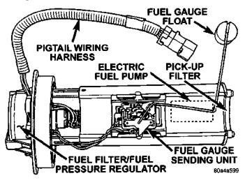
Fig. 2 Fuel Pump Module Components
