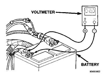
Fig. 2 Test Battery Negative Connection Resistance
