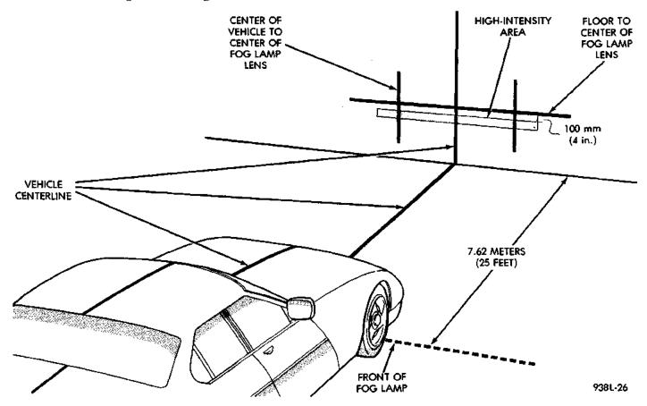
Fig. 3 Fog Lamp Alignment —Typical
