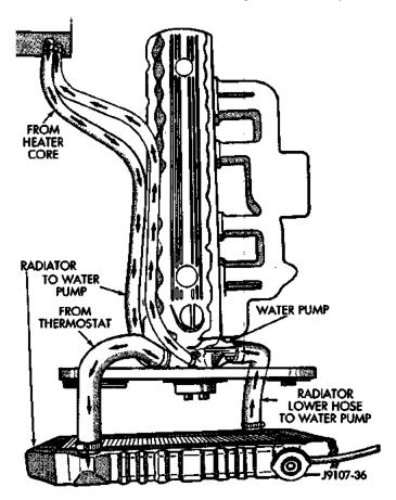
Fig. 2 Coolant Flow-4.0L Engine
