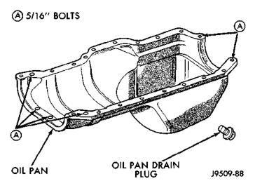
Fig. 52 Position of 5/16 inch Oil Pan Bolts
