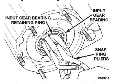
Fig. 33 Removing Input Gear Retaining Ring
