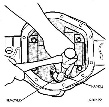
Fig. 29 Front Bearing Cup Removal
