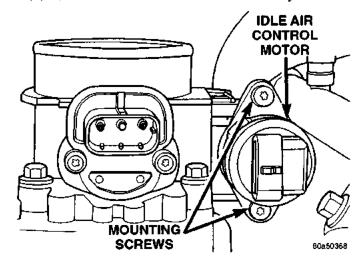
Fig. 37 Mounting Bolts (Screws)—IAC Motor
