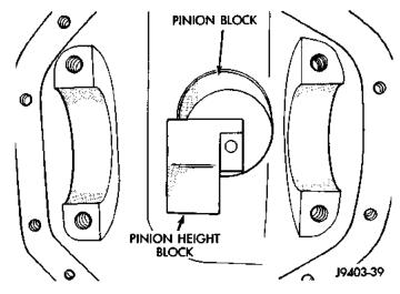
Fig. 50 Pinion Height Block—Typical
