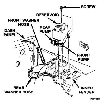
Fig. 18 Washer Reservoir & Pumps Remove/Install
