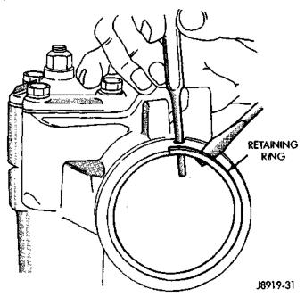
Fig. 5 End Plug Retaining Ring
