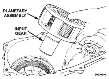
Fig. 34 Input Gear And Planetary Carrier Removal
