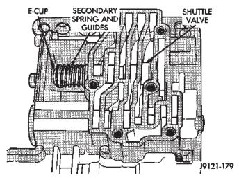
Fig. 54 Shuttle Valve E-Clip And Secondary Spring
