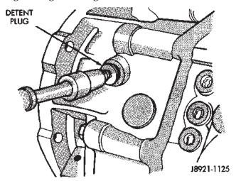
Fig. 20 Remove Detent Ball Plug
