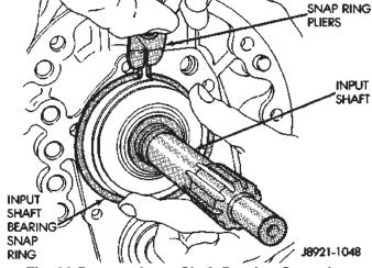
Fig. 30 Remove Input Shaft Bearing Snap-ring
