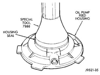
Fig. 54 Oil Pump Seal Installation
