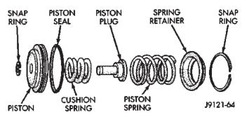
Fig. 172 Rear Servo Components
