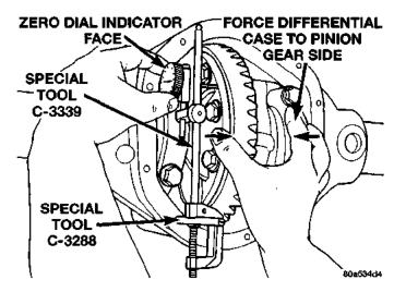
Fig. 79 Hold Differential Case and Zero Dial Indicator
