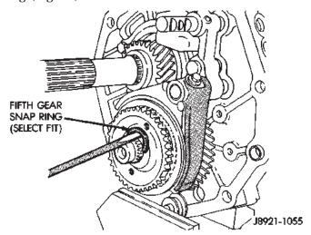
Fig. 50 Remove Fifth Gear Snap-ring
