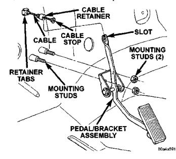
Fig. 26 Accelerator Pedal Mounting
