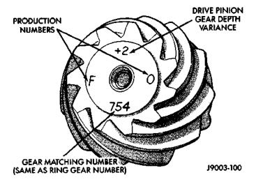
Fig. 67 Pinion Gear ID Numbers
