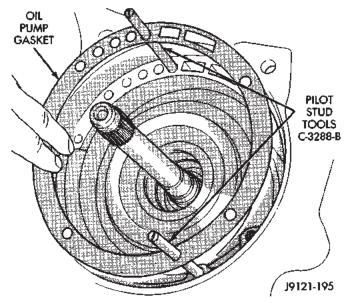
Fig. 108 Installing Pilot Studs And Oil Pump Gasket
