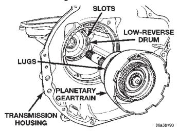
Fig. 79 Planetary Geartrain
