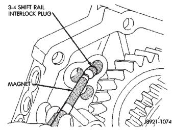
Fig. 88 Install 3-4 Shift Rail Interlock Plug
