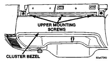
Fig. 6 Cluster Bezel Upper Screws Remove/Install
