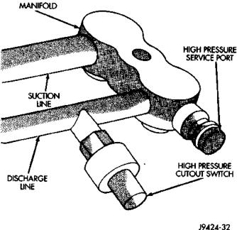
Fig. 23 High Pressure Cut-Off Switch - Typical
