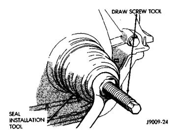
Fig. 52 Timing Case Cover Oil Seal Installation
