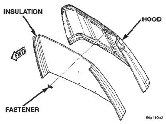
Fig. 3 Hood Insulation Panel
