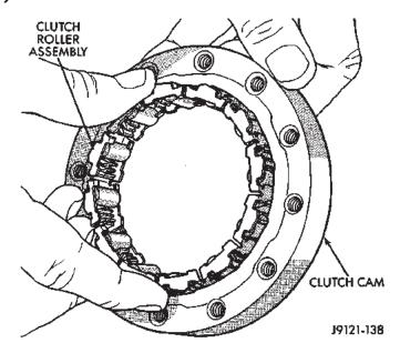
Fig. 113 Assembling Overrunning Clutch And Cam
