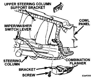
Fig. 3 Combination Flasher Remove/Install
