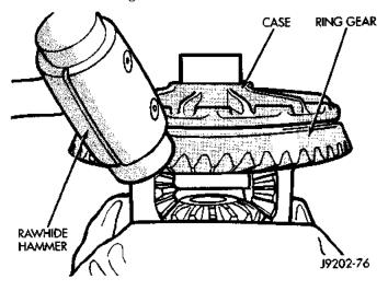
Fig. 28 Ring Gear Removal
