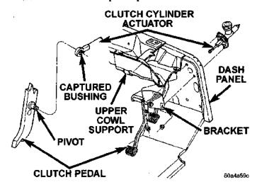
Fig. 12 Clutch Pedal Mounting—Right Hand Drive
