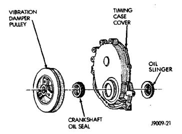
Fig. 30 Timing Case Cover Components
