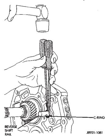
Fig. 77 Remove Reverse Shift Rail C-ring
