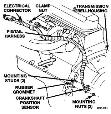
Fig. 39 Crankshaft Position Sensor—2.5L 4-Cyl. Engine—Auto. Trans.
