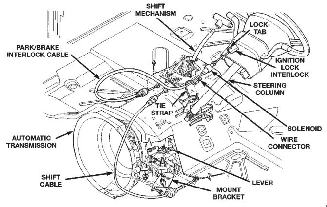
Fig. 26 Cable and Shifter
