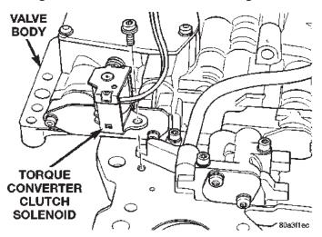
Fig. 62 Converter Clutch Solenoid
