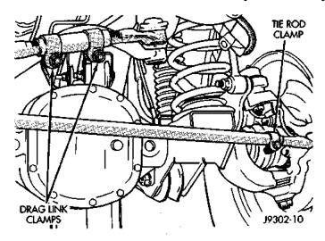
Fig. 3 Tie Rod/Drag Link Clamp Bolt
