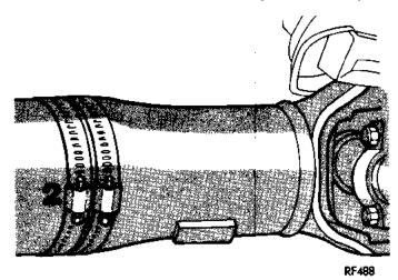
Fig. 6 Two Clamp Screws At The Same Position
