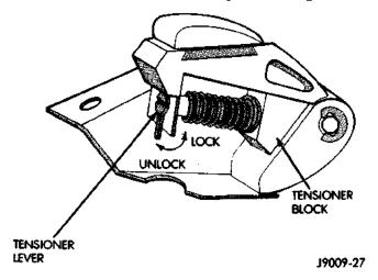
Fig. 39 Loading Timing Chain Tensioner
