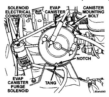
Fig. 7 EVAP Canister and Purge Solenoid Location
