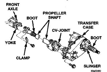
Fig. 13 Front Propeller Shaft
