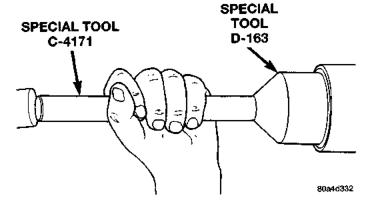
Fig. 41 Pinion Seal Installation
