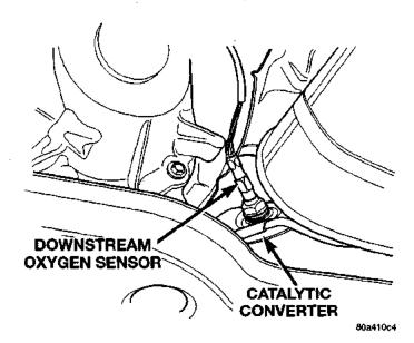
Fig. 6 Downstream Oxygen Sensor
