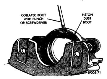
Fig. 47 Caliper Piston Dust Boot Removal
