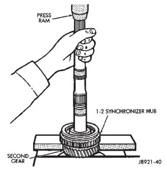
Fig. 115 Remove Second Gear And 1–2 Synchronizer/Reverse Gear
