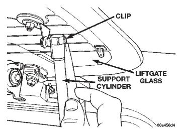
Fig. 74 Support Rod Cylinder
