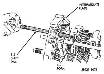
Fig. 87 Install 1-2 Shift Rail
