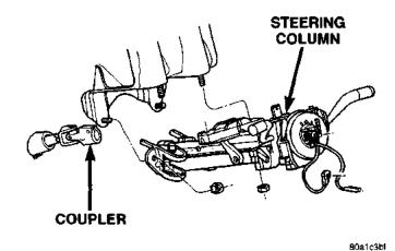
Fig. 19 Steering Column Mounting
