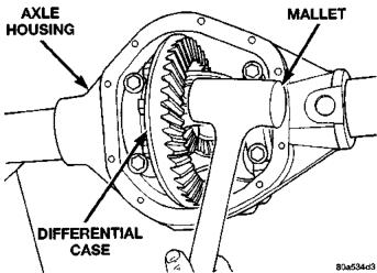
Fig. 56 Seat Ring Gear Side Differential Dummy Side Bearing
