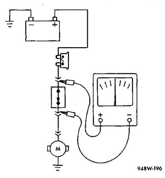
Fig. 10 Testing for Voltage Drop
