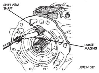
Fig. 26 Remove Shifter Shaft
