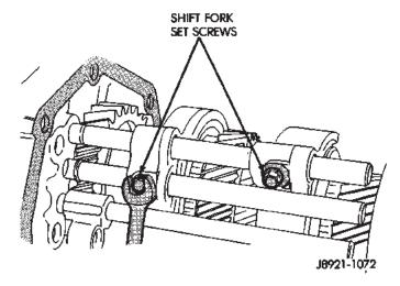
Fig. 90 Install Shift Fork To Shift Rail Bolts
