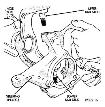
Fig. 5 Steering Knuckle Removal/Installation
