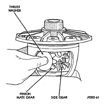
Fig. 52 Pinion Mate Gear Removal
