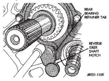
Fig. 93 Install Output Shaft Rear Bearing Retainer
