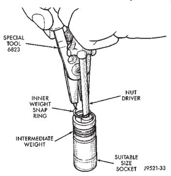
Fig. 37 Inner Weight Snap Ring
