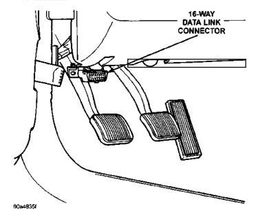
Fig. 10 Data Link Connector Location
