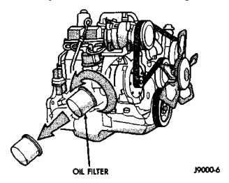
Fig. 9 Oil Filter-2.5L Engine
