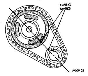
Fig. 37 Crankshaft—Camshaft Alignment
