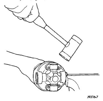
Fig. 25 Remove Bearing From Yoke
