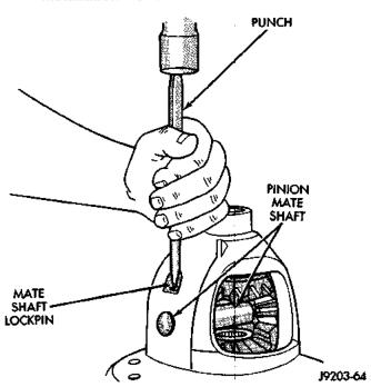
Fig. 66 Mate Shaft Roll Pin Installation
