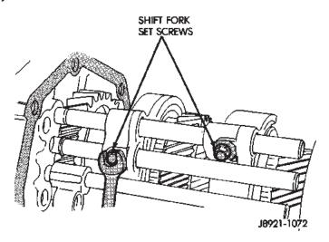
Fig. 70 Remove Shift Fork To Shift Rail Bolts
