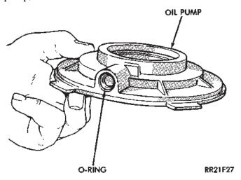
Fig. 14 Pick-up Tube O-ring Location
