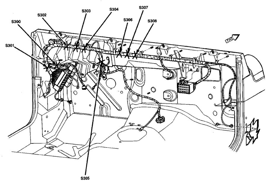
Fig. 5 Cowl Panel Wiring Splices
