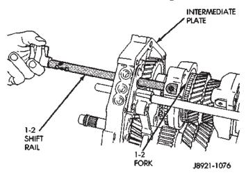
Fig. 74 Remove 1-2 Shift Rail
