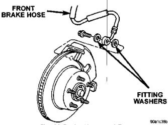
Fig. 23 Brake Hose And Bolt
