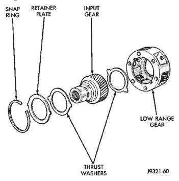
Fig. 56 Input/Low Range Gear Components
