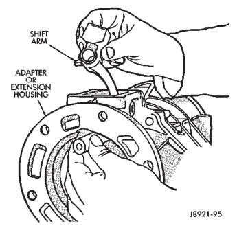
Fig. 43 Install Shifter Arm Shaft
