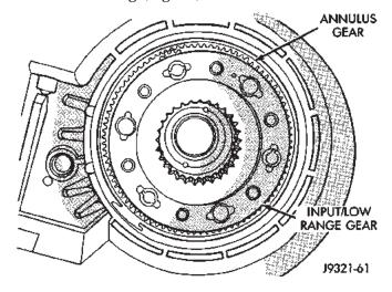
Fig. 57 Input/Low Range Gear Installation
