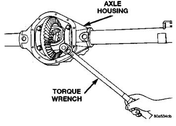
Fig. 22 Tighten Differential Bearing Cap Bolts
