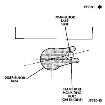
Fig. 50 Distributor Engaged Position—4.0L 6-Cylinder Engine
