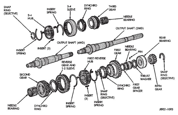
Fig. 110 Output Shaft And Gears
