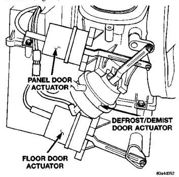
Fig. 34 Defrost/Demist, Floor, and Panel Door Vacuum Actuators
