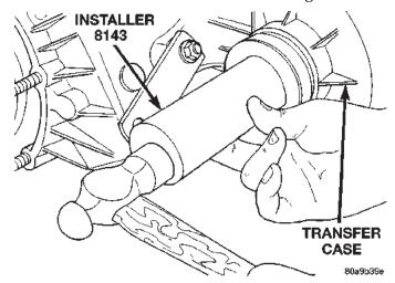
Fig. 7 Front Output Seal Installation
