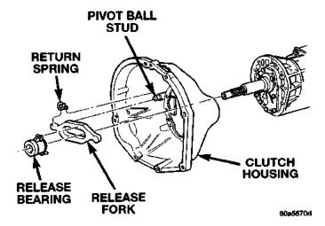
Fig. 6 Release Bearing Attachment
