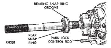
Fig. 30 Output Shaft Rear Bearing—Typical
