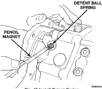
Fig. 45 Install Detent Spring
