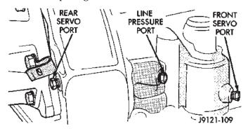
Fig. 6 Pressure Test Ports At Side Of Case
