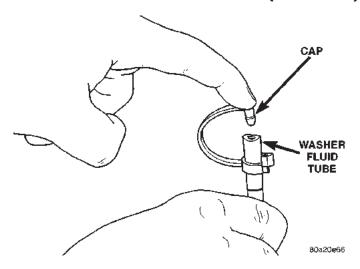
Fig. 46 Rear Washer Fluid Tube
