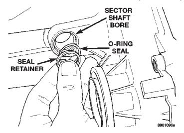
Fig. 27 Sector Bushing And O-Ring Removal
