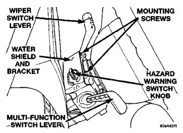
Fig. 14 Water Shield Upper Screws Remove/Install water shield and bracket to the steering column (Fig. 15).
