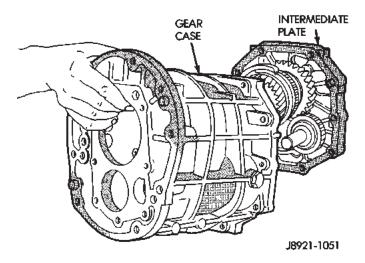
Fig. 35 Remove Intermediate Plate from Transmission Case
