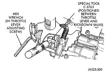
Fig. 183 Throttle Pressure Adjustment
