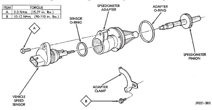
Fig. 4 Speedometer Components
