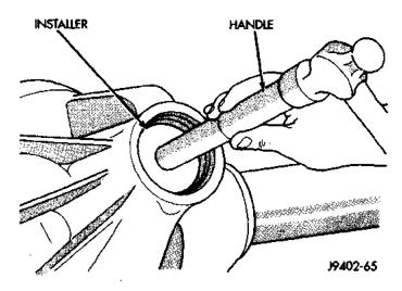
Fig. 34 Pinion Outer Bearing Cup Installation
