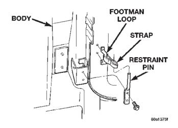
Fig. 19 Restraint Strap
