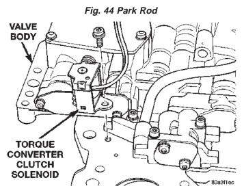
Fig. 45 Converter Clutch Solenoid
