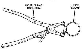
Fig. 25 Hose Clamp Tool-Typical
