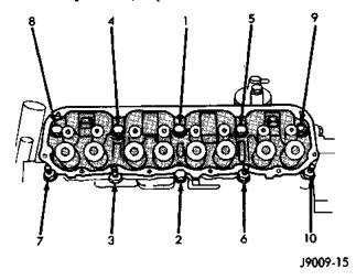
Fig. 31 Engine cylinder head Bolt Tightening Sequence
