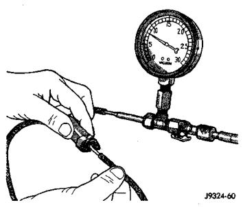
Fig. 7 Vacuum Circuit Test
