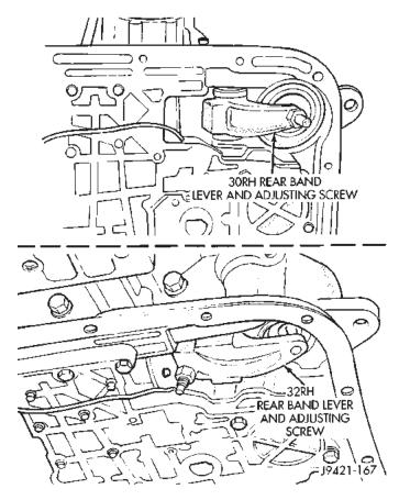
Fig. 181 Rear Band Adjustment Screw Location
