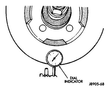
Fig. 10 Checking Rotor Runout And Thickness
