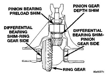
Fig. 73 Axle Adjustment Shim Locations
