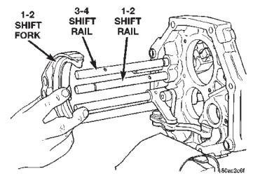
Fig. 65 Remove 1-2 Shift Fork
