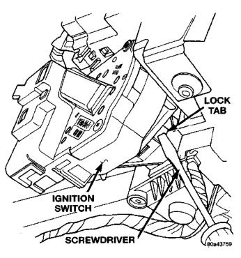
Fig. 54 Ignition Switch Lock Tab
