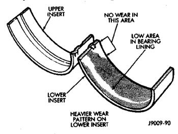
Fig. 16 Main Bearing Wear Patterns
