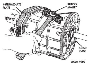
Fig. 31 Separate Intermediate Plate and Transmission Case
