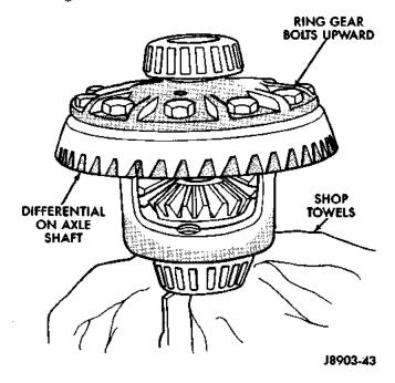
Fig. 49 Differential Case Holding Tool
