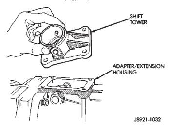
Fig. 17 Remove Shift Tower
