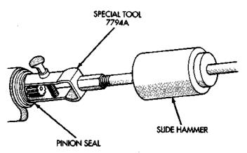
Fig. 9 Seal Removal
