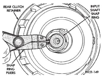
Fig. 138 Removing/Installing Input Shaft Snap-Ring ASSEMBLY
