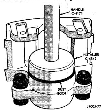
Fig. 54 Piston Dust Boot Installation
