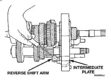
Fig. 88 Reverse Shift Arm Position
