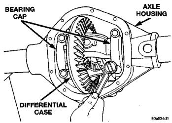
Fig. 75 Tighten Boits Holding Bearing Caps
