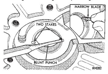
Fig. 124 Staking Oil Pump Bushing
