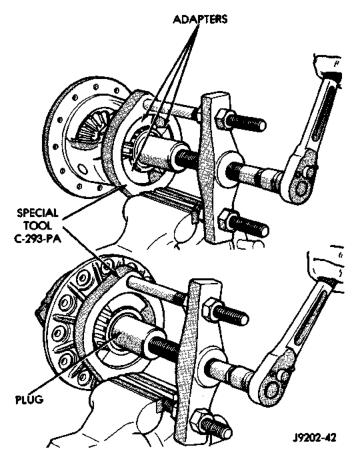
Fig. 23 Differential Bearing Removal
