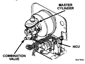
Fig. 12 Combination Valve Brake Lines
