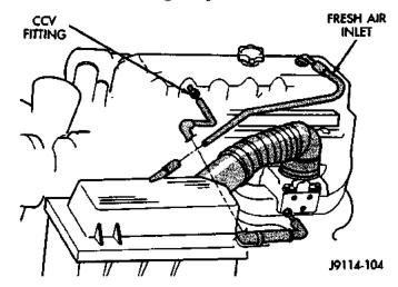
Fig. 24 Engine Cylinder Head Cover
