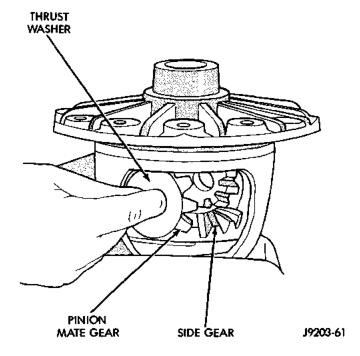
Fig. 48 Pinion Mate Gear Removal
