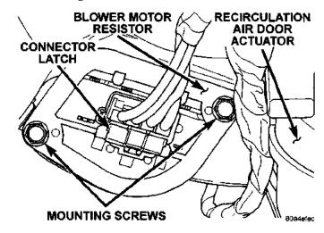
Fig. 33 Blower Motor Resistor Remove/Install
