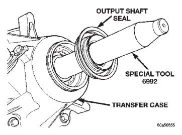
Fig. 77 Output Shaft Seal and Protector
