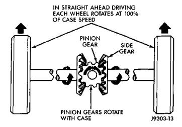
Fig. 2 Differential Operation—Straight Ahead Driving
