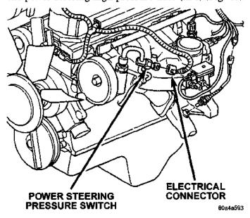
Fig. 40 Power Steering Pressure Switch
