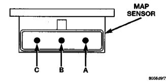
Fig. 27 MAP Sensor Connector Terminals—Typical
