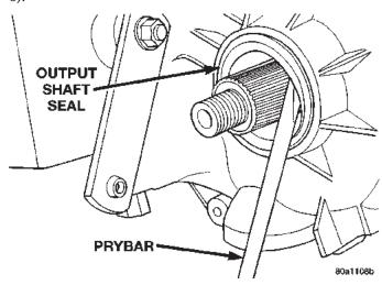
Fig. 6 Remove Front Output Shaft Seal
