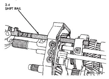
Fig. 71 Remove 3-4 Shift Rail
