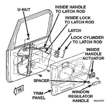
Fig. 24 Latch Rods
