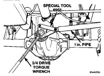
Fig. 14 Tightening Pinion Shaft Nut
