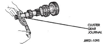
Fig. 125 Check Output Shaft Tolerances
