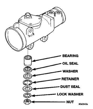
Fig. 2 Pitman Shaft Seal
