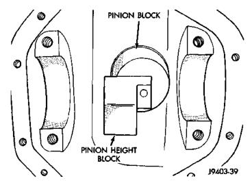
Fig. 70 Pinion Height Block—Typical
