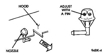
Fig. 2 Windshield Washer Nozzles
