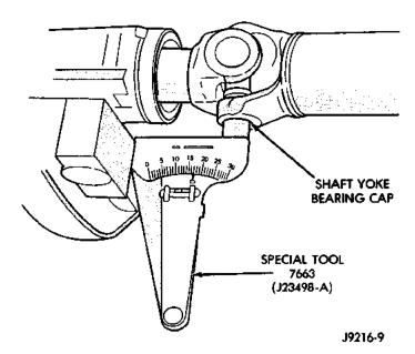
Fig. 10 Propeller Shaft Angle Measurement (C)—Typical
