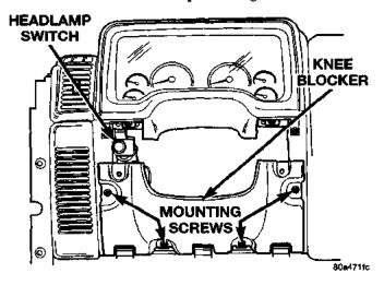
Fig. 3 Knee Blocker Remove/Install
