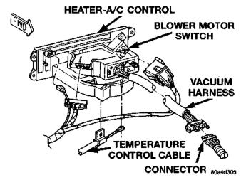
Fig. 29 Heater-A/C Control Connectors
