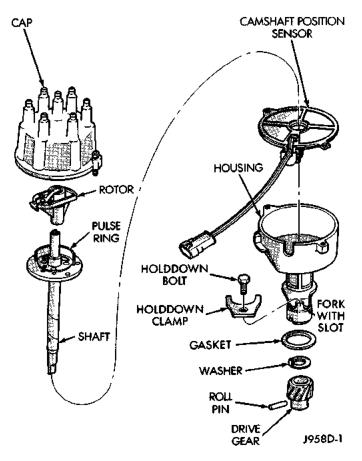
Fig. 43 Distributor—2.5L Or 4.0L Engines—Typical
