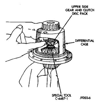
Fig. 60 Upper Side Gear & Clutch Disc Pack Installation
