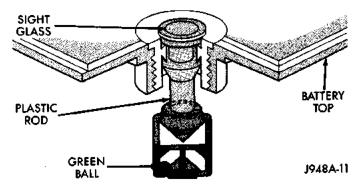
Fig. 2 Built-In Test Indicator
