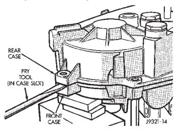
Fig. 19 Loosening Rear Case
