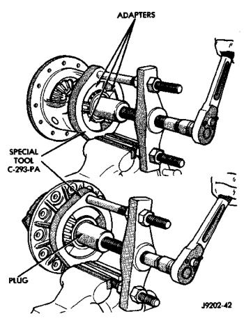
Fig. 26 Differential Bearing Removal
