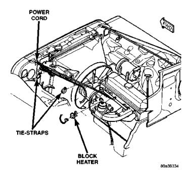
Fig. 31 Block Heater and Cord—2.5L Engine FAN
