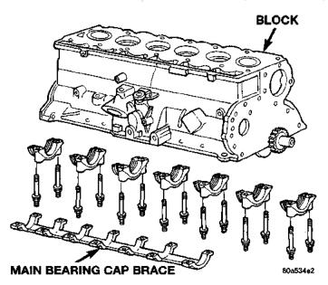
Fig. 46 Main Bearing Caps and Brace.
