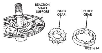
Fig. 121 Pump Gear Removal
