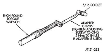
Fig. 180 Band Adjustment Adapter Tool
