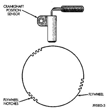
Fig. 8 Sensor Operation—4.0L 6-Cyl. Engine— Automatic Transmission
