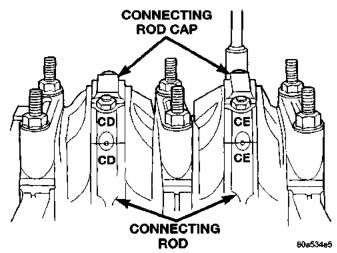
Fig. 47 Stamped Connecting Rods and Caps
