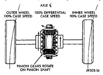
Fig. 2 Differential Operation-On Turns
