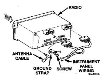
Fig. 4 Radio Connections - Typical
