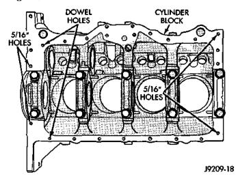
Fig. 51 Position of Dowels in Cylinder Block
