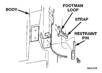
Fig. 35 Restraint Strap
