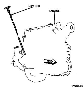
Fig. 6 Engine Oil Dipstick Location—Typical
