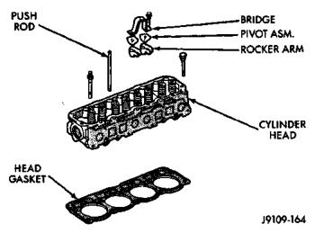
Fig. 28 Engine Cylinder Head Assembly INSTALLATION
