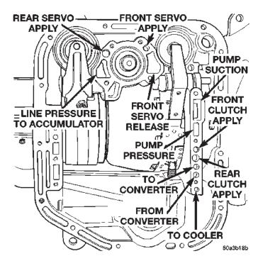
Fig. 10 Air Pressure Test Passages
