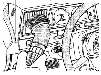
Fig. 3 Vacuum Heater and A/C Outlets
