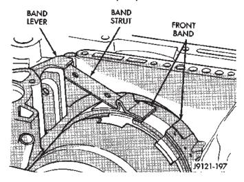
Fig. 105 Front Band Linkage Installation
