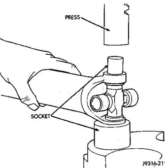
Fig. 19 Press Out Bearing
