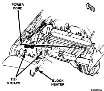
Fig. 32 Block Heater and Cord-4.0L Engine
