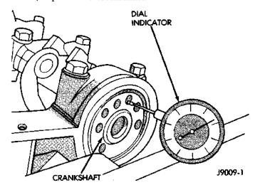
Fig. 49 Crankshaft End Play Measurement
