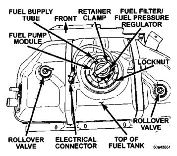
Fig. 1 Fuel Tank/Fuel Pump Module (Top View)
