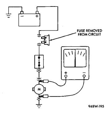
Fig. 9 Testing for Continuity
