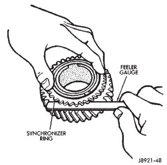
Fig. 123 Check Synchronizer Ring Wear
