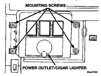
Fig. 10 Accessory Switch Bezel Remove/install
