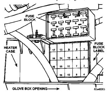
Fig. 15 Fuseblock Module Remove/Install
