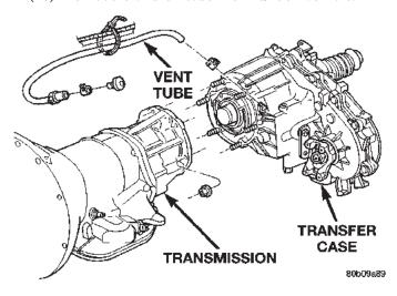
Fig. 2 Transfer Case Mounting
