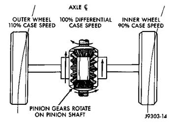
Fig. 3 Differential Operation—On Turns
