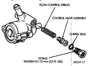
Fig. 8 Flow Control Valve
