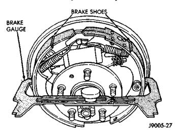
Fig. 60 Adjusting Gauge On Brake Shoes
