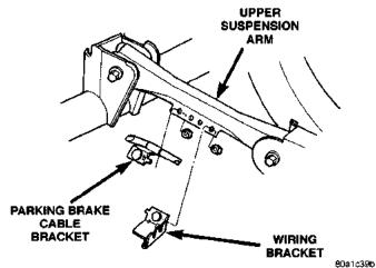
Fig. 38 Parking Brake Cable Bracket
