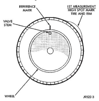
Fig. 8 First Measurement On Tire
