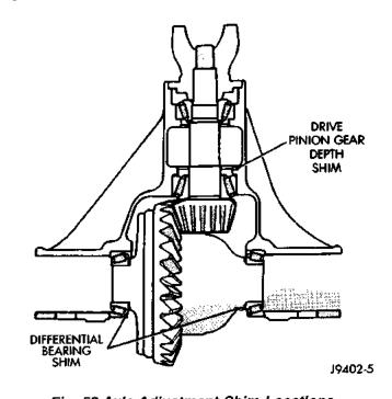
Fig. 53 Axle Adjustment Shim Locations
