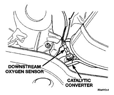
Fig. 29 Downstream Oxygen Sensor Location
