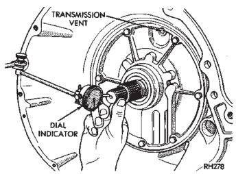
Fig. 110 Checking Input Shaft End Play
