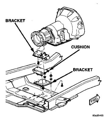
Fig. 22 Rear Mount (AutomaticTransmission)
