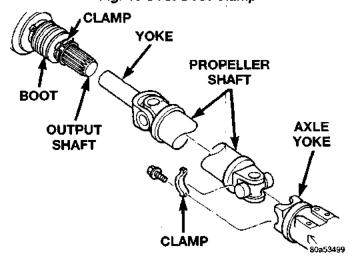
Fig. 16 Rear Propeller Shaft
