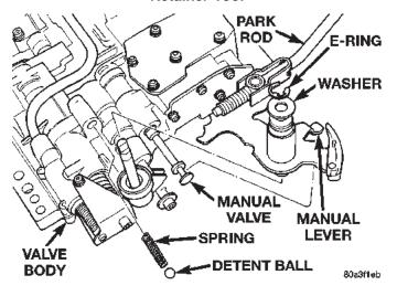
Fig. 42 Manual And Throttle Levers
