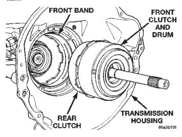
Fig. 75 Front/Rear Clutch Assemblies
