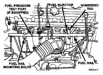
Fig. 11 Fuel Injectors—Typical 4.0L Shown
