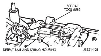
Fig. 64 Securing Detent Ball And Spring With Retainer Tool
