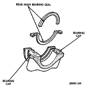
Fig. 50 Rear Main Bearing Oil Seal
