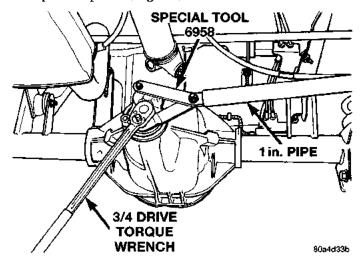
Fig. 45 Tightening Pinion Nut
