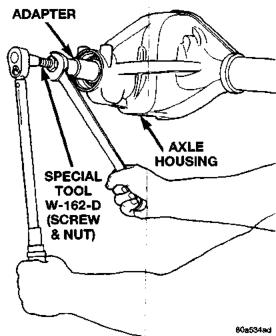
Fig. 44 Outer Pinion Bearing Install
