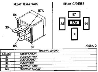
High Speed Blower Motor Relay
