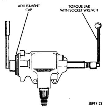
Fig. 16 Worm Bearing Preload
