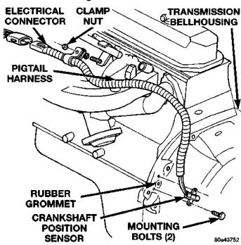
Fig. 40 Crankshaft Position Sensor—Manual Transmission (Typical)
