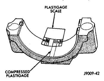
Fig. 18 Measuring Bearing Clearance with Plastigage
