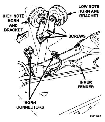
Fig. 2 Horn(s) Remove/Install - Typical
