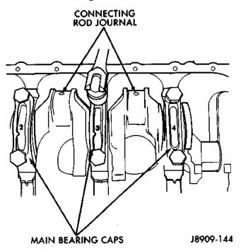
Fig. 46 Removing Main Bearing Caps and Lower Inserts
