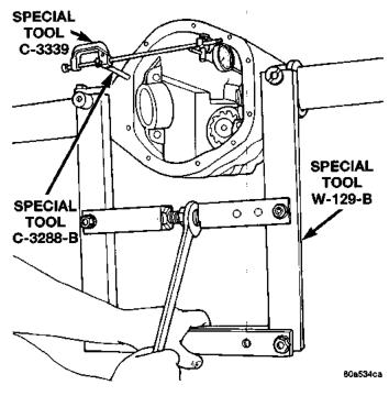
Fig. 23 Spread Axle Housing
