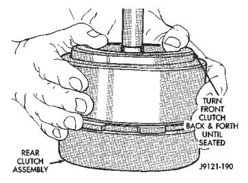
Fig. 100 Assembling Front And Rear Clutch Units
