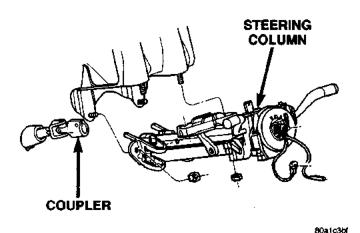
Fig. 5 Steering Column Mounting
