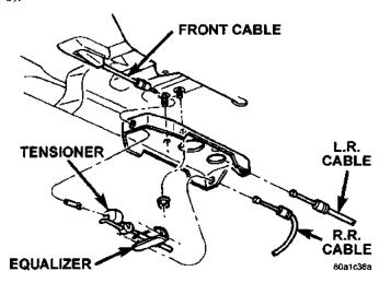
Fig. 6 Parking Brake Components
