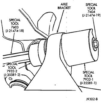
Fig. 5 Bushing Installation
