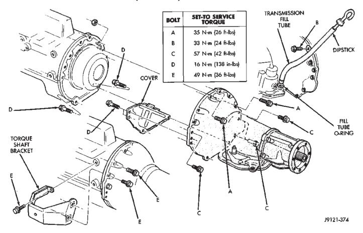
Fig. 19 Transmission Attachment
