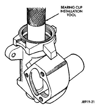
Fig. 13 Upper Bearing Cup Installation
