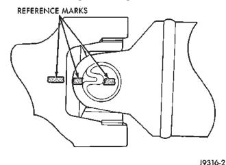
Fig. 6 Marking Propeller Shaft And Axle Yokes
