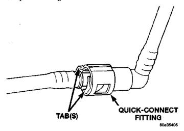
Flg. 8 Typical Two-Tab Type Quick-Connect Fitting
