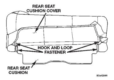
Fig. 9 Hook And Loop Fasteners
