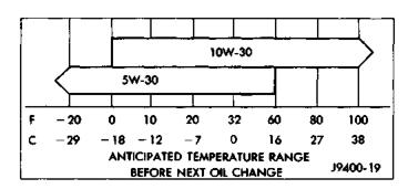
Fig. 4 Temperature/Engine Oil Viscosity
