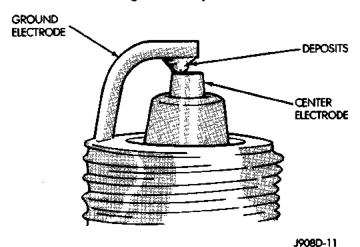
Fig. 26 Electrode Gap Bridging
