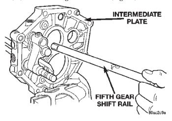
Fig. 84 Install Fifth Gear Shift Rail
