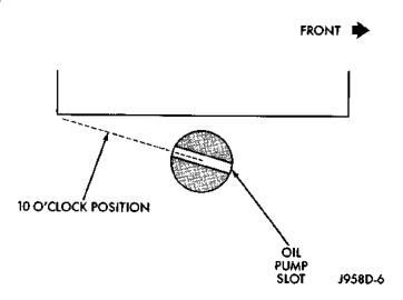
Fig. 45 Slot At 10 O'clock Position—2.5L Engine
