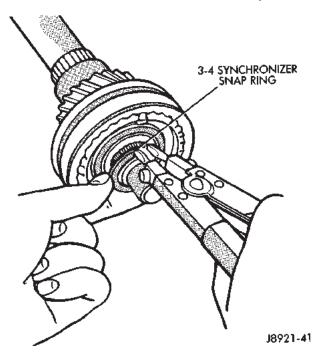
Fig. 116 Remove 3-4 Synchronizer Snap Ring
