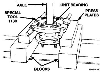
Fig. 17 Axle Bearing and Seal Remove
