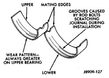
Fig. 11 Connecting Rod Bearing Inspection CONNECTING RODS
