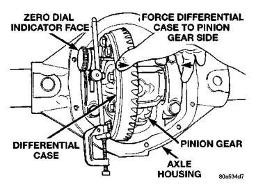
Fig. 60 Hold Differential Case and Zero Dial Indicator
