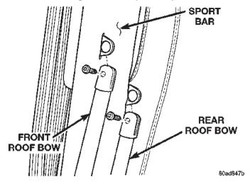
Fig. 48 Roof Bow Removal
