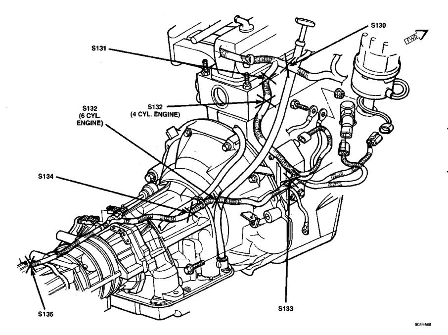
Fig. 4 Engine Wiring Splices
