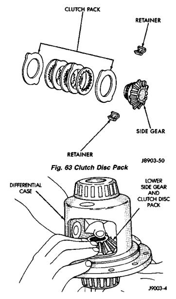
Fig. 64 Clutch Discs and Ring Gear Side Gear Installation
