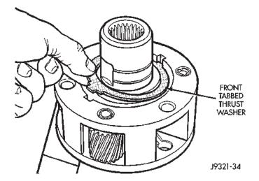
Fig. 37 Front Tabbed Thrust Washer Removal
