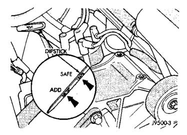
Fig. 7 Engine Oil Dipstick—2.5L Engine
