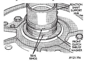
Fig. 106 Reaction Shaft Support Seal Rings
