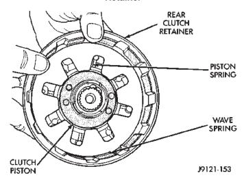
Fig. 142 Piston Spring/Wave Spring Position
