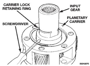
Fig. 35 Input Gear Snap-Ring Removal
