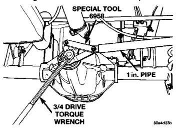
Fig. 13 Tightening Pinion Shaft Nut
