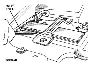
Fig. 13 Removing Cell Caps - Typical
