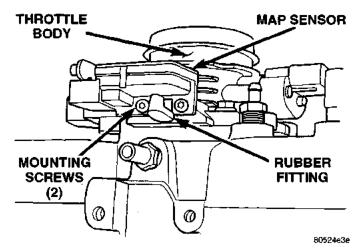
Fig. 19 Rubber L-Shaped Fitting—MAP Sensor-to-Throttle Body
