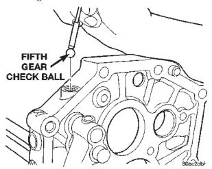
Fig. 83 Install Fifth Gear Check Ball
