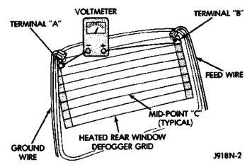
Fig. 1 Rear Glass Heating Grid Test
