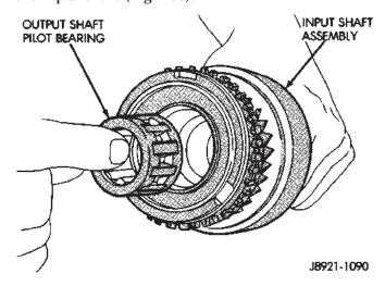
Fig. 107 Remove Output Shaft Pilot Bearing
