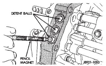
Fig. 66 Remove Lock Ball And Spring
