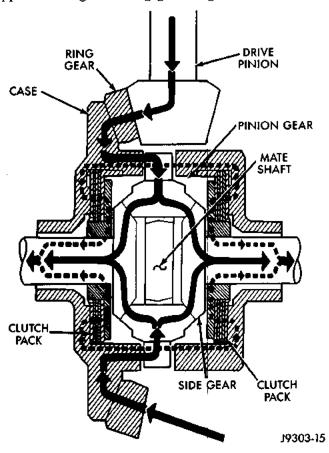
Fig. 4 Trac-lok Limited Slip Differential Operation
