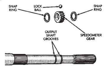
38921-1119 Fig. 28 Speedometer Drive Gear Assembly
