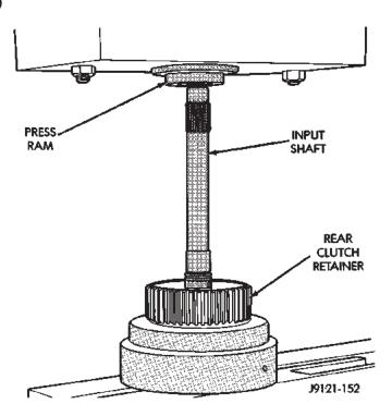
Fig. 141 Pressing Input Shaft Into Rear Clutch Retainer
