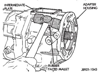
Fig. 26 Loosen Adapter/Extension Housing
