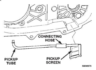
Fig. 20 Oil Pickup Tube Removal
