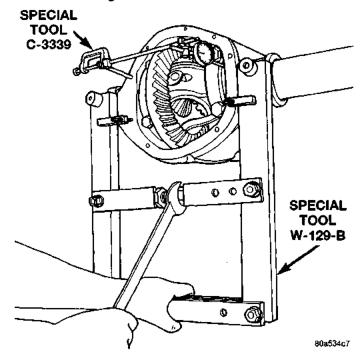
Fig. 18 Spread Axle Housing
