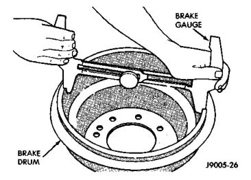
Fig. 59 Adjusting Gauge On Drum
