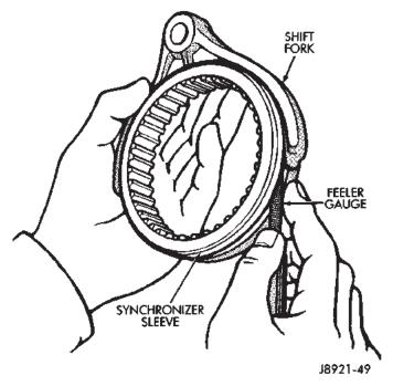
Fig. 124 Check Fork-To-Hub Clearance
