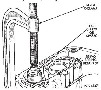
Fig. 92 Compressing Rear Servo Spring
