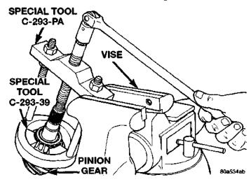
Fig. 39 Inner Bearing Cone Removal
