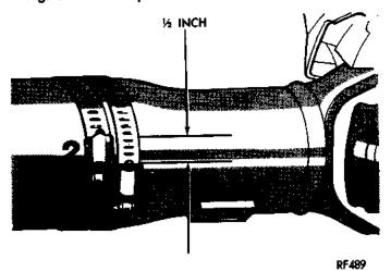
Fig. 7 Clamp Screws Separated RUNOUT SPECIFICATIONS
