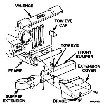
Fig. 2 Front Bumper Components
