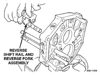
Fig. 70 Remove Reverse Shift Rail
