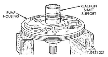
Fig. 129 Assembling Reaction Shaft Support And Pump Housing
