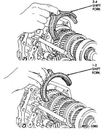
Fig. 84 Install Shift Forks
