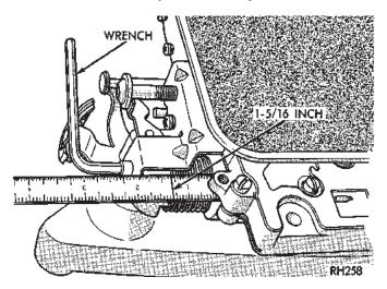
Fig. 182 Line Pressure Adjustment
