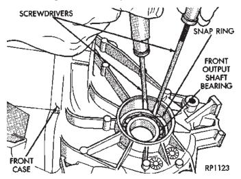
Fig. 41 Front Output Shaft Bearing Retaining Ring Removal
