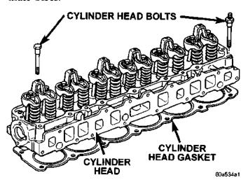
Fig. 26 Engine Cylinder Head Assembly
