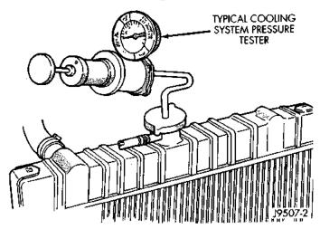
Fig. 16 Pressurizing System—Typical
