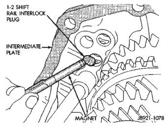
Fig. 76 Remove 1–2 Shift Rail Interlock Plug
