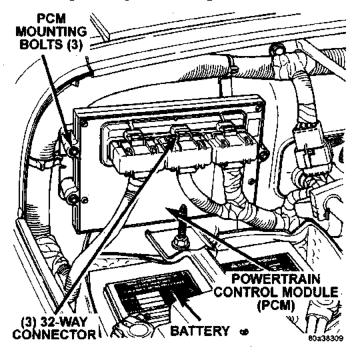
Fig. 1 Powertrain Control Module (PCM) Location The ignition system is controlled by the PCM.
