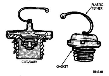
Fig. 9 Fuel Tank Filler Tube Cap—Typical removed prior to disconnecting any fuel system component or before draining the fuel tank.
