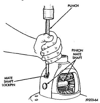
Fig. 53 Mate Shaft Roll Pin Installation
