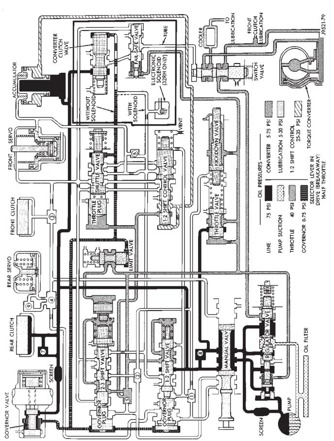
HYDRAULIC FLOW IN D-FIRST GEAR
