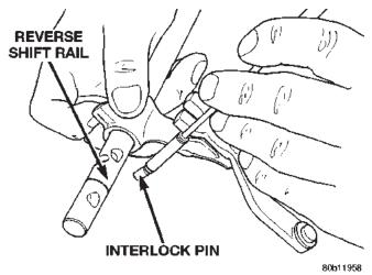
Fig. 79 Install Reverse Interlock Pin
