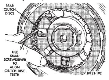
Fig. 102 Aligning Rear Clutch Disc Lugs
