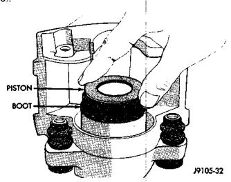
Fig. 53 Caliper Piston Installation
