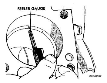
Fig. 8 Gap Measurement
