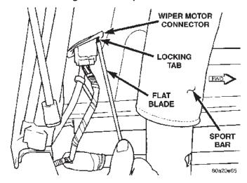
Fig. 45 Rear Wiper Wire Harness Connector
