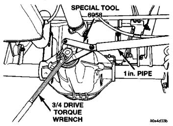
Fig. 48 Tightening Pinion Nut
