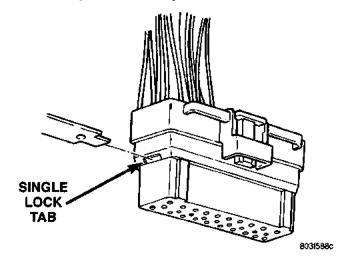
Fig. 16 Single Lock Tab
