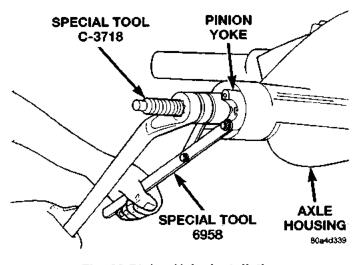
Fig. 38 Pinion Yoke Installation
