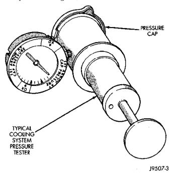
Fig. 18 Pressure Testing Radiator Pressure Cap—Typical
