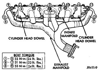
Fig. 9 Intake/Engine Exhaust Manifold Installation 4.0L Engine
