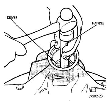
Fig. 30 Rear Bearing Cup Removal
