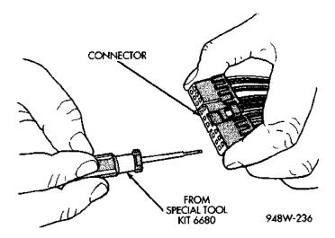
Fig. 22 Terminal Removal
