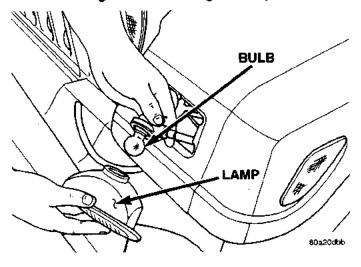
Fig. 5 Park/Turn Signal Lamp Bulb
