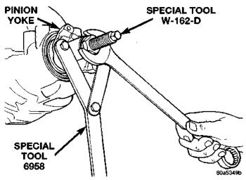
Fig. 11 Pinion Yoke, Install
