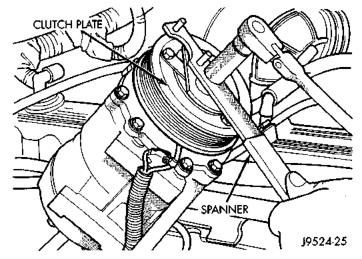
Fig. 12 Clutch Nut Remove
