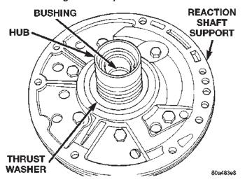
Fig. 122 Support Hub Thrust Washer
