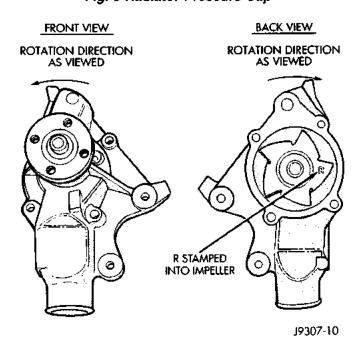
Fig. 6 Reverse Rotating Water Pump—Typical
