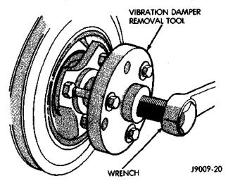
Fig. 33 Vibration Damper Removal Tool 7697
