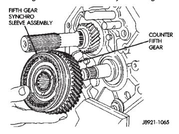
Fig. 58 Remove Fifth Gear And Synchro Assembly
