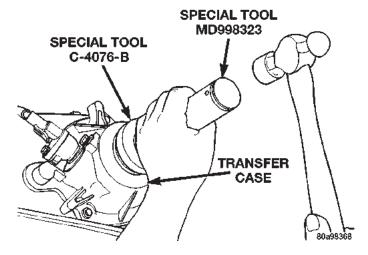
Fig. 78 Rear Seal Installation
