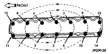
Fig. 27 Engine Cylinder Head Bolt Tightening Sequence
