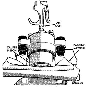
Fig. 46 Caliper Piston Removal
