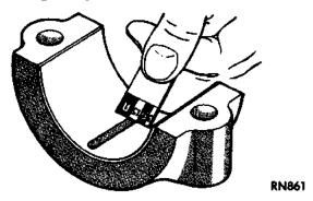
Fig. 3 Clearance Measurement
