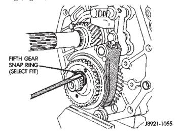
Fig. 52 Remove Fifth Gear Snap-ring
