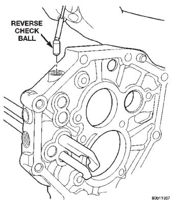
Fig. 72 Remove Reverse Check Ball
