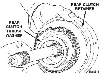
Fig. 144 Installing Rear Clutch Thrust Washer
