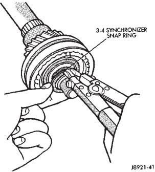
Fig. 106 Remove 3-4 Synchronizer Snap Ring
