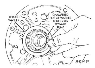
Fig. 107 Front Clutch Thrust Washer Installation
