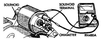
Fig. 8 Continuity Test Between Solenoid Terminal and Solenoid Case
