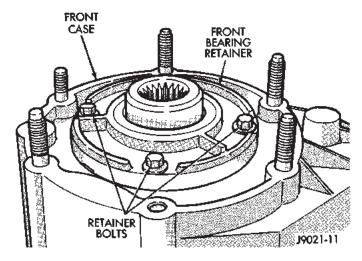
Fig. 31 Front Bearing Retainer Bolts
