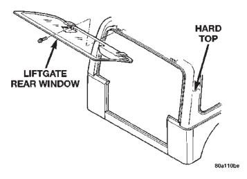
Fig. 77 Liftgate Glass
