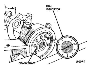
Fig. 45 Crankshaft End Play Measurement
