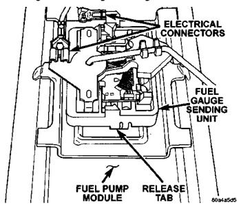
Fig. 18 Fuel Gauge Sending Unit Release Tab
