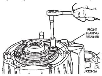
Fig. 59 Install Front Bearing Retainer
