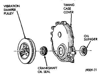
Fig. 35 Timing Case Cover Components
