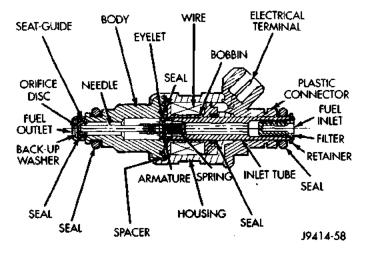
Fig. 7 Fuel Injector Internal Components—Typical
