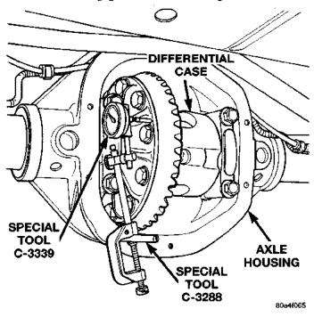
Fig. 72 Differential Side play Measurement
