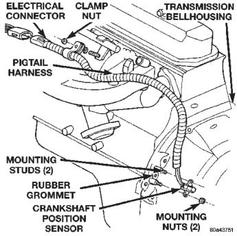
Fig. 6 Crankshaft Position Sensor—2.5L Engine
