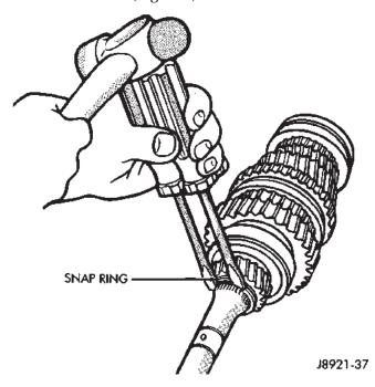
Fig. 113 Remove Fifth Gear Snap-ring
