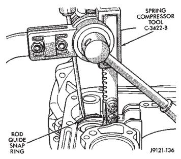
Fig. 91 Compressing Front Servo
