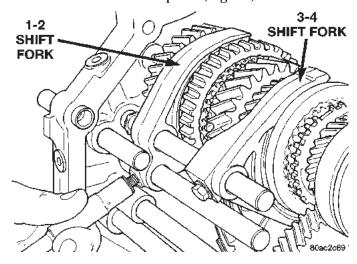
Fig. 59 Remove Shift Fork To Shift Rail Bolts
