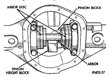
Fig. 66 Gauge Tools in Housing—Typical
