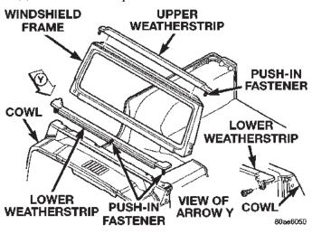
Fig. 9 Windshield Frame Weatherstrip
