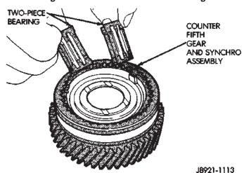
Fig. 97 Install Countershaft Fifth Gear Bearings
