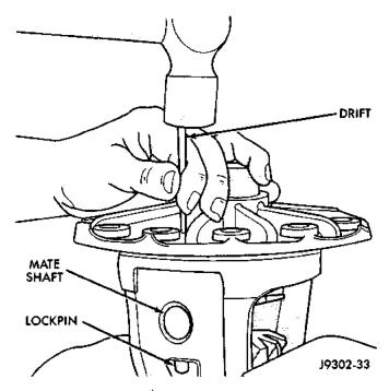
Fig. 44 Mate Shaft Roll Pin Removal
