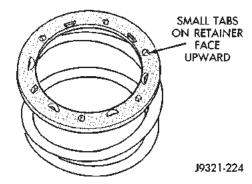
Fig. 135 Correct Spring Retainer Installed Position
