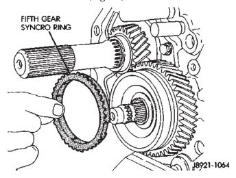
Fig. 53 Remove Fifth Gear Synchro Ring
