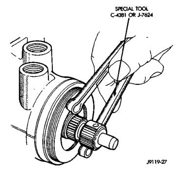
Fig. 8 Adjustment Plug
