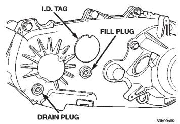
Fig. 1 Fill/Drain Plug And I.D. Tag Locations
