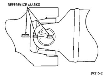
Fig. 11 Align Propeller Shaft And Rear Axle Yokes
