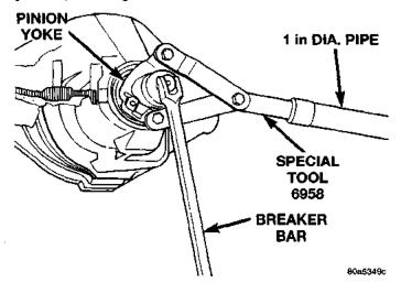
Fig. 7 Pinion Nut
