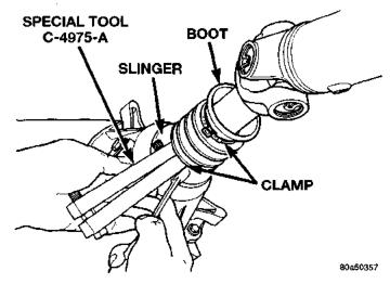
Fig. 17 Crimping Dust Boot Clamp—Typical
