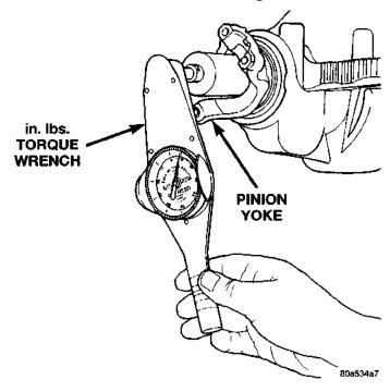
Fig. 12 Check Pinion Rotation Torque
