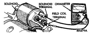
Fig. 7 Continuity Test Between Solenoid Terminal and Field Coll Terminal
