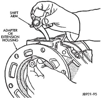
Fig. 40 Install Shifter Arm Shaft
