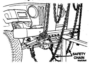
Fig. 4 Safety Chain Attachment
