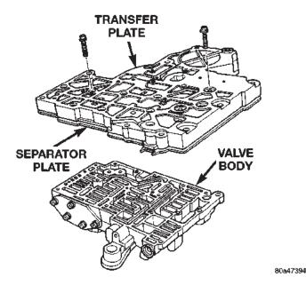
Fig. 48 Valve Body Transfer Plate Screws
