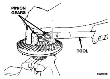
Fig. 56 Pinion Gear Removal
