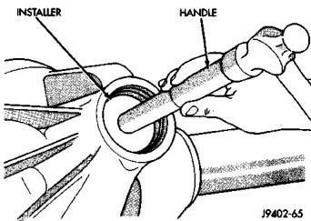
Fig. 42 Pinion Front Bearing Cup Install
