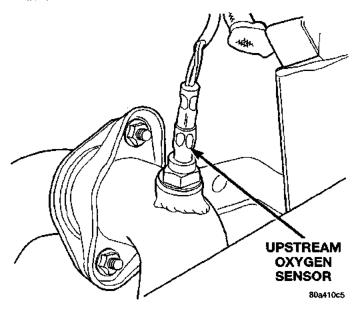
Fig. 5 Upstream Oxygen Sensor
