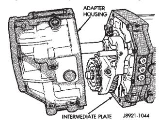
Fig. 29 Remove Adapter/Extension Housing
