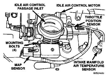
Fig. 7 Intake Air Temp. Sensor Location—Typical
