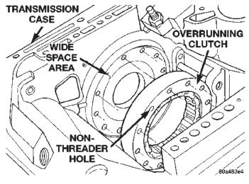
Fig. 93 Clutch Cam Alignment
