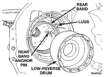
Fig. 84 Low- Reverse Band and Drum—32RH
