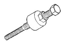
Installer, Power Steering Pulley C-4063-B
