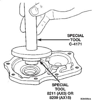
Fig. 12 Install Front Bearing Retainer Seal
