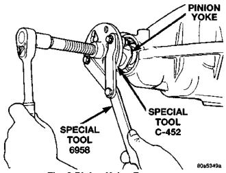
Fig. 8 Pinion Yoke, Remove
