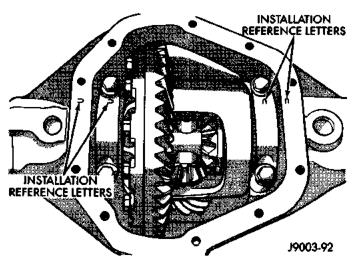
Fig. 15 Bearing Cap Identification
