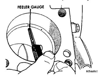
Fig. 8 Gap Measurement
