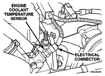
Fig. 4 Engine Coolant Temperature Sensor—Typical
