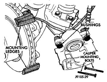
Fig. 29 Caliper Lubrication Points
