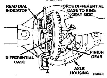
Fig. 82 Hold Differential Case and Read Dial Indicator
