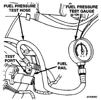
Fig. 6 Fuel Pressure Gauge Installation—Typical Test Port Shown
