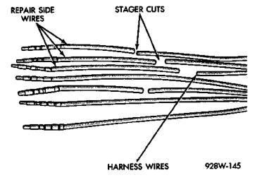
Fig. 20 Stagger Cutting Wires
