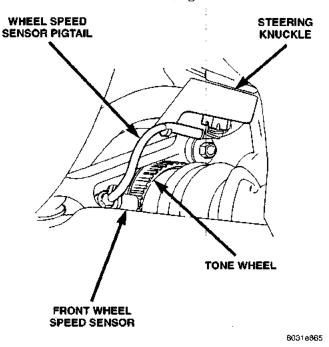
Fig. 9 Front Wheel Speed Sensor
