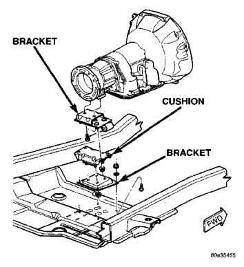
Fig. 22 Rear Mount (AutomaticTransmission)
