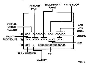
Fig. 3 Body Code Plate Decoding
