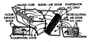
Fig. 1 Common Blend-Air Heater-Air Conditioner System - Typical
