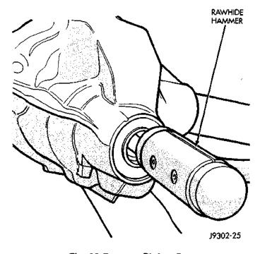
Fig. 28 Remove Pinion Gear
