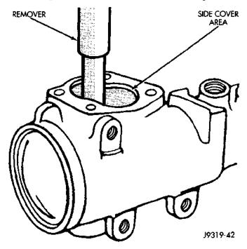
Fig. 26 Needle Bearing Removal
