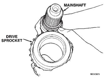
Fig. 30 Drive Sprocket Removal
