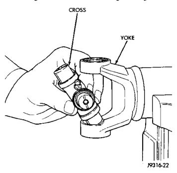
Fig. 21 Install Cross In Yoke
