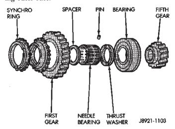
Fig. 122 First And Fifth Gear Components
