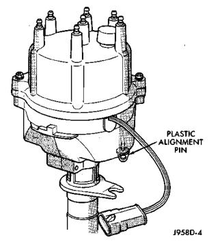
Fig. 42 Plastic Alignment Pin
