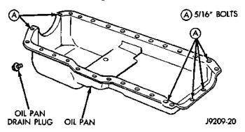
Fig. 40 Position of 5/16 inch Oil Pan Bolts
