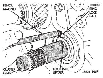
Fig. 93 Install Fifth Gear Thrust Ring Lock Ball
