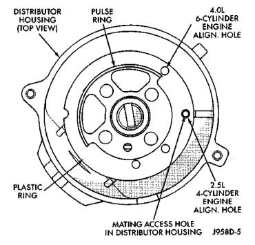
Fig. 47 Pin Alignment Holes
