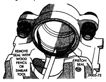
Fig. 48 Piston Seal Removal
