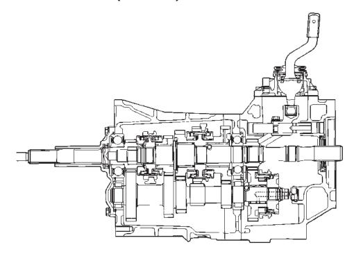
Fig. 1 AX5 Manual Transmission
