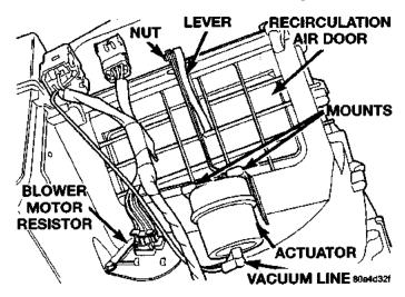
Fig. 35 Recirculation Air Door Vacuum Actuator Remove/Install
