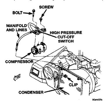
Fig. 11 Compressor Remove/Install
