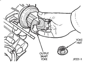
Fig. 75 Output Shaft Yoke Installation
