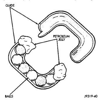
Fig. 23 Balls in the Return Guide
