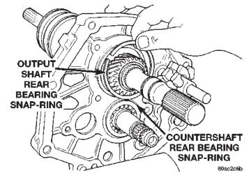
Fig. 61 Remove Output Shaft Rear Bearing Snap-ring
