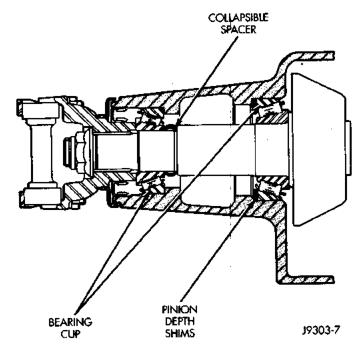
Fig. 38 Pinion Shim and Spacer Locations—typical
