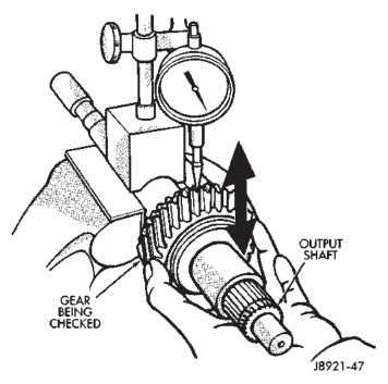
Fig. 126 Check Gear-To-Shaft Oil Clearance
