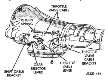
Fig. 178 Throttle Cable Attachment At Transmission
