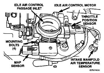
Fig. 34 Throttle Body and Sensor Locations-4.0L Shown
