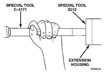
Fig. 14 Install Extension Housing Seal
