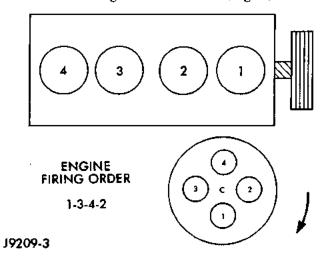
Fig. 1 Engine Firing Order
