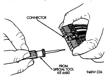
Fig. 18 Terminal Removal
