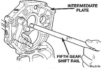
Fig. 67 Remove Fifth Gear Shift Rail
