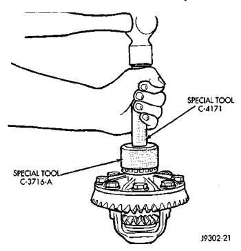
Fig. 24 Install Differential Side Bearings
