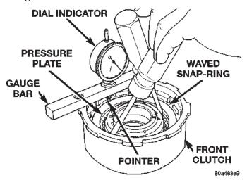
Fig. 136 Measuring Front Clutch Pack Clearance REAR CLUTCH
