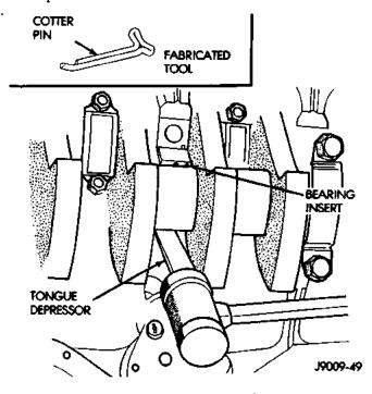
Fig. 47 Removing Upper Inserts
