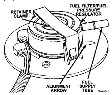
Fig. 11 Fuel Filter/Fuel Pressure Regulator
