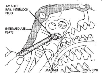
Fig. 85 Install 1-2 Shift Rail Interlock Plug
