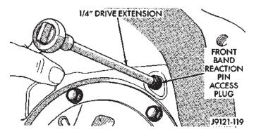
Fig. 87 Front Band Reaction Pin Access Plug
