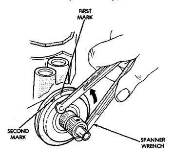
Fig. 30 Aligning To The Second Mark
