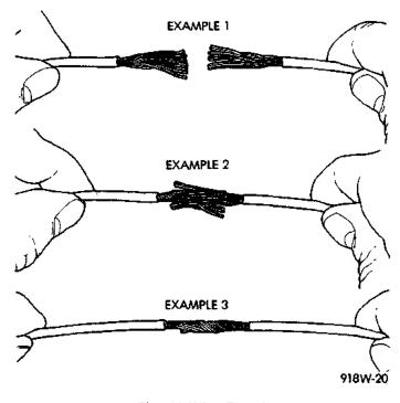
Fig. 11 Wire Repair
