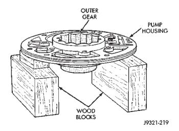
Fig. 126 Supporting Pump And Installing Outer Gear
