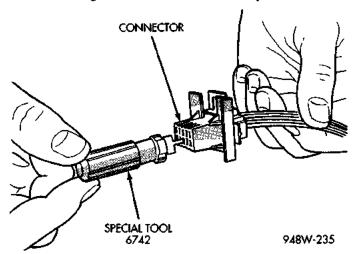
Fig. 13 Using Special Tool 6742
