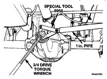
Fig. 13 Tightening Pinion Shaft Nut
