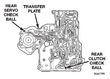
Fig. 50 Rear Servo and Rear Clutch Check Balls
