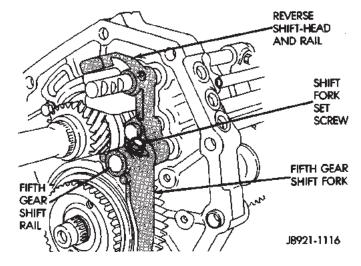
Fig. 103 Install Fifth Gear Shift Fork Retainer Bolt
