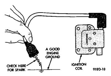
Fig. 10 Checking for Spark-Typical
