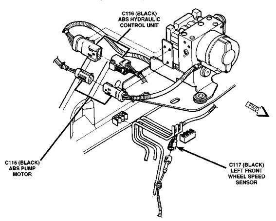
Fig. 5 ABS Hydraulic Control Unit
