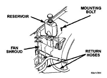
Fig. 4 Pump Reservoir-2.5L
