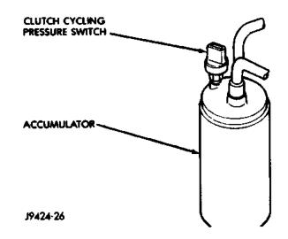
Fig. 5 Low Pressure Cycling Clutch Switch
