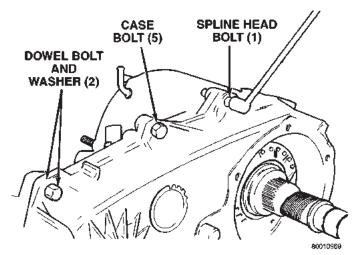
Fig. 18 Rear Case Alignment Bolt Locations
