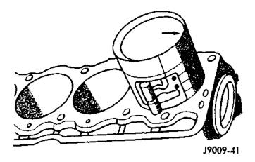
Fig. 14 Rod and Piston Assembly Installation
