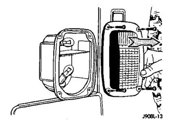
Fig. 2 Lens Removal
