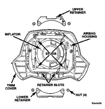
Fig. 7 Trim Cover Retainers Remove/Install
