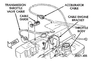
Fig. 177 Throttle Cable Attachment At Engine
