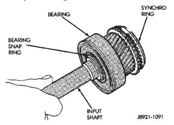
Fig. 98 Input Shaft Components
