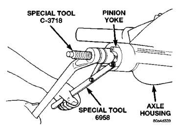
Fig. 44 Pinion Yoke Installation
