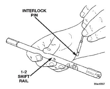
Fig. 77 Install 1-2 Shift Rail Interlock Pin
