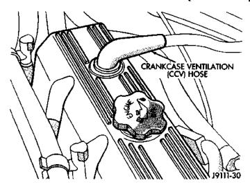
Fig. 7 Crankcase Ventilation (CCV) Hose (2.5L Engine)
