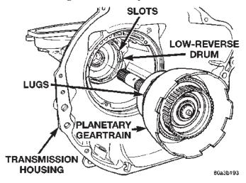
Fig. 96 Output Shaft And Planetary Geartrain
