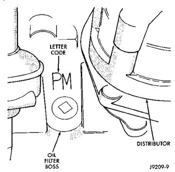
Fig. 4 Oversize and Undersize Component Code Location
