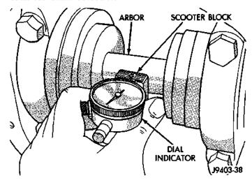
Fig. 67 Pinion Gear Depth Measurement—Typical
