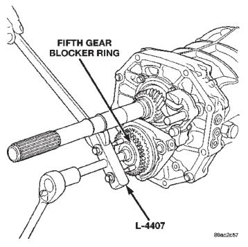
Fig. 52 Remove Fifth Gear Blocker Ring
