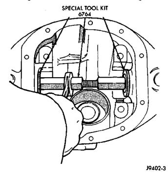
Fig. 25 Axle Seal Installation
