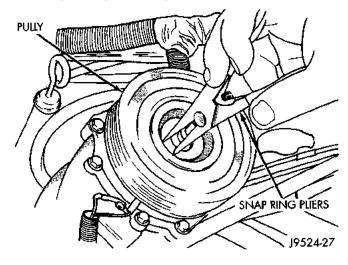
Fig. 14 External Snap Ring Remove
