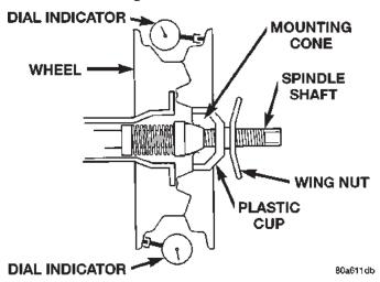
Fig. 4 Lateral Runout
