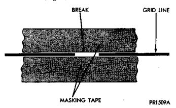
Fig. 3 Grid Line Repair - Typical
