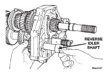
Fig. 57 Remove Reverse Idler Shaft
