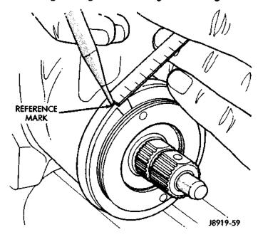
Fig. 29 Remarking The Housing
