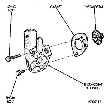
Fig. 28 Thermostat Removal/Installation
