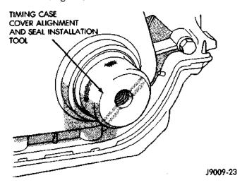
Fig. 36 Timing Case Cover Alignment and Seal Installation Tool 6139
