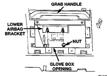
Fig. 20 Passenger Airbag Module Lower Bracket
