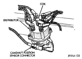
Fig. 17 Distributor and Wiring—Typical (4.0L Engine Shown)
