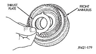
Fig. 160 Positioning Thrust Plate On Front Annulus Support
