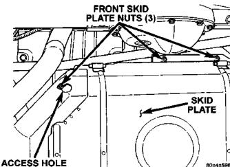
Fig. 25 Fuel Tank Mounting Nuts—Front
