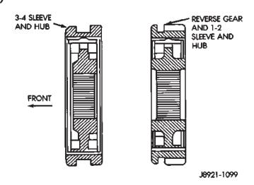
Fig. 118 Synchronizer Identification
