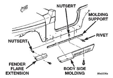
Fig. 16 Body Side Molding
