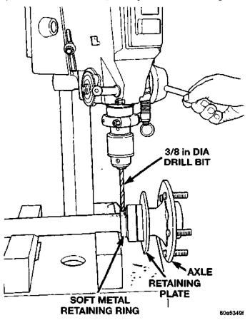
Fig. 15 Drill Retaining Ring
