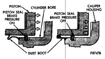
Fig. 4 Lining Wear Compensation By Piston Seal
