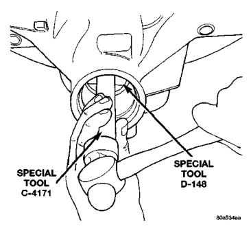
Fig. 38 Rear Bearing Cup Removal
