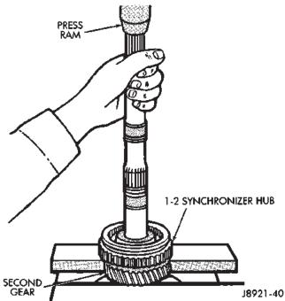
Fig. 105 Remove Second Gear, Reverse Gear, And 1–2 Synchronizer
