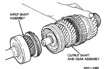
Fig. 97 Separate Input and Output Shafts
