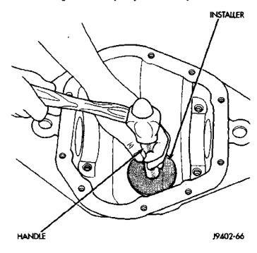
Fig. 33 Pinion Inner Bearing Cup Installation
