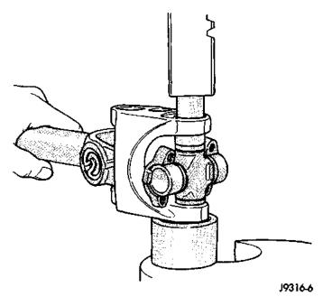
Fig. 24 Press Out Bearing
