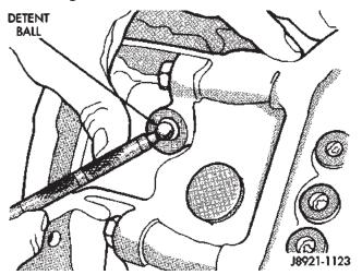
Fig. 47 Install Detent Ball
