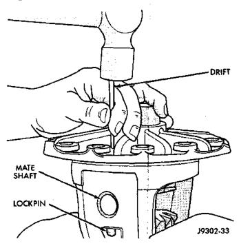
Fig. 51 Mate Shaft Roll Pin Removal
