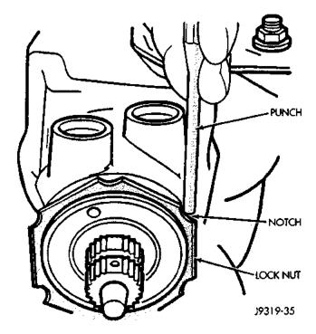
Fig. 13 Tighten Lock Nut
