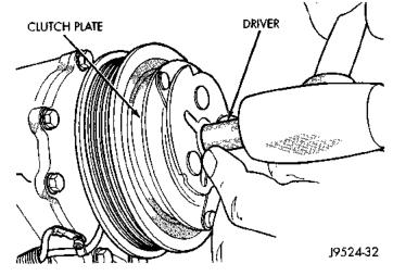
Fig. 20 Clutch Plate Driver
