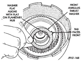
Fig. 161 Installing Front Annulus Thrust Washer
