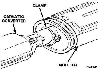
Fig. 5 Catalytic Converter to Muffler Connection
