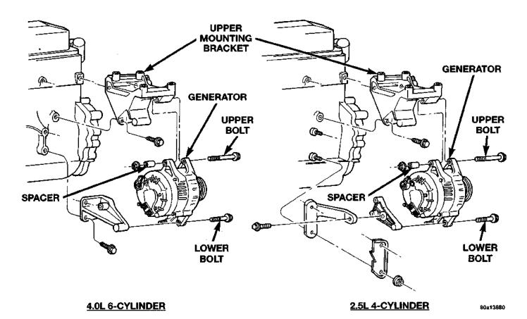
Fig. 4 Generator Remove/Install
