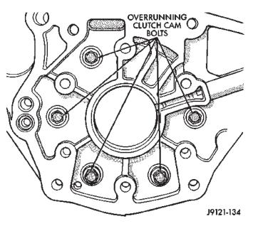
Fig. 83 Overrunning Clutch Cam Bolt Locations
