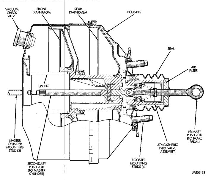
Fig. 1 Power Brake Booster-Typical
