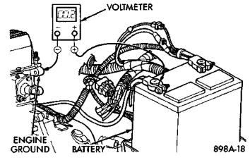
Fig. 5 Test Ground Circuit Resistance - Typical
