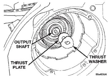
Fig. 77 Output Shaft Thrust Plate and Washer
