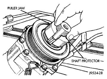
Fig. 15 Shaft Protector and Puller
