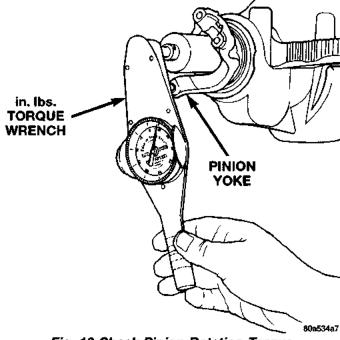
Fig. 12 Check Pinion Rotation Torque
