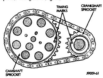
Fig. 32 Crankshaft—Camshaft Alignment—Typical
