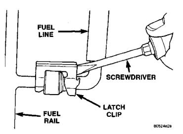
Fig. 9 Latch Clip Removal—Typical
