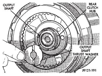
Fig. 101 Output Shaft Thrust Washer
