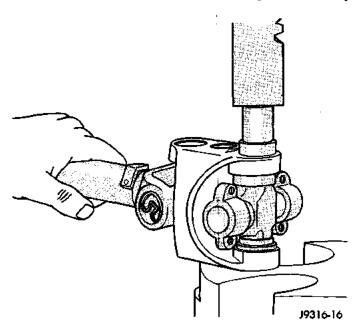
Fig. 34 Press In Bearing Assembly
