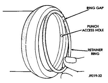
Fig. 7 Installing The Retaining Ring
