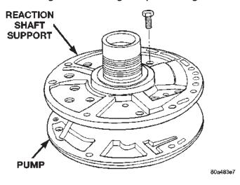
Fig. 119 Pump Support Bolts
