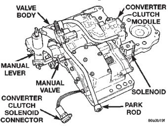
Fig. 39 Valve Body Assembly
