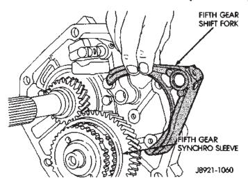
Fig. 54 Remove Fifth Gear Shift Fork
