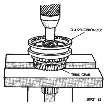
Fig. 117 Remove 3-4 Synchronizer And Third Gear
