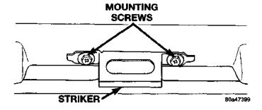
Fig. 14 Glove Box Latch Striker Remove/Install
