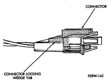
Fig. 17 Connector Locking Wedge
