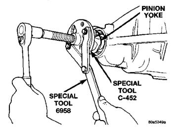
Fig. 27 Pinion Yoke Removal
