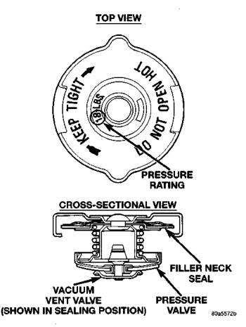
Fig. 5 Radiator Pressure Cap
