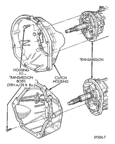
Fig. 10 Clutch Housing
