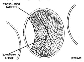
Fig. 1 Cylinder Bore Crosshatch Pattern
