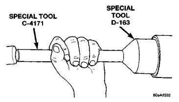
Fig. 35 Pinion Seal Installation
