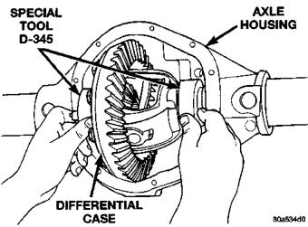
Fig. 74 Install Differential Case W/Dummy Bearings
