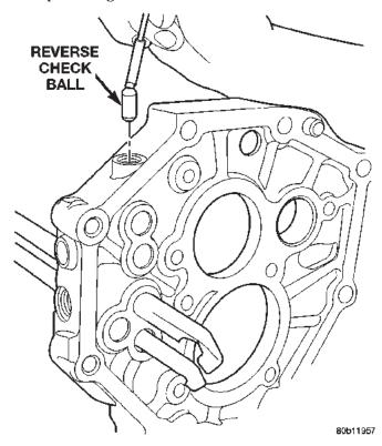
Fig. 78 Install Reverse Check Ball
