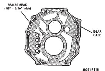
Fig. 33 Apply Sealer to Transmission Gear Case
