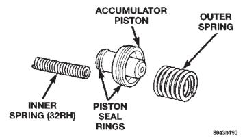
Fig. 28 Accumulator Piston And Springs
