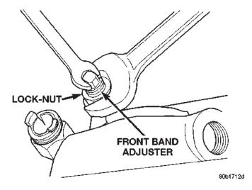
Fig. 179 Front Band Adjustment Screw Location
