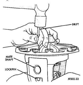
Fig. 55 Mate Shaft Roll Pin Removal
