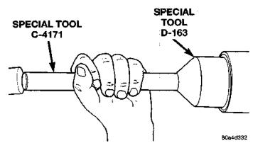
Fig. 10 Pinion Seal Installation
