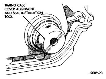
Fig. 45 Timing Case Cover Alignment and Seal Installation Tool 6139
