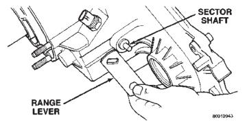
Fig. 17 Range Lever Removal
