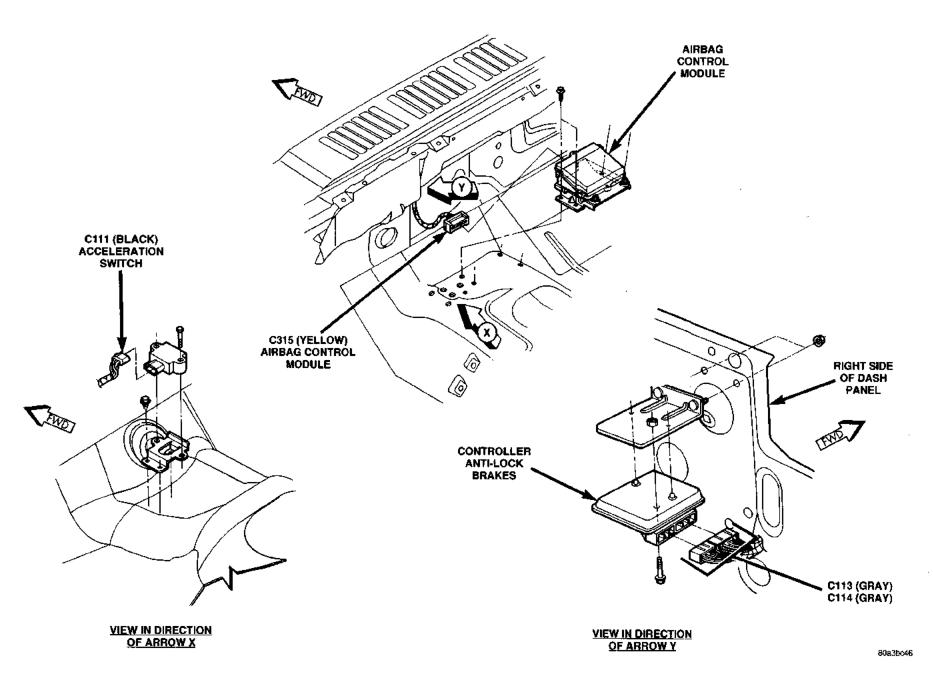
Fig. 15 Airbag Control Module and Controller, Antilock Brakes
