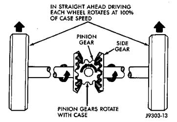
Fig. 2 Differential Operation—Straight Ahead Driving
