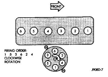
Fig. 33 Engine Firing Order—4.0L 6-Cylinder Engine
