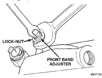
Fig. 72 Front Band Adjusting Screw Lock Nut
