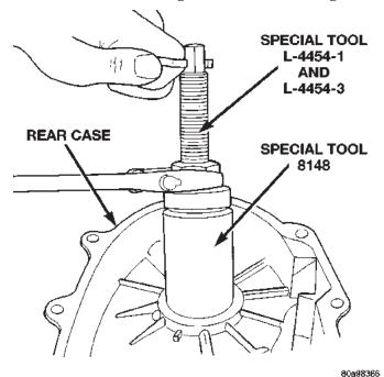
Fig. 46 Output Shaft Rear Bearing Removal
