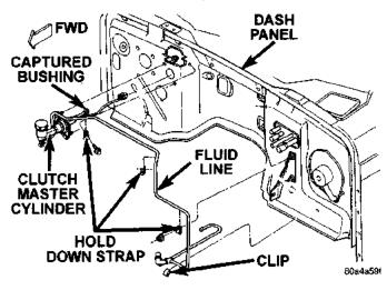
Fig. 10 Right Hand Drive Clutch Master Cylinder INSTALLATION
