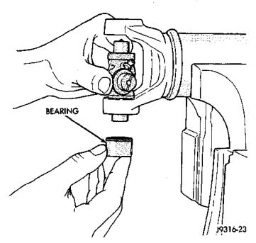
Fig. 22 Install Bearing On Trunnion
