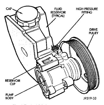
Fig. 1 Typical TC Series Pump With Integral Reservoir
