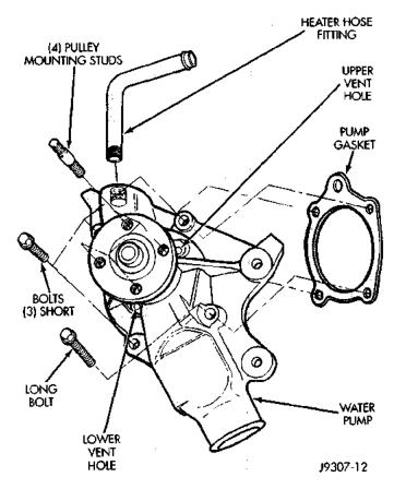
Fig. 27 Water Pump Remove/Install—Typical
