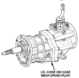
Fig. 2 Transmission Identification
