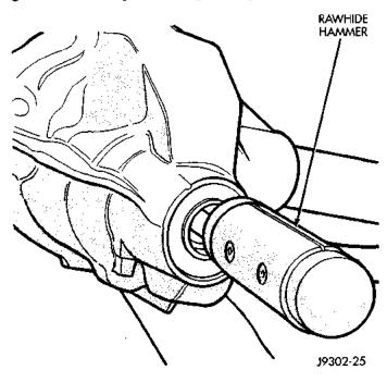
Fig. 32 Remove Pinion Gear
