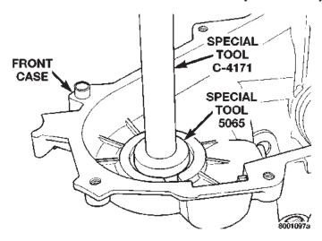
Fig. 42 Front Output Shaft Bearing Removal
