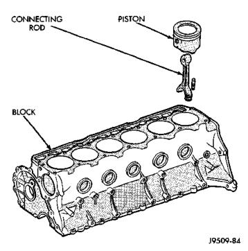
Fig. 48 Removal of Connecting Rod and Piston
