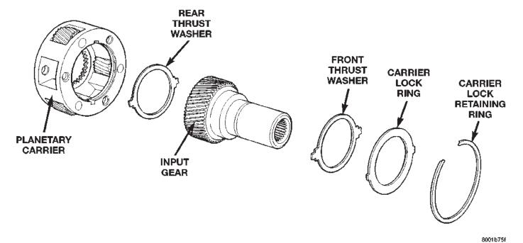
Fig. 81 Input Gear And Carrier Components
