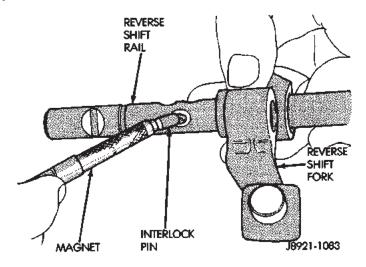
Fig. 79 Remove Reverse Shift Rail Interlock Pin
