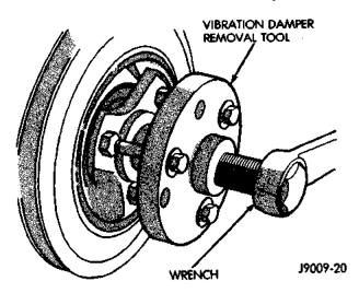
Fig. 29 Vibration Damper Removal Tool 7697
