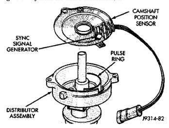
Fig. 3 Camshaft Position Sensor—Typical
