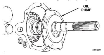
Fig. 13 Oil Pump Removal
