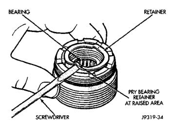
Fig. 9 Bearing Retainer
