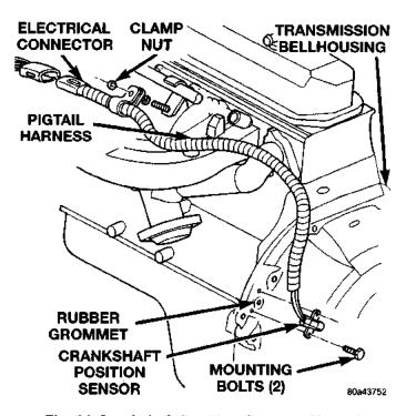
Fig. 21 Crankshaft Position Sensor—Manual Transmission (Typical)
