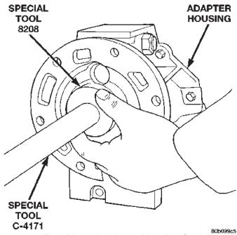
Fig. 15 Install Adapter Housing Seal
