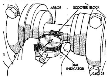
Fig. 52 Pinion Gear Depth Measurement—Typical
