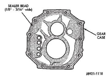
Fig. 36 Apply Sealer to Transmission Gear Case
