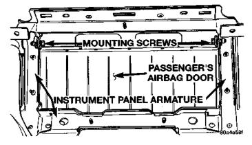
Fig. 11 Passenger Airbag Door Remove/Install
