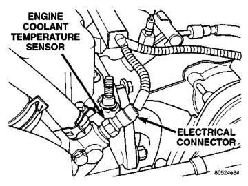
Fig. 20 Engine Coolant Temp. Sensor—4.0L Shown
