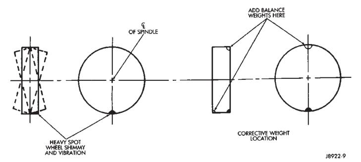
Fig. 7 Dynamic Unbalance & Balance
