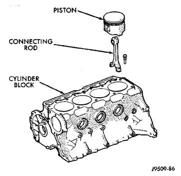
Fig. 55 Removal of Connecting Rod and Piston Assembly
