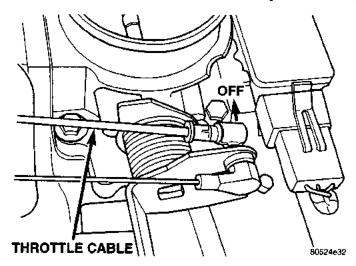
Fig. 28 Throttle Cable at Throttle Body—Typical
