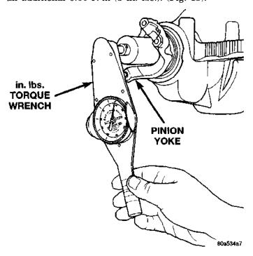
Fig. 13 Check Pinion Rotation Torque
