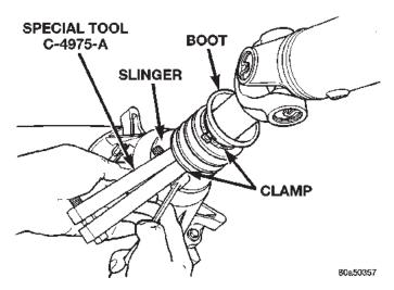
Fig. 79 Slinger Boot Installation
