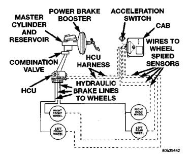
Fig. 1 Antilock Brake System
