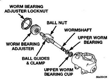
Fig. 9 Worm Shaft and Ball Nut
