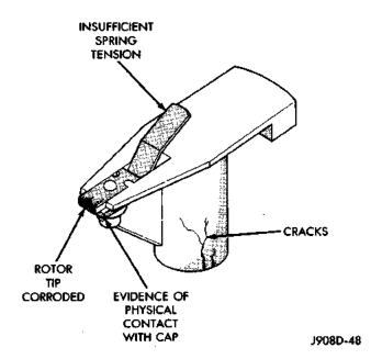
Fig. 18 Rotor Inspection—Typical
