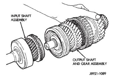
Fig. 106 Separate Input and Output Shafts
