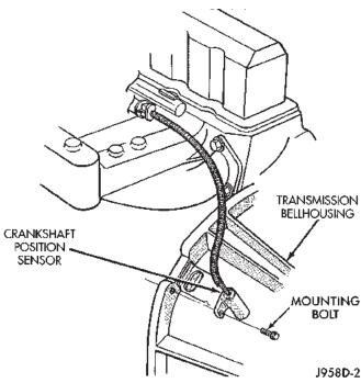
Fig. 17 Crankshaft Position Sensor—4.0L Engine
