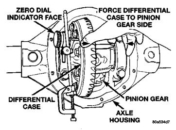
Fig. 81 Hold Differential Case and Zero Dial Indicator
