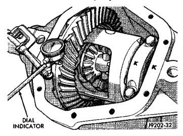
Fig. 83 Ring Gear Backlash Measurement
