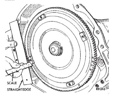
Fig. 20 Checking Torque Converter Seating EXTENSION HOUSING
