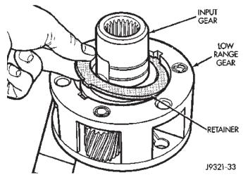
Fig. 36 Input Gear Retainer Removal
