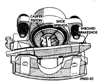
Fig. 28 Inboard Brake Shoe Removal
