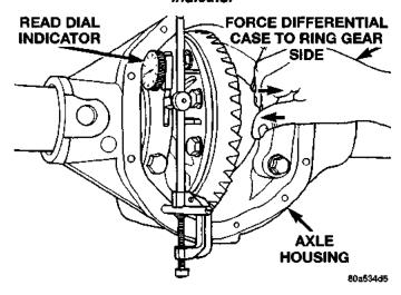
Fig. 80 Hold Differential Case and Read Dial Indicator
