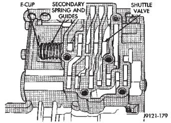
Fig. 52 Shuttle Valve E-Clip And Secondary Spring
