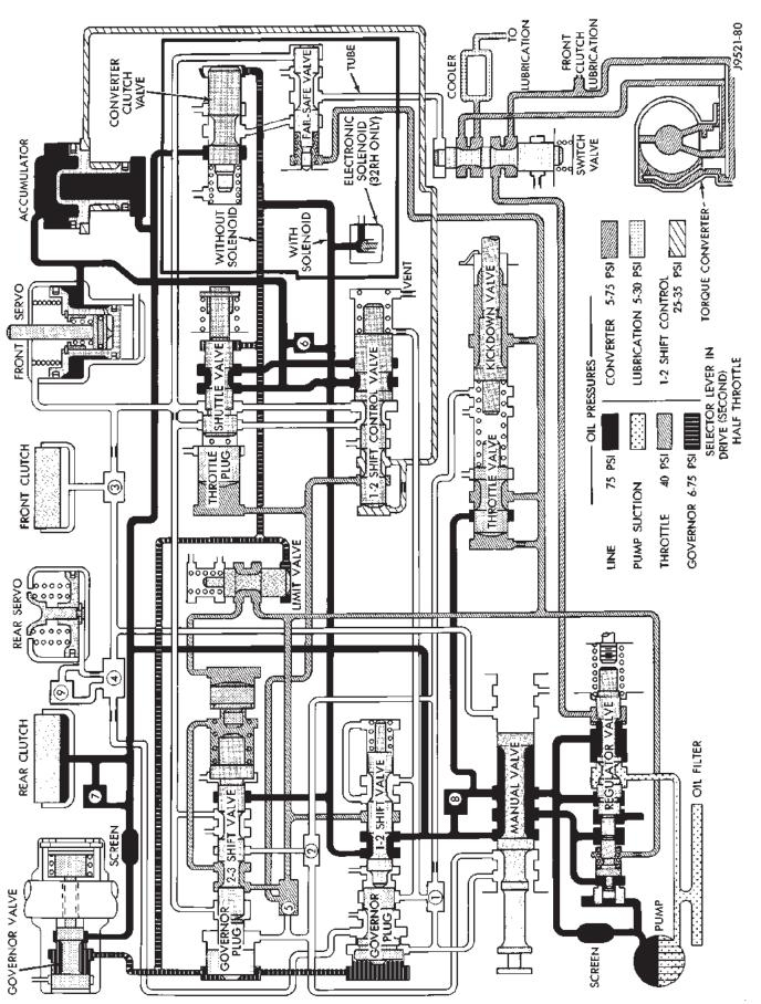
HYDRAULIC FLOW IN D-SECOND GEAR
