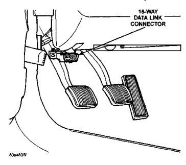
Fig. 1 Data Link (Diagnostic) Connector Location
