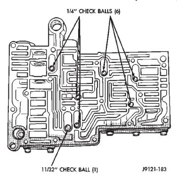
Fig. 58 Correct Position Of Valve Body Check Balls
