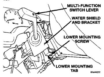
Fig. 15 Water Shield Lower Screw Remove/Install
