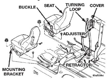
Fig. 60 Bucket Seat Removal
