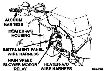
Fig. 32 High Speed Blower Motor Relay
