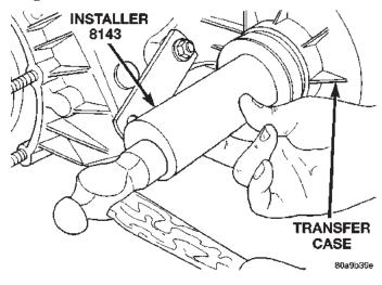
Fig. 45 Front Output Seal Installation
