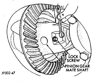
Fig. 14 Mate Shaft Lock Screw
