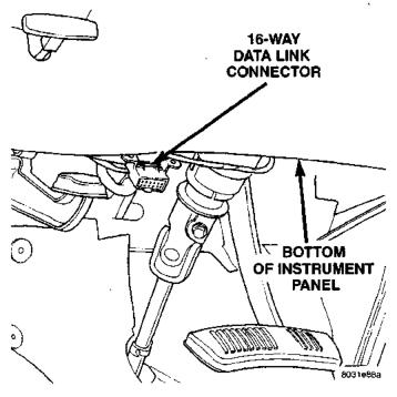
Fig. 12 16–Way Data Link Connector—Typical EXAMPLES:
