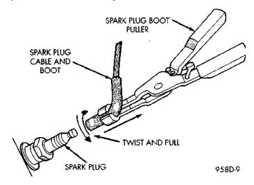
Fig. 9 Cable Removal
