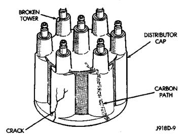
Fig. 16 Cap Inspection—External—Typical
