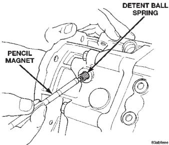
Fig. 20 Remove Detent Spring
