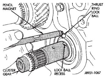
Fig. 56 Remove Fifth Gear Thrust Ring Lock Ball
