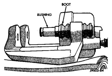
Fig. 50 Bushings And Boots Installation
