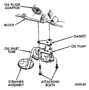
Fig. 53 Oil Pump Assembly
