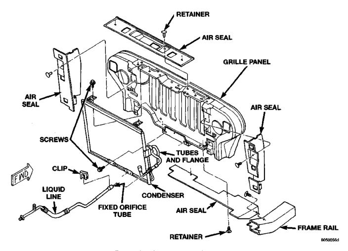
Fig. 24 Condenser Remove/Install
