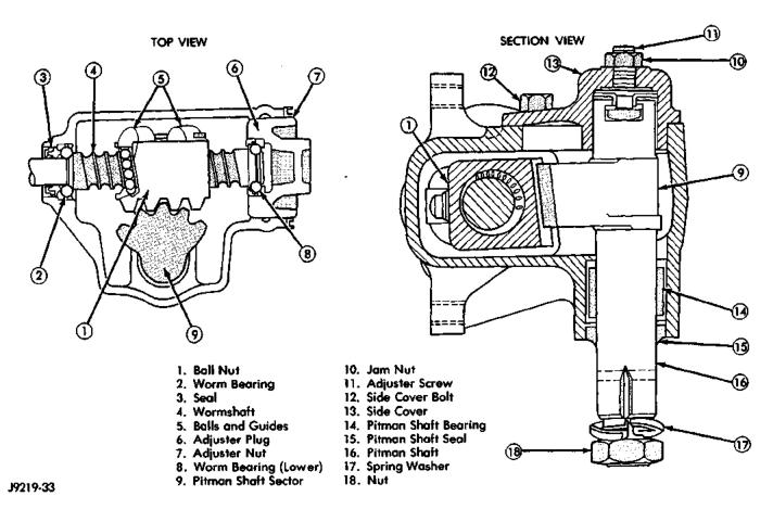
Fig. 1 Manual Steering Gear
