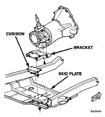
Fig. 21 Rear Mount (Manual Transmission)
