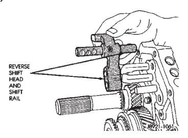
Fig. 101 Install Reverse Shift Head And Rail Assembly
