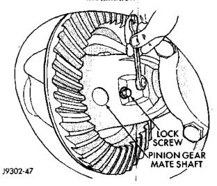
Fig. 61 Mate Shaft Roll Pin Installation
