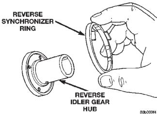
Fig. 118 Remove Reverse Idler Gear Synchronizer Ring
