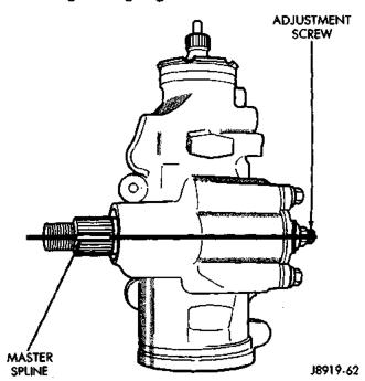
Fig. 31 Steering Gear Centered
