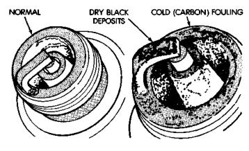
Fig. 24 Normal Operation and Cold (Carbon) Fouling
