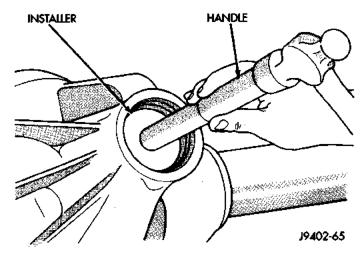
Fig. 40 Pinion Outer Bearing Cup Install
