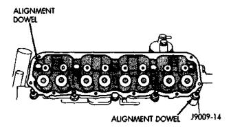
Fig. 30 Alignment Dowel Locations
