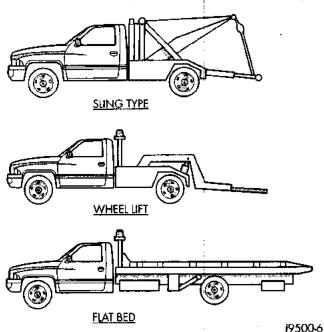
Fig. 2 Tow Vehicles With Approved Equipment SAFETY PRECAUTIONS
