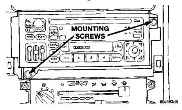
Fig. 3 Radio Remove/Install
