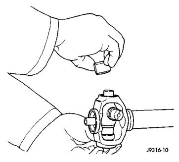
Fig. 28 Install Bearing Assembly
