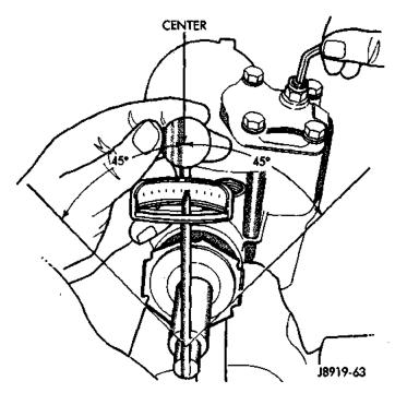
Fig. 32 Checking Over-center Rotation Torque
