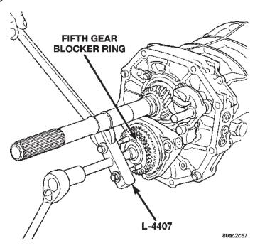
Fig. 56 Remove Fifth Gear Blocker Ring
