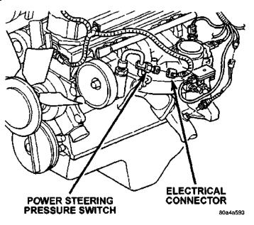
Fig. 9 Power Steering Pump Pressure Switch—2.5L Engine
