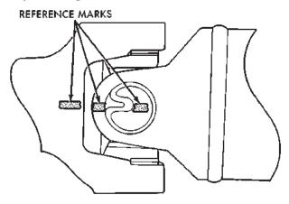
J9316-2 Fig. 10 Align Propeller Shaft And Rear Axle Yokes Alignment Marks
