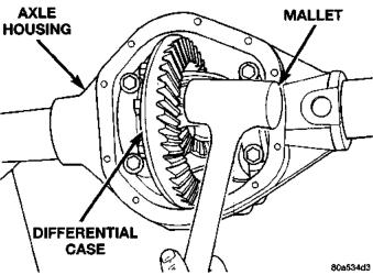
Fig. 71 Seat Ring Gear Side Differential Dummy Side Bearing
