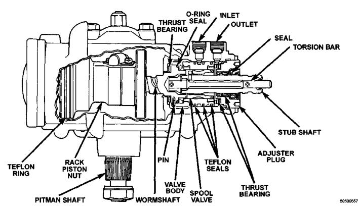
Fig. 1 Power Steering Gear
