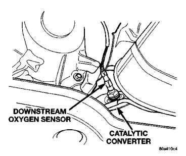
Fig. 22 Downstream Oxygen Sensor
