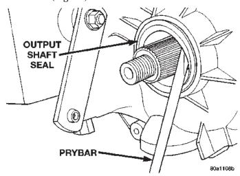
Fig. 40 Front Output Seal Removal
