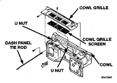
Fig. 10 Cowl Plenum Cover/Grille Panel Remove/ Install
