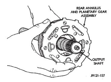
Fig. 150 Installing Rear Annulus And Planetary On Output Shaft
