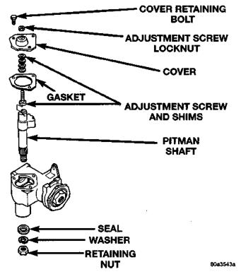
Fig. 5 Manual Steering Gear
