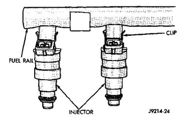
Fig. 20 Injector Mounting
