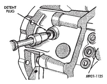
Fig. 49 Install Detent Ball Plug
