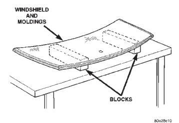
Fig. 3 Work Surface Set up and Molding Installation
