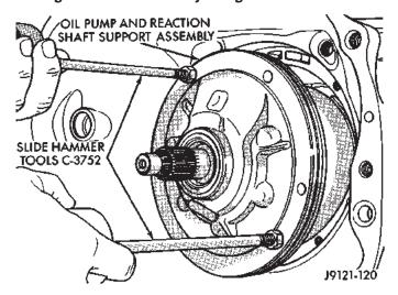
Fig. 73 Oil Pump/Reaction Shaft Support
