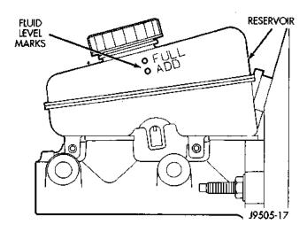
Fig. 2 Master Cylinder-Typical
