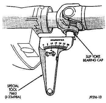
Fig. 9 Front (Output) Angle Measurement (A)— Typical
