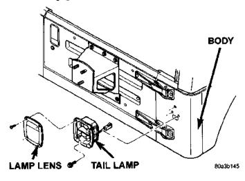
Fig. 6 Tail Lamp Housing
