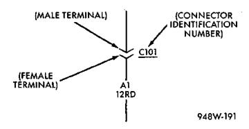
Fig. 4 Connector Identification
