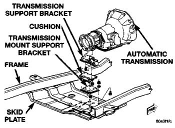
Fig. 4 Transmission Mount—Automatic
