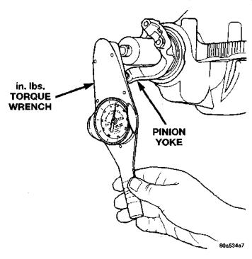
Fig. 40 Check Pinion Gear Rotation Torque
