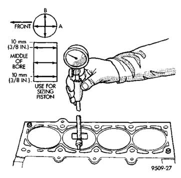
Fig. 66 Cylinder Bore Measurement
