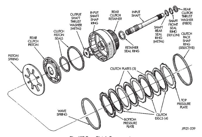
Fig. 137 Rear Clutch Components
