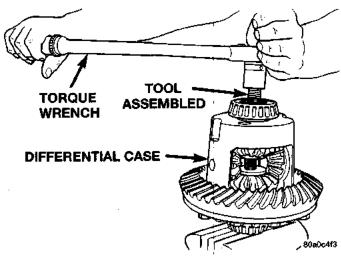
Fig. 54 Tighten Believille Spring Compressor Tool
