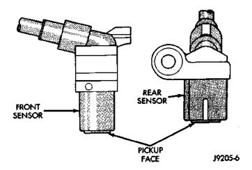
Fig. 4 Typical Wheel Speed Sensors
