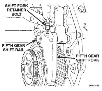
Fig. 51 Remove Shift Fork Retainer Bolt
