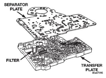
Fig. 57 Transfer And Separator Plates
