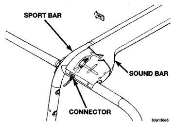
Fig. 7 Sound Bar Wiring Connector Remove/Install
