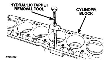
Fig. 28 Hydraulic Valve Tappet Removal— Installation Tool
