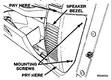
Fig. 5 Instrument Panel Speaker Bezel Remove/ Install
