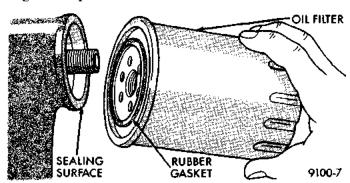
Fig. 10 Oil Filter Sealing Surface—Typical **USED ENGINE OIL DISPOSAL**
