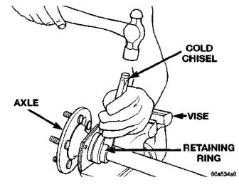
Fig. 16 Cut Retaining Ring
