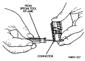
Fig. 23 Terminal Removal Using Special Tool
