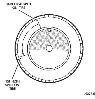
Fig. 10 Remount Tire 90 Degrees In Direction of Arrow
