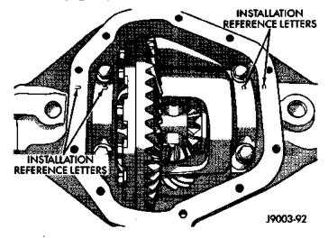
Fig. 18 Bearing Cap Identification
