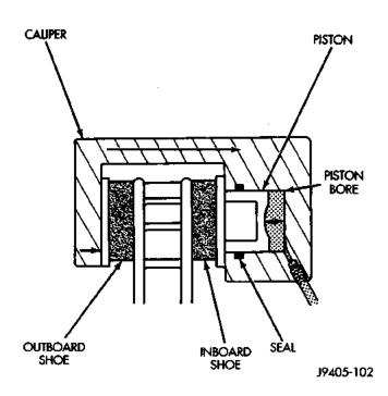
Fig. 3 Brake Caliper Operation
