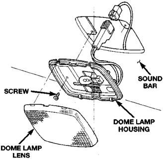
Fig. 9 Sound Bar Dome Lamp
