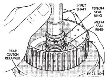
Fig. 97 Input Shaft Seal Ring Location
