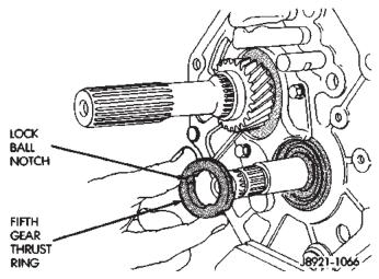
Fig. 94 Install Fifth Gear Thrust Ring
