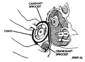
Fig. 38 Camshaft and Crankshaft Sprockets and Chain
