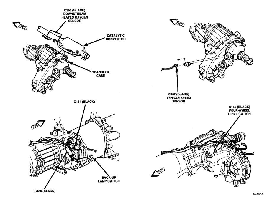
Fig. 12 Transmission and Transfer Case Connectors
