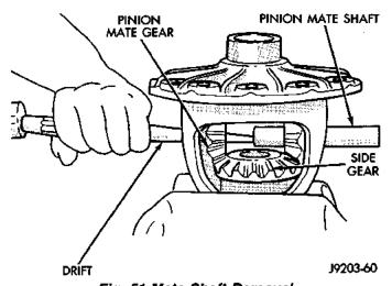
Fig. 51 Mate Shaft Removal
