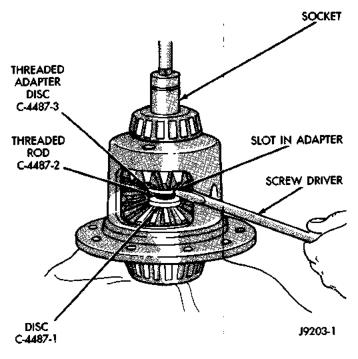
Fig. 53 Threaded Adapter Installation
