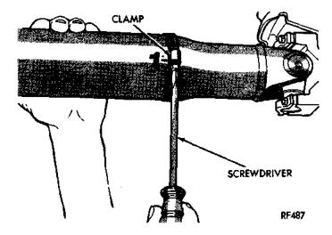
Fig. 5 Clamp Screw At Position 1
