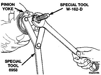
Fig. 11 Pinion Yoke, Install
