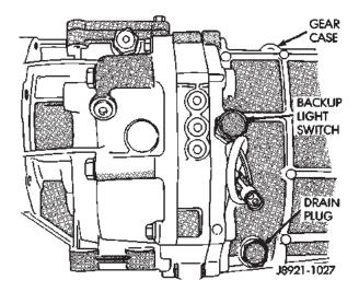
Fig. 4 Drain Plug Location
