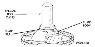
Fig. 130 Pump Oil Seal Installation
