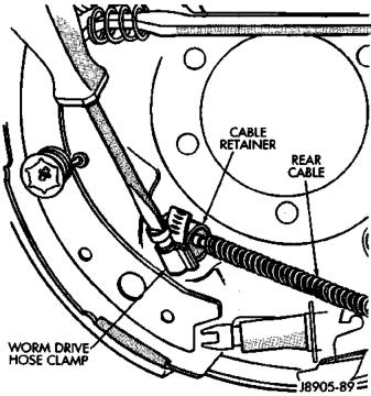
Fig. 39 Cable Retainer
