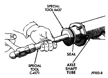
Fig. 17 Axle Shaft Seal Installation
