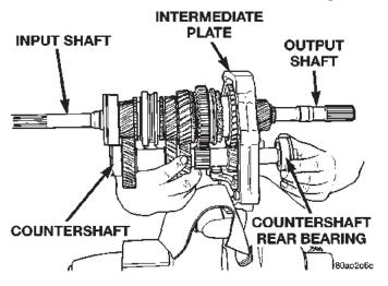
Fig. 62 Remove Countershaft and Countershaft Rear Bearing
