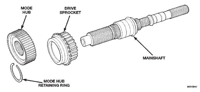
Fig. 80 Mainshaft, Mode Hub, And Drive Sprocket
