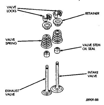
Fig. 26 Valve and Valve Components
