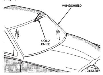
Fig. 1 Cutting Urethane Around Windshield—Typical
