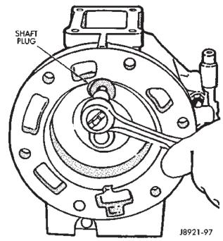
Fig. 42 Shifter Arm Shaft Plug Installation
