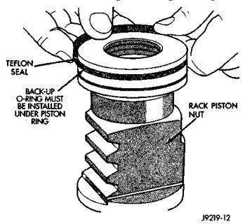
Fig. 21 Rack Piston Teflon Ring and O-Ring
