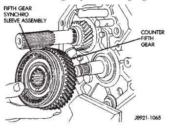
Fig. 98 Install Countershaft Fifth Gear Assembly
