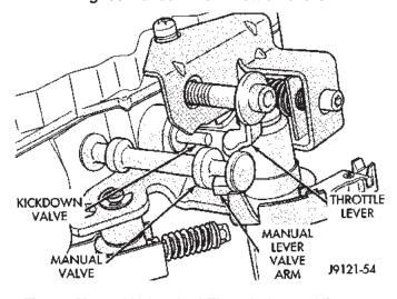
Fig. 67 Manual Valve And Throttle Lever Alignment
