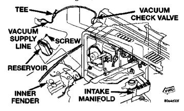
Fig. 27 Vacuum Reservoir Remove/Install
