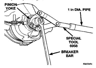
Fig. 7 Pinion Nut
