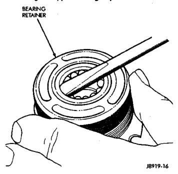
Fig. 14 Lower Bearing Retainer
