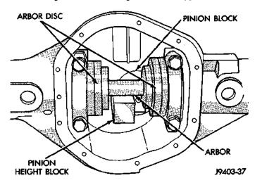
Fig. 51 Gauge Tools In Housing—Typical
