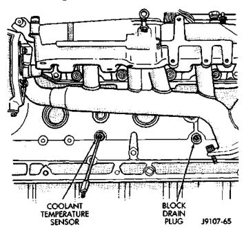
Fig. 19 Draining Coolant—4.0L 6-Cylinder Engine
