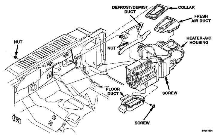
Fig. 36 Heater-A/C Housing Remove/Install
