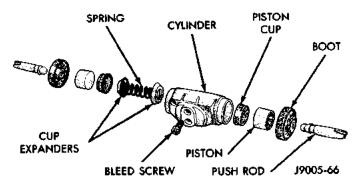
Fig. 55 Wheel Cylinder Components
