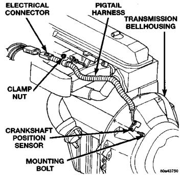
Fig. 38 Crankshaft Position Sensor—4.0L 6-Cyl. Engine—Auto. Trans.
