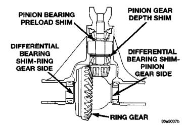
Fig. 1 Axie Adjustment Shims
