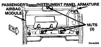
Fig. 5 Passenger Airbag Module Remove/Install
