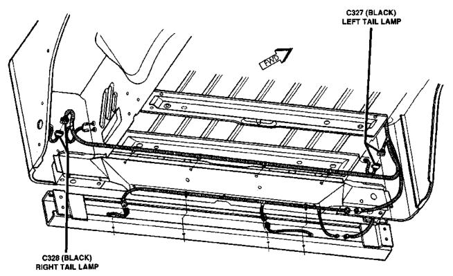
Fig. 19 Rear Body Wiring Connectors
