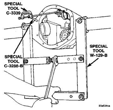
Fig. 20 Spread Axle Housing
