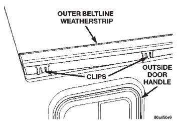
Fig. 30 Full Door Outer Belt Seal
