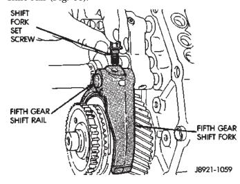
Fig. 53 Remove Fifth Gear Shift Fork Retainer Bolt
