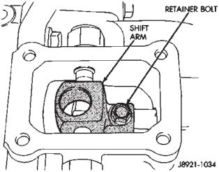
Fig. 41 Install Shift Arm Retainer Bolt
