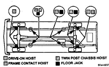
Fig. 5 Vehicle Lifting Locations
