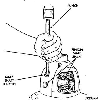
Fig. 46 Mate Shaft Roll Pin Installation
