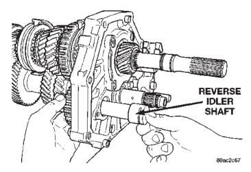
Fig. 90 Install Reverse Idler Shaft
