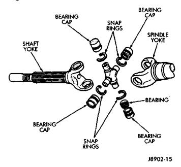
Fig. 42 Axle Shaft Outer U-Joint
