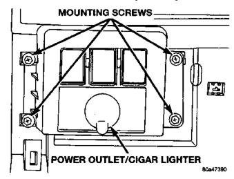
Fig. 17 Accessory Switch Bezel Remove/Install
