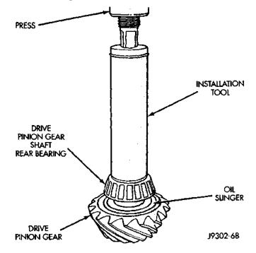
Fig. 36 Shaft Inner Bearing Installation
