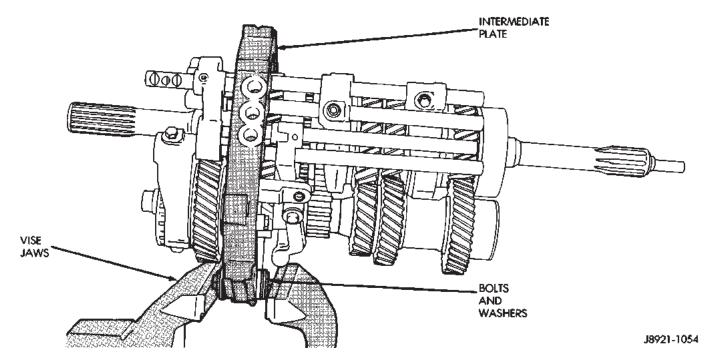
Fig. 51 Positioning Intermediate Plate In Vise
