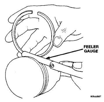
Fig. 7 Ring Side Clearance Measurement Ring Gap Measurement
