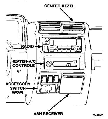
Fig. 2 Center Bezel Remove/Install
