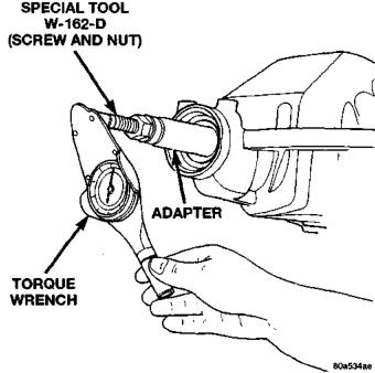
Fig. 45 Measure Pinion Bearing Preload.
