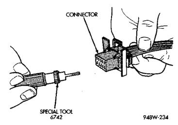
Fig. 12 Molex Connector Repair
