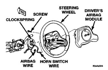
Fig. 4 Driver Airbag Module Remove/Install
