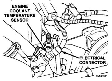
Fig. 30 Engine Coolant Temperature Sensor— Typical
