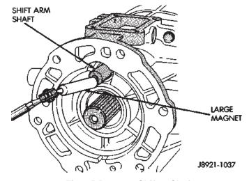
Fig. 25 Remove Shifter Shaft
