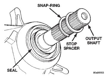
Fig. 9 Slinger Stop Spacer and Snap-ring
