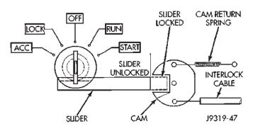
Fig. 4 Ignition Key Cylinder Actuation
