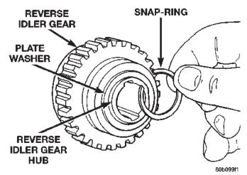
Fig. 115 Remove Reverse Idler Gear Snap-ring
