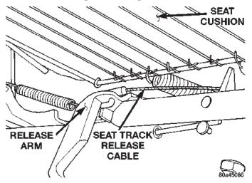
Fig. 3 Seat Track Release Cable
