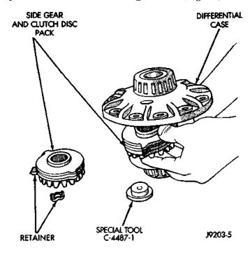
Fig. 57 Side Gear & Clutch Disc Removal
