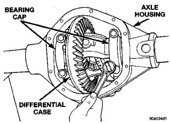
Fig. 69 Tighten Bolts Holding Bearing Caps
