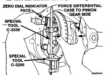
Fig. 58 Hold Differential Case and Zero Dial Indicator
