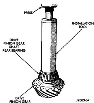
Fig. 42 Shaft Rear Bearing Installation
