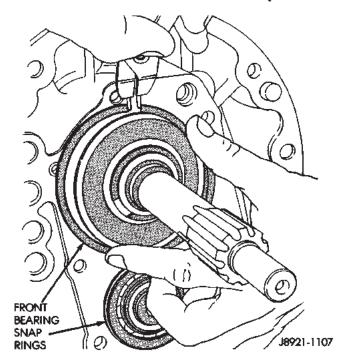
Fig. 38 Install Front Bearing Snap-rings
