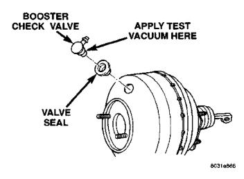
Fig. 9 Vacuum Check Valve And Seal COMBINATION VALVE
