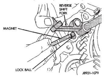
Fig. 68 Remove Fifth Gear Shift Rail Lock Ball
