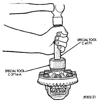
Fig. 27 Install Differential Side Bearings
