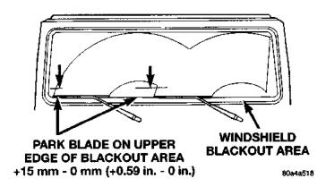
Fig. 8 Front Wiper Arm Installation
