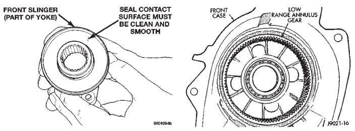
Fig. 85 Seal Contact Surface Of Yoke Slinger
