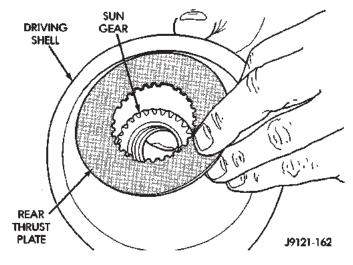
Fig. 154 Installing Driving Shell Rear Thrust Plate
