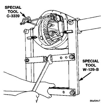
Fig. 21 Spread Axle Housing
