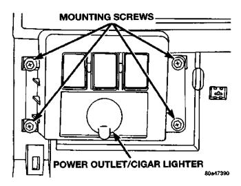
Fig. 5 Accessory Switch Bezel Remove/Install
