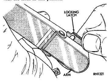
Fig. 7 Wiper Arm Remove/Install
