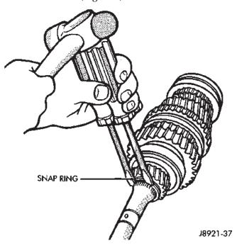
Fig. 102 Remove Fifth Gear Snap-ring
