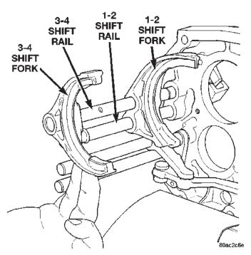
Fig. 64 Remove 3-4 Shift Fork
