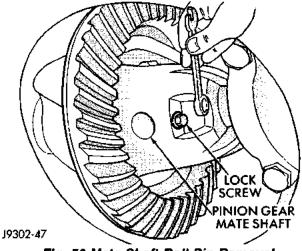
Fig. 50 Mate Shaft Roll Pin Removal
