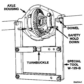
Fig. 19 Install Axle Housing Spreader
