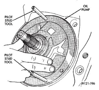
Fig. 109 Installing Oil Pump And Reaction Shaft Support
