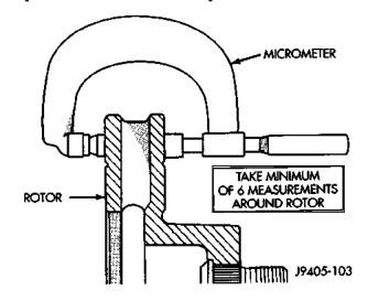
Fig. 11 Measuring Rotor Thickness
