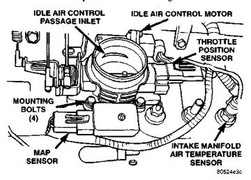
Fig. 31 Intake Manifold Air Temperature Sensor— Typical
