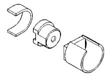
Remover/Installer Suspension Bushing 7932 (J-35581)
