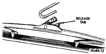
Fig. 6 Front or Rear Wiper Blade Remove/Install - Typical
