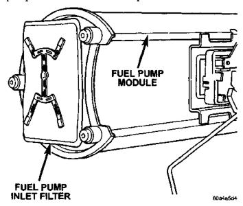
Fig. 16 Fuel Pump Inlet Filter
