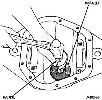
Fig. 41 Pinion Rear Bearing Cup Install
