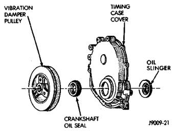
Fig. 35 Timing Case Cover Components
