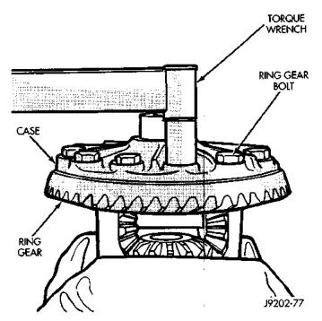
Fig. 29 Ring Gear Bolt Installation
