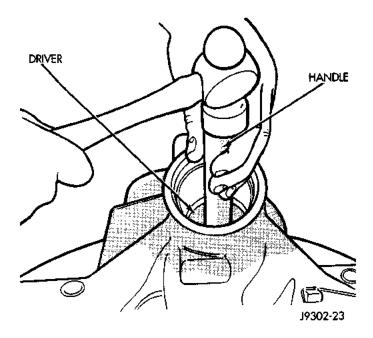
Fig. 35 Inner Bearing Cup Removal
