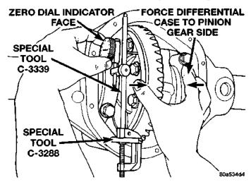
Fig. 73 Hold Differential Case and Zero Dial Indicator
