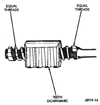
Fig. 11 Worm Shaft and Ball Nut
