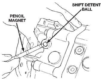
Fig. 21 Remove Detent Ball
