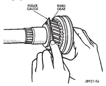
Fig. 120 Check Third Gear Clearance
