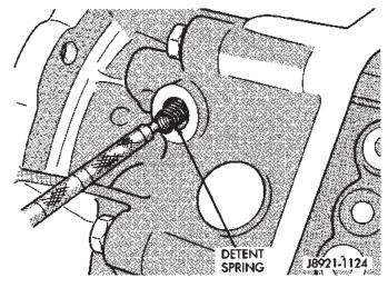
Fig. 21 Remove Detent Spring
