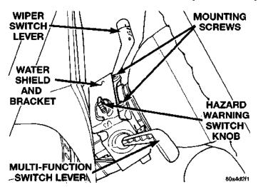
Fig. 5 Water Shield Upper Screws Remove/Install
