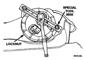
Fig. 15 Locknut Removal/Installation—Typical
