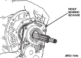
Fig. 29 Remove Front Bearing Retainer
