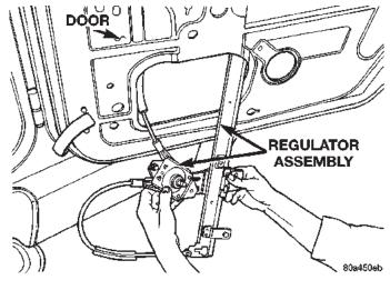
Fig. 34 Regulator Removal
