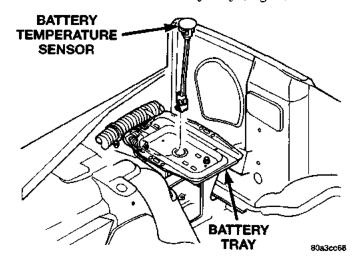
Fig. 1 Battery Temperature Sensor Location
