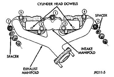
Fig. 10 Intake/Engine Exhaust Manifold Installation 2.5L Engine
