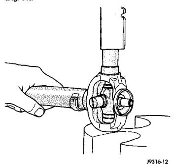
Fig. 30 Press in Bearing Assembly
