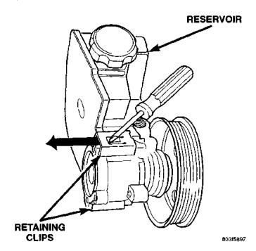
Fig. 7 Pump Reservoir Clips
