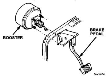
Fig. 22 Booster Mounting Nuts
