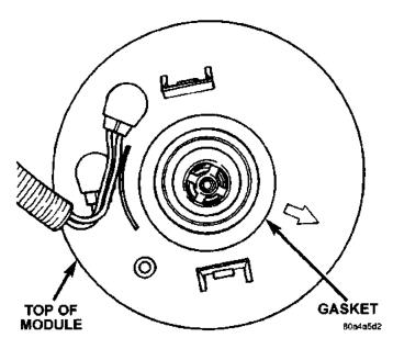
Fig. 12 Fuel Filter/Fuel Pressure Regulator Gasket
