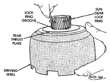
Fig. 156 Installing Sun Gear Lock Ring
