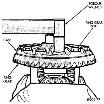
Fig. 32 Ring Gear Bolt Installation
