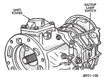
Fig. 50 Installing Shift Tower And Backup Lamp Switch
