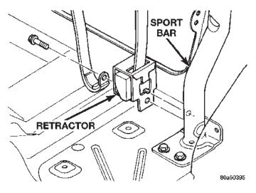
Fig. 52 Front Retractor
