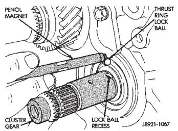
Fig. 60 Remove Fifth Gear Thrust Ring Lock Ball
