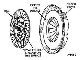
Fig. 4 Clutch Disc And Pressure Plate Inspection
