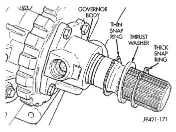
Fig. 32 Snap Rings And Spacer
