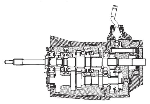
Fig. 1 AX15 Manual Transmission
