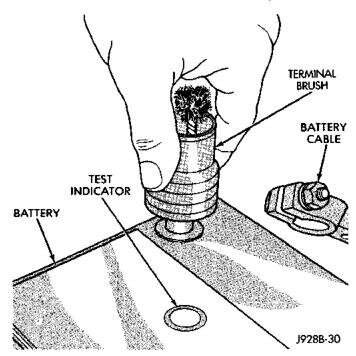
Fig. 15 Clean Battery Terminal Post - Typical
