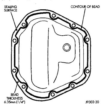
Fig. 3 Typical Housing Cover With Sealant
