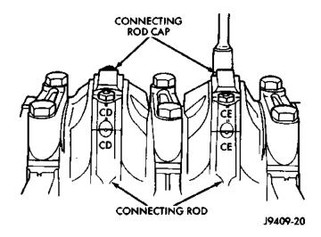
Fig. 54 Stamped Connecting Rods and Caps
