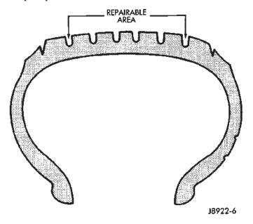
Fig. 11 Tire Repair Area
