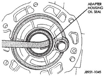
Fig. 14 Remove Adapter Housing Seal
