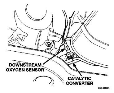
Fig. 42 Downstream Oxygen Sensor Location
