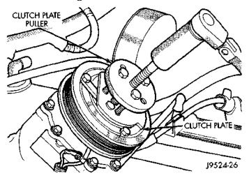
Fig. 13 Clutch Plate Remove
