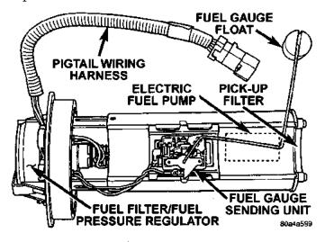
Fig. 17 Fuel Gauge Sending Unit Location
