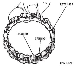
Fig. 112 Overrunning Clutch Rollers, Springs, Retainer
