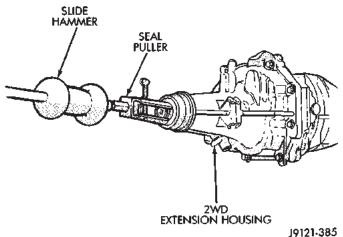
Fig. 12 Remove Extension Housing Seal
