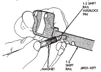
Fig. 86 Install 1-2 Shift Rail Interlock Pin
