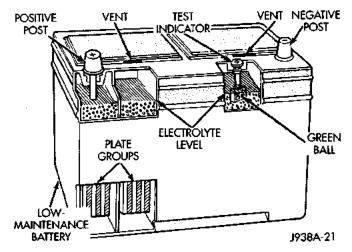
Fig. 1 Low-Maintenance Battery - Typical
