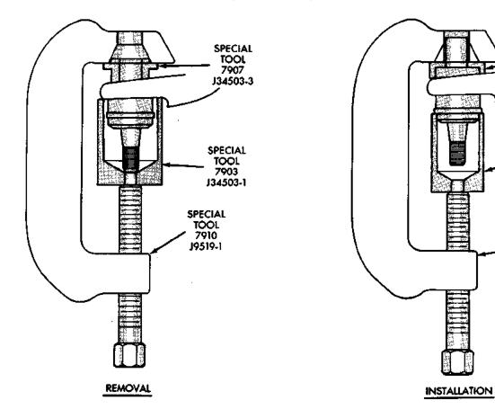
Fig. 7 Lower Ball Stud Remove/Install
