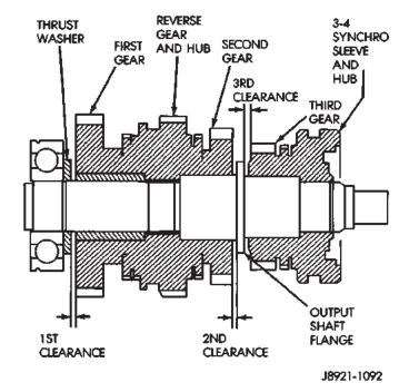
Fig. 112 Check Output Shaft Gear Thrust Clearance
