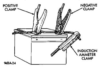
Fig. 1 Volts-Amps Tester Connections - Typical
