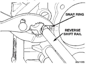
Fig. 82 Install Reverse Snap-ring
