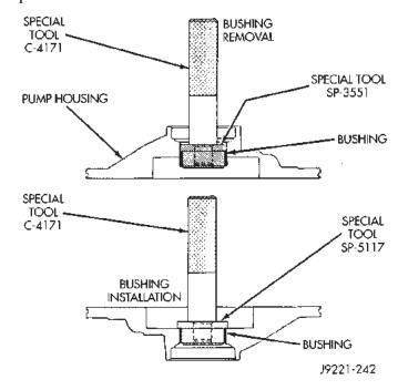
Fig. 123 Removing Oil Pump Bushing
