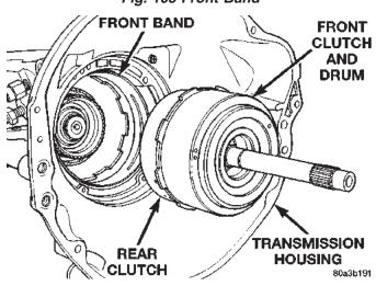
Fig. 104 Installing Front/Rear Clutch
