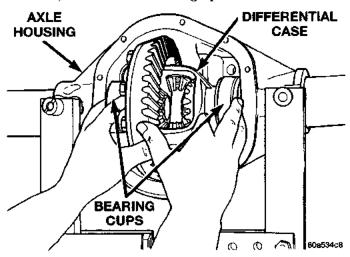
Fig. 25 Differential Case and Side Bearings
