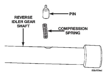
Fig. 89 Install Compression Spring And Pin
