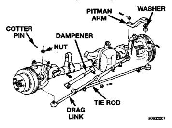
Fig. 1 Steering Linkage
