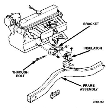
Fig. 19 Left Front Engine Mount
