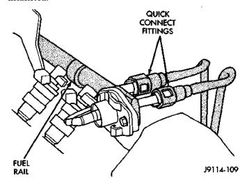
Fig. 23 Fuel Line Quick-Connect Couplings
