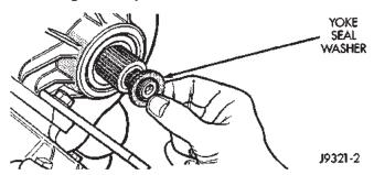
Fig. 76 Yoke Seal Washer Installation
