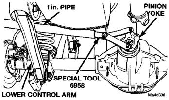
Fig. 33 Pinion Yoke Holder
