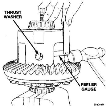
Fig. 60 Remove Pinion Thrust Washer—Shown With 6963-A Holder
