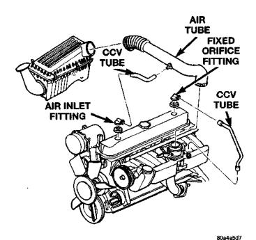
Fig. 5 CCV System-4.0L Engine
