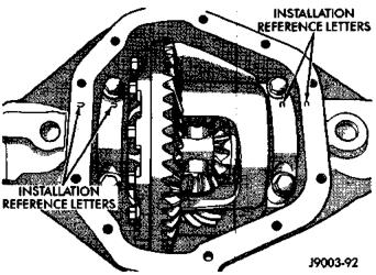
Fig. 21 Bearing Cap Identification
