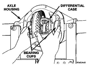
Fig. 19 Differential Case and Side Bearings
