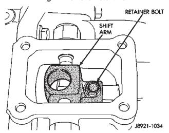
Fig. 23 Shift Arm Retainer Bolt Removal
