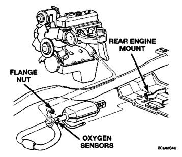
Fig. 3 Exhaust Pipe with Catalytic Converter 2.5 L Engine
