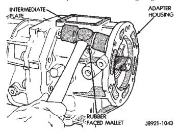
Fig. 28 Loosen Adapter/Extension Housing
