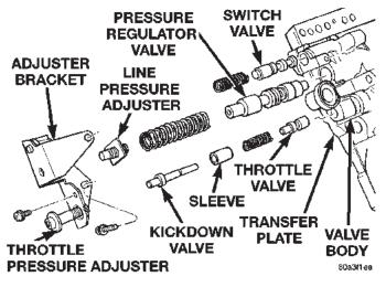
Fig. 40 Adjusting Screw Bracket, Springs, Valve Removal
