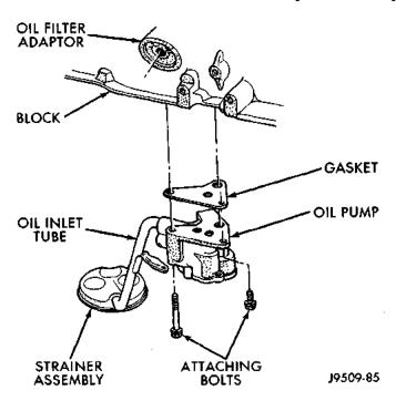
Fig. 41 Oil Pump Assembly
