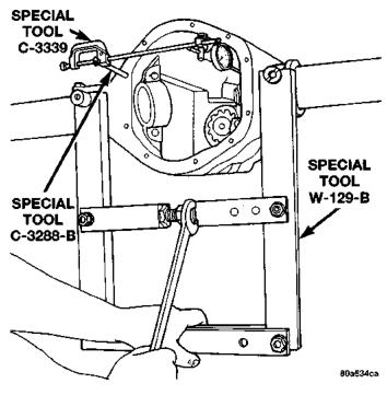
Fig. 26 Spread Axle Housing
