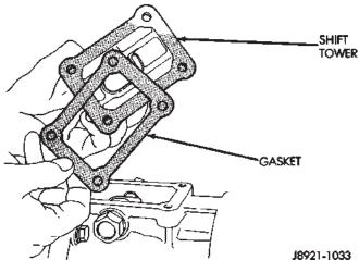
Fig. 17 Remove Shift Tower Gasket
