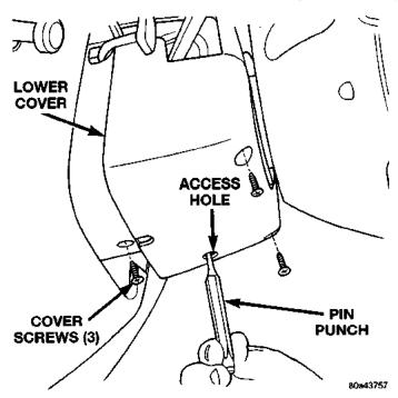
Fig. 52 Key Cylinder and Cover Removal
