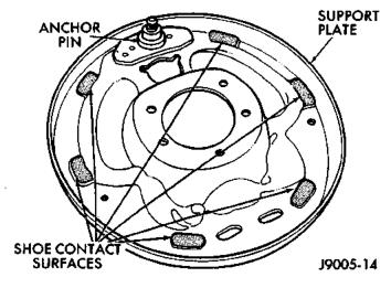
Fig. 34 Shoe Contact Surfaces
