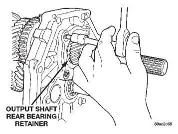
Fig. 58 Remove Output Shaft Rear Bearing Retainer
