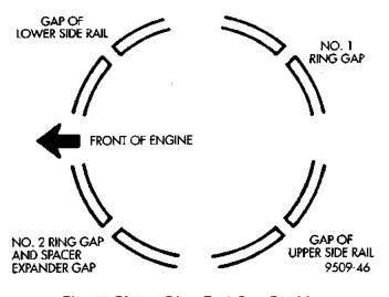
Fig. 10 Piston Ring End Gap Position
