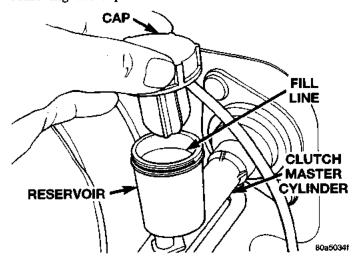
Fig. 3 Clutch Master Cylinder Reservoir And Cap FLYWHEEL
