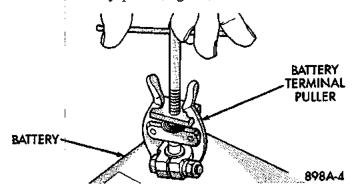
Fig. 10 Remove Battery Terminal Clamp - Typical
