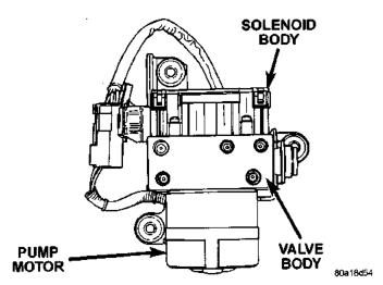
Fig. 3 Hydraulic Controller Unit
