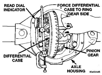
Fig. 61 Hold Differential Case and Read Dial Indicator
