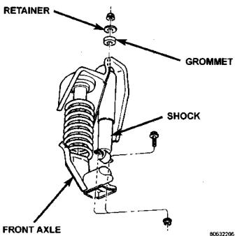
Fig. 1 Coil Spring & Shock Absorber
