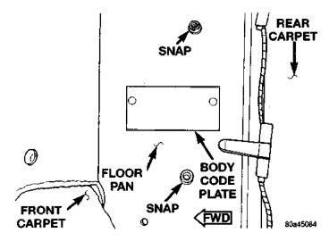
Fig. 2 Body Code Plate Location
