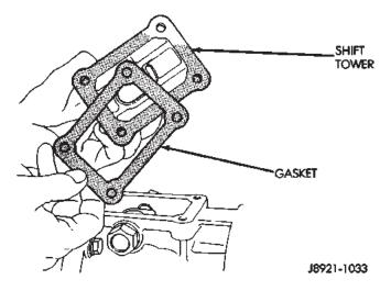
Fig. 18 Remove Shift Tower Gasket
