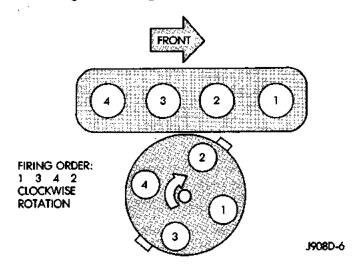
Fig. 32 Engine Firing Order—2.5L 4-Cylinder Engine
