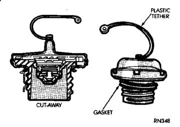
Fig. 3 Fuel Tank Filler Tube Cap—Typical
