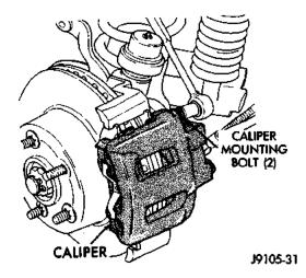
Fig. 25 Caliper Mounting Bolts
