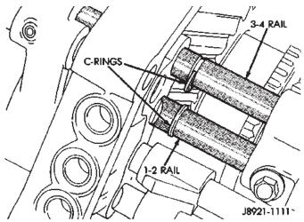
Fig. 91 Install Shift Rail C-rings
