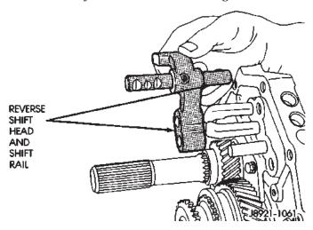
Fig. 55 Remove Reverse Shift Head Assembly
