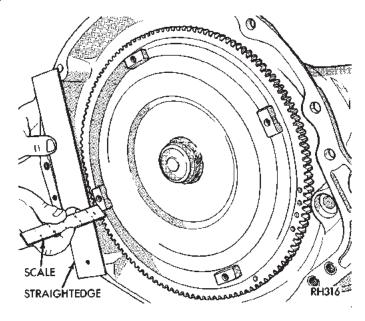
Fig. 18 Typical Method Of Checking Converter Seating
