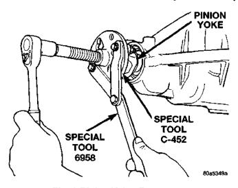
Fig. 9 Pinion Yoke, Remove
