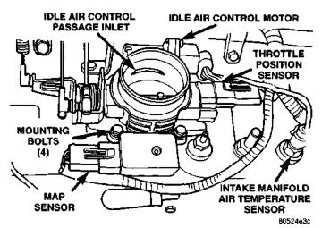
Fig. 18 Sensor Locations-4.0L Engine Shown
