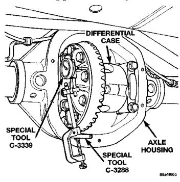
Fig. 57 Differential Side play Measurement
