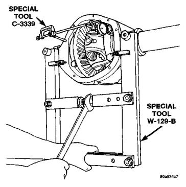
Fig. 24 Spread Axie Housing
