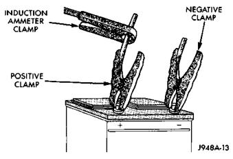
Fig. 6 Volt-Ammeter-Load Tester Connections
