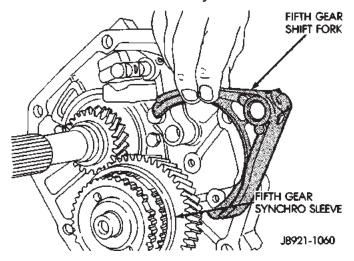
Fig. 102 Install Fifth Gear Shift Fork
