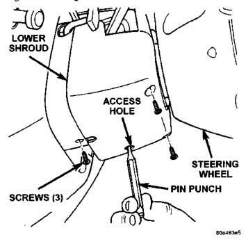
Fig. 4 Steering Column Shrouds Remove/Install
