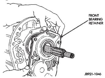
Fig. 36 Install Front Bearing Retainer
