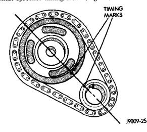
Fig. 43 Timing Chain Alignment
