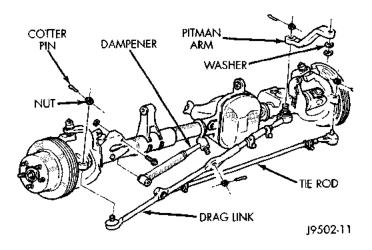
Fig. 3 Steering Linkage
