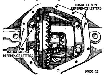
Fig. 21 Differential Bearing Cap Reference Letters
