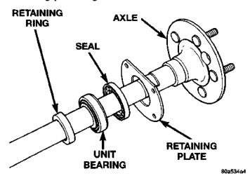
Fig. 18 Axle Bearing and Seal Components
