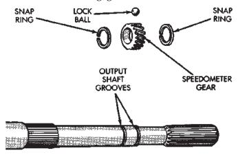
38921-1119 Fig. 37 Speedometer Drive Gear Assembly
