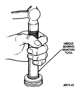
Fig. 11 Needle Bearing Removal
