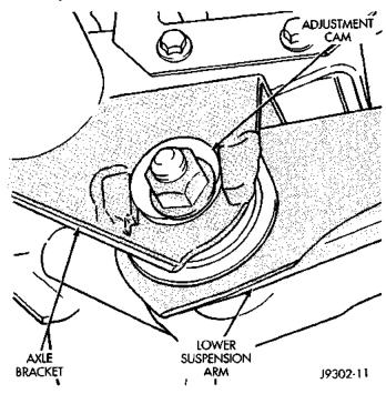
Fig. 37 Angle Adjustment With Cams-Typical
