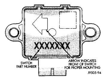
Fig. 15 Acceleration Switch Position Indicator
