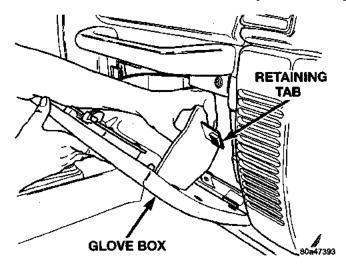
Fig. 12 Glove Box Remove/Install
