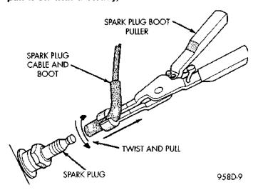
Fig. 31 Cable Removal
