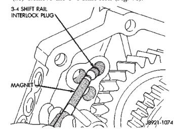
Fig. 72 Remove 3-4 Shift Rail Interlock Plug
