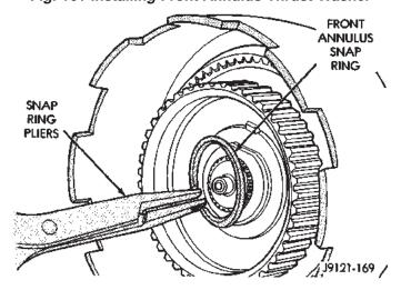
Fig. 162 Installing Front Annulus Snap Ring
