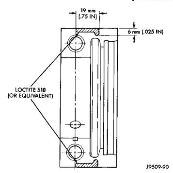
Fig. 48 Location of Loctite 518 (or equivalent)
