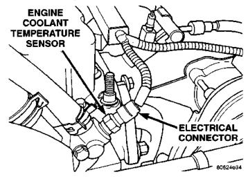
Fig. 44 Engine Coolant Temperature Sensor— Typical
