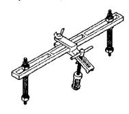
Valve Spring Compressor Tool MD-998772A
