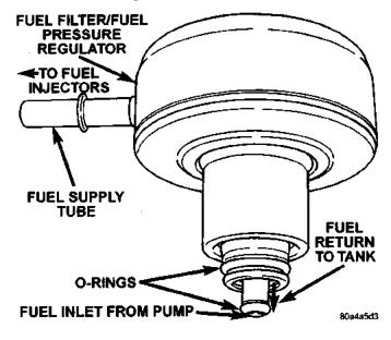
Fig. 3 Fuel Filter/Fuel Pressure Regulator
