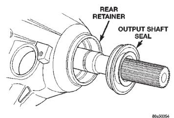
Fig. 10 Rear Retainer Seal
