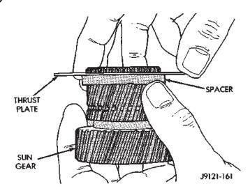
Fig. 153 Installing Driving Shell Front Thrust Plate
