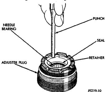
Fig. 12 Install Retainer
