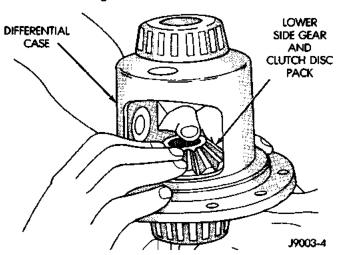
Fig. 59 Clutch Discs and Ring Gear Side Gear installation
