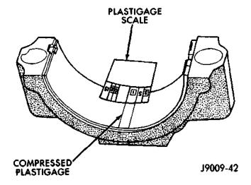
Fig. 15 Measuring Bearing Clearance with Plastigage
