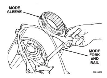
Fig. 24 Mode Fork And Sleeve Removal
