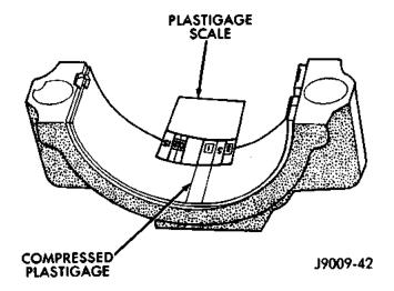
Fig. 15 Measuring Bearing Clearance with Plastigage
