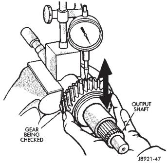
Fig. 122 Check Gear-To-Shaft Oil Clearance
