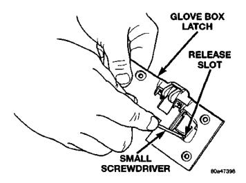
Fig. 13 Glove Box Lock Cylinder Remove/Install
