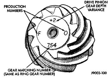
Fig. 47 Pinion Gear ID Numbers
