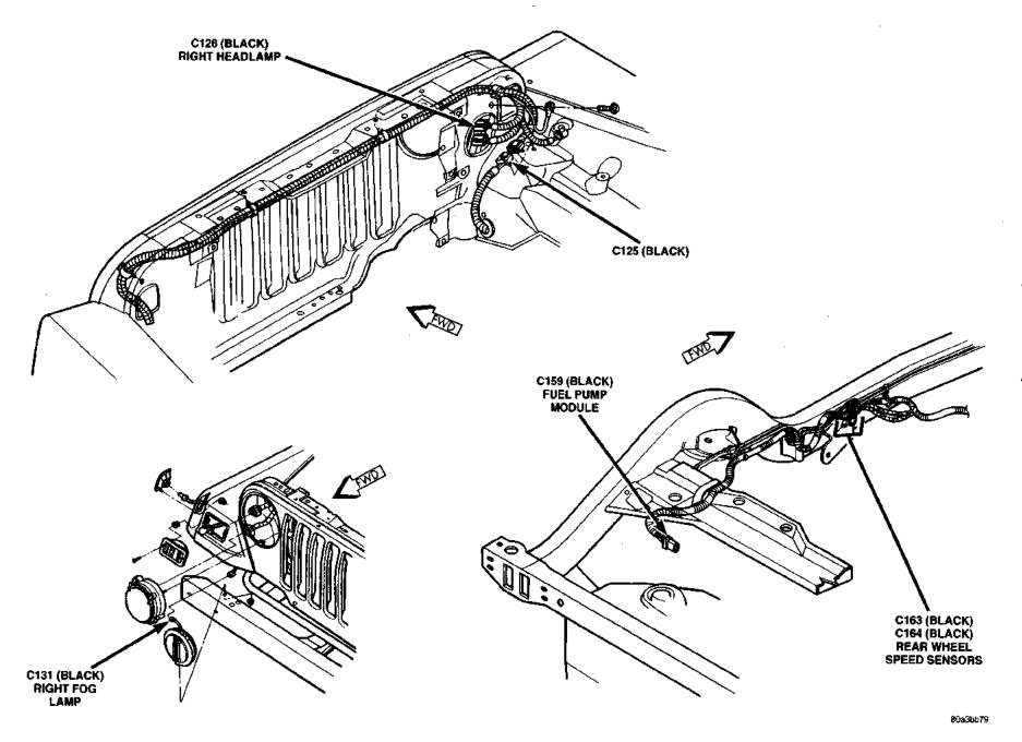
Fig. 1 Front End Wiring Connectors
