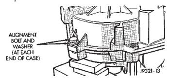
Fig. 73 Alignment Bolt Location
