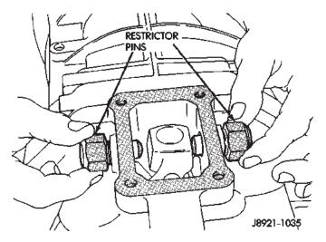
Fig. 24 Shift Arm Rstrictor Pins
