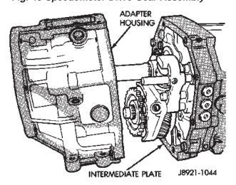
Fig. 41 Install Adapter/Extension Housing
