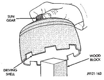
Fig. 155 Supporting Sun Gear On Wood Block
