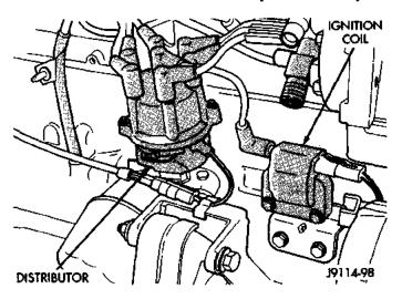
Fig. 16 Ignition Coil—Typical (4.0L Engine Shown)
