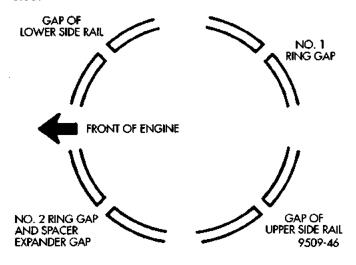
Fig. 10 Piston Ring End Gap Position
