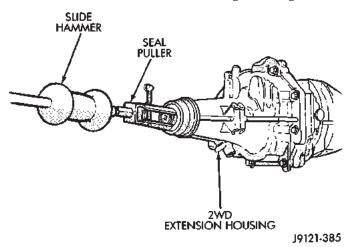
Fig. 13 Remove Extension Housing Seal
