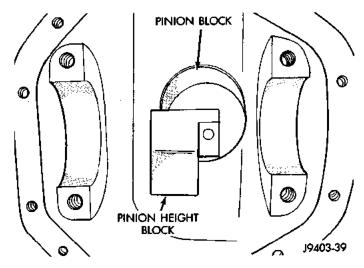
Fig. 65 Pinion Height Block-Typical
