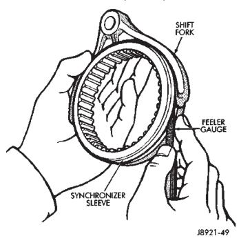
Fig. 128 Check Fork-To-Hub Clearance
