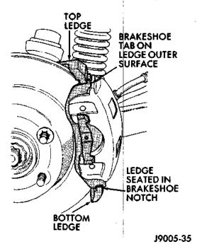
Fig. 30 Caliper Installation
