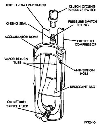
Fig. 2 Accumulator - Typical
