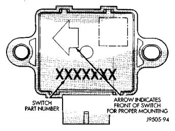
Fig. 5 Acceleration Switch
