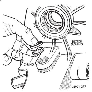
Fig. 60 Sector O-Ring And Bushing Installation
