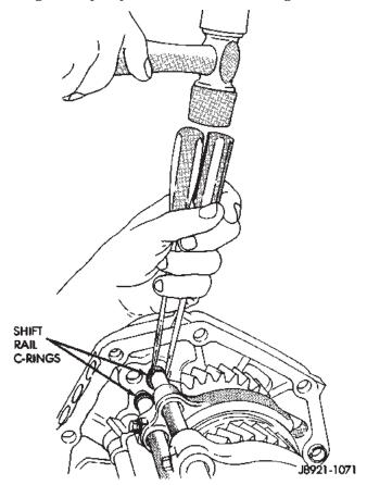
Fig. 69 Remove Shift Rail C-rings
