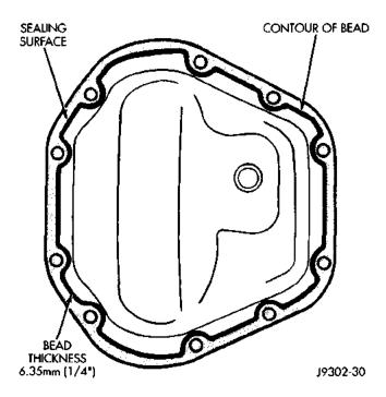
Fig. 47 Typical Housing Cover With Sealant
