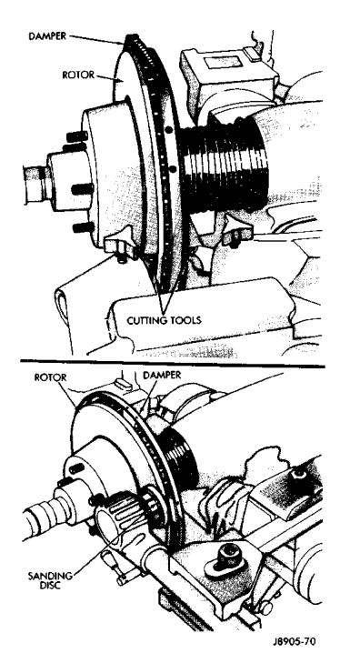
Fig. 15 Rotor Refinishing
