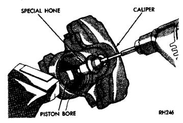
Fig. 56 Lightly Polishing Piston Bore With Tool
