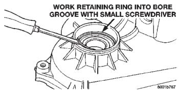
Fig. 44 Installing Output Shaft Front Bearing Retaining Ring
