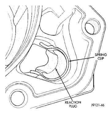
Fig. 168 Park Sprag Reaction Plug And Spring
