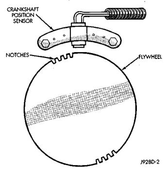
Fig. 6 Sensor Operation—2.5L 4-Cyl. Engine .
