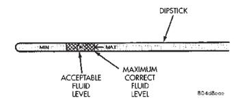
Fig. 13 Dipstick Fluid Level Marks—Typical
