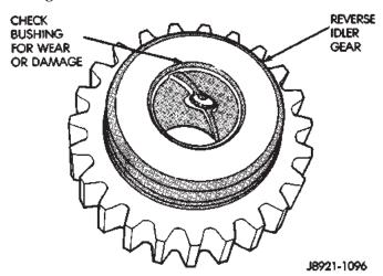
Fig. 129 Reverse Idler Gear Bushing
