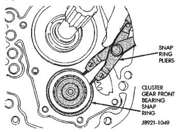
Fig. 33 Remove Cluster Gear Snap-ring
