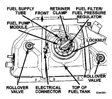
Fig. 8 Rollover Valve Location
