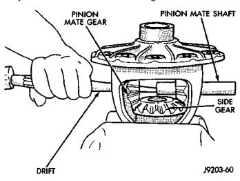
Fig. 56 Mate Shaft Removal
