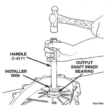
Fig. 47 Output Shaft Rear Bearing Installation
