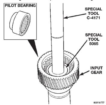
Fig. 52 Install Input Gear Pilot Bearing
