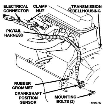
Fig. 5 Crankshaft Position Sensor—Manual Transmission (Typical)
