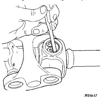
Fig. 35 Seat Snap Rings In Groove
