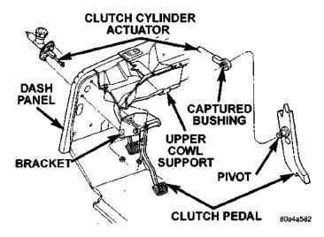
Fig. 11 Clutch Pedal Mounting
