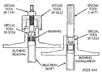
Fig. 125 Replacing Reaction Shaft Support Bushing ASSEMBLY
