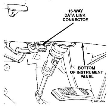
Fig. 1 16-Way Data Link Connector - Typical
