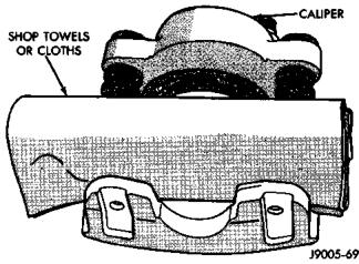
Fig. 45 Padding Caliper Interior
