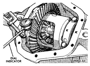
Fig. 62 Ring Gear Backlash Measurement
