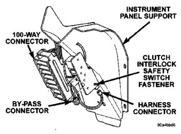
Fig. 1 Clutch Interlock Safety Switch By-Pass
