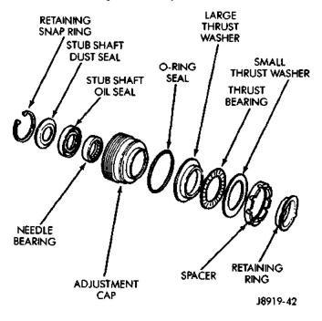
Fig. 10 Adjustment Plug Components
