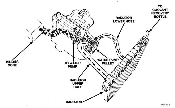
Fig. 1 Coolant Flow—2.5L Engine
