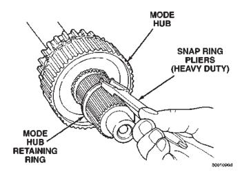
Fig. 28 Mode Hub Retaining Ring Removal
