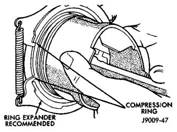
Fig. 9 Compression Ring Installation
