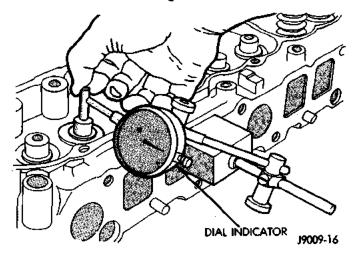
Fig. 56 Measurement of Lateral Movement of Valve Stem
