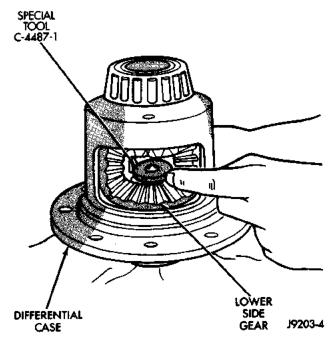
Fig. 57 Step Plate Tool Installation—Shown With 6963-A Holder
