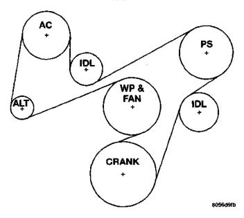
Fig. 35 Vehicles with 2.5L or 4.0L Engine-With A/C
