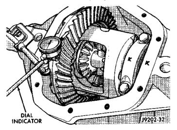
Fig. 77 Ring Gear Backlash Measurement
