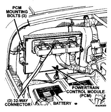
Fig. 14 PCM and Three 32-Way Connectors
