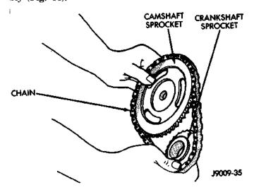
Fig. 44 Camshaft and Crankshaft Sprocket and Chain
