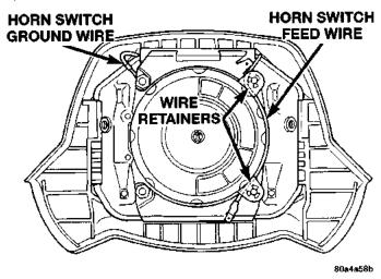
Fig. 6 Horn Switch Wires Remove/Install
