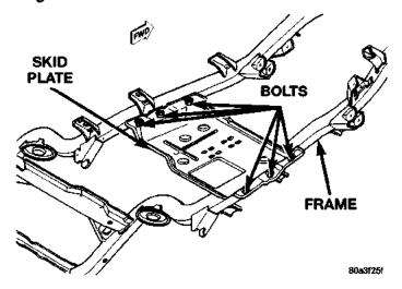
Fig. 6 Transfer Case Skid Plate
