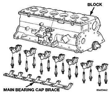
Fig. 42 Main Bearing Caps and Brace.
