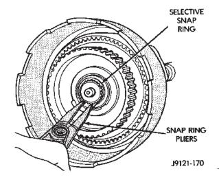
Fig. 163 Installing Planetary Selective Snap Ring
