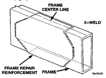
Fig. 2 Frame Reinforcement
