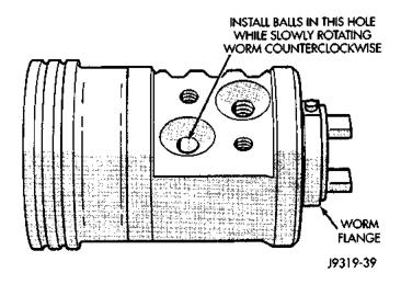
Fig. 22 Installing Balls in Rack Piston
