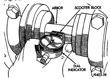
Fig. 72 Pinion Gear Depth Measurement—Typical
