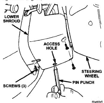
Fig. 18 Steering Column Shrouds Remove/Install
