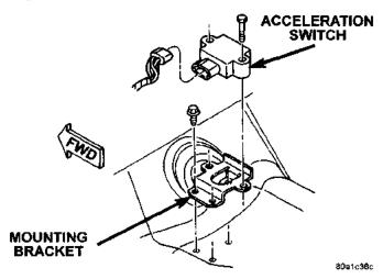
Fig. 14 Acceleration Switch
