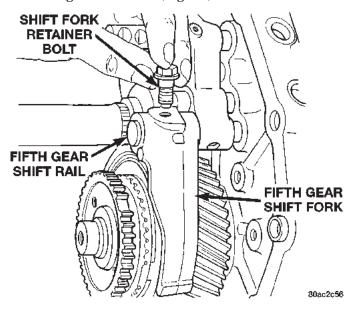
Fig. 95 Install Fifth Gear Retainer Bolt
