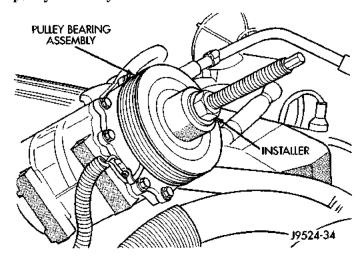
Fig. 19 Clutch Pulley Install
