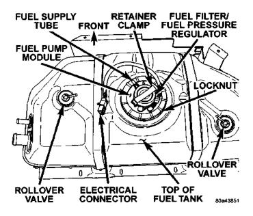
Fig. 1 Rollover Valve Location
