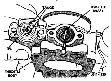
Fig. 36 Throttle Position Sensor—Installation
