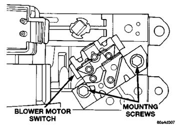
Fig. 30 Blower Motor Switch Remove/Install
