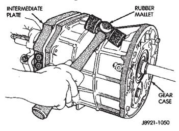
Fig. 34 Separate Intermediate Plate and Transmission Case
