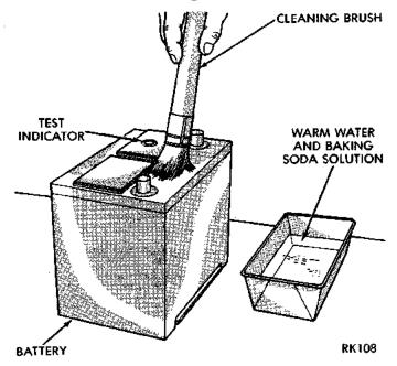
Fig. 14 Clean Battery - Typical
