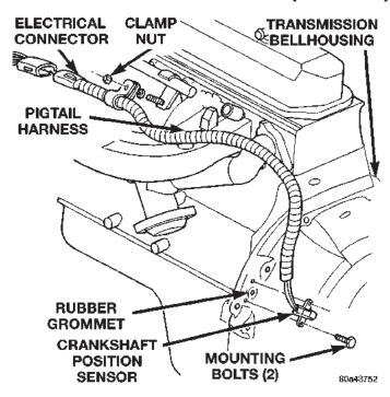
Fig. 7 Crankshaft Position Sensor —4.0L Engine
