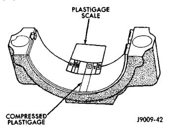
Fig. 18 Measuring Bearing Clearance with Plastigage
