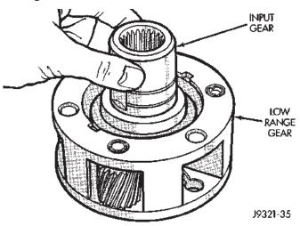
Fig. 38 Input Gear Removal
