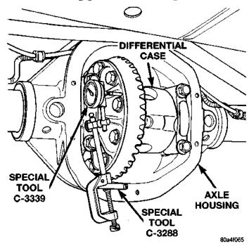
Fig. 78 Differential Side play Measurement
