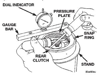
Fig. 143 Checking Rear Clutch Pack Clearance
