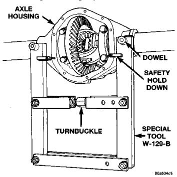
Fig. 16 Install Axle Housing Spreader
