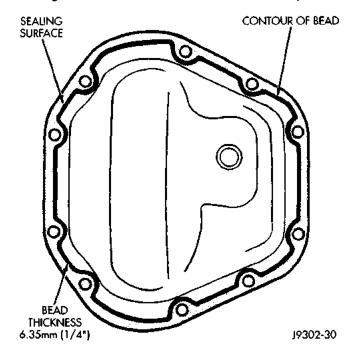
Fig. 41 Typical Housing Cover With Sealant
