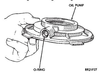
Fig. 71 Pickup Tube O-Ring Position
