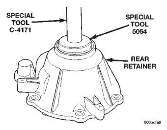
Fig. 55 Installing Rear Bearing In Retainer
