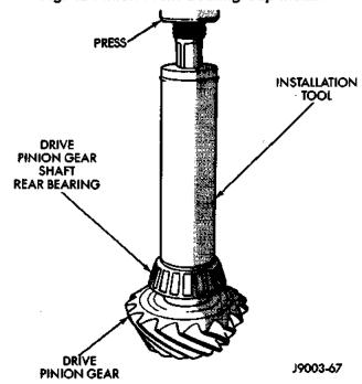
Fig. 43 Inner Pinion Bearing Cone Install
