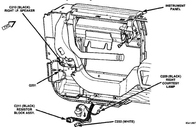
Fig. 17 Instrument Panel Connectors — Right Side
