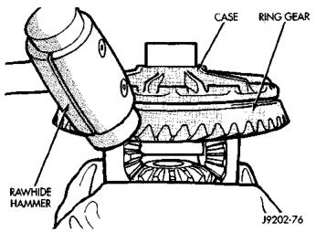
Fig. 31 Ring Gear Removal
