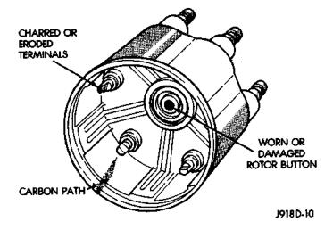
Fig. 17 Cap Inspection—Internal—Typical
