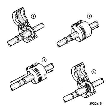
Fig. 10 Spring Lock Coupling Disconnect
