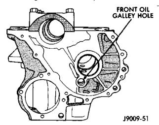
Fig. 64 Front Oil Galley Hole
