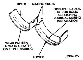
Fig. 11 Connecting Rod Bearing Inspection
