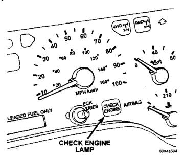
Fig. 12 Check Engine Lamp—Typical
