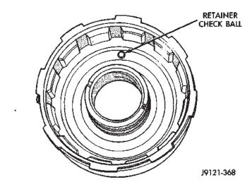
Fig. 173 Front Clutch Piston Retainer Check Ball Location
