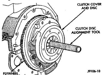
Fig. 5 Typical Method Of Aligning Clutch Disc
