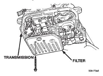
Fig. 15 Transmission Filter
