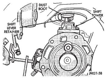
Fig. 9 Removing/Installing Shift Lever
