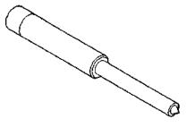
Remover/Installer Steering Rack Piston C-4175
