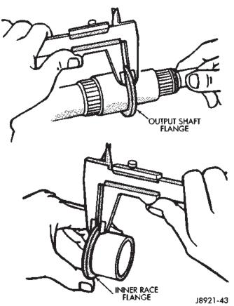
Fig. 119 Check Shaft And Bearing Race Flange Thickness
