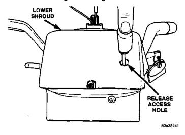
Fig. 2 Key Cylinder Release Access Hole
