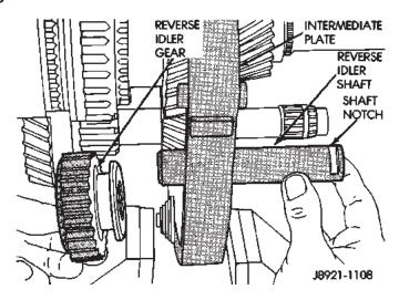
Fig. 92 Install Reverse Idler Gear And Shaft
