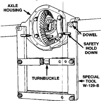
Fig. 22 Install Axle Housing Spreader
