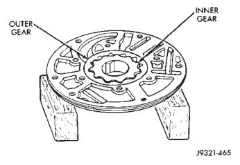
Fig. 127 Pump Inner Gear Installation
