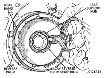
Fig. 95 Low-Reverse Drum Snap Ring
