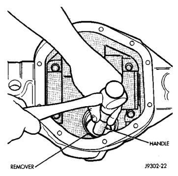
Fig. 34 Outer Bearing Cup Removal
