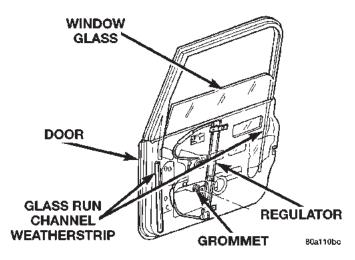
Fig. 31 Full Door Glass Run Channel Weatherstrip INSTALLATION
