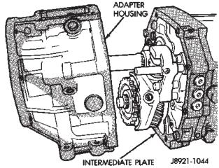
Fig. 38 Install Adapter/Extension Housing-Typical
