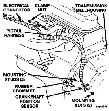
Fig. 4 Crankshaft Position Sensor—2.5L 4-Cyl. Engine—Auto. Trans.
