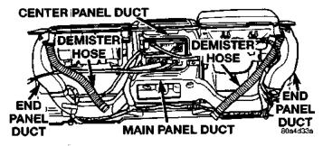
Heater-A/C Ducts and Outlets Remove/install
