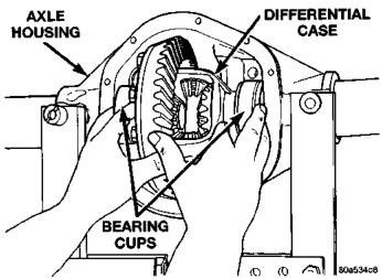
Fig. 22 Differential Case and Side Bearings
