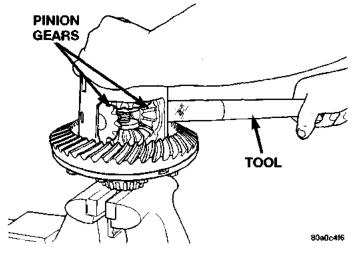
Fig. 61 Pinion Gear Removal—Shown With 6963-A Holder
