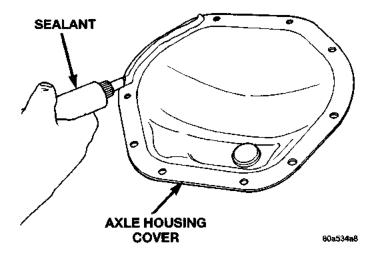
Fig. 6 Apply Sealant
