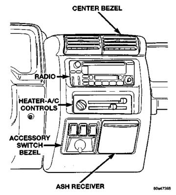
Fig. 4 Center Bezel Remove/Install
