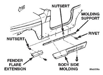
Fig. 14 Body Side Molding
