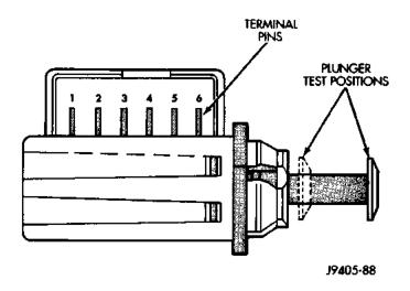
Fig. 7 Stop Lamp Switch Terminal Identification
