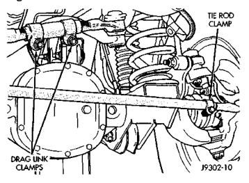
Fig. 2 Drag Link and Tie Rod Clamp
