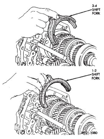
Fig. 73 Remove Shift Forks
