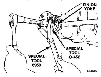
Fig. 31 Pinion Yoke Removal
