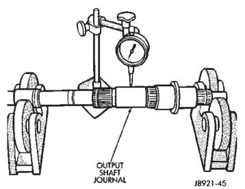
Fig. 120 Check Output Shaft Runout
