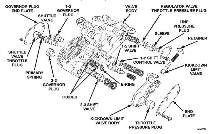
Fig. 53 Control Valves, Shift Valves, And Governor Plugs
