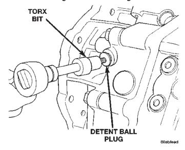
Fig. 19 Remove Detent Ball Plug
