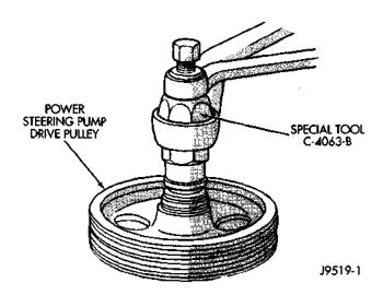
Fig. 6 Pulley Installation
