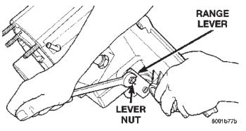
Fig. 62 Range Lever Installation
