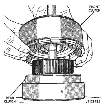
Fig. 76 Separating Front Clutch From Rear Clutch
