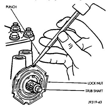
Fig. 27 Loosening the Adjuster Plug
