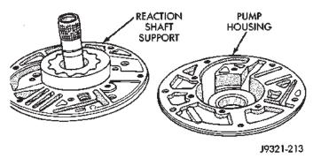
Fig. 120 Separating Pump Housing From Reaction Shaft Support
