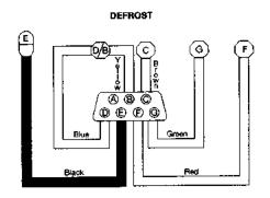
Fig. 9 Vacuum Circuits - Heater-A/C
