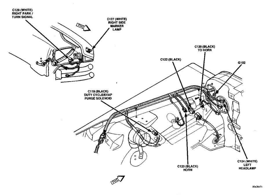
Fig. 4 Engine Compartment Connectors — Right Side
