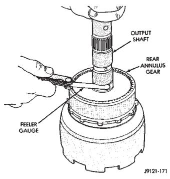
Fig. 164 Checking Planetary Geartrain End Play
