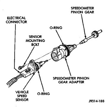
Fig. 47 Sensor Removal/Installation
