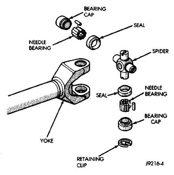
Fig. 2 Single Cardan Universal Joint
