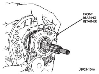
Fig. 39 Install Front Bearing Retainer
