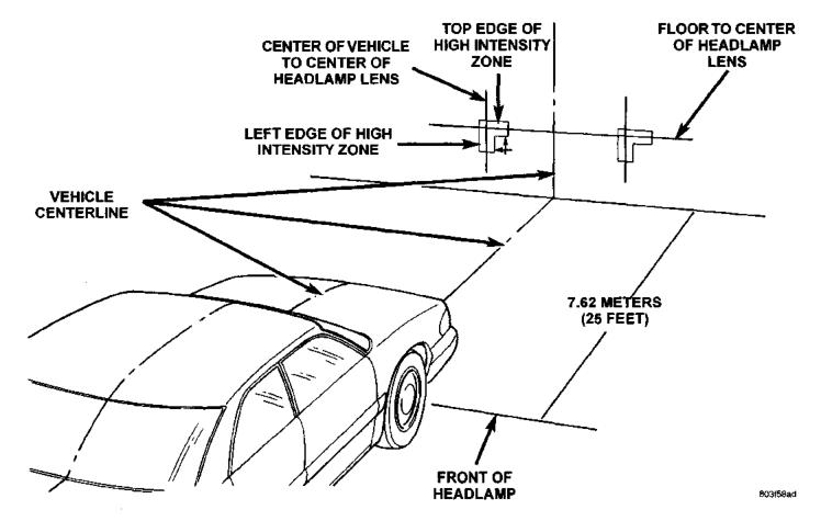
Fig. 1 Headlamp Alignment Screen-Typical
