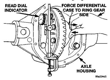
Fig. 59 Hold Differential Case and Read Dial Indicator
