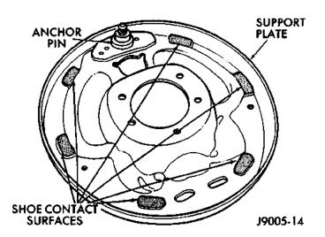
Fig. 57 Shoe Contact Surfaces
