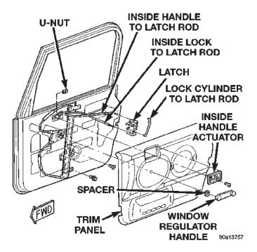
Fig. 22 Latch Rods
