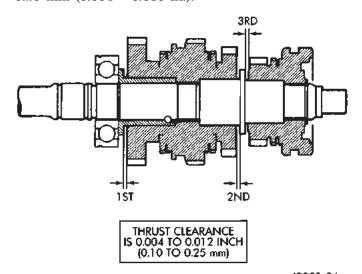
J8921-36 Fig. 101 Check Output Shaft Gear Thrust Clearance
