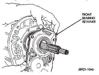
Fig. 31 Remove Front Bearing Retainer
