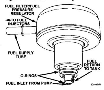
Fig. 13 Fuel Filter/Fuel Pressure Regulator O-Rings o-rings. Do not install o-rings separately into fuel pump module. They will be damaged when installing filter/regulator.
