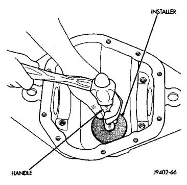
Fig. 39 Pinion Inner Bearing Cup Install
