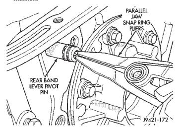
Fig. 90 Rear Band Servo Lever Pin
