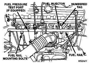
Fig. 19 Fuel Rail Mounting—Typical
