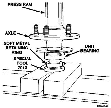
Fig. 20 Press Bearing Retaining Ring On Axle
