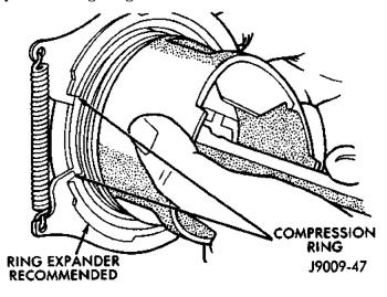
Fig. 9 Compression Ring Installation
