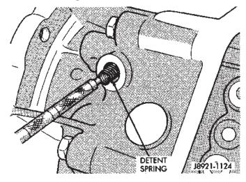
Fig. 48 Install Detent Spring
