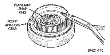
Fig. 146 Front Planetary Snap Ring Removal
