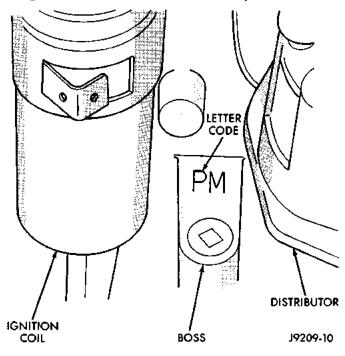
Fig. 4 Oversize and Undersize Component Code Location
