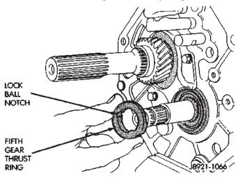
Fig. 96 Install Fifth Gear Thrust Ring
