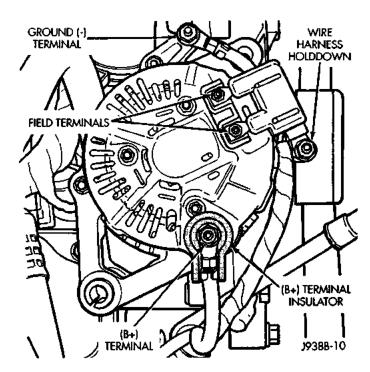
Fig. 3 Remove/Install Generator Connectors— Typical
