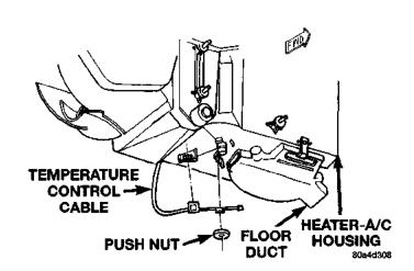
Fig. 31 Temperature Control Cable Remove/Install
