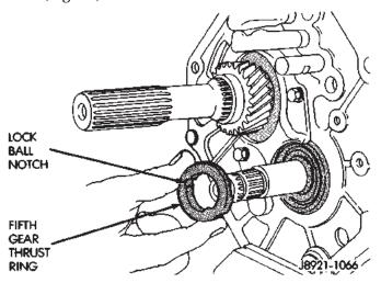
Fig. 59 Remove Fifth Gear Thrust Ring
