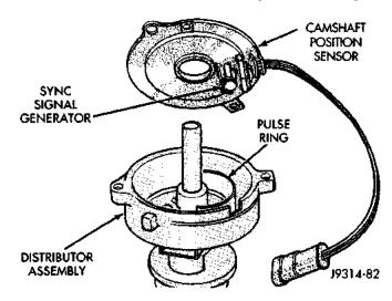
Fig. 23 Camshaft Position Sensor—Typical
