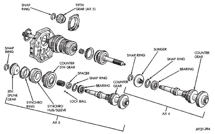
Fig. 4 Geartrain Components
