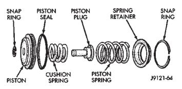
Fig. 117 Rear Servo Components
