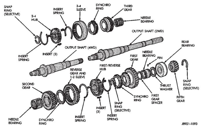
Fig. 5 Output Shaft and Gears
