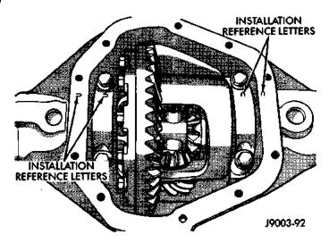
Fig. 24 Differential Bearing Cap Reference Letters
