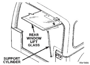
Fig. 75 Support Rod Cylinder Removal
