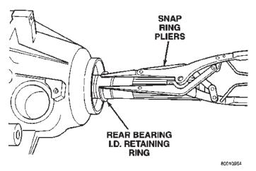
Fig. 11 Output Shaft Rear Bearing Retaining Ring
