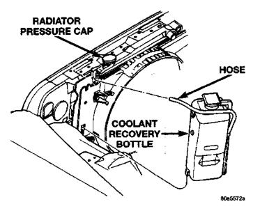
Fig. 4 Coolant Recovery Bottle
