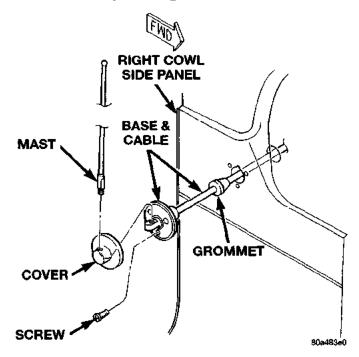
Fig. 9 Antenna Remove/Install
