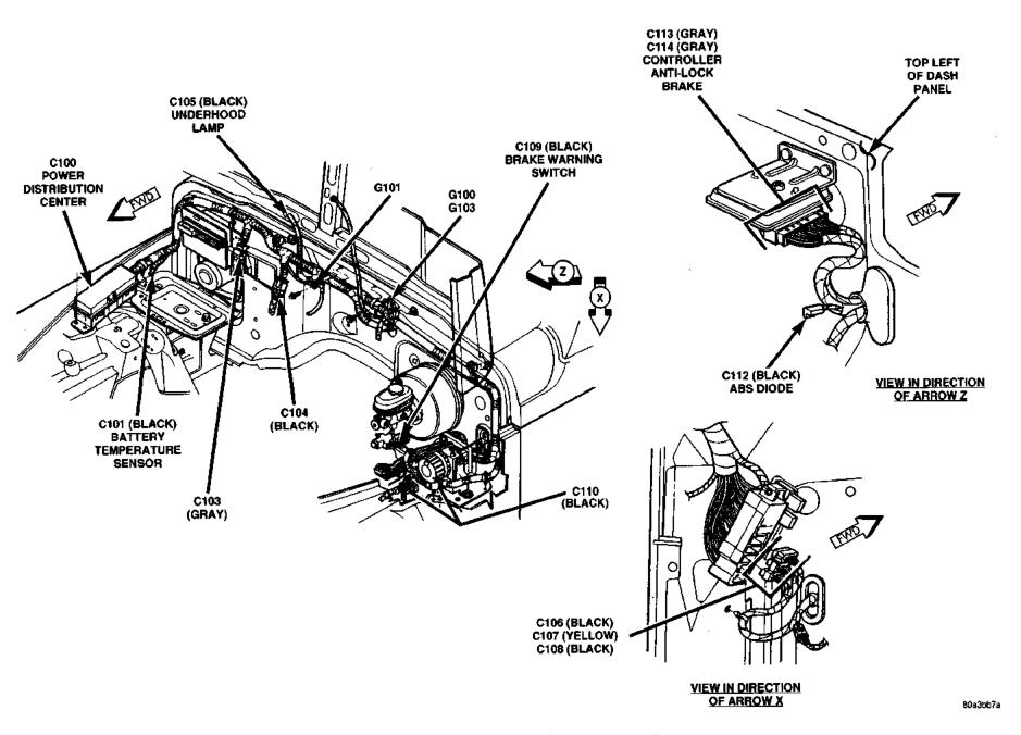
Fig. 2 Engine Compartment Connectors — Rear
