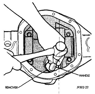
Fig. 37 Front Bearing Cup Removal
