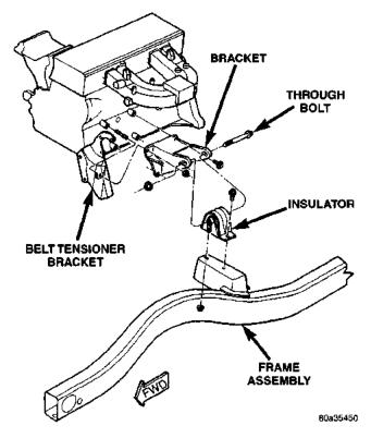
Fig. 19 Left Front Mount-2.5L Engine
