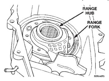
Fig. 63 Install Range Fork And Hub Assembly
