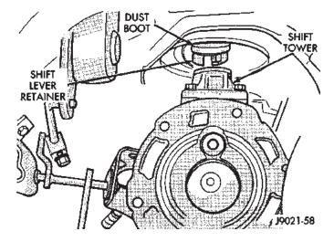
Fig. 8 Removing/Installing Shift Lever
