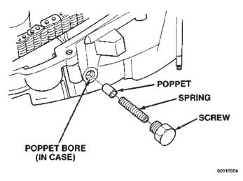
Fig. 67 Shift Detent Components
