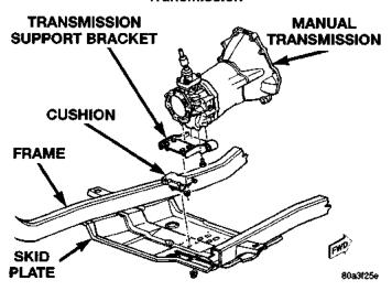
Fig. 5 Transmission Mount—Manual Transmission
