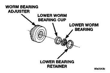
Fig. 15 Lower Bearing Cup
