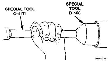
Fig. 11 Pinion Seal Installation
