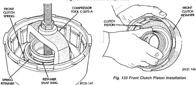
Fig. 132 Compressing Front Clutch Piston Spring
