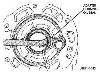
Fig. 15 Remove Adapter Housing Seal
