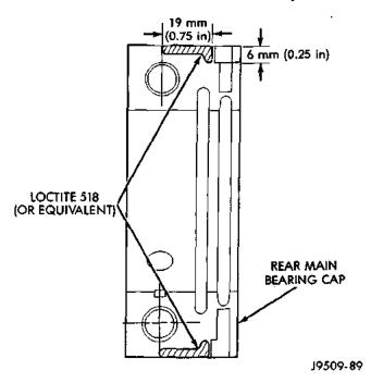
Fig. 51 Location of Loctite 518 (or equivalent)
