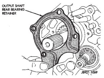
Fig. 62 Remove Output Shaft Rear Bearing Retainer
