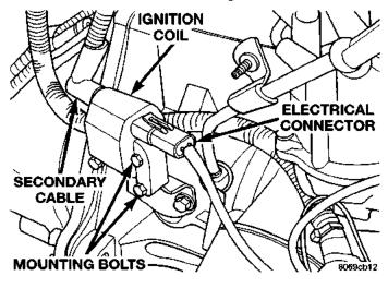
Fig. 35 Ignition Coil—2.5L Engine
