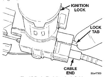
Fig. 25 Brake/Park Interlock Cable
