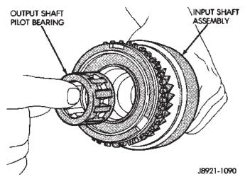
Fig. 111 Remove Output Shaft Pilot Bearing
