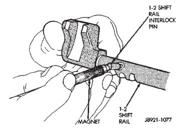
Fig. 75 Remove 1-2 Shift Rail Interlock Pin
