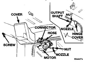
Fig. 12 Rear Wiper and Washer System
