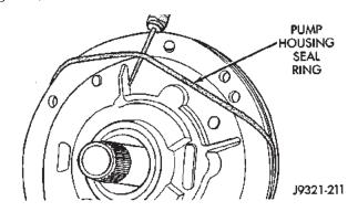
Fig. 118 Removing Pump Seal Ring
