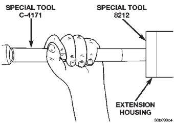
Fig. 13 Install Extension Housing Seal
