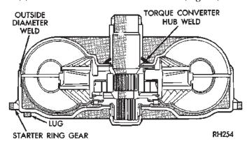
Fig. 12 Converter Leak Points—Typical
