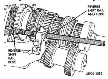
Fig. 78 Remove Reverse Shift Rail
