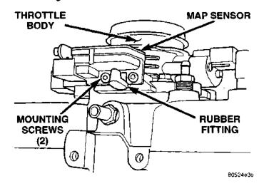
Fig. 26 Rubber L-Shaped Fitting—MAP Sensor-to-Throttle Body
