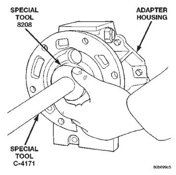
Fig. 16 Install Adapter Housing Seal
