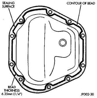
Fig. 50 Typical Housing Cover With Sealant
