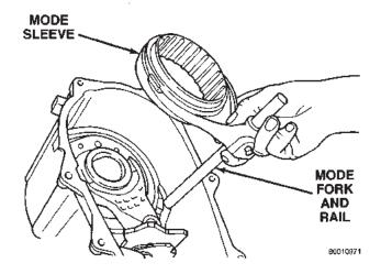
Fig. 65 Assembling Mode Fork And Sleeve
