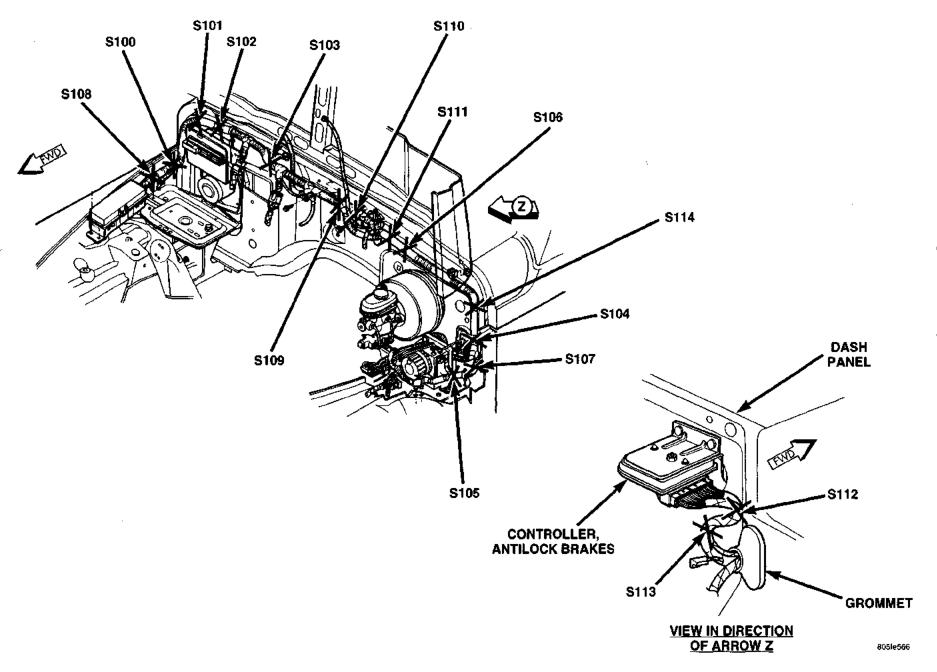
Fig. 2 Engine Compartment Splices—Rear
