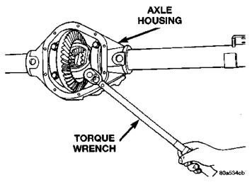
Fig. 25 Tighten Differential Bearing Cap Bolts
