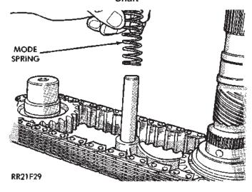
Fig. 69 Install Mode Fork Spring
