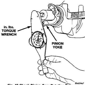
Fig. 49 Check Pinion Gear Rotation Torque
