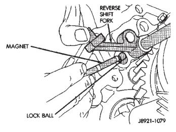
Fig. 94 Install Fifth Gear Shift Rail Lock Ball
