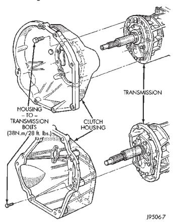
Fig. 19 Clutch Housing
