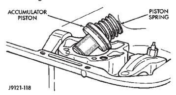
Fig. 71 Accumulator Piston And Spring
