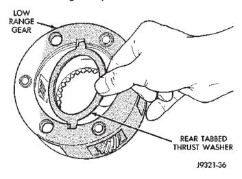
Fig. 39 Rear Tabbed Thrust Washer Removal
