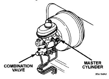
Fig. 19 Combination Valve/Master Cylinder
