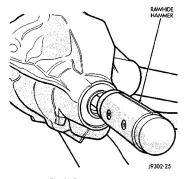
Fig. 35 Remove Pinion Gear
