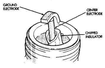
Fig. 28 Chipped Electrode Insulator
