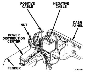
Fig. 16 Battery Cables
