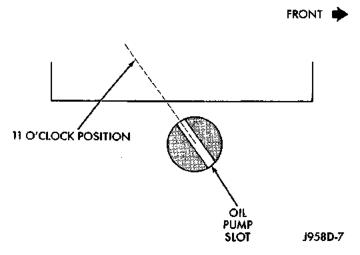
Fig. 46 Slot At 11 O'clock Position—4.0L Engine
