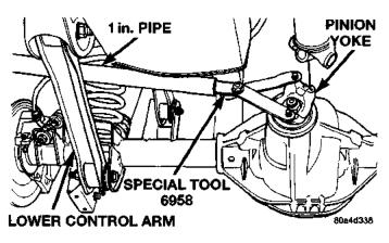
Fig. 26 Pinion Yoke Holder
