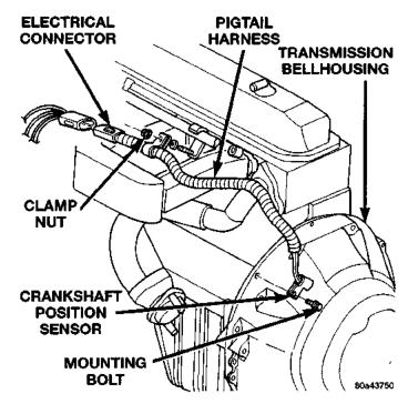
Fig. 3 Crankshaft Position Sensor—4.0L 6-Cyl. Engine—Auto. Trans.
