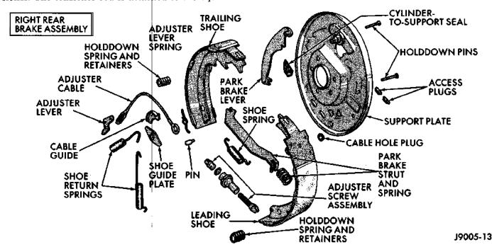
Fig. 5 Brake Components
