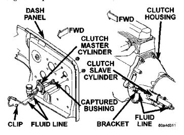
Fig. 9 Slave Cylinder and Left Hand Drive Clutch Master Cylinder
