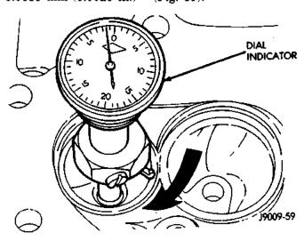
Fig. 59 Measurement of Valve Seat Runout
