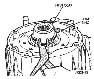
Fig. 58 Install Snap-Ring
