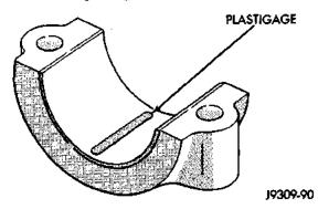
Fig. 2 Placement of Plastigage in Bearing Shell
