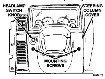
Fig. 2 Steering Column Cover Remove/Install
