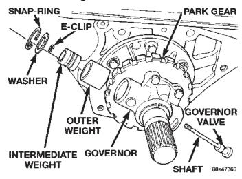
Fig. 36 Snap Ring, Washer, and Outer Weight
