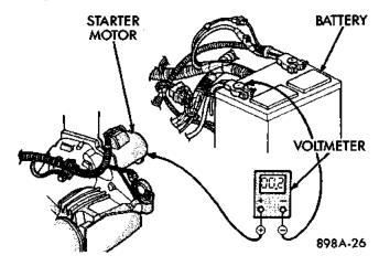
Fig. 6 Test Starter Ground - Typical
