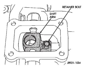
Fig. 44 Install Shift Arm Retainer Bolt
