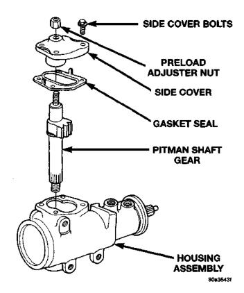
Fig. 4 Side Cover and Pitman Shaft
