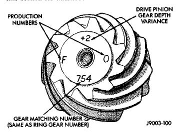
Fig. 62 Pinion Gear ID Numbers
