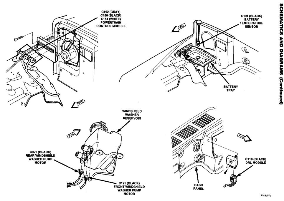
Fig. 3 Engine Compartment Connectors
