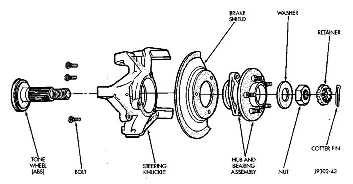
Fig. 4 Hub, Knuckle and Axle Shaft
