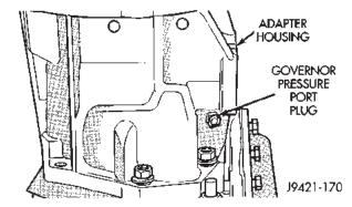
Fig. 8 Pressure Test Ports At Rear Of Case—4WD
