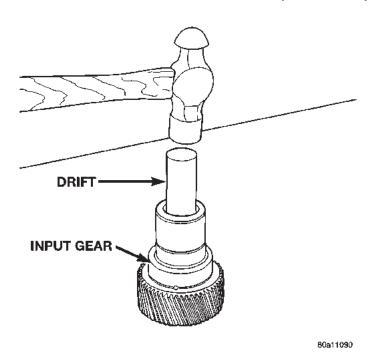
Fig. 51 Remove Input Gear Pilot Bearing
