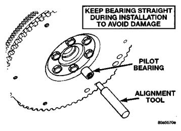
Fig. 7 Pilot Bearing Installation
