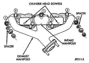
Fig. 8 Intake/Exhaust Manifold 2.5L Engine
