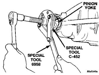
Fig. 34 Pinion Yoke Removal
