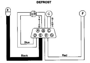
Fig. 8 Vacuum Circuits - Heater Only
