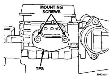
Fig. 35 TPS Mounting Screws
