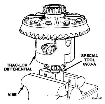
Fig. 54 Differential Case Holding Tool
