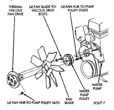
Fig. 23 Fan Mounting Nuts
