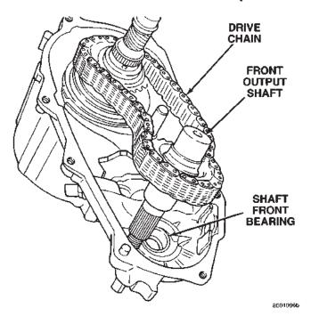
Fig. 22 Remove Front Output Shaft And Chain
