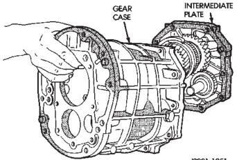
Fig. 32 Remove Intermediate Plate from
