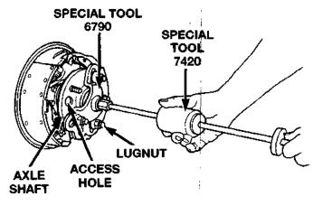
Fig. 14 Axle Shaft, Remove
