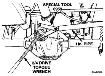
Fla. 39 Tightening Pinion Nut
