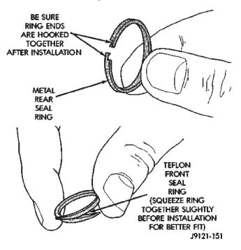
Fig. 140 Input Shaft Seal Ring Identification
