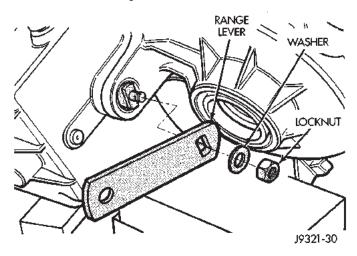
Fig. 74 Range Lever Installation
