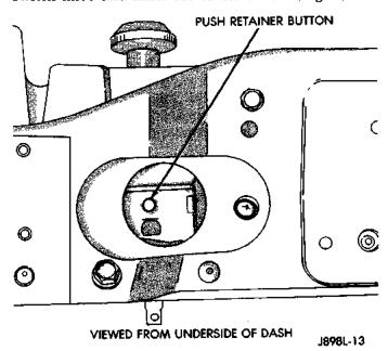
Fig. 4 Headlamp Switch Knob and Shaft Remove/ Install - Typical
