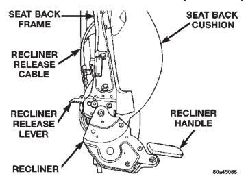
Fig. 4 Recliner Release Cable
