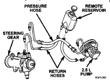
Fig. 2 Power Steering Gear & Pump—2.5L
