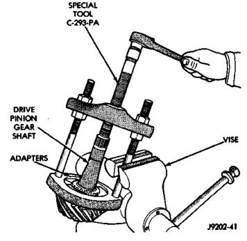
Fig. 37 Inner Bearing Removal
