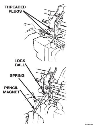
Fig. 66 Remove Lock Ball And Spring
