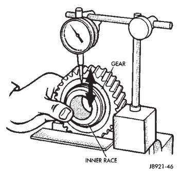
Fig. 121 Check Gear-To-Race Clearance
