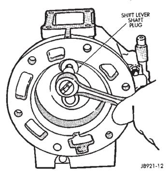
Fig. 25 Removing Shift Lever Shaft Plug
