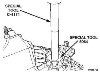
Fig. 43 Front Output Shaft Bearing Installation
