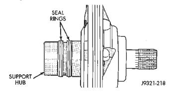
Fig. 128 Hub Seal Ring Position
