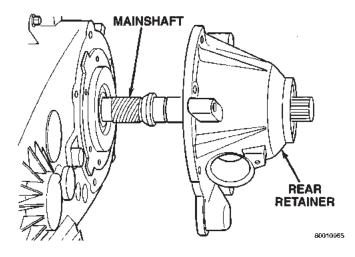
Fig. 12 Rear Retainer Removal
