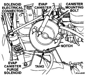
Fig. 2 EVAP Canister and Canister Purge Solenoid
