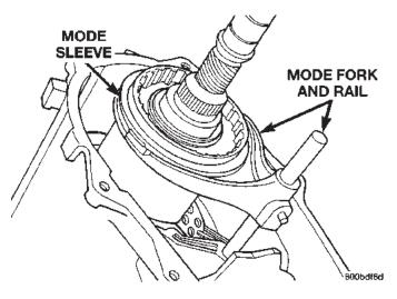
Fig. 66 Mode Fork And Sleeve Installation
