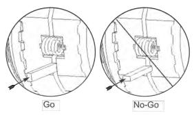
**32.** Check the gap between drivers using check block. The narrow side of the block should fit inbetween drivers, but the wider side should not fit.
