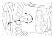
**37.** Insert retaining bolt/roll-pin into case/shaft.
