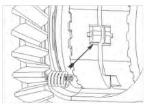
**27.** Compress inner spring and install spring assembly into spring slot.
