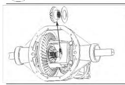
**10.** Remove passenger-side side gear and thrust washer.
