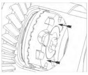
**20.** Verify spacer paddle is aligned with paddle opening in synchro ring and press driver/spacer down onto coupler. Driver teeth should be fully engaged all the way around.
