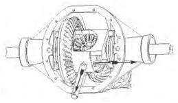
**8.** Remove the axle retaining bolts for the passenger side axle shaft located on the inside of the brake backing plate. Pull out passenger side axle shaft 2"-3".
