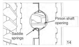
**34.** Keeping both drivers fully engaged, rotate both wheels back 1/4 turn to expose pinion shaft opening. Make sure saddle springs are all fully seated.
