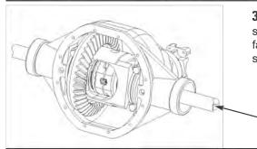
**33.** Push passenger side axle shaft inward through coupler as far as it will go and bolt axle shaft back to housing.
