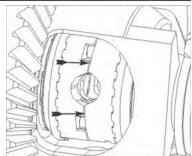
**25.** Wedge both drivers in engagement with couplers. Rotate driver's side wheel forward 1/4 turn to reveal spring slot.
