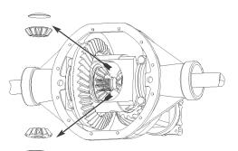
**9.** Remove both spider gears and their thrust washers.
