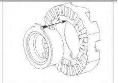
**19.** Insert driver/spacer as shown, making sure spacer paddle is facing out towards you.
