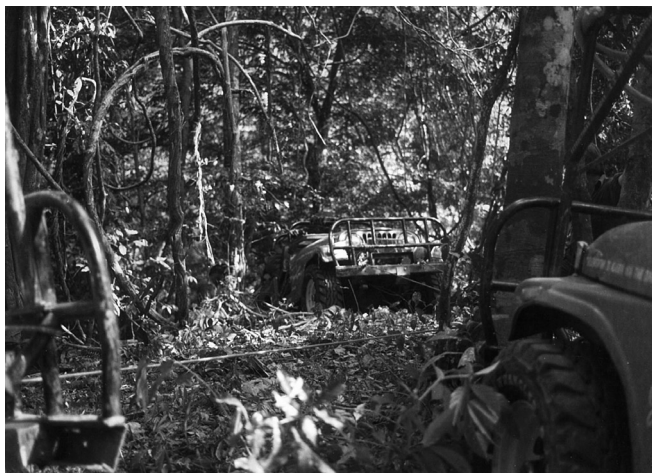
Using two winches to help a Jeep up an 85% hill
