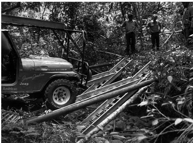
Using bridging ladders for crossing ravines or climbing steep banks
