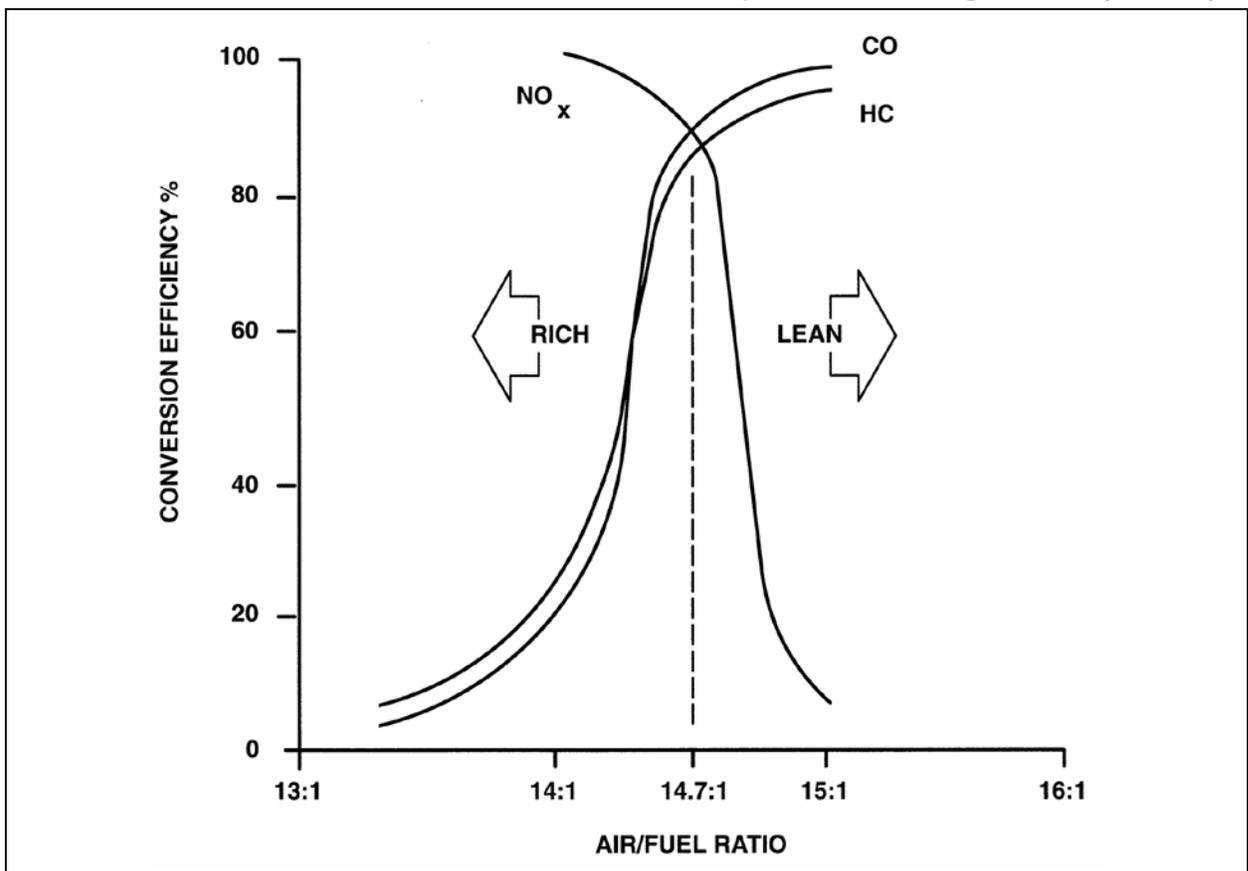
Figure 28 Three-Way Catalyst Conversion Efficiency
