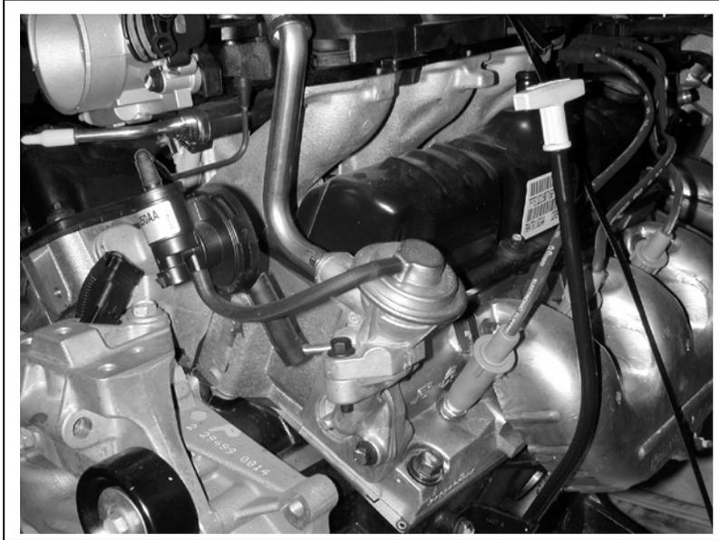
Figure 115 Typical Back Pressure Transducer EGR Valve
