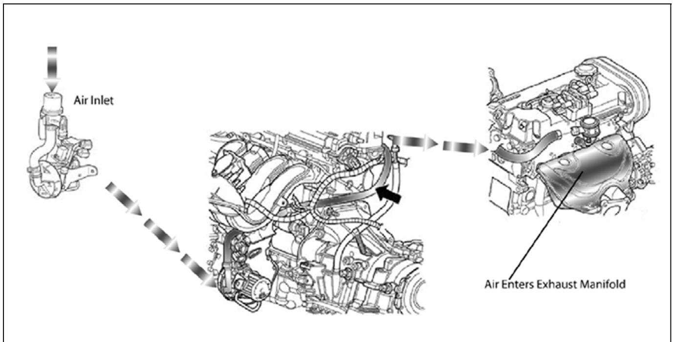
Figure 126 Secondary Air System
