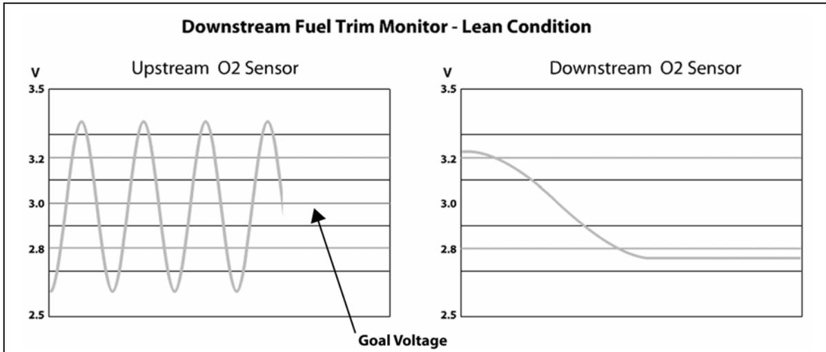
Figure 100 Upstream and Downstream O<sub>2</sub> Sensors – Lean Condition (excess oxygen)
