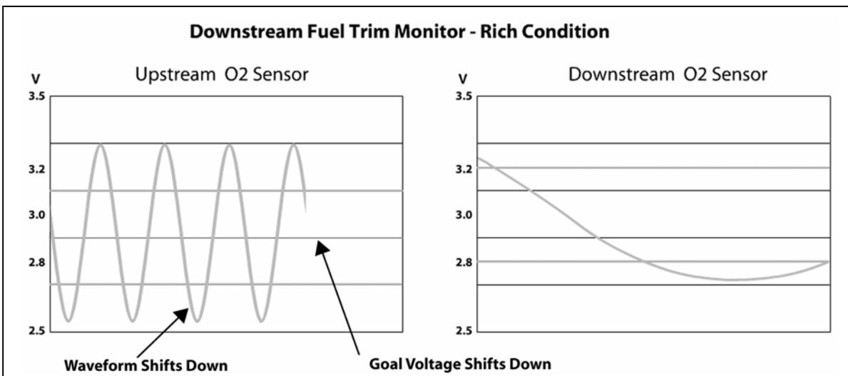
Figure 99 Upstream Goal Voltage Shifts Downward to Increase Oxygen
