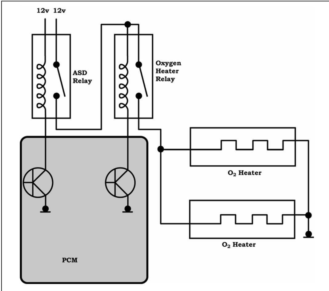
Figure 63 Oxygen Sensor Heater Element – Relay Power/Constant Ground
