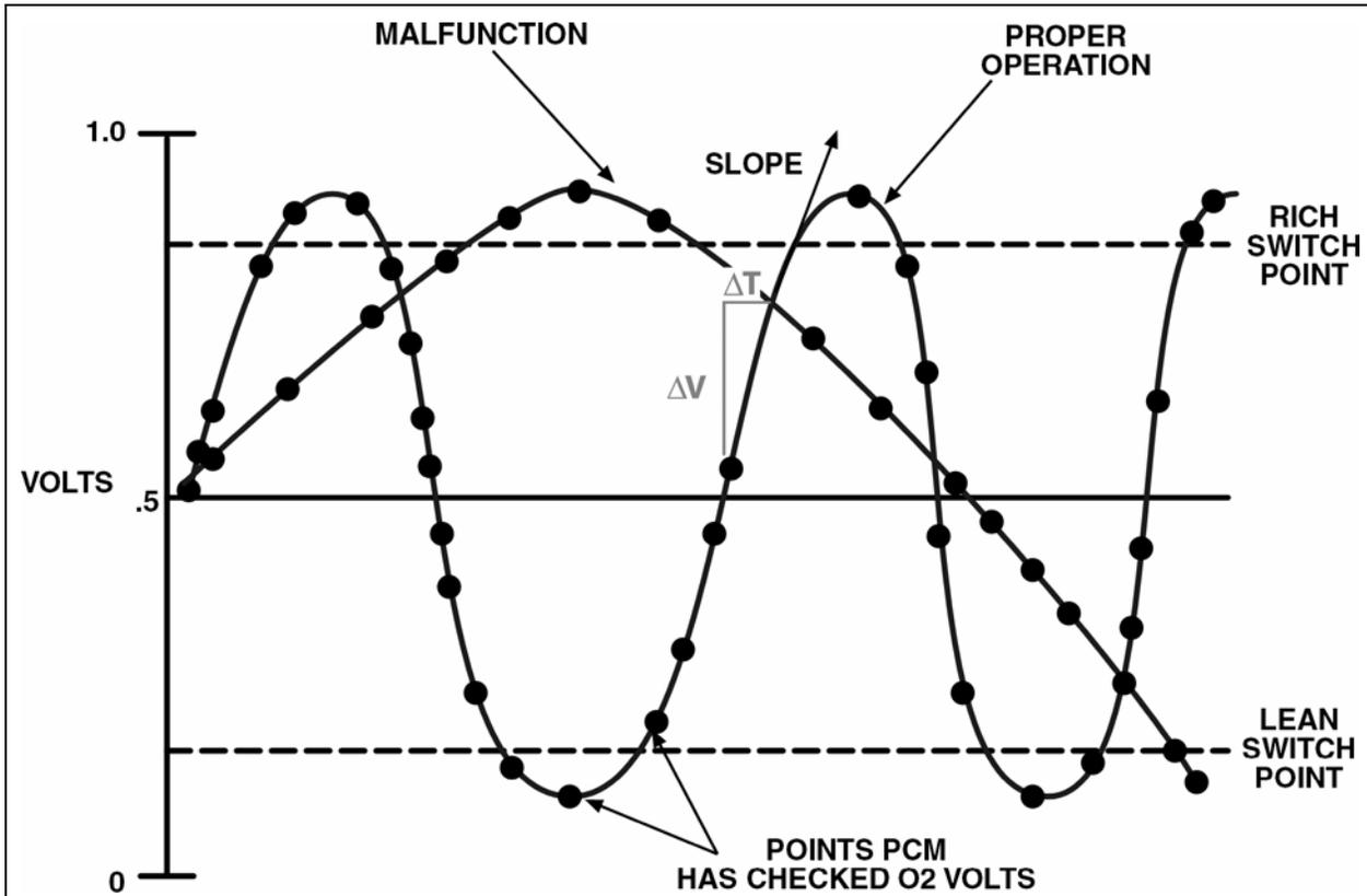
Figure 12 JTEC/SBEC Oxygen Sensor Big Slope
