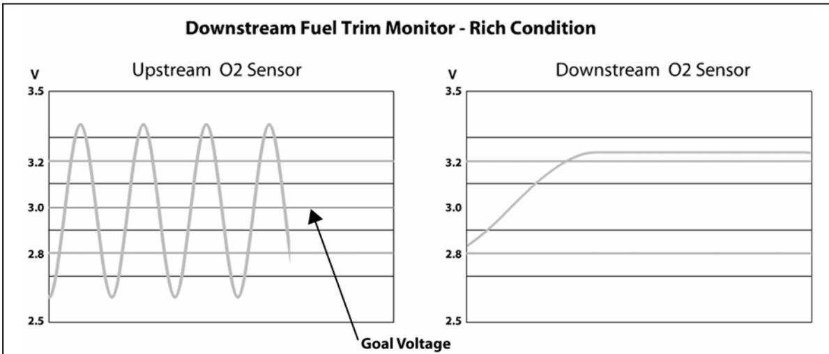
Figure 98 Upstream and Downstream O<sub>2</sub> Sensors – Rich Condition (lack of oxygen)
