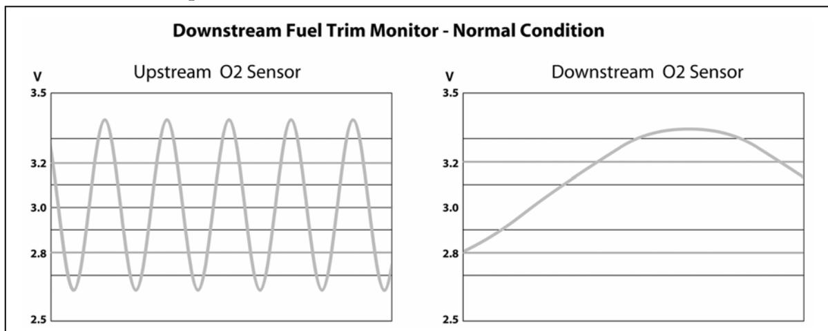
Figure 97 Upstream and Downstream O<sub>2</sub> Sensors Switching Normally
