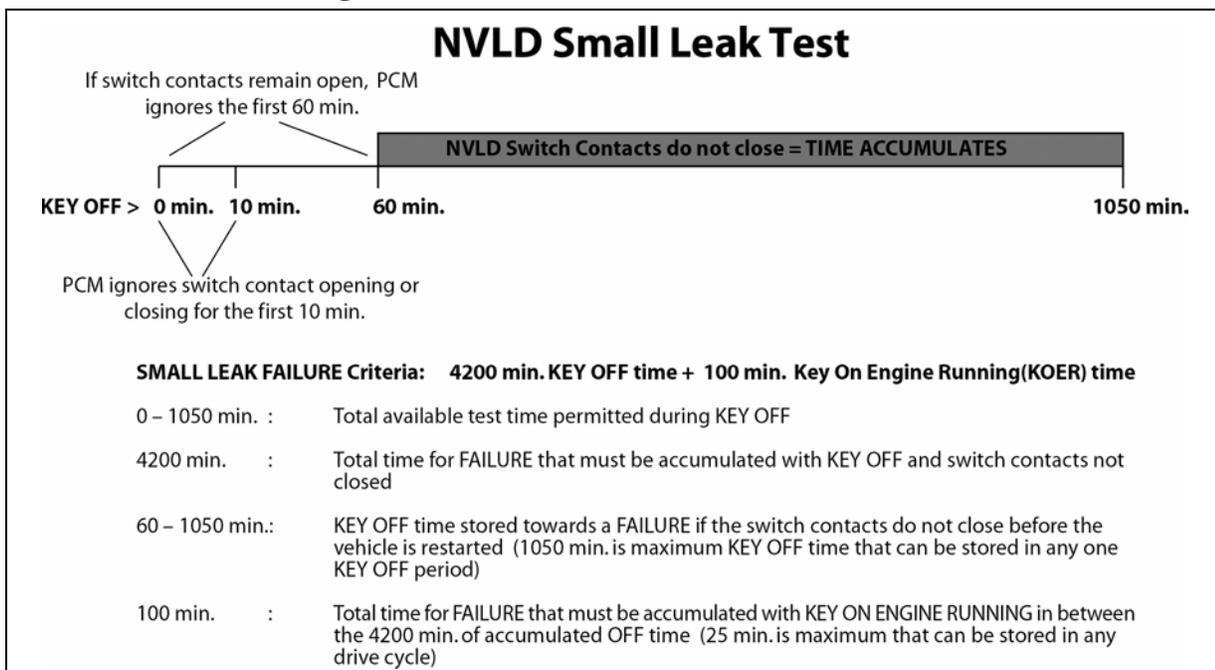
Figure 71 Small Leak Failure Time Thresholds
