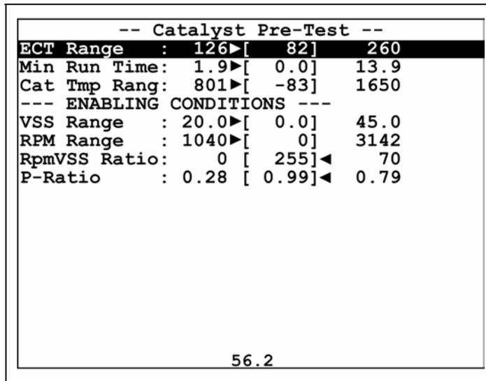
Figure 41 NGC SOC Catalyst Monitor Pretest Screen
