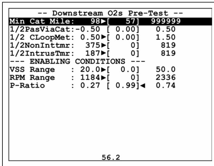
Figure 50 NGC Downstream Oxygen Sensor Monitor Pretest Screen
