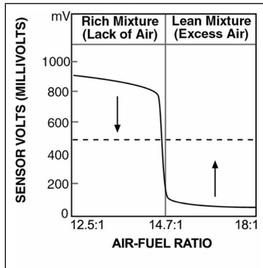
Figure 10 O<sub>2</sub> Sensor Signal
