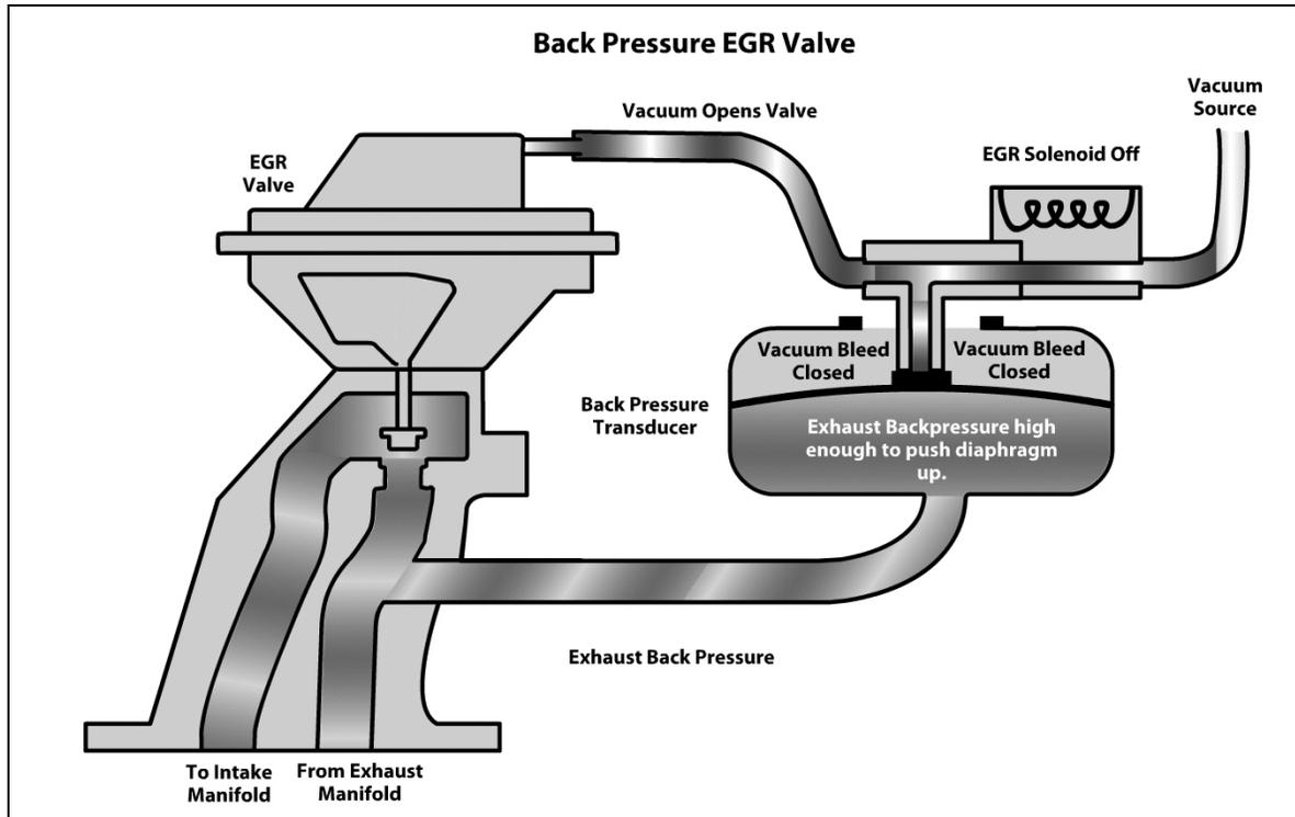
Figure 116 Back Pressure EGR Valve – High Back Pressure
