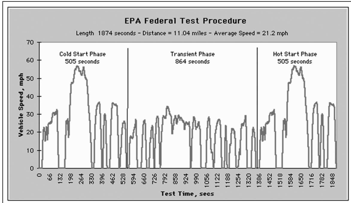
Figure 7 EPA Federal Test Procedure Drive Cycle
