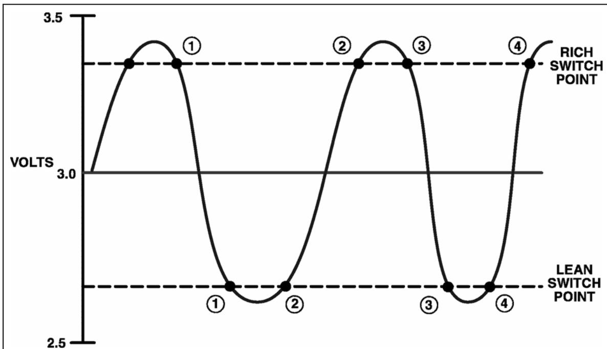
Figure 14 NGC Oxygen Sensor Switch Counts
