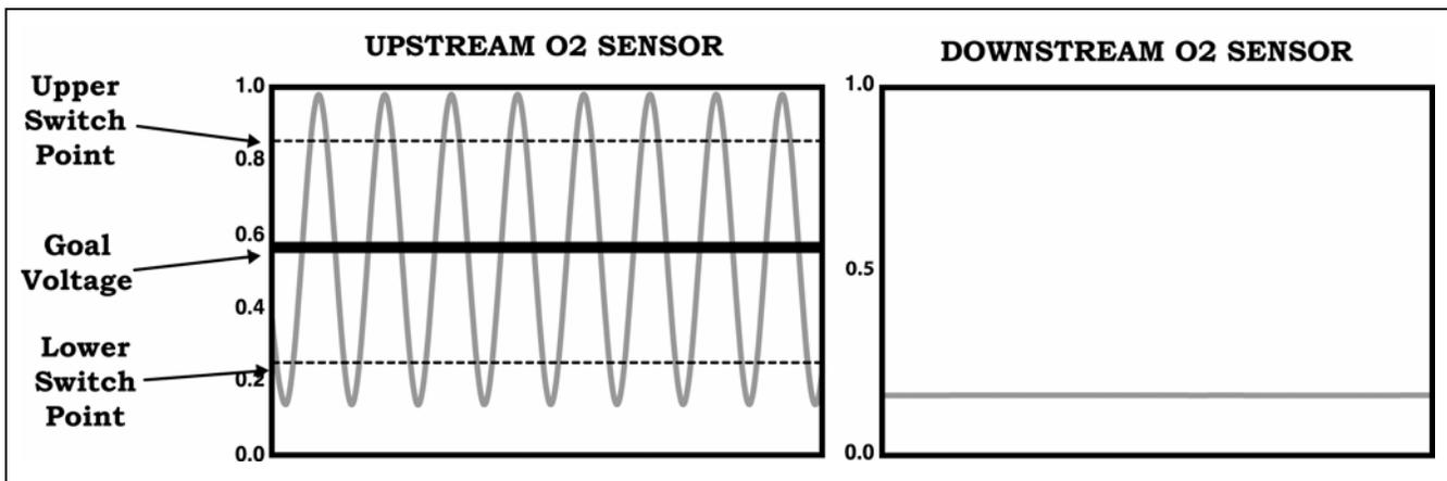
Figure 48 Goal Voltage and Switch Points Shift to Reduce High O<sub>2</sub> Content
