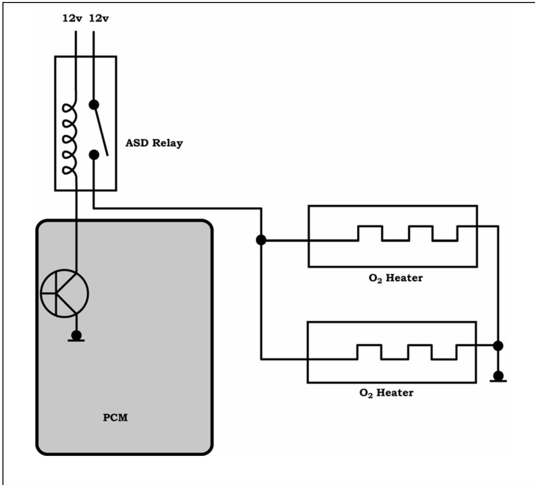
Figure 61 Oxygen Sensor Heater Element – ASD Power/Constant Ground
