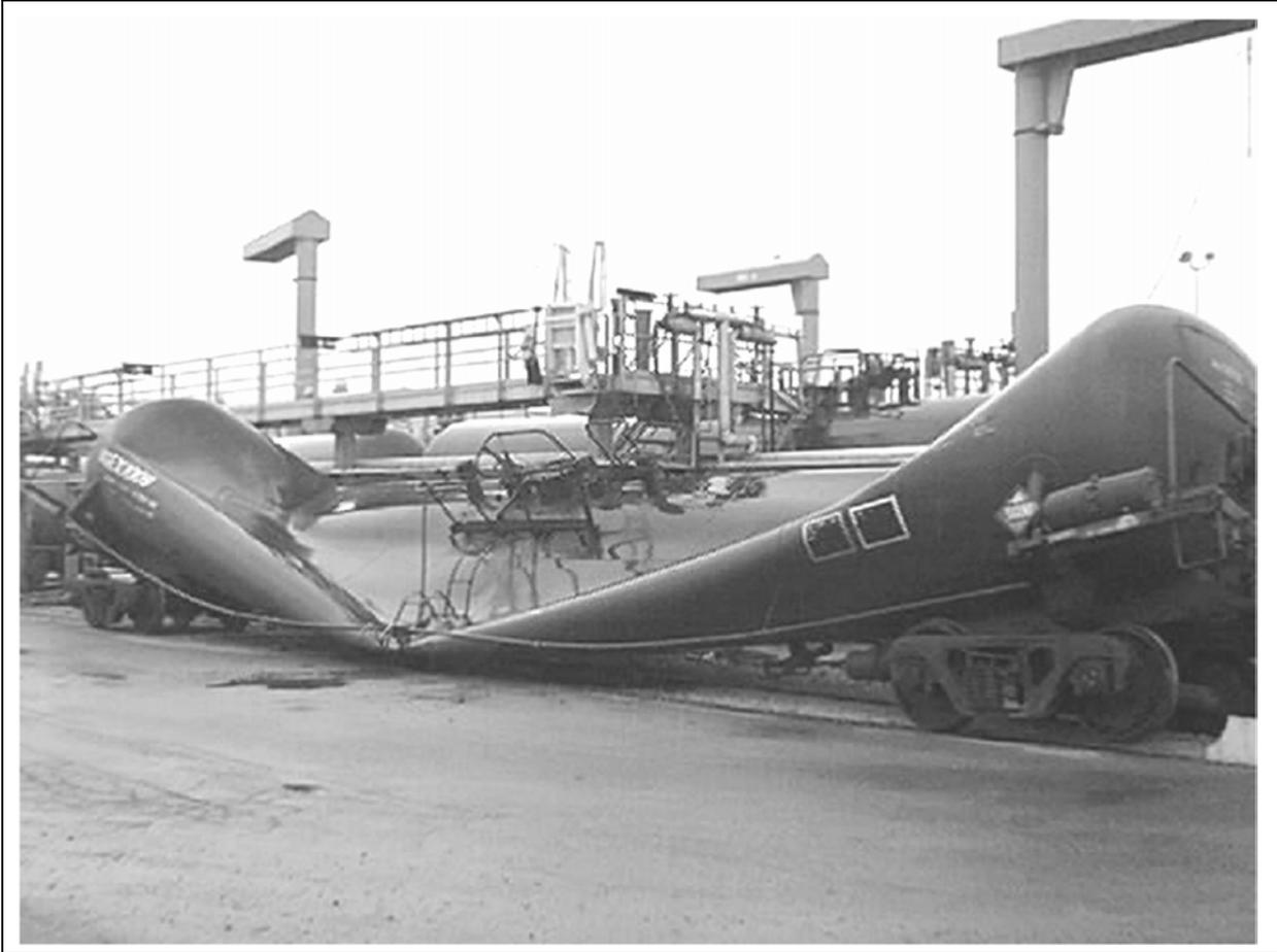
Figure 67 Natural Vacuum Principle Demonstrated
