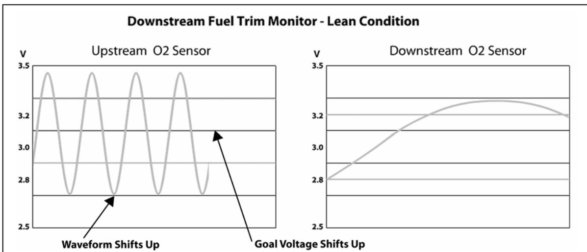
Figure 101 Upstream Goal Voltage Shifts Upward to Decrease Oxygen
