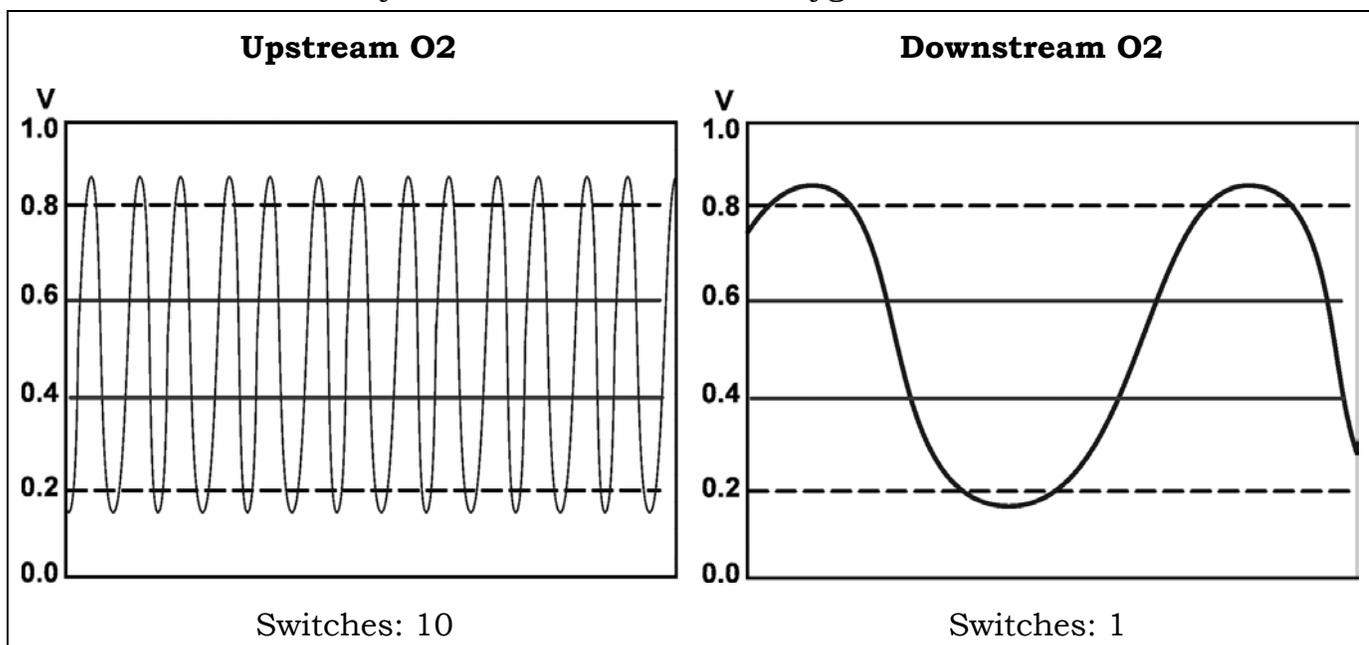
Figure 30 10% Switching Ratio = Good Catalyst
