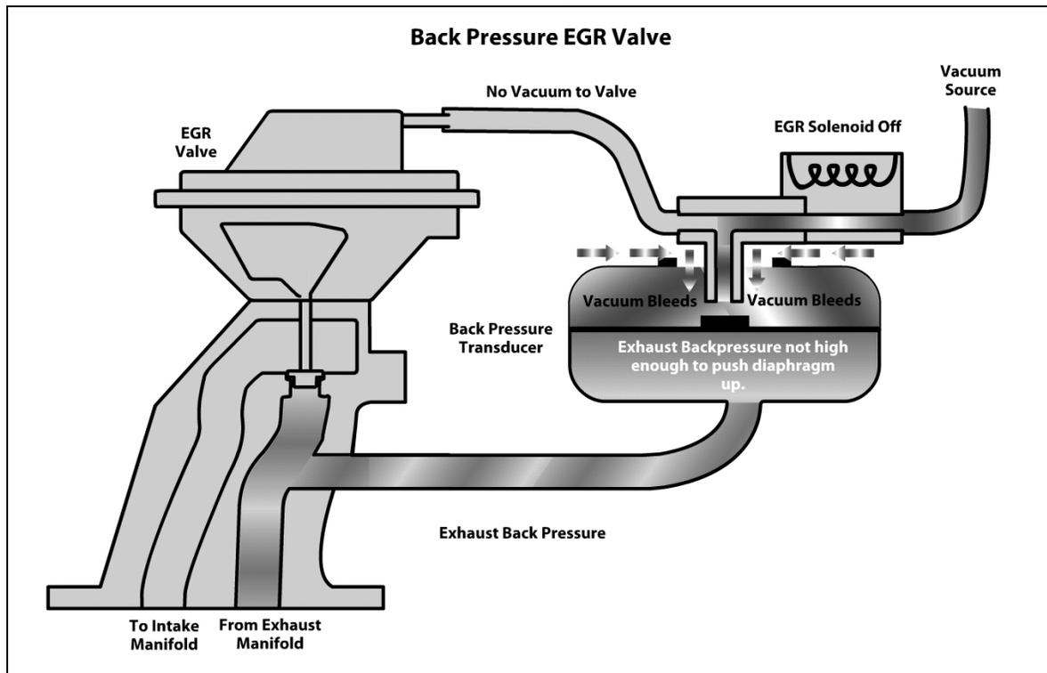
Figure 117 Back Pressure EGR Valve – Low Back Pressure
