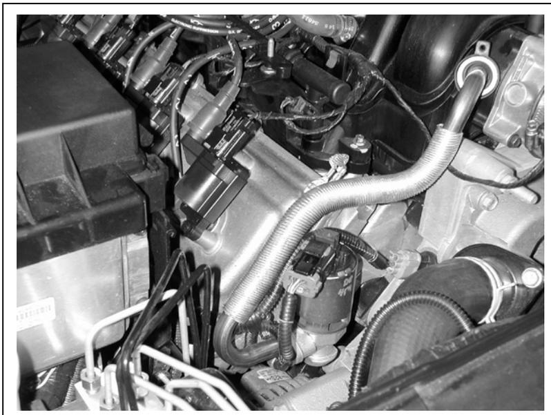
Figure 113 Typical Linear EGR Valve
