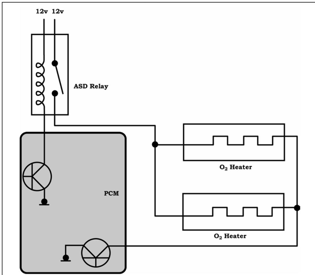
Figure 62 Oxygen Sensor Heater Element – ASD Power/PWM Ground
