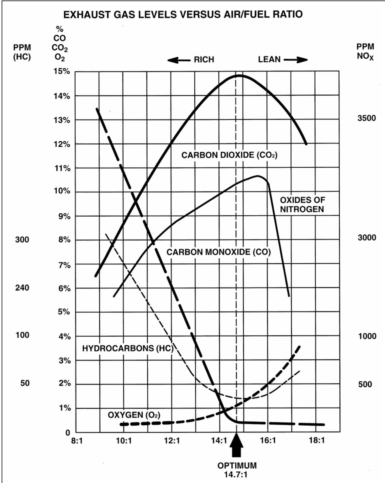
Figure 84 Exhaust Emissions vs. Air/Fuel Ratio
