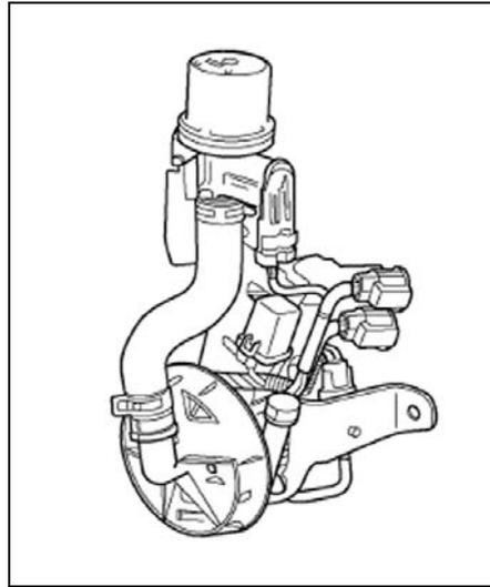
Figure 127 Secondary Air Pump
