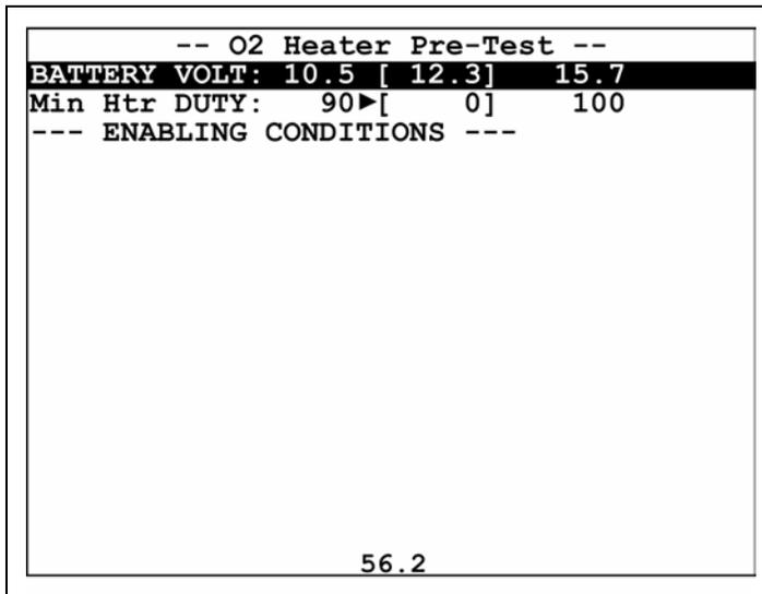
Figure 59 NGC Oxygen Sensor Heater Monitor Pretest Screen
