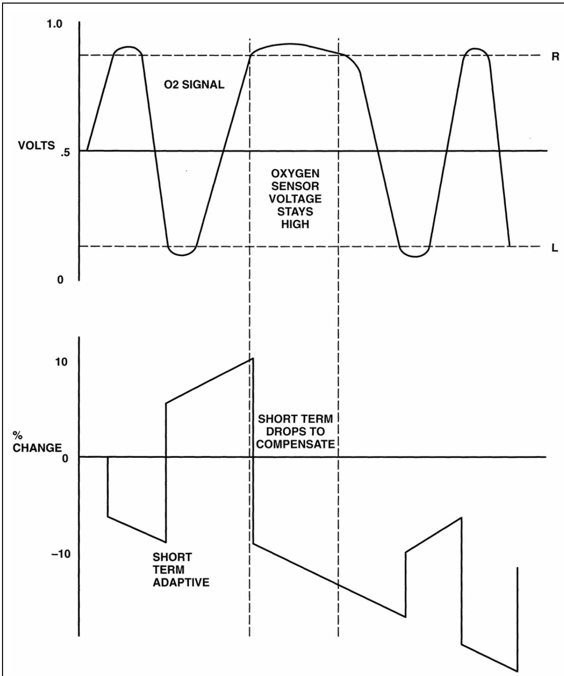
Figure 87 Short Term Adaptive vs. O<sub>2</sub> Sensor Voltage
