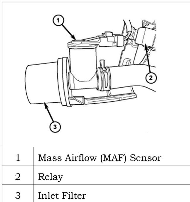
Figure 128 Secondary Air MAF Sensor
