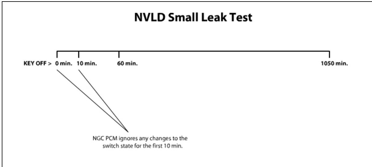
Figure 69 Small Leak Test Main Time Thresholds
