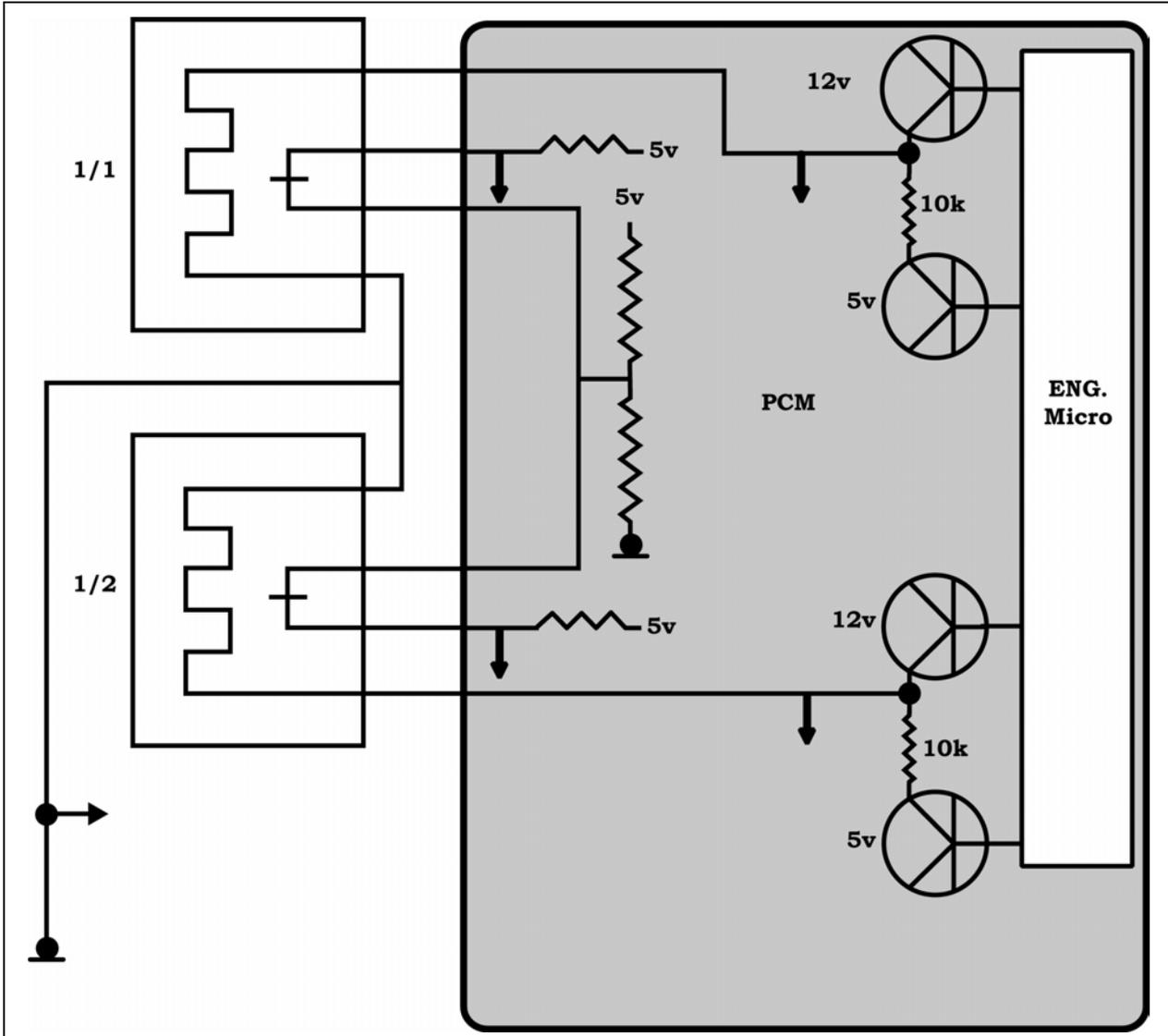
Figure 58 NGC Oxygen Sensor Heater Circuit
