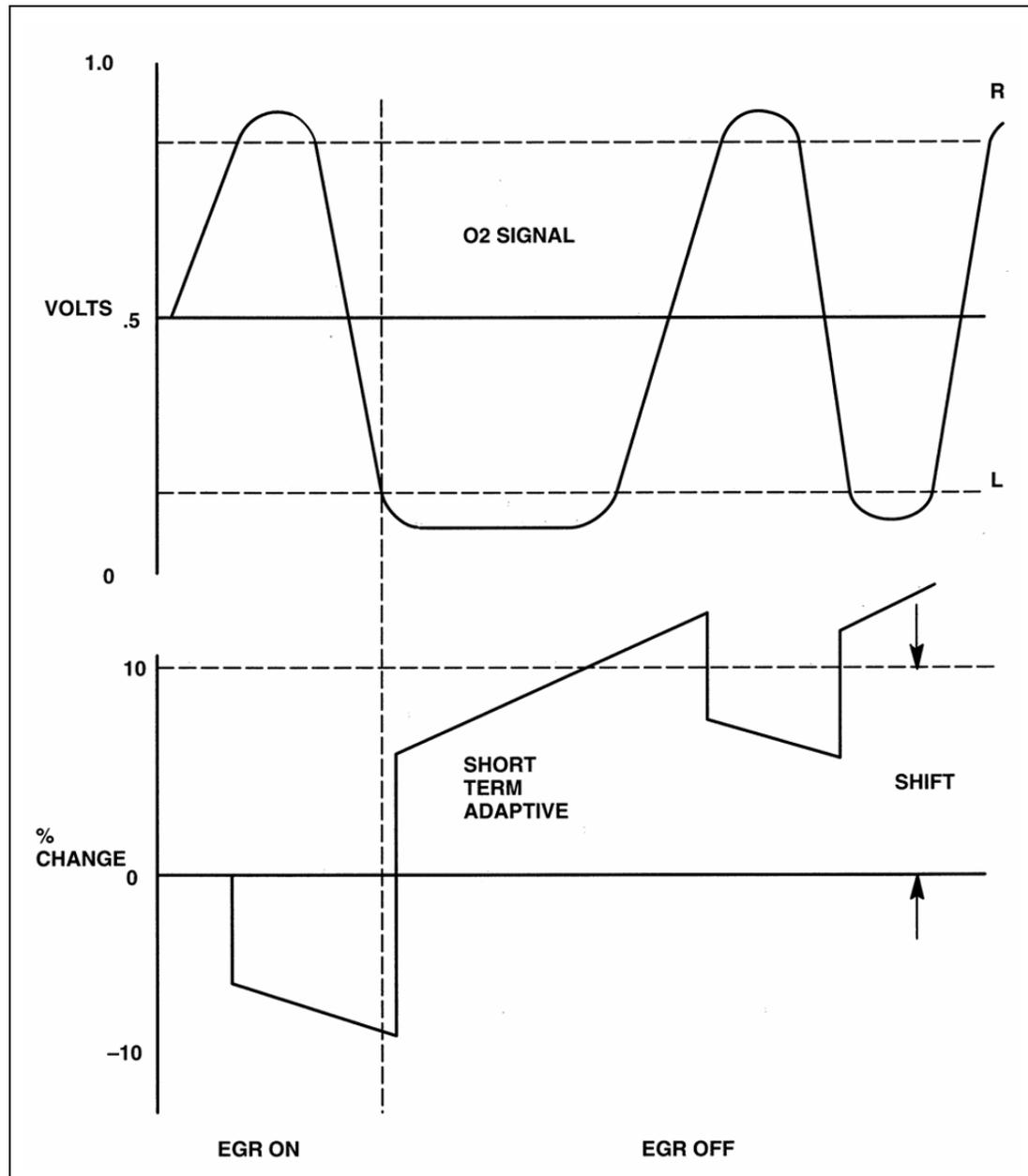
Figure 119 Fuel System Adaptive Shift
