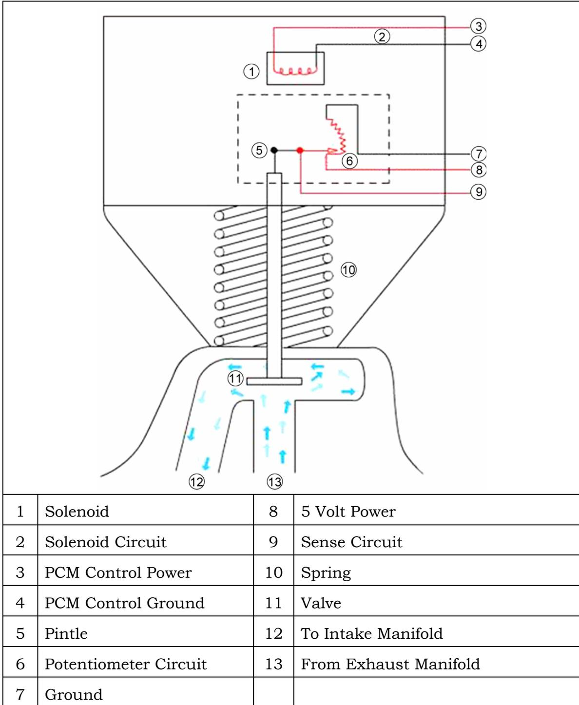
Figure 114 Linear EGR Valve Components
