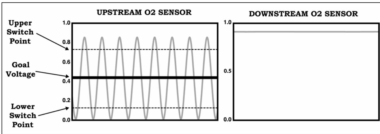
Figure 49 Goal Voltage and Switch Points Shift to Increase Low O<sub>2</sub> Content
