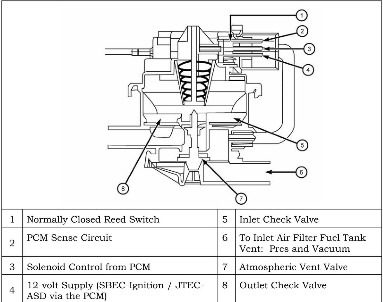
Figure 80 Leak Detection Pump
