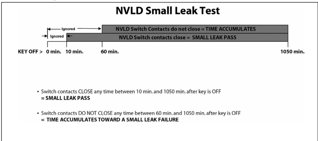
Figure 70 Small Leak Pass or Fail
