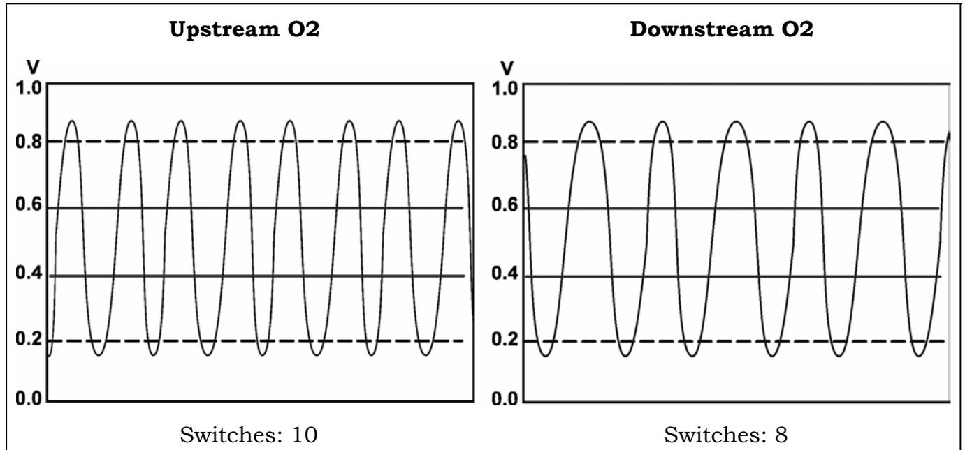
Figure 31 80% Switching Ratio = Failed Catalyst
