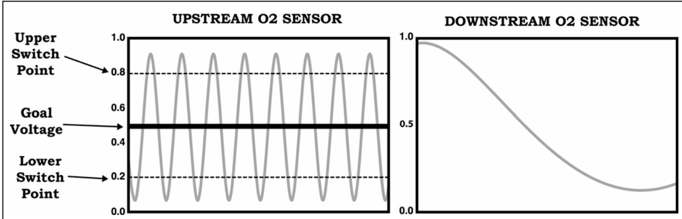
Figure 47 Upstream vs Downstream Oxygen Sensor Waveforms
