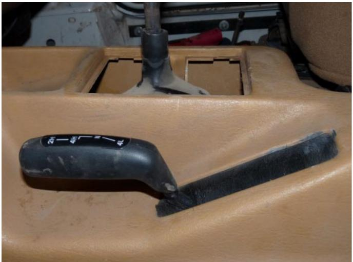
**Installing the NP231 Shifter Assembly**
