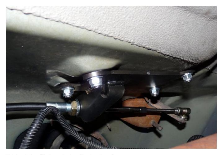
**Cable to Transfer Case Anchor Bracket Attachment**
