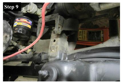
On the passenger side, remove the motor mount through bolt and the motor mount out of the vehicle.
