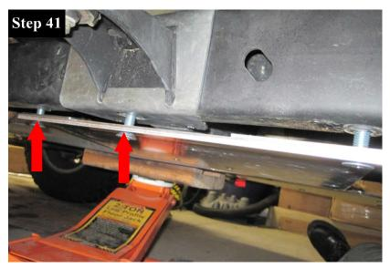
Loosely install the remaining (2) 12mm X 1.75 X 40mm Flat Head Allen Screws and Wing Spacers (D).
