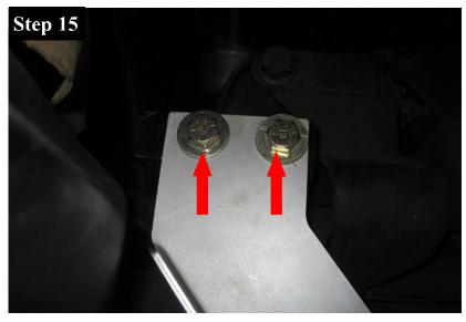
On the passenger side, install and tighten the (2) 3/8 - 16 X 3/4" G8 Zinc Bolts and 3/8 heavy washers.
