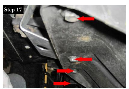
At this point <u>SLOWLY</u> raise the drivetrain at the output shaft of the transfercase so that the transmission studs are clear of the transfercase skid.
