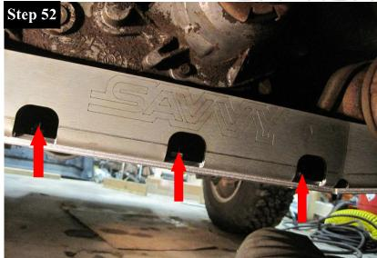
Tighten the (3) 5/16 - 18 X 1" Flat Head Phillips Screws and 5/16 - 18 Flange Nuts.
