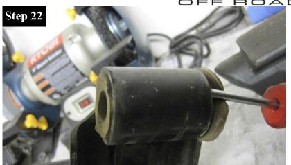
Using a flat head screw driver as a shoehorn, carefully tug the exhaust hanger bushing from the stock transmission mount.
