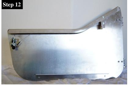
At this point the Left Trail Door is fully assembled and ready for install.
