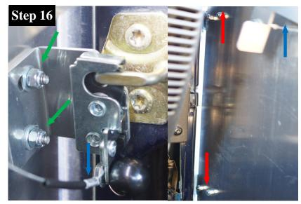
Fully close the Trail Door taking care to adjust the Door Latch to allow closure against the Tub Striker.
