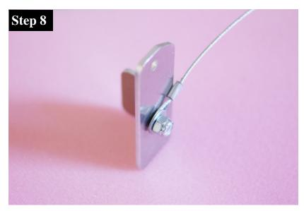
Assemble the Door Cable to the Left Door Handle with (1) 1/4" -  $20 \times 5/8$ " HHCS, (2) 1/4" Washers one on each side of the Door Handle and (1) 1/4" - 20 Nylock Nut.
