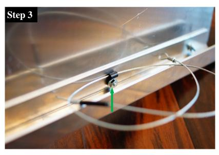
Slip the Door Cable through the Plastic Clip that you previously threaded such that the black plastic sleeve on the cable end loop is near where the door latch will be installed. Install a 10 - 24 x 5/8" Flat Head Philips Screw and 10 - 24 Flange Nut to secure the Door Cable.
