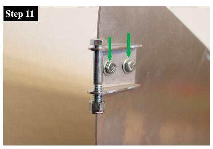
Assemble the Door Hinge to the Door Skin as shown. Note that the 1/4" Washers are below the head of the HHCS on the Door Hinge as shown in the green arrows.
