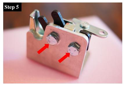
Assemble the Left Door Latch to the Left Door Latch Bracket using (2) 1/4" - 20 x 5/8" HHCS as shown in the red arrows.
