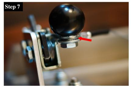
At this point the supplied Door Latch Knob should be installed as shown with the Door Cable between the Washer and Door Latch as illustrated in the red arrow.
