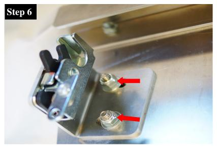
Loosely attach the Left Door Latch Bracket to the Left Door Skin using (2) 1/4" - 20 x 3/4 SHBS. The (2) 1/4" Washers and (2) 1/4" - 20 Nylock Nuts should be fastened such that the 1/4" Washers are on the Left Door Latch Bracket as shown.
