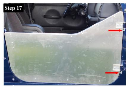
Now tighten the 3/8" - 16 Nylock Nuts that secure the Door Hinges to the Tub.
