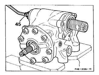
13 Tighten pitman arm shaft/bearing cover (51) with new self-locking bolts (59), (30-35 Nm).
