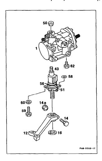
Steering gear (1) ...... mount on assembly support 140 589 00 59 00 with two screws and clamp in vise (number 1).
