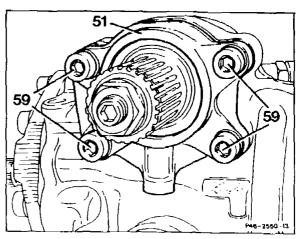
7 Unscrew collar nut from adjusting screw, holding adjusting screw tight.
