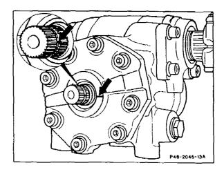
6 Unscrew self-locking bolts (59) for attaching pitman arm shaft/bearing cover (51).
