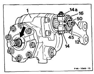
5 Pull pitman arm (12) off the pitman arm shaft, use puller 000 589 88 33 00, if necessary.
