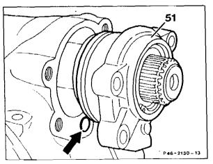
12 Screw adjusting screw (45) into the steering gear housing far enough for it to make contact. Unscrew center position inspection bolt and fit screw plug with new seal (35–40 Nm).
