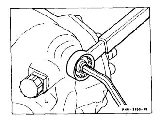
8 With steering in center position, turn adjusting screw clockwise; this causes the pitman arm shaft (43) to be pressed out of the steering gear housing together with the bearing cover/pitman arm shaft (51).
