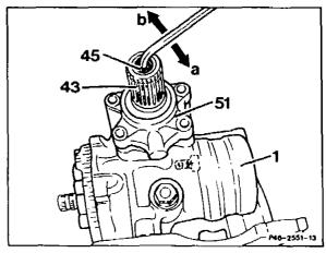
16 Tighten pitman arm shaft/bearing cover (51) with new self-locking bolts (59) Tightening torque 30–35 Nm.
