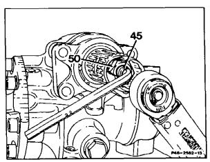
20 Clean shaft spline of the pitman arm shaft and pitman arm (12). Both parts must be free of oil and grease.
