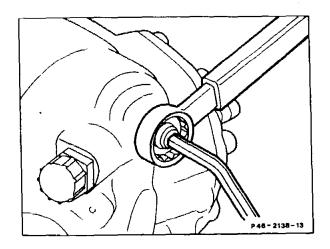
17 Clean shaft spline on the pitman arm shaft and on the pitman arm (12). Both parts must be free of oil and grease.
