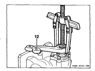
5 Turn steering gear into center position by unscrewing bolt (62) and screwing in center position inspection bolt 201 589 06 21 00.
