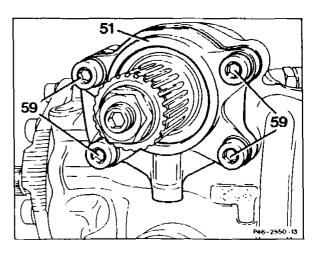
17 Test and adjust friction torque of the steering gear (46-0120).
