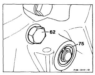
Position steering gear with external centering (as of 1/90) to mark (arrows).
