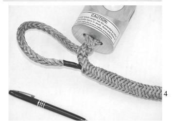
When most of the tail has been inserted into the main line, pull the taped end out through the side of the compressed main line.
