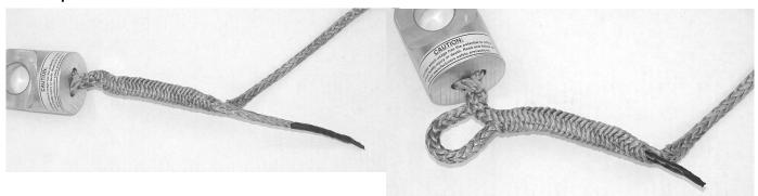
Remove the tape; slide the compressed line back down over the tail as far as possible. If done correctly, you should only have 1-2 inches of the tail sticking out of the side of the main line. If you have more, remove the tail, compress more of the main line around the ink pen and repeat.
