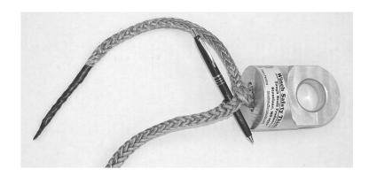
Thread the tail through this hole and pull it tight.
