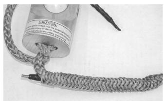
Slide the taped tail into this hole (keep the main line compressed).
