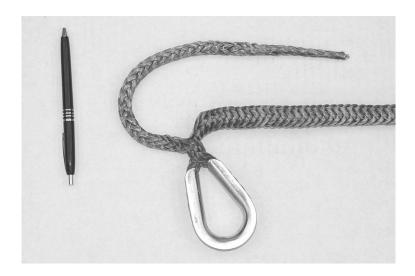
Next, pull the main line back through the tail; you must pull the entire length of the main line through.
